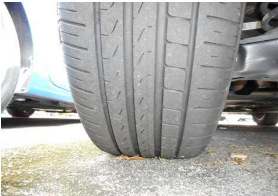
Photo 9 shows the condition of the rear left tyre of the Motor Car, which was observed to be in serviceable condition with remaining tread depth of approximately 4.5mm. The tyre, which was wrapped around alloy wheel rim, was also observed to be sufficiently inflated for vehicular operation. The 4 tyres of the Motor Car were wrapped around standard alloy wheel rims.
