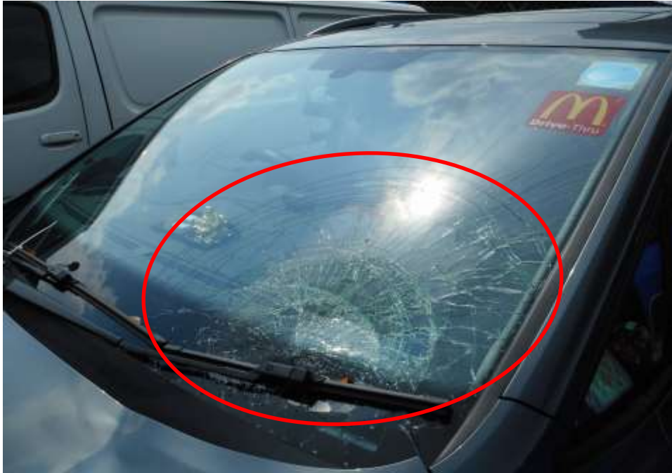
Photo 2 shows the close up view of the Motor Car's front body at the time of my inspection. The Motor Car was observed to have sustained damage at its front windscreen (circled) as a result of the accident.
