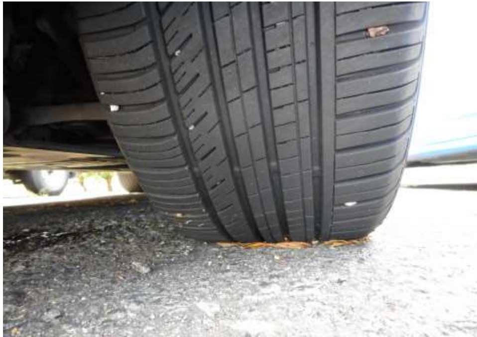
Photo 10 shows the condition of the front left tyre of the Motor Car, which was observed to be in serviceable condition with remaining tread depth of approximately 6.7mm. There was also no tear, cut or burst mark(s) on the outer and the inner sidewalls as well as across the tread of the Motor Car's 4 tyres.
