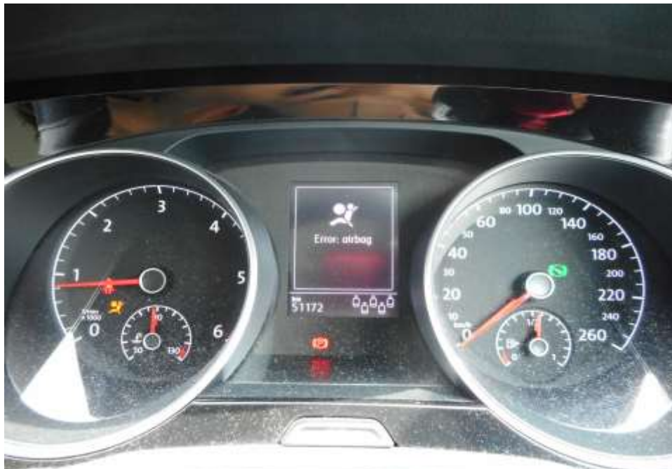
Photo 24 shows the Supplemental Restraint System (SRS) warning lights illuminated on with an error warning message on the instrument panel of the Motor Car after the engine was cranked as a result of the accident. However the other warning light disappeared after cranking, this would suggest that there was no abnormality to the various electronic operating systems of the Motor Car, like the ABS, EPS and TC etc.
