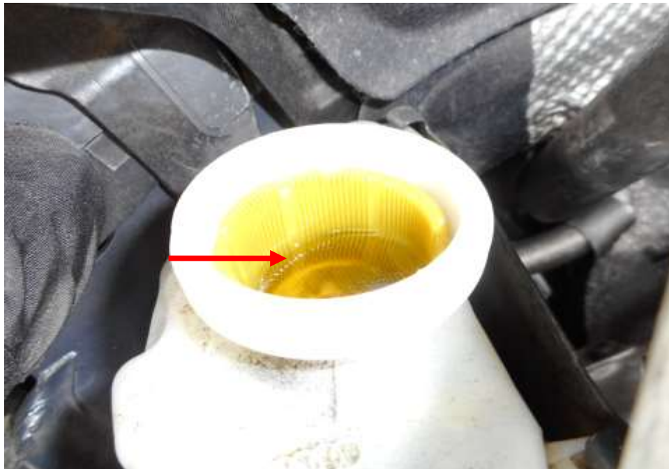
Photo 12 shows the brake fluid reservoir of the Motor Car at the time of my inspection. The brake fluid was observed to be of sufficient level (arrowed) and without any visible contamination.
