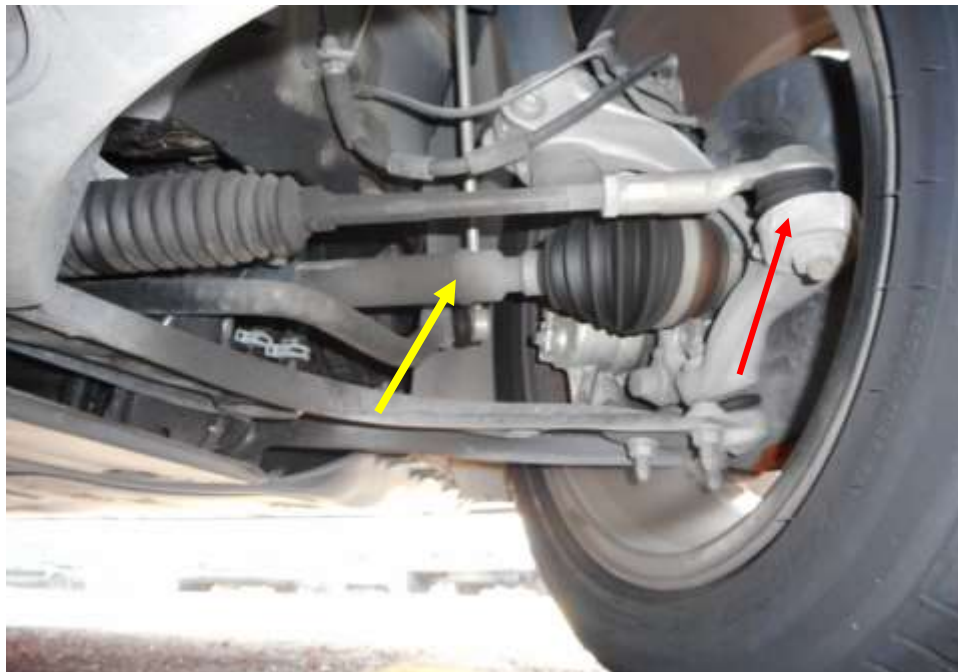
Photo 21 shows the various undercarriage components at the front right wheel of the Motor Car, in particular the steering tie rod (red arrow) and drive shaft (yellow arrow). The various steering components were all found to be intact, suggesting that the steering system of the Motor Car was likely to be in serviceable condition at the material time of accident. There was also no sign of fluid stain observed on the various undercarriage components at the front right wheel of the Motor Car.
