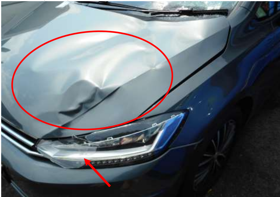
Photo 3 shows the close up view of the Motor Car's front body at the time of my inspection. The Motor Car was observed to have sustained damage at its front bonnet (circled) and left headlamp (arrowed) as a result of the accident.
