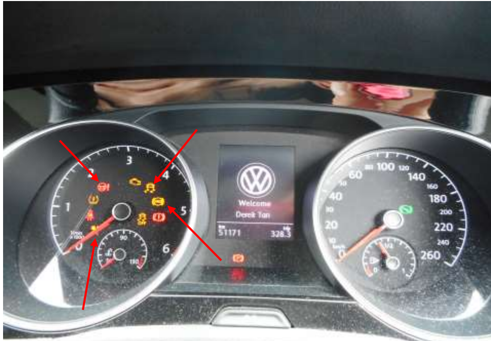
Photo 23 shows the warning light for Anti-Lock Brake System (ABS) Traction Control System (TC), Electric Power Steering System (EPS) and Supplemental Restraint System (SRS) appearing on the instrument panel of the Motor Car during the self-test of its various electronic operating systems when its engine was cranked.
