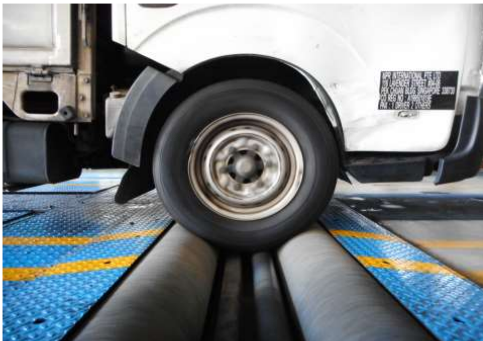
Photo 28 shows the Motor Lorry front right wheel on the roller brake test machine upon testing process. The purpose is to test the braking efficiency of the Motor lorry's braking system at the point of accident.
