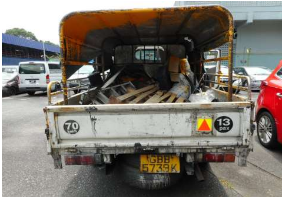
Photo 7 shows a general view of the rear portion body of the Motor Lorry at the time of my inspection. Its rear was observed to be intact and unaffected by the accident.
