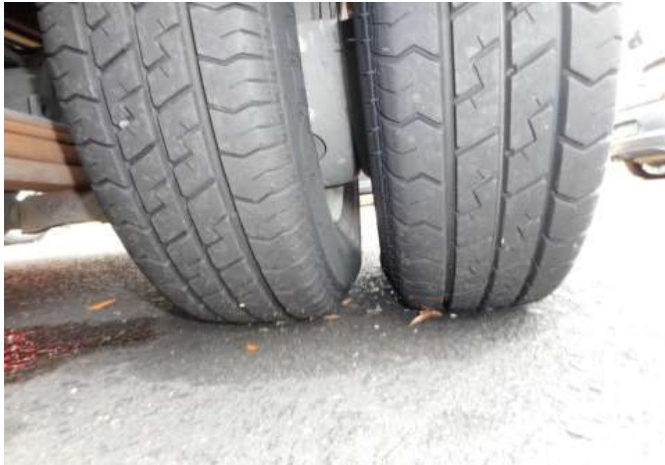
Photo 10 shows the condition of the rear left tyres of the Motor Lorry, which was observed to be in serviceable condition with remaining tread depth of approximately 7.3mm. The tyres, which were wrapped around standard steel wheel rim, were also observed to be sufficiently inflated for vehicular operation. There was also no damage found on all 6 steel wheel rims of the Motor Lorry.
