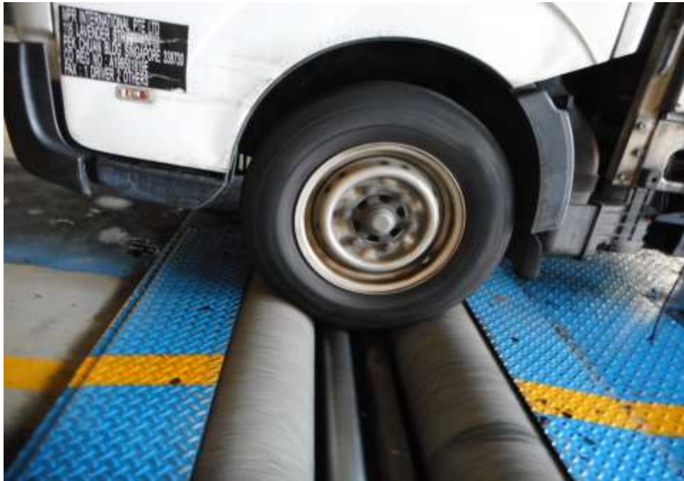
Photo 29 shows the Motor Lorry front left wheel on the roller brake test machine upon testing process. The purpose is to test the braking efficiency of the Motor lorry's braking system at the point of accident.
