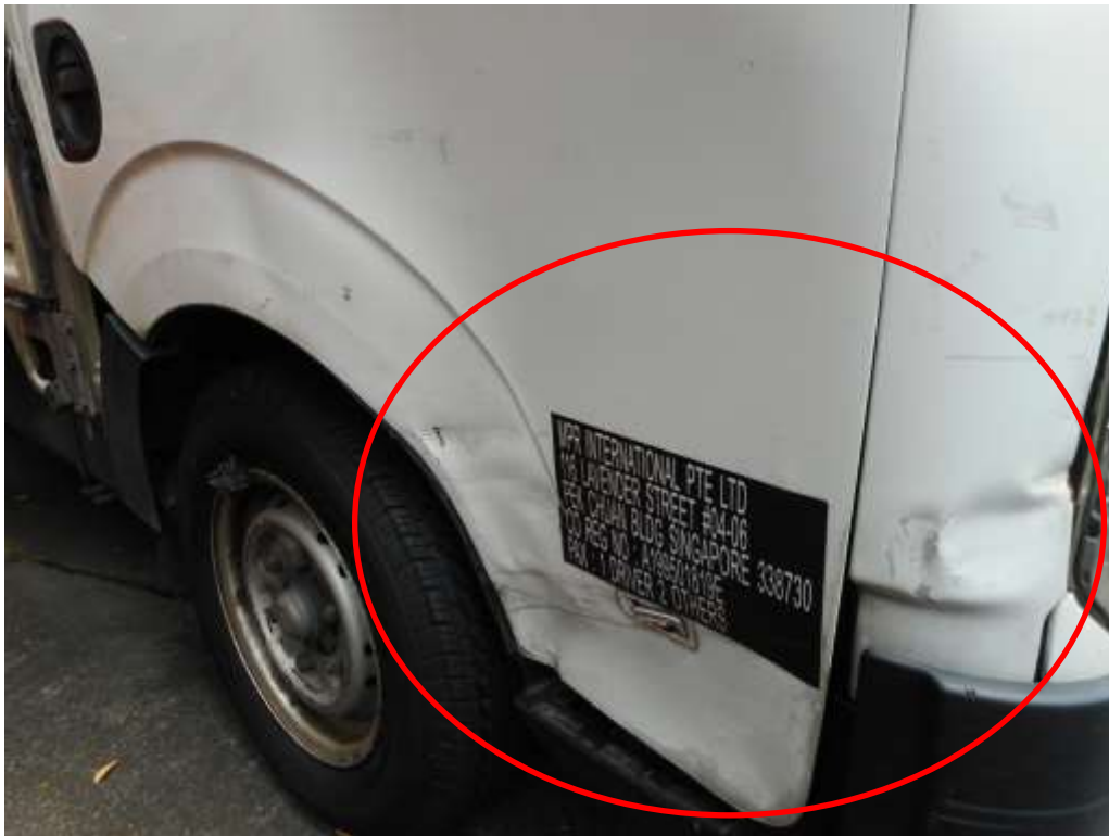
Photo 5 shows a close up view of the front portion of the Motor Lorry at the time of my inspection. Its right door panel was damage as a result of the accident at the time of my inspection.
