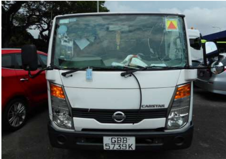
Photo 2 shows a general view of the Motor Lorry's front portion at the time of my inspection. Its front windscreen, front right headlamp, left and right door panel were damage as a result of the accident at the time of my inspection
