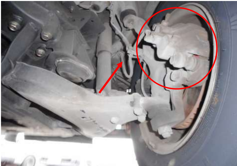
Photo 21 shows the brake hose/pipe (arrowed) at the front right wheel of the Motor Lorry. No leakage of brake fluid was observed. Visual examination of the various components of the braking system like the brake caliper (circled), brake booster, brake pedal etc had revealed all to be intact and without visible damage at the time of accident. There was also no sign of fluid stain(s) observed on the various undercarriage components.
