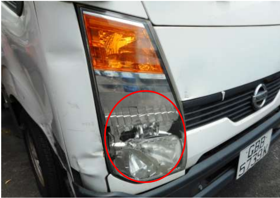
Photo 4 shows a close up view of the front portion of the Motor Lorry at the time of my inspection. Its front right headlamp was damage as a result of the accident at the time of my inspection.
