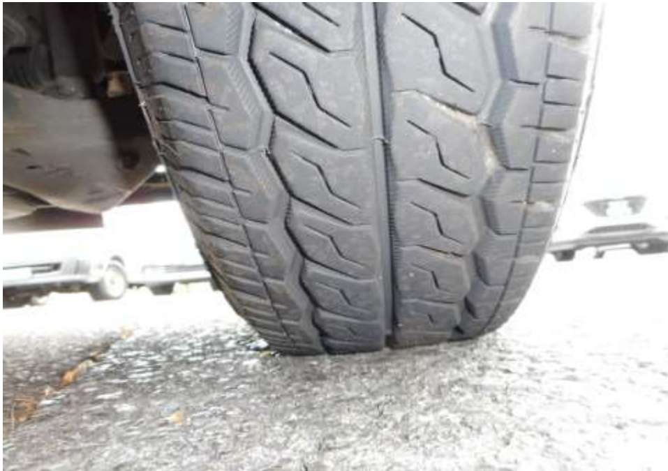
Photo 8 shows the condition of the front right tyre of the Motor Lorry, which was observed to be in serviceable condition with remaining tread depth of approximately 7.6mm. The tyre, which was wrapped around standard steel wheel rim, was also observed to be sufficiently inflated for vehicular operation. There was no tear, cut or burst mark(s) on the outer and the inner sidewalls as well as across the tread of the 6 tyres that were fitted on the Motor Lorry.
