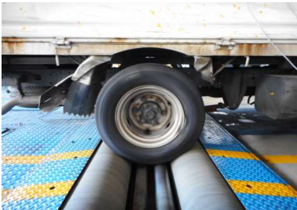
Photo 30 shows the Motor Lorry rear right wheel on the roller brake test machine upon testing process. The purpose is to test the braking efficiency of the Motor lorry's braking system at the point of accident.
