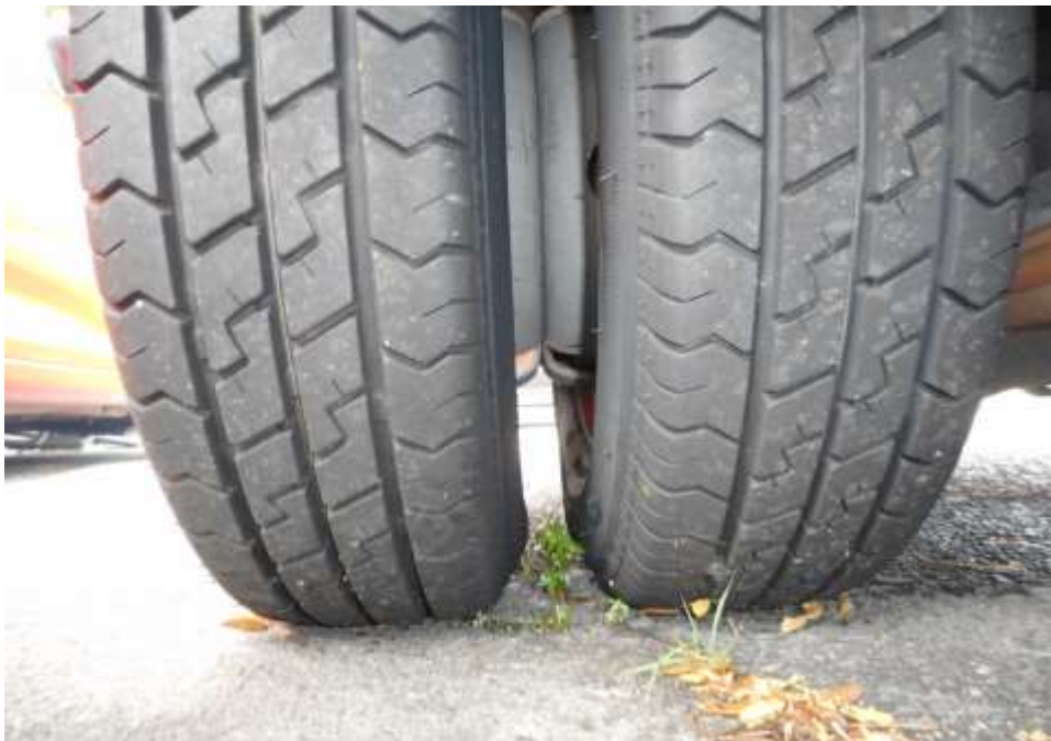
Photo 9 shows the condition of the rear right tyre of the Motor Lorry, which was observed to be in serviceable condition with remaining tread depth of approximately 7mm. The tyre, which was wrapped around standard steel wheel rim, was also observed to be sufficiently inflated for vehicular operation.
