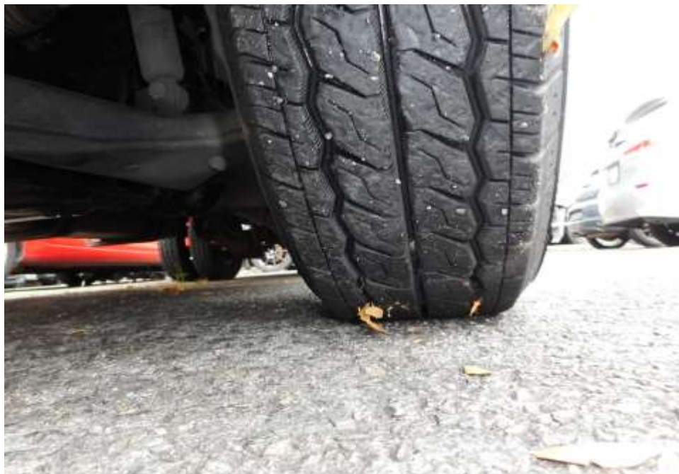
Photo 11 shows the condition of the rear right tyres of the Motor Lorry, which were observed to be in serviceable condition with remaining tread depth of approximately 7.7mm. There was also no tear, cut or burst mark(s) on the outer and the inner sidewalls as well as across the tread of the 6 tyres that were fitted on the Motor Lorry.
