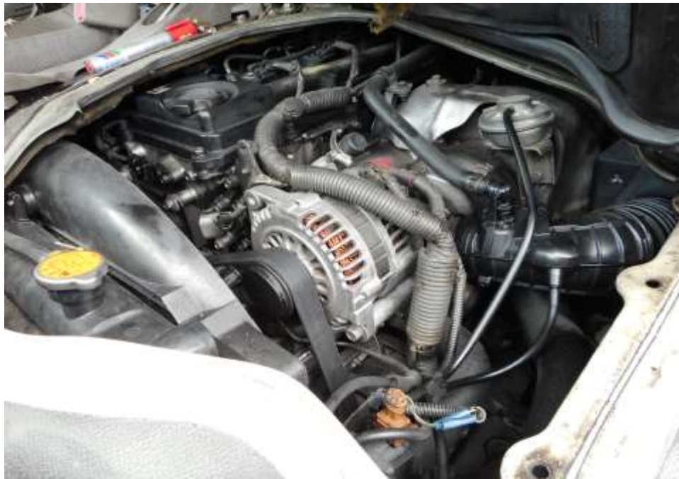
Photo 12 shows a general view of the Motor Lorry's engine compartment, which was accessed by lifting the front cabin of the Motor Lorry. The various parts and components inside the engine compartment were unaffected by the accident. There was also no sign(s) or indication(s) of fresh fluid leakage and/or fluid stain within the engine compartment (photograph shows the engine compartment as viewed from the right front side of the Motor Lorry).
