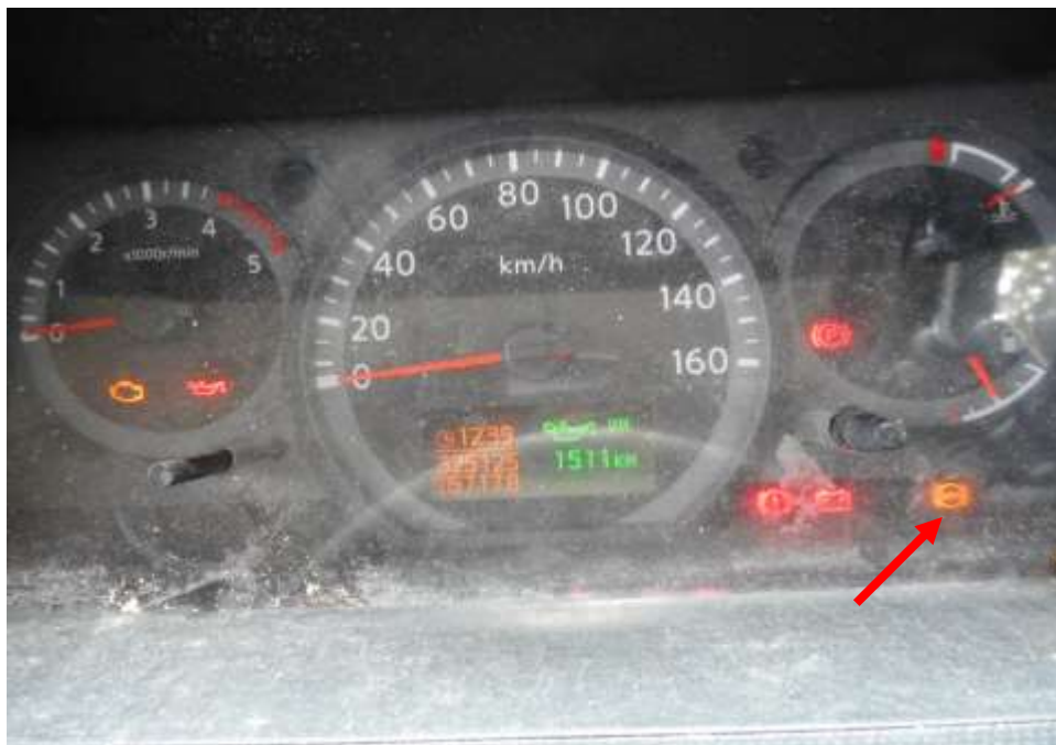
Photo 24 shows the warning light for Anti-Lock Brake System (ABS) (arrowed) appearing on the instrument panel of the Motor Lorry during the self-test of its various electronic operating system when its engine was cranked.
