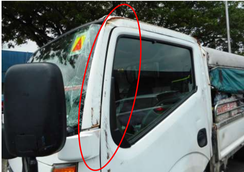
Photo 6 shows a general view of the left portion body of the Motor Lorry at the time of my inspection. Its left door panel was observed to be intact and unaffected by the accident.
