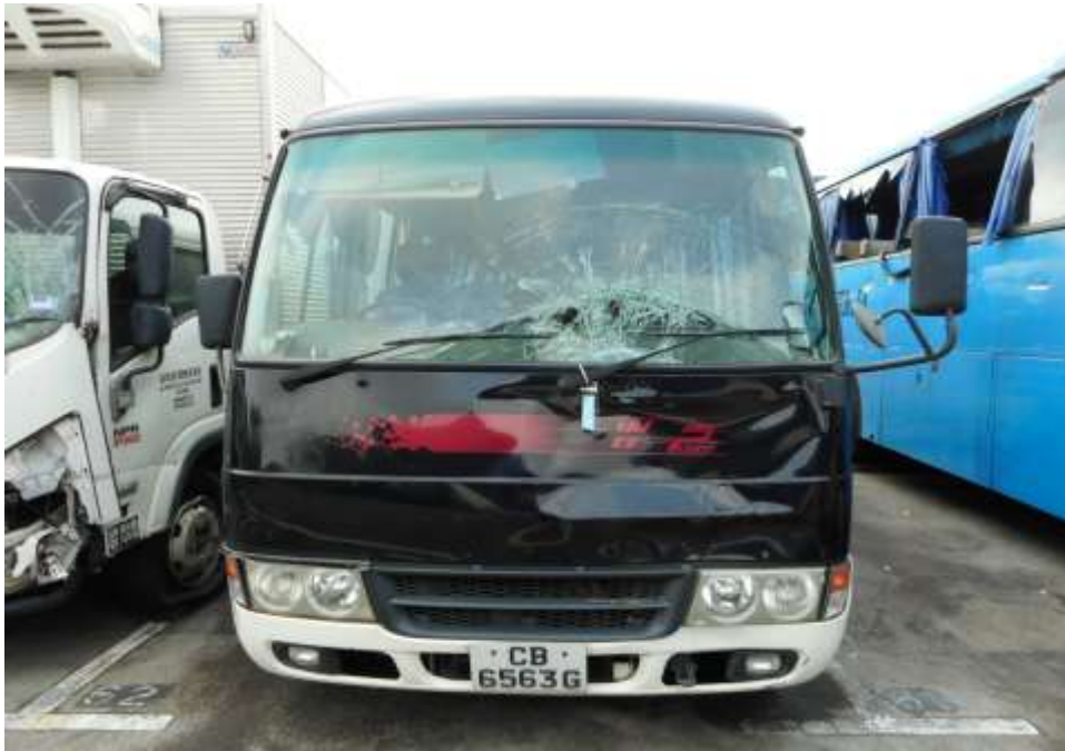
Photo 2 shows a general view of the frontal portion of the Motor Bus at the time of my inspection. The Motor Bus was observed to have sustained moderate damages at its frontal portion. Its front windscreen and front body panel was damaged as a result of the accident at the time of my inspection.
