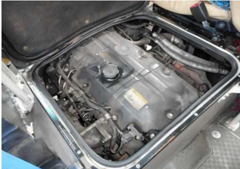
Photo 11 shows a general view of the Motor Bus's engine compartment, which was accessed in front cabin of the Motor Bus. The various parts and components inside the engine compartment were unaffected by the accident. There was also no sign(s) or indication(s) of fresh fluid leakage and/or fluid stain within the engine compartment
