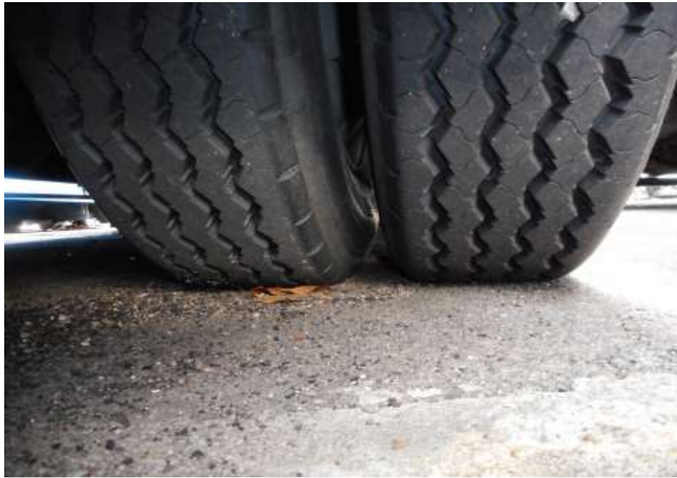
Photo 8 shows the condition of the rear right tyre of the Motor Bus, which was observed to be in serviceable condition with remaining tread depth of approximately 12.1mm. The tyre, which was wrapped around standard steel wheel rim, was also observed to be sufficiently inflated for vehicular operation.
