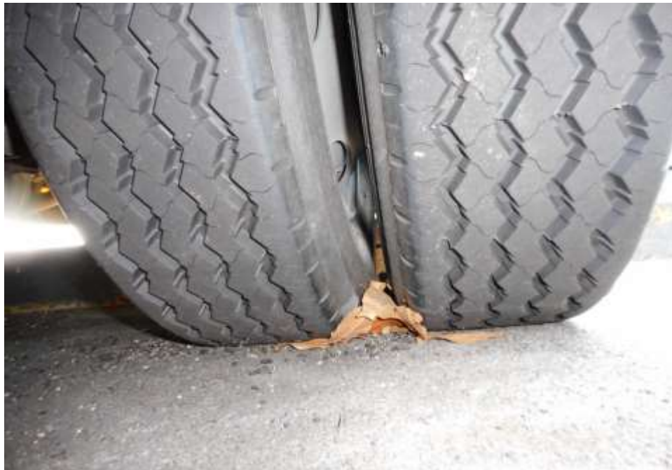
Photo 9 shows the condition of the rear left tyres of the Motor Bus, which was observed to be in serviceable condition with remaining tread depth of approximately 11.9mm. The tyres, which were wrapped around standard steel wheel rim, were also observed to be sufficiently inflated for vehicular operation. There was also no damage found on all 6 steel wheel rims of the Motor Bus.
