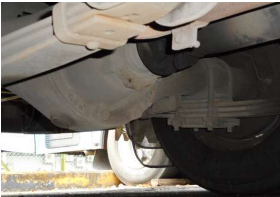
Photo 23 shows the undercarriage of the Motor Bus, at the area where the driveshaft housing is located. We observed it to be intact without any visible damage. There was also no sign of fluid stain(s) observed on the various undercarriage components.
