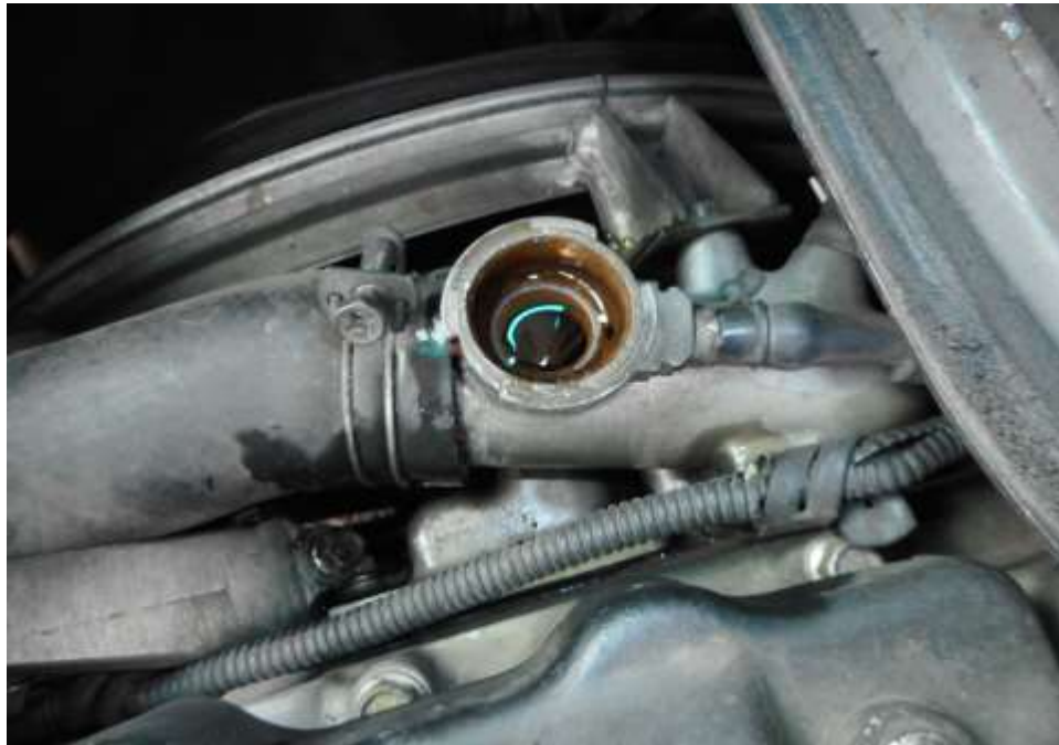
Photo 13 shows the engine coolant reservoir of the Motor Bus at the time of my inspection. The engine coolant was observed to be of sufficient level and without any visible contamination.
