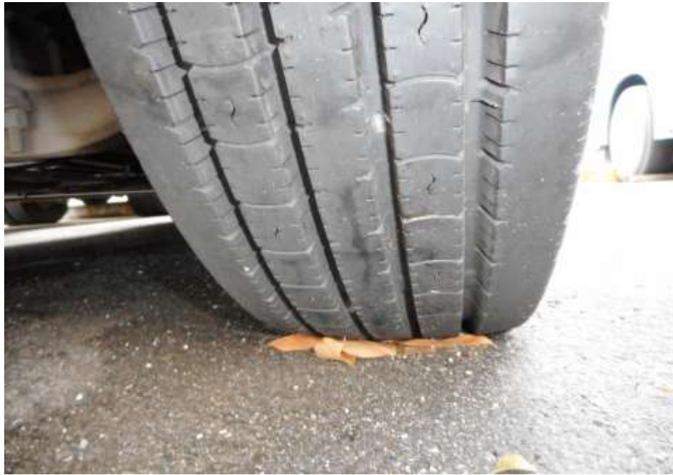
Photo 10 shows the condition of the front left tyres of the Motor Bus, which were observed to be in serviceable condition with remaining tread depth of approximately 11.6mm. There was also no tear, cut or burst mark(s) on the outer and the inner sidewalls as well as across the tread of the 6 tyres that were fitted on the Motor Bus.
