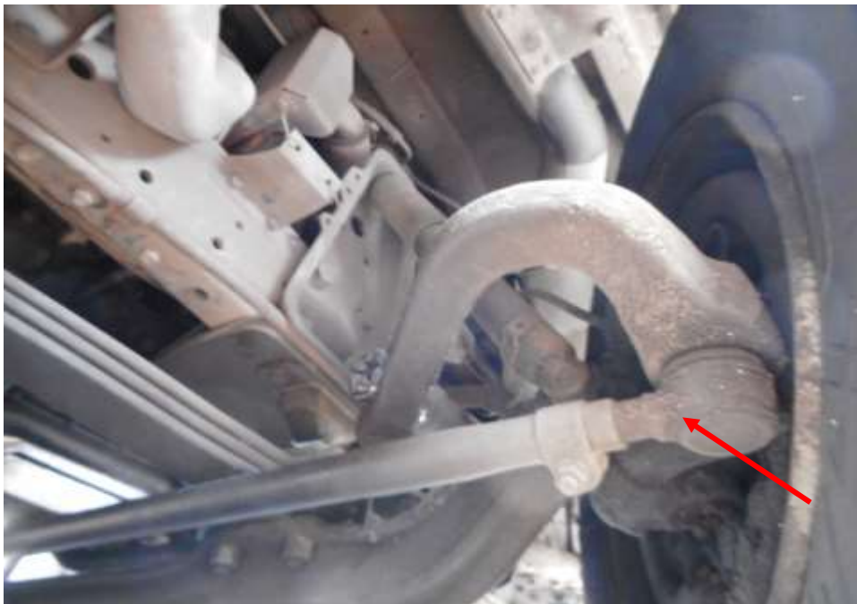
Photo 19 shows the various undercarriage components at the front right wheel of the Motor Bus, in particular the steering tie rod end (arrowed). The various steering components were all found to be intact, suggesting that the steering system of the Motor Bus was likely to be in serviceable condition at the material time of accident. There was also no sign of fluid stain(s) observed on the various undercarriage components.
