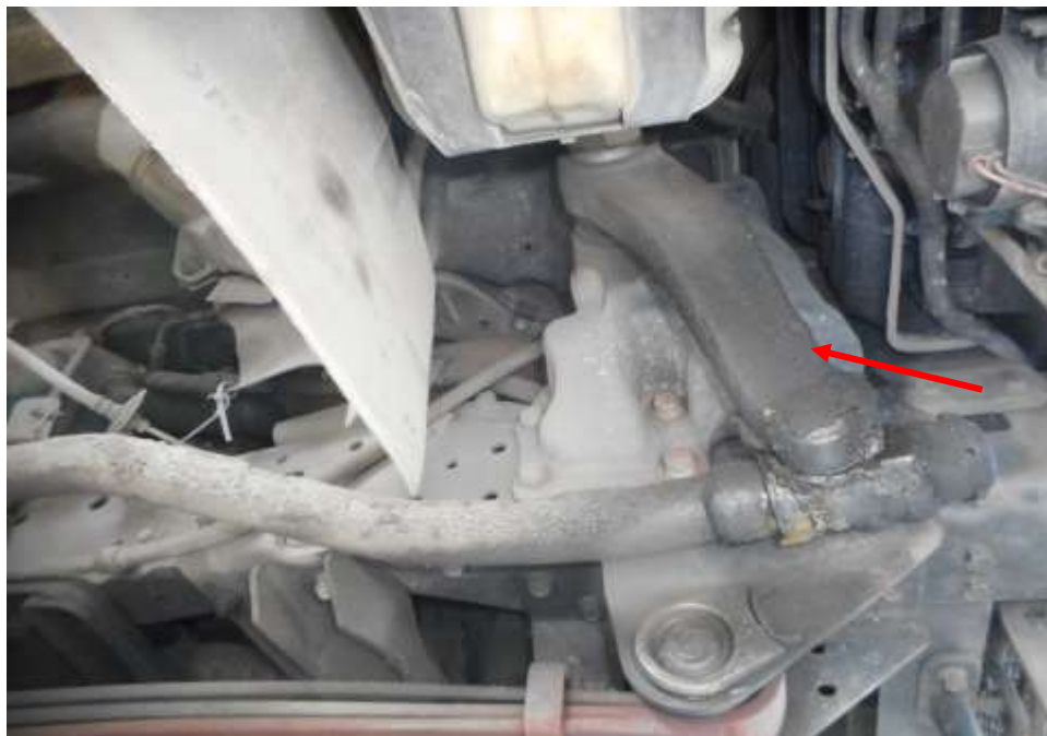
Photo 21 shows the steering box component (arrowed) at the undercarriage of the Motor Bus was found to be intact without any visible damage. There was also no sign of fluid stain(s) observed on the various undercarriage components.
