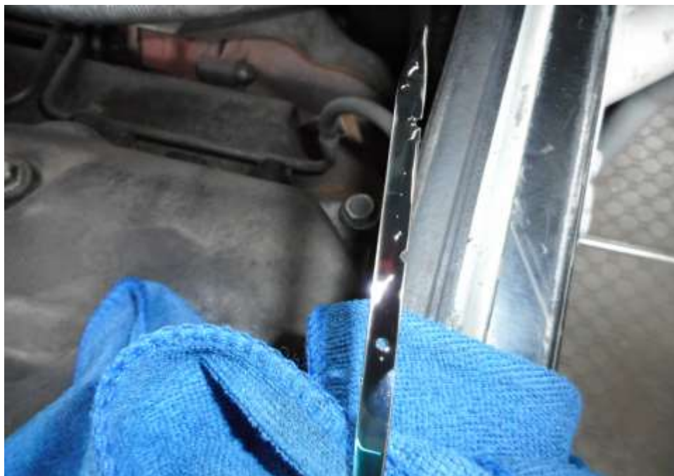
Photo 14 shows the engine oil dip stick system of the Motor Bus at the time of my inspection. The engine oil was observed to be of sufficient level for operation and without any visible contamination.
