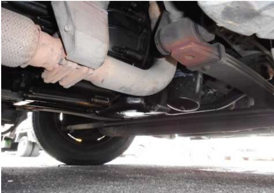
Photo 22 shows the undercarriage of the Motor Bus, at the area where the engine housing located. We observed minor fresh fluid stains on the surface of the engine oil sump. However the engine oils in the Motor Bus engine is sufficient and in serviceable condition.
