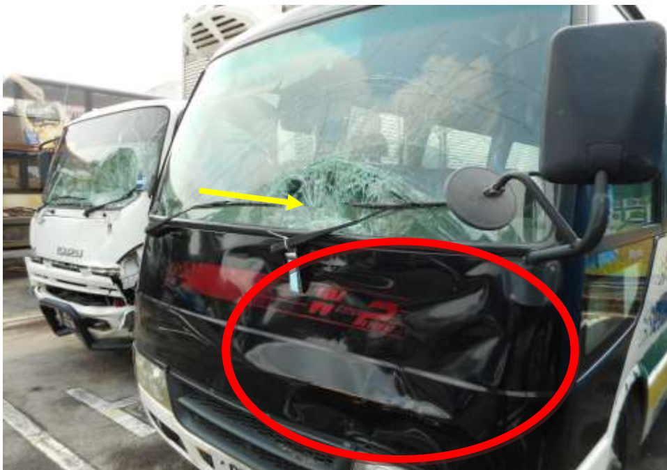
Photo 3 shows a close up view of the frontal portion of the Motor Bus at the time of my inspection. The Motor Bus was observed to have sustained moderate damages at its frontal portion. Its front windscreen (yellow arrow) and front body panel (circled) was damaged as a result of the accident at the time of my inspection.
