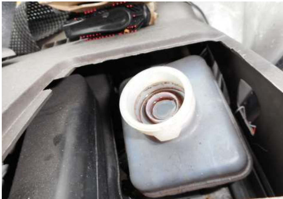
Photo 12 shows the brake fluid reservoir of the Motor Bus at the time of my inspection. The brake fluid was observed to be of sufficient level (arrowed) and without any visible contamination.
