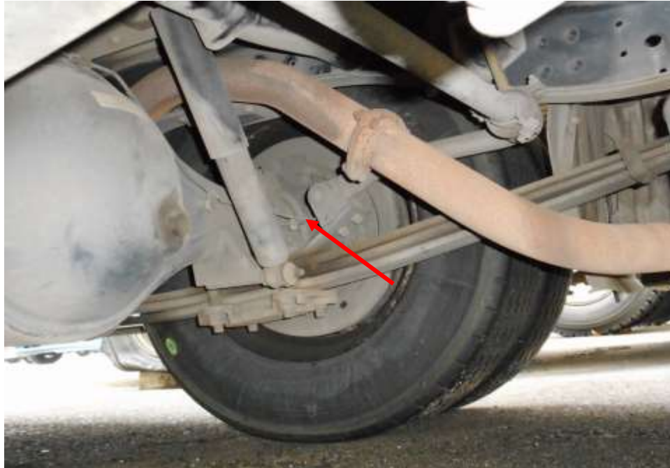
Photo 15 shows the brake pipe (arrowed) at the rear right wheel of the Motor Bus. I did not observe any leakage of brake fluid at the time of my inspection of the Motor Bus. My static tests of the Motor Bus's braking system, along with my visual examination of the various mechanical components in the braking system, had indicated that there was no internal leakage of pressure/vacuum. Hence the braking system of the Motor Bus was likely to be in serviceable condition at the material time of accident.
