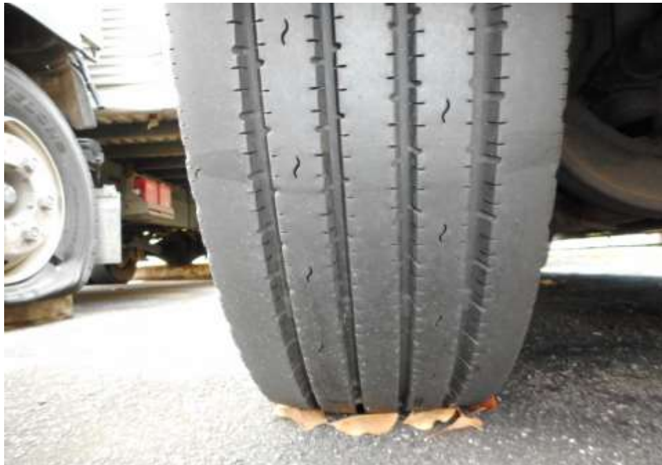
Photo 7 shows the condition of the front right tyre of the Motor Bus, which was observed to be in serviceable condition with remaining tread depth of approximately 10mm. The tyre, which was wrapped around standard steel wheel rim, was also observed to be sufficiently inflated for vehicular operation. There was no tear, cut or burst mark(s) on the outer and the inner sidewalls as well as across the tread of the 6 tyres that were fitted on the Motor Bus.
