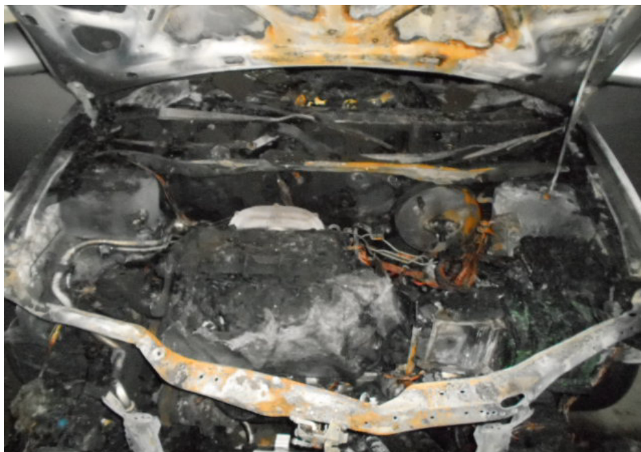
Photo 3 shows the engine compartment of the Insured Vehicle at the time of my inspection. The entire engine compartment of the Insured Vehicle was observed to be severely burnt. Most of the parts inside the engine compartment were found to be burnt and/or melted as a result of the fire.
