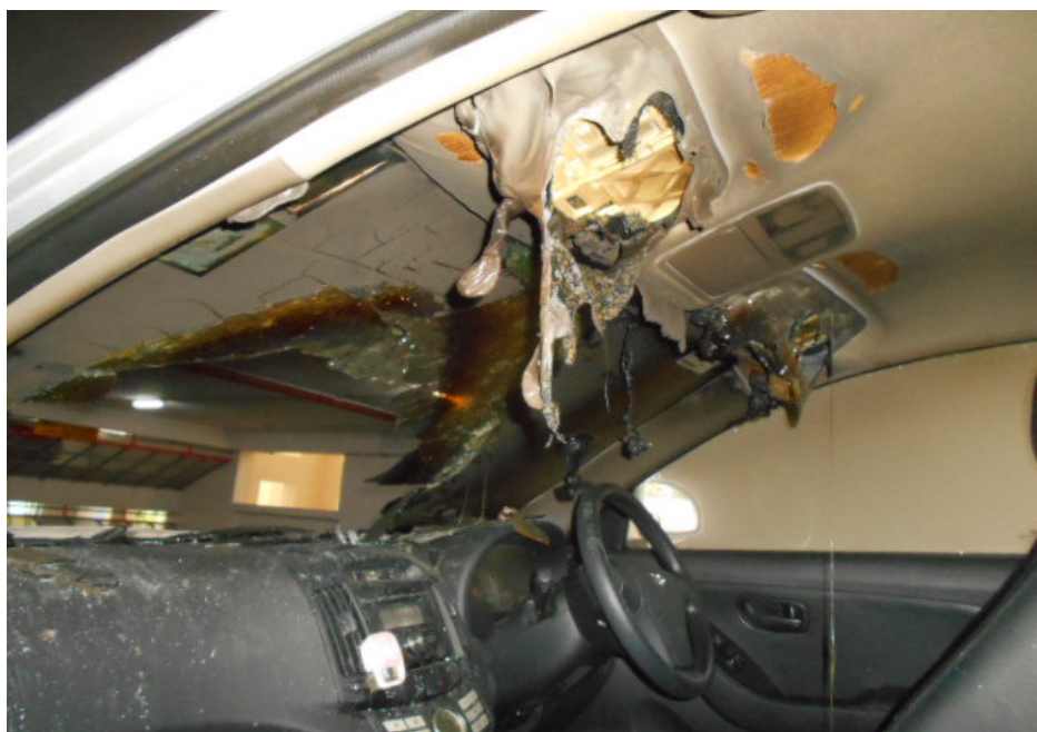
Photo 4 shows the interior compartment of the Insured Vehicle, which was observed to be partially burnt and/or melted at the front area. The front windscreen, front dashboard, plastic trims and roof upholstery were amongst the parts that were found to have been burnt and/or melted as a result of the fire.
