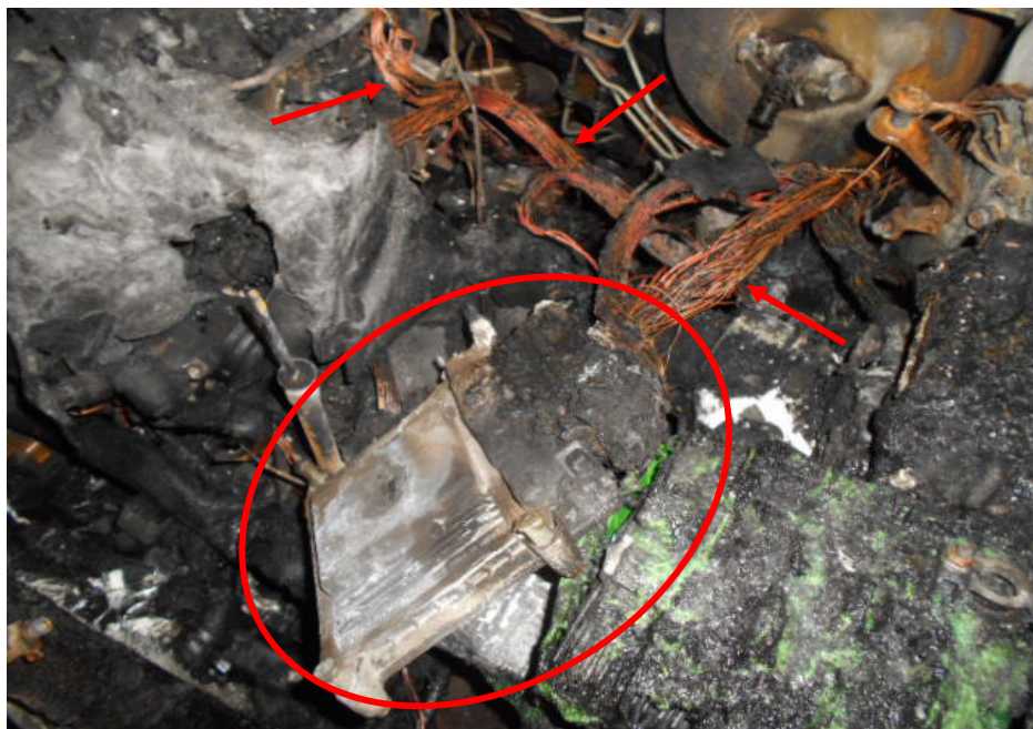
Photo 10 shows a closer view of the wirings (arrowed) that were found to be burnt to its bare copper state. These wirings were all original wiring harnesses leading to the Engine Control Module (ECM) (circled) of the Insured Vehicle.
