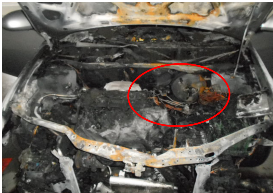
Photo 6 shows a general view of where the fire to the Insured Vehicle had originated, which was somewhere around the centre and towards the rear of the engine compartment (circled). This was established from the burn pattern and the rust that had developed on the underside of Insured Vehicle's front bonnet, as well as taking into consideration the characteristic of heat rising upwards.
