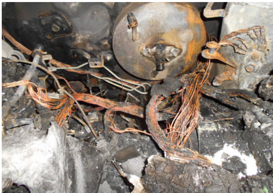
Photo 8 shows a closer view of the wirings that were found to be burnt to its bare copper state. Such condition normally indicates internal heating of copper wires which is a sign of an electrical short circuit occurring. These wirings were all original wiring harnesses of the Insured Vehicle.
