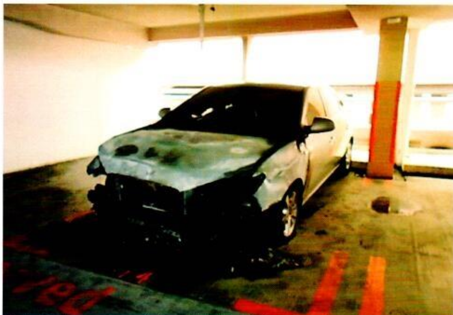
Photo 2 shows a general view of the front left portion of the Insured Vehicle at the time of my inspection. The fire damage to the Insured Vehicle was observed to be relatively severe. Its front bumper, front bonnet, front left headlamp and front left fender were amongst the body parts that were found to have been affected as a result of the fire.
