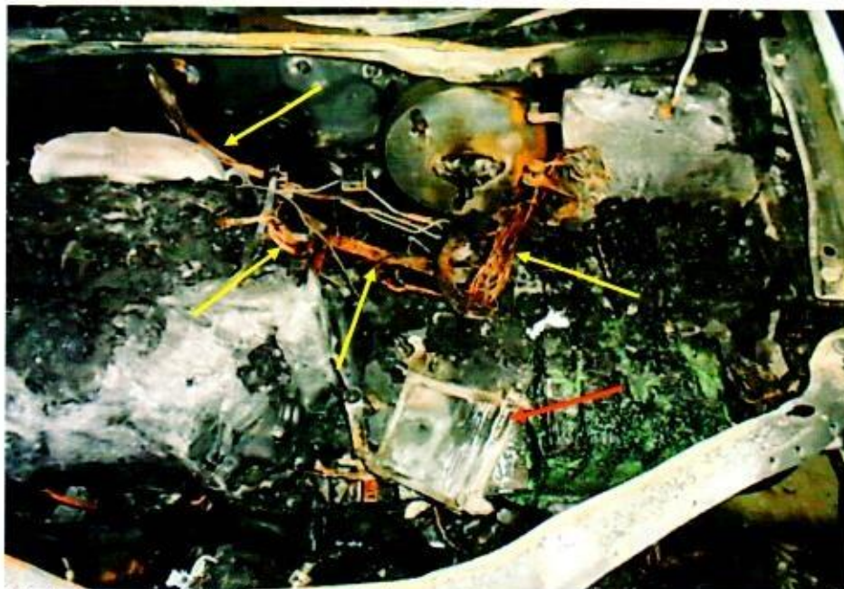
Photo 7 shows the wirings around the centre and towards the rear of the engine compartment, which was where the fire to the Insured Vehicle had started. Several stretches of wirings (yellow arrow) were found to be burnt to its bare copper state. The bright reddish colour of the copper wires suggest that the wirings were exposed to high heat. Such condition normally indicates internal heating of copper wires which is a sign of an electrical short circuit. The wirings were original wiring harnesses connecting the Engine Control Module (ECM) (arrowed) of the Insured Vehicle to multiple sub-control units, sensors and actuators for vehicular operation.
