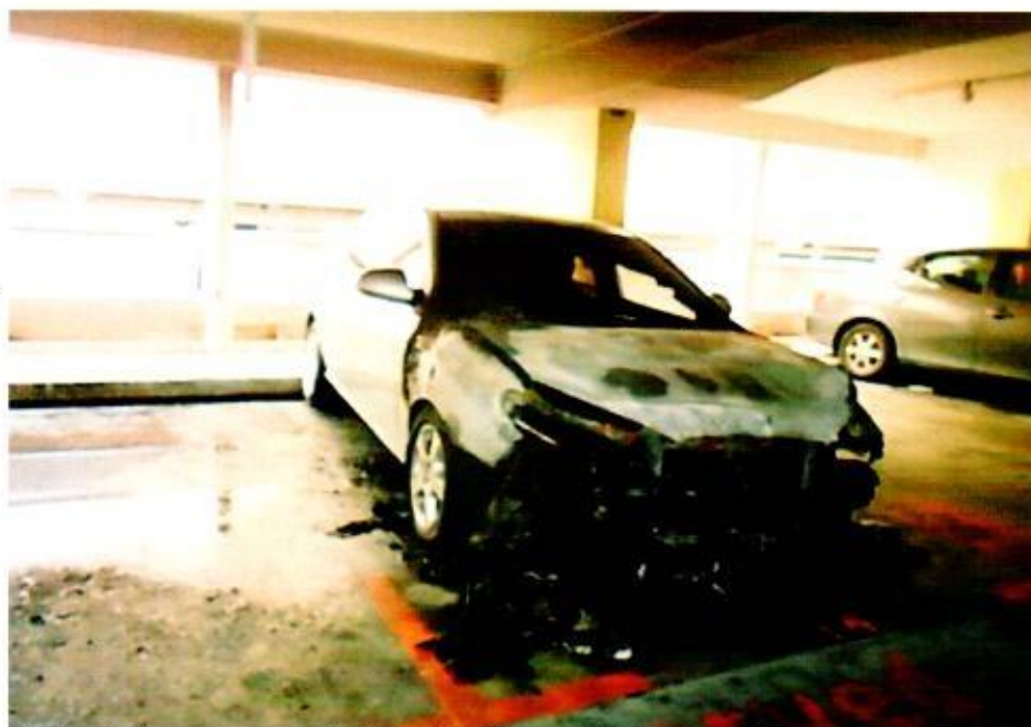
Photo 1 shows a general view of the front right portion of the Insured Vehicle at the time of my inspection. The fire damage to the Insured Vehicle was confined to its frontal portion. Its front bumper, front bonnet, front grille, front right headlamp and front right fender were amongst the body parts that were found to have been affected as a result of the fire.
