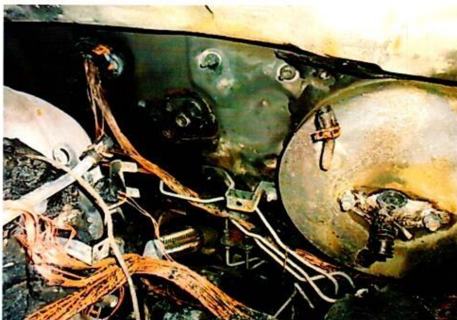
Photo 9 shows a closer view of another stretch of bright reddish coloured copper wires that were found within the engine compartment of the Insured Vehicle. Such condition normally indicates internal heating of copper wires, which is a sign of an electrical short circuit. The wirings were original wiring harnesses of the Insured Vehicle.
