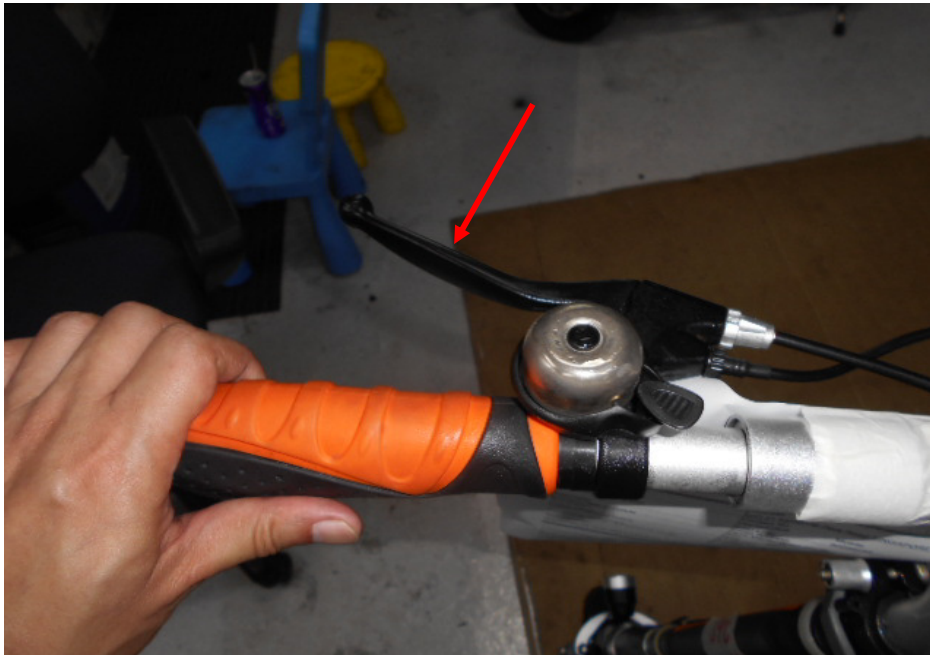
Photo 13 shows the lever (arrowed) that operates the braking function of the electric scooter. The lever is operated manually. When depressed, the brake is activated by cable and spring pushing the brake shoe outwards to clamp onto the brake drum at the rear wheel of the electric scooter. Frictional resistance from this clamping action reduces the rotation of the rear wheel, hence creating the braking effect for the electric scooter.
