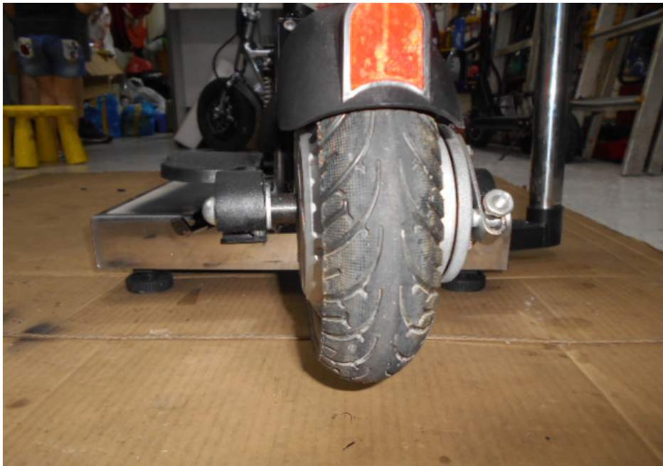
Photo 4 shows the rear tyre that was fitted on the electric scooter. The rear tyre was observed to be of serviceable condition with the tread pattern clearly visible. Similar to the front tyre, the rear tyre of the electric scooter was sufficiently inflated for operation.
