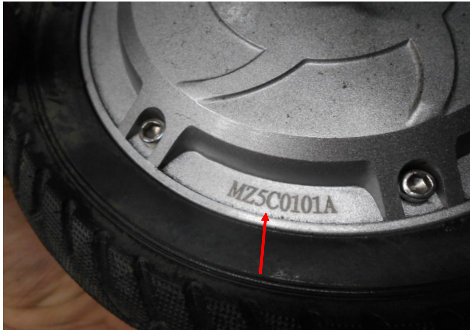
Photo 9 shows the electric motor that was fitted on the rear wheel of the electric scooter. The motor in this electric motor turns/rotates when electric power is supplied from the battery of the electric scooter. From the serial number (arrowed) engraved on the electric motor, the electric motor fitted was a standard original electric motor.
