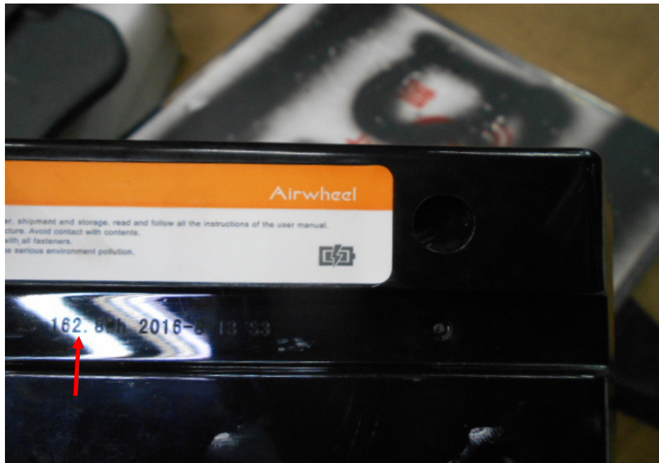
Photo 11 shows the battery that was fitted on the electric scooter. This battery supplies the electric power to the electric motor in order for the electric scooter to accelerate/move. The capacity of the battery was indicated as 162.8 Watt/hour (arrowed), a standard original battery for the electric scooter.
