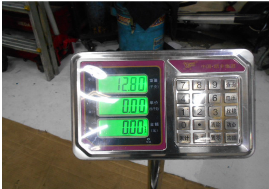
Photo 7 shows the weight of the electric scooter that was recorded by the digital weighing scale. The weight recorded was 12.80kg.
