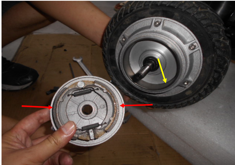
Photo 15 shows the rear brake of the electric scooter after it was dismantled. When the brake is activated, cable and spring actions pushes the brake shoe (red arrow) outwards to clamp onto the inner surface (yellow arrow) of the brake drum. Frictional resistance from this clamping action reduces the rotation of the rear wheel, hence creating the braking effect for the electric scooter.
