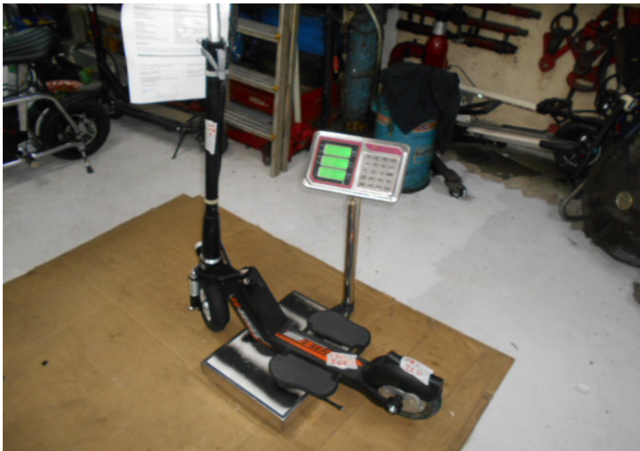
Photo 6 shows the electric scooter being weighed on a digital weighing scale. The digital weighing scale was first calibrated to zero prior to the weighing.
