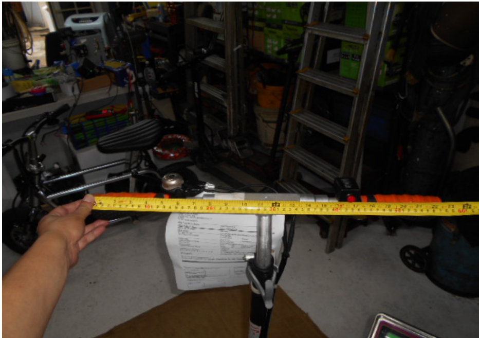
Photo 5 shows measurements being carried out to the electric scooter. The length of the electric scooter (leading edge of front tyre to trailing edge of rear tyre) was measured to be approximately 80cm while the width of the electric scooter was measured to be approximately 58cm.
