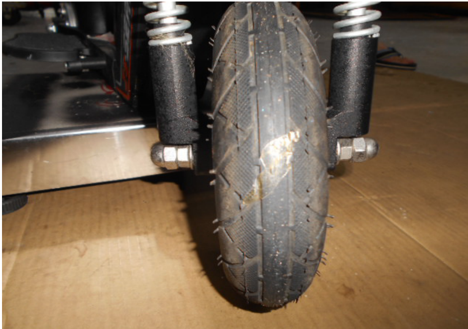
Photo 3 shows a general view of the front tyre of the electric scooter. The front tyre fitted on the electric scooter was observed to be of serviceable condition with the tread pattern clearly visible. It was also sufficiently inflated for operation.
