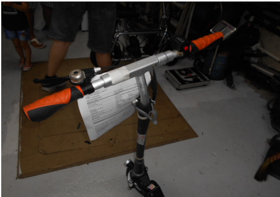
Photo 2 shows a general view of the handle bar of the electric scooter. The width of the electric scooter was measured to be approximately 58cm. This was the length of the handle bar from one side to the other side, which typically represents the width of an electric scooter given that the handle bar extends laterally out from the body of an electric scooter.
