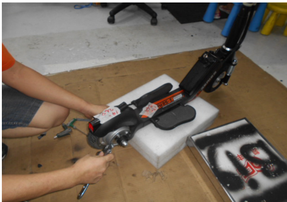
Photo 8 shows dismantling of the rear wheel being carried out to check on the electric motor and rear brake of the electric scooter.
