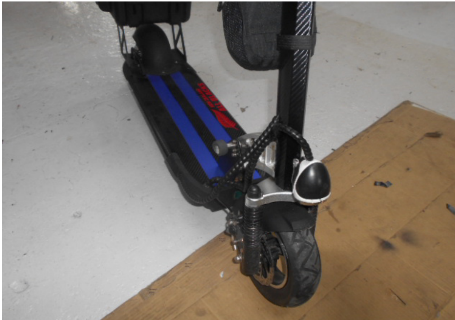
Photo 3 shows a general view of the frontal body and front tyre of the electric scooter. The front tyre fitted on the electric scooter was observed to be of serviceable condition with the tread pattern clearly visible.
