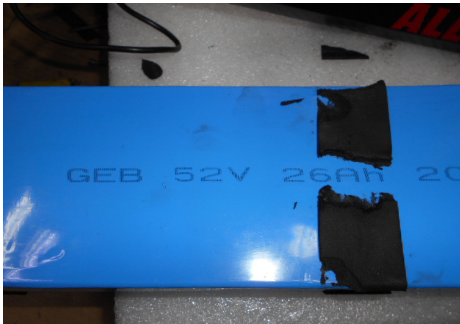
Photo 10 shows the battery fitted on the electric scooter was a 52 Volt with 26 Ampere/hour battery. This battery supplies the electric power to the electric motor in order for the electric scooter to accelerate/move.
