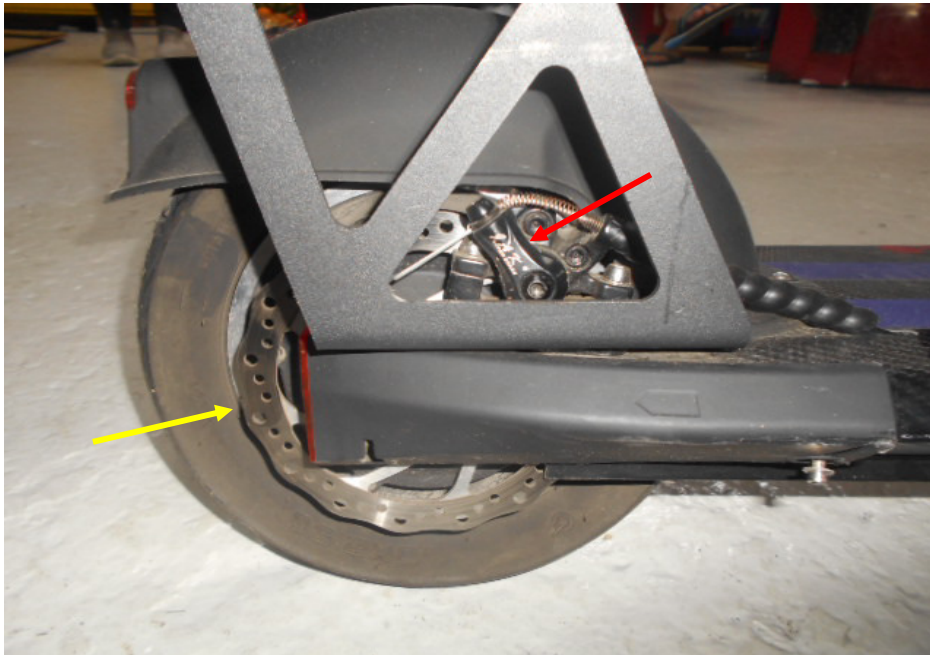
Photo 15 shows the braking components at the rear wheel of the electric scooter. When the rear brake lever of the electric scooter is depressed, the brake pad (red arrow) clamps against the brake disc (yellow arrow), via cable and spring, hence providing the frictional resistance to reduce the rotation of the rear wheel.
