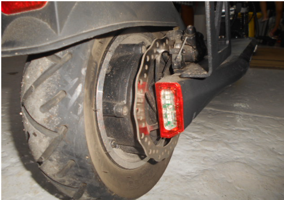
Photo 4 shows the rear tyre that was fitted on the electric scooter. The rear tyre was observed to be of serviceable condition with the tread pattern clearly visible.
