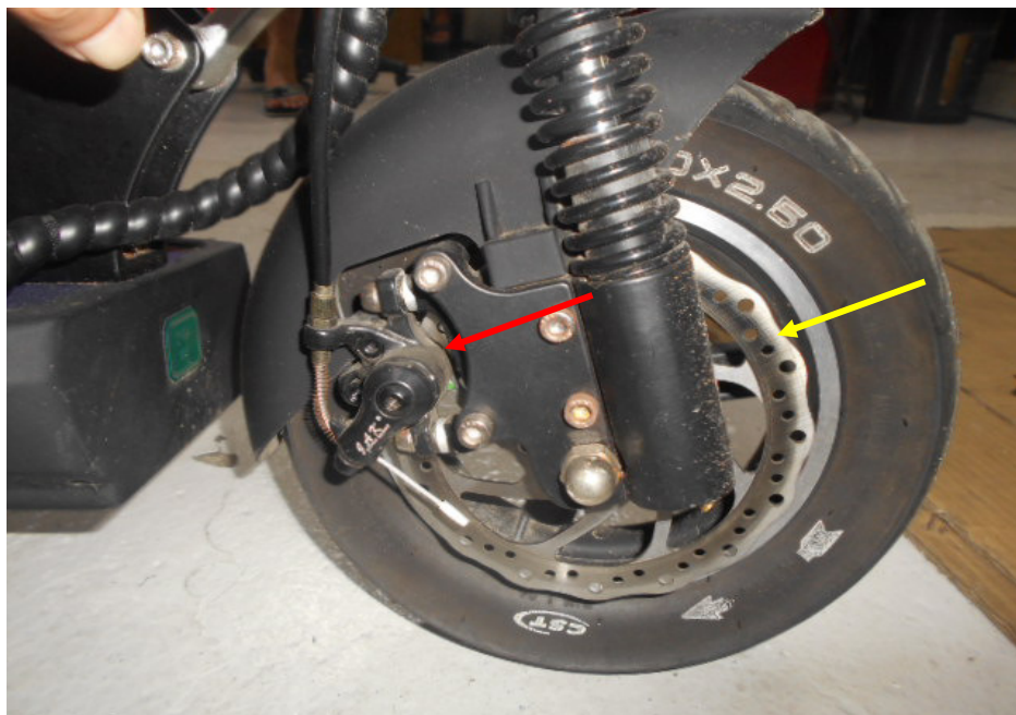
Photo 14 shows the braking components at the front wheel of the electric scooter. When the front brake lever of the electric scooter is depressed, the brake pad (red arrow) is pushed towards the brake disc (yellow arrow) via cable and spring. The brake pad clamps against the brake disc providing the frictional resistance to reduce the rotation of the front wheel, hence creating the braking effect for the electric scooter.
