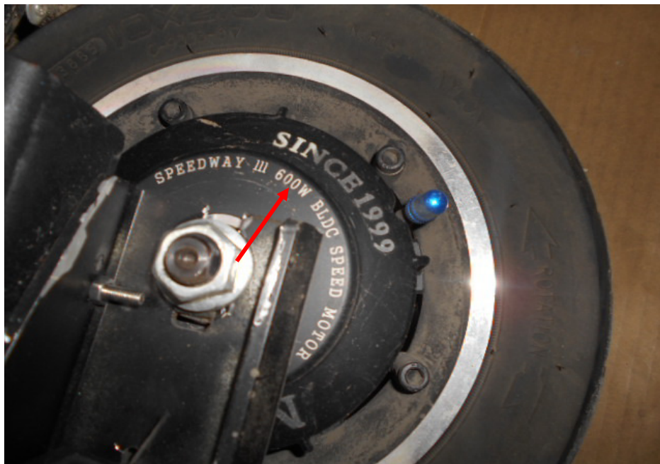
Photo 8 shows the electric motor that was fitted on the rear wheel of the electric scooter. The power rating of the electric motor was observed to be 600 Watt (arrowed). The motor in this electric motor turns/rotates when electric power is supplied from the battery of the electric scooter.
