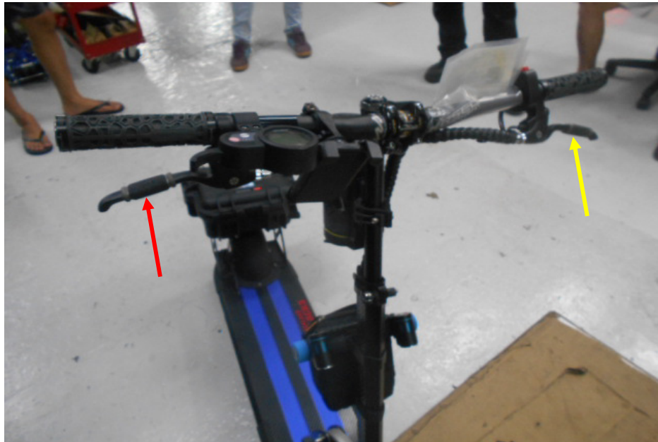
Photo 13 shows the levers that operates the braking function of the electric scooter. The lever (red arrow) at the right side of the handle bar operates the brake for the front wheel while the lever (yellow arrow) at the left side of the handle bar operates the brake for the rear wheel. The levers can be simultaneously depressed or individual depressed.
