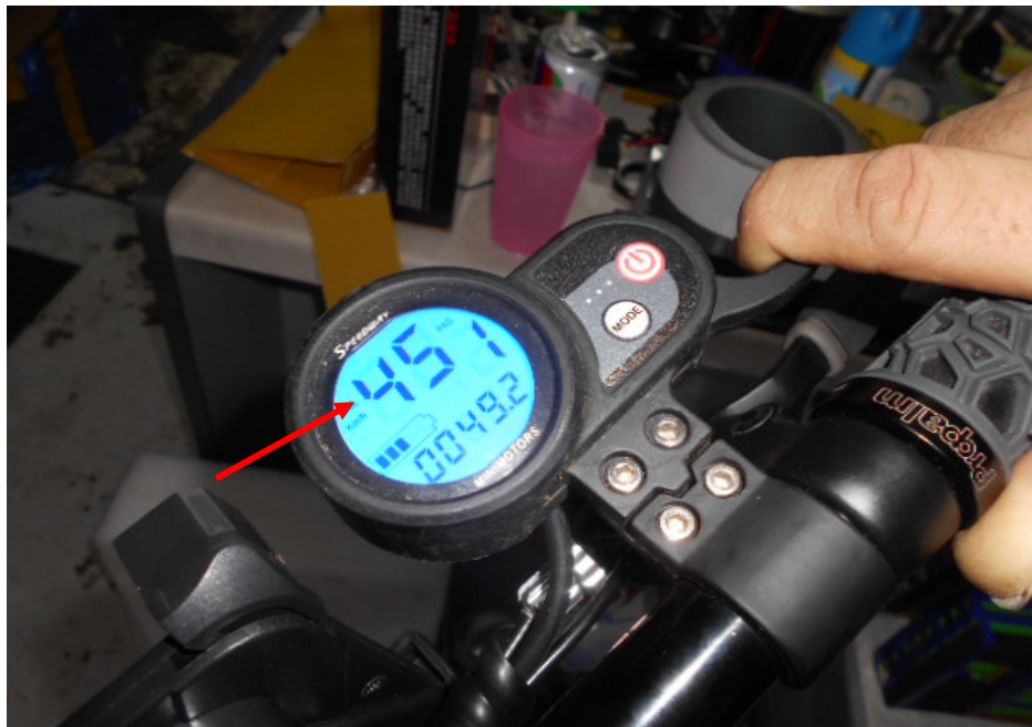
Photo 12 shows the lever (arrowed) for the acceleration/movement function of the electric scooter being depressed with the speed (arrowed) of the electric scooter displayed on the digital meter. To maintain acceleration/movement, the lever will have to be continuously depressed.
