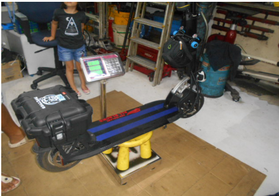
Photo 6 shows the electric scooter being weighed on a digital weighing scale. The yellow plastic chair supporting the electric scooter on the weighing scale was to prevent the tyres of the electric scooter from touching the ground during the weighing. The digital weighing scale was first calibrated to zero when the yellow plastic chair was placed on the scale.
