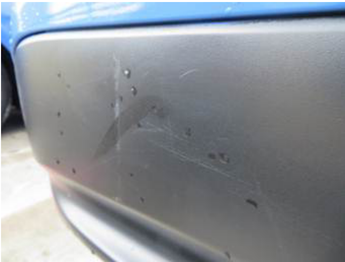
The above photos shows a closer view of the rear bumper under cover portion that sustained damages and the point of impact between both vehicles. The damages observed to the taxi's rear portion shows a vertical indentation which may likely correspond to the front number plate of your vehicle that is the most protruding portion that may have likely in contact with the rear bumper under cover of the taxi (please refer to the below scene photo).
