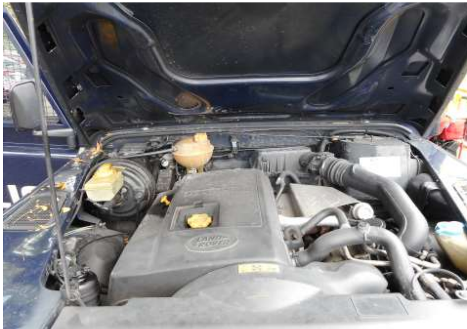
Photo 12 shows a general view of the Motor Jeep's engine compartment. The various parts and components inside the engine compartment were unaffected by the accident. There was also no sign(s) or indication(s) of fluid leakage and/or fluid stain within the engine compartment.
