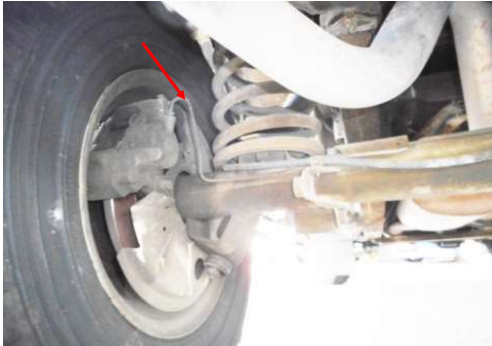
Photo 19 shows the brake hose/pipe (arrowed) at the rear left wheel of the Motor Jeep. I did not observe any leakage of brake fluid at the time of my inspection of the Motor Jeep. Static tests of the Motor Jeep's braking system had indicated that there was no internal leakage of pressure/vacuum. The undercarriage components of the Motor Jeep were also all found to be intact and without any visible damage.
