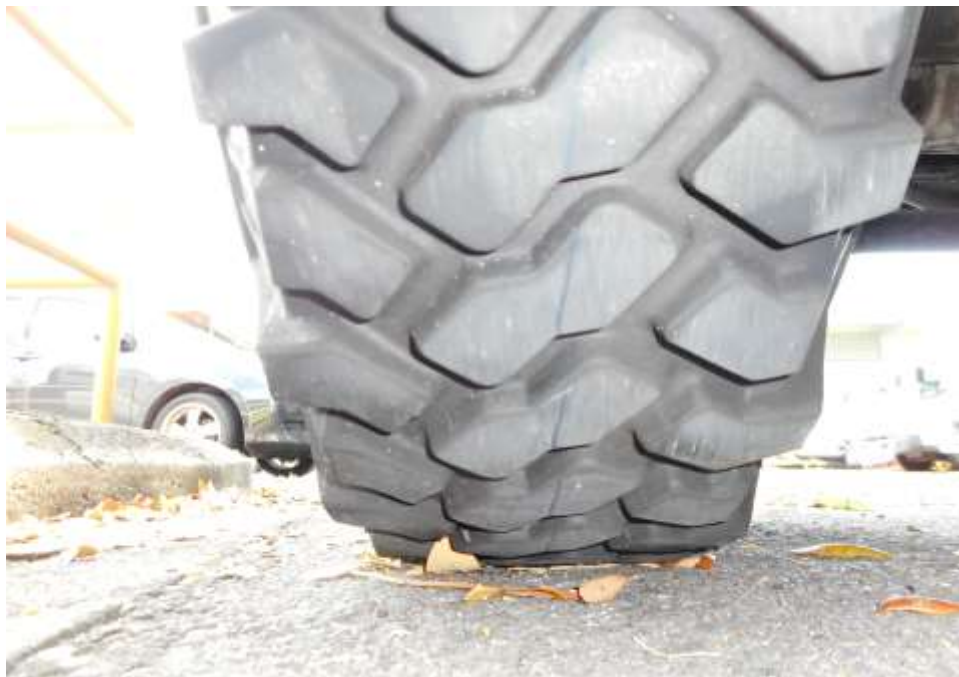
Photo 11 shows the condition of the rear right tyre of the Motor Jeep, which was observed to be in serviceable condition with remaining tread depth of approximately 9.1mm. There was also no tear, cut or burst mark(s) on the outer and the inner sidewalls as well as across the tread of the Motor Jeep's 4 tyres.
