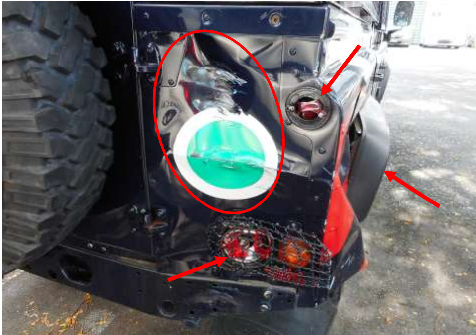
Photo 2 shows a close up view of the damaged rear portion. Its rear right body panel (circled), rear right brake lamp and rear right fender (arrowed) were amongst the body parts that were damaged as a result of the accident.
