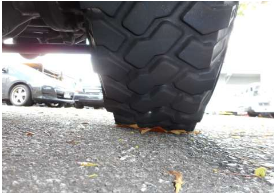
Photo 8 shows the condition of the front right tyre of the Motor Jeep, which was observed to be in serviceable condition with remaining tread depth of approximately 9.6mm. The tyre was sufficiently inflated for vehicular operation with no tear, cut or burst mark(s) on the outer and the inner sidewalls as well as across the tread. The 4 tyres of the Motor Jeep were wrapped around standard steel wheel rims without any damage.
