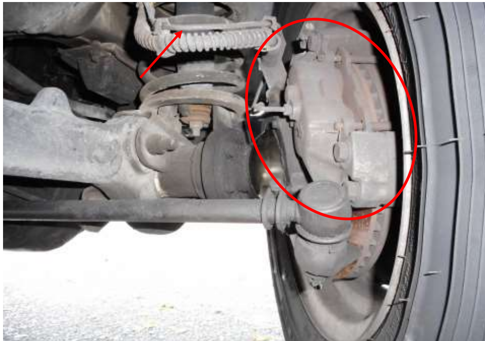
Photo 20 shows the brake hose/pipe (arrowed) at the front right wheel of the Motor Jeep. No leakage of brake fluid was observed. Visual examination of the various components of the braking system like the brake caliper (circled), brake booster, brake pedal etc had revealed all to be intact and without visible damage.
