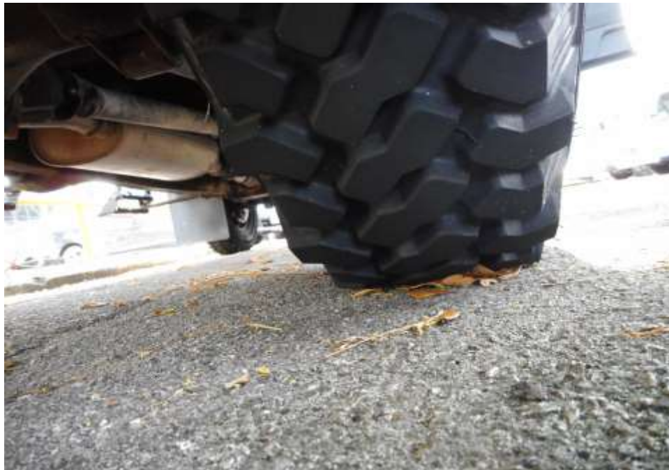
Photo 9 shows the condition of the rear right tyre of the Motor Jeep, which was observed to be in serviceable condition with remaining tread depth of approximately 12.3mm. The tyre was also observed to be sufficiently inflated for vehicular operation with no tear, cut or burst mark(s).
