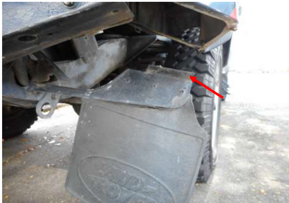
Photo 3 shows a close up view of the damaged rear portion rear right mud flaps were amongst the body parts that were damaged as a result of the accident. (arrowed) were amongst the body parts that were damaged as a result of the accident.
