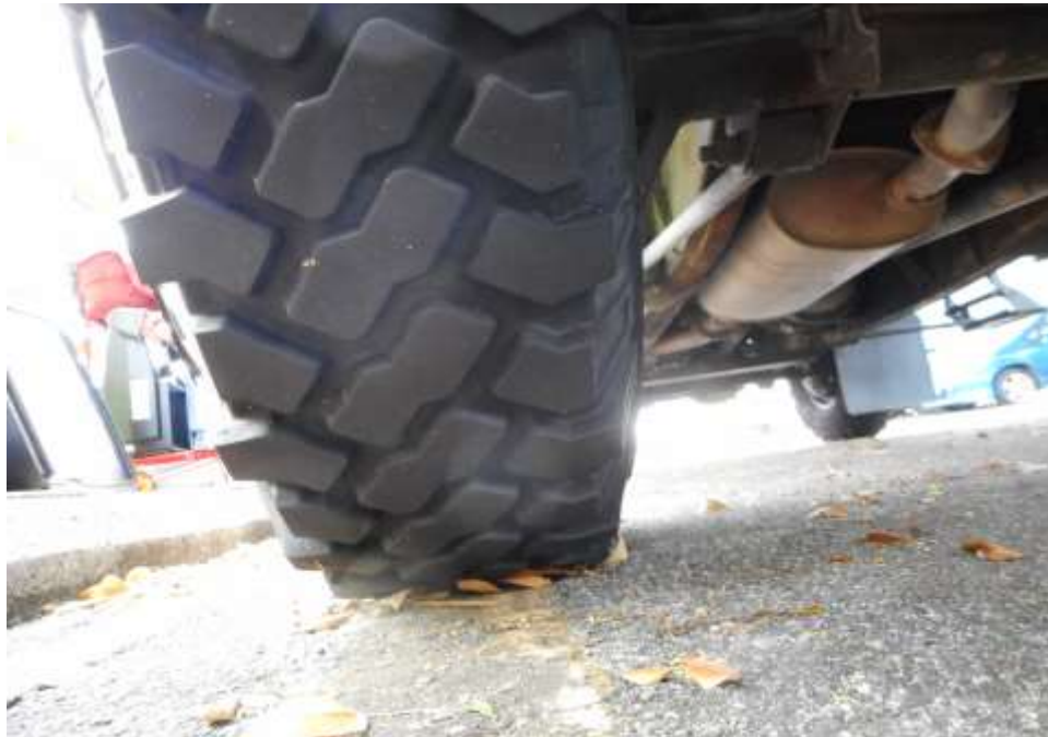
Photo 10 shows the condition of the rear left tyre of the Motor Jeep, which was observed to be in serviceable condition with remaining tread depth of approximately 9mm. The tyre was sufficiently inflated for vehicular operation with no tear, cut or burst mark(s) on the outer and the inner sidewalls as well as across the tread. The 4 tyres of the Motor Jeep were wrapped around standard steel wheel rims without any damage.
