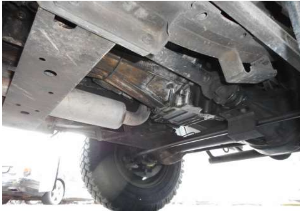
Photo 17 shows the undercarriage of the Motor Jeep, at the area where the engine housing, transmission housing and front axle differential housing are located. I did not find any sign(s) or indication(s) of fluid leak and/or fluid stain(s) on the underside of the Motor Jeep.
