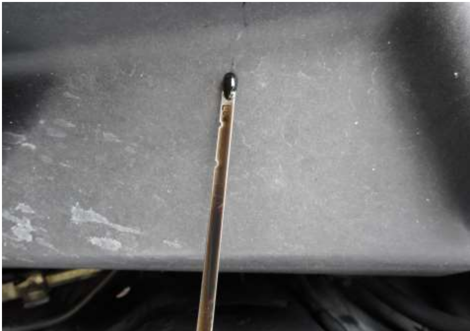
Photo 16 shows the engine oil dip stick of the Motor Jeep at the time of my inspection. The engine oil was observed to be of sufficient level and without any visible contamination.
