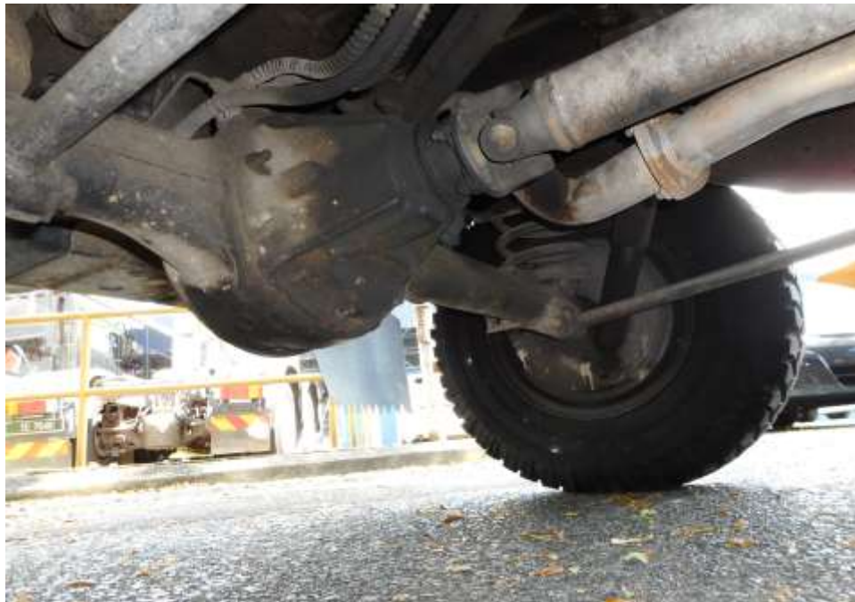
Photo 18 shows the undercarriage of the Motor Jeep, at the area where the rear axle differential housing are located. I did not find any sign(s) or indication(s) of fluid leak and/or fluid stain(s) on the underside of the Motor Jeep.
