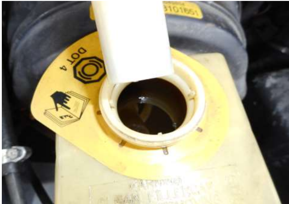
Photo 13 shows the brake fluid reservoir of the Motor Jeep at the time of my inspection. The brake fluid was observed to be of sufficient level and without any visible contamination.
