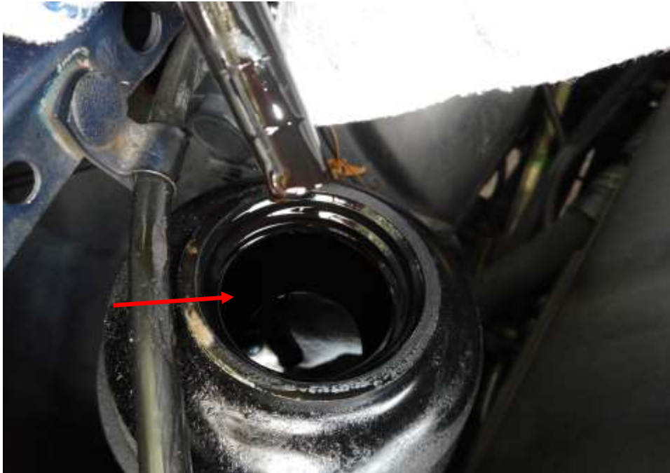
Photo 15 shows checks being carried out to the power steering reservoir of the Motor Jeep at the time of my inspection. The steering fluid was observed to be of sufficient level (arrowed) and without any visible contamination.
