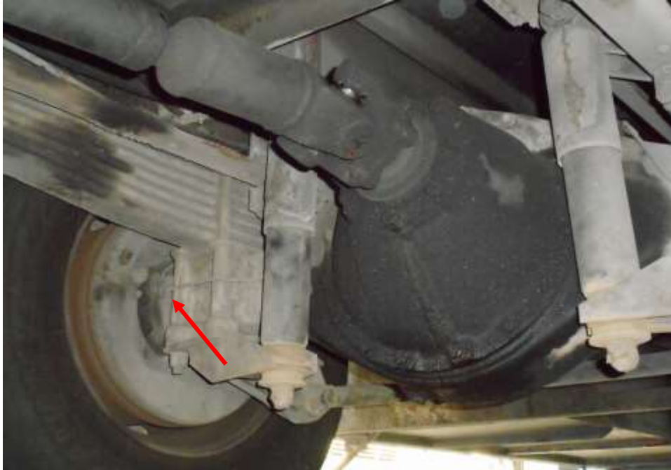
Photo 16 shows the brake pipe (arrowed) at the rear right wheel of the Motor Bus. I did not observe any leakage of brake fluid at the time of my inspection of the Motor Bus. My static tests of the Motor Bus's braking system, along with my visual examination of the various mechanical components in the braking system, had indicated that there was no internal leakage of pressure/vacuum. Hence the braking system of the Motor Bus was likely to be in serviceable condition at the material time of accident.
