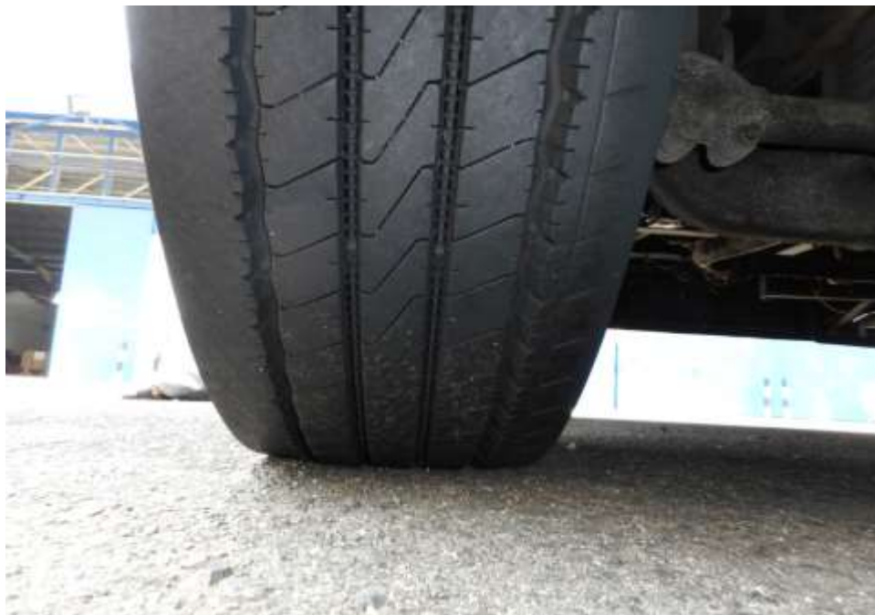
Photo 9 shows the condition of the front left tyres of the Motor Bus, which were observed to be in serviceable condition with remaining tread depth of approximately 8.9mm. There was also no tear, cut or burst mark(s) on the outer and the inner sidewalls as well as across the tread of the 6 tyres that were fitted on the Motor Bus.
