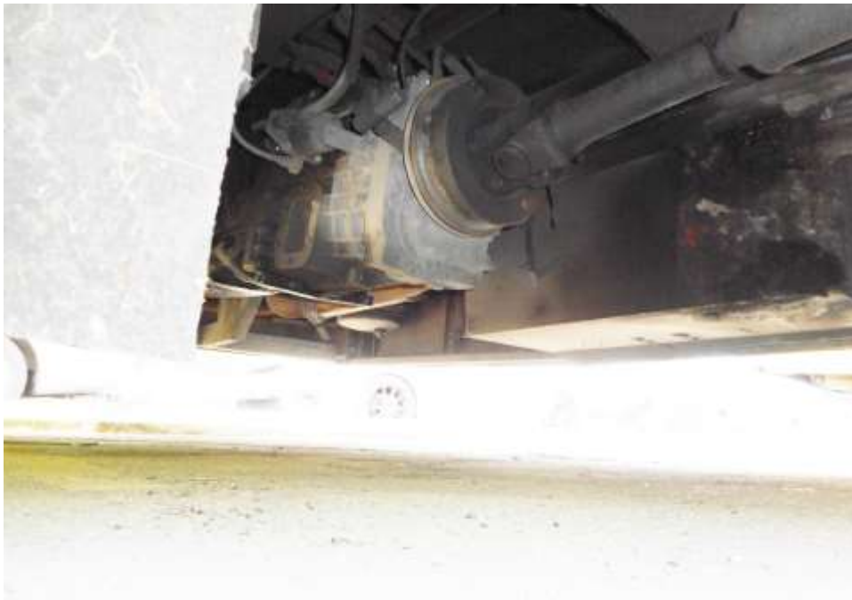
Photo 23 shows the undercarriage of the Motor Bus, at the area where the engine housing located. I did not find any sign(s) or indication(s) of fluid leak and/or fluid stain(s) on the underside of the Motor Bus.
