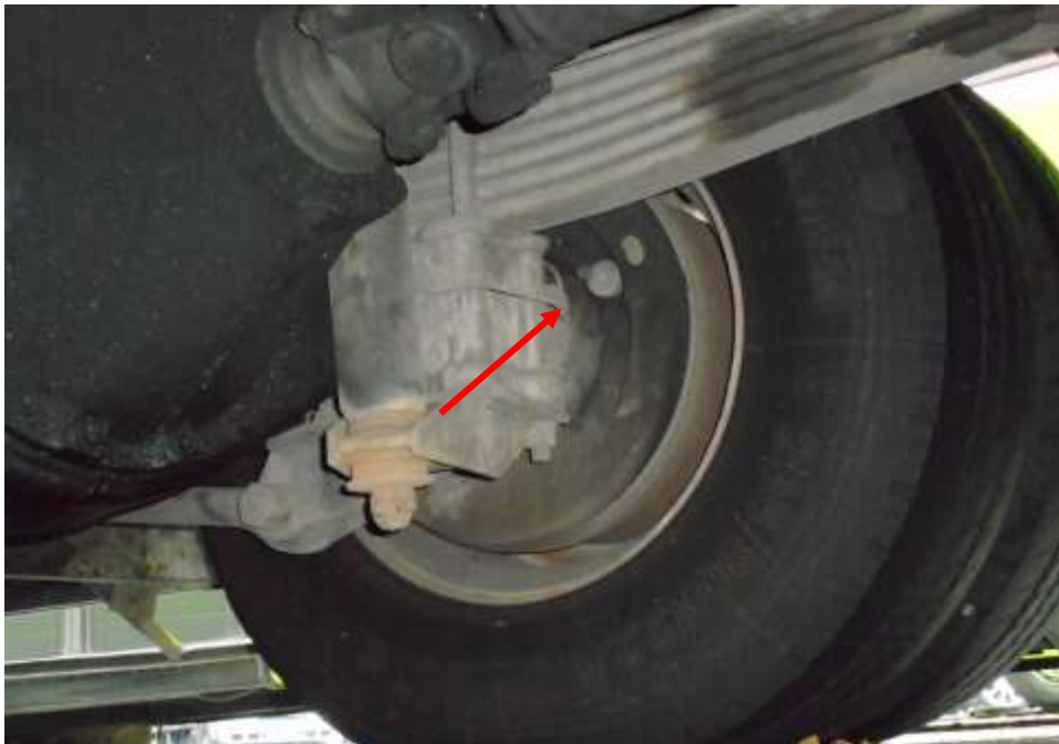
Photo 17 shows the brake pipe (arrowed) at the rear left wheel of the Motor Bus. I did not observe any leakage of brake fluid at the time of my inspection of the Motor Bus. My static tests of the Motor Bus's braking system, along with my visual examination of the various mechanical components in the braking system, had indicated that there was no internal leakage of pressure/vacuum. Hence the braking system of the Motor Bus was likely to be in serviceable condition at the material time of accident.
