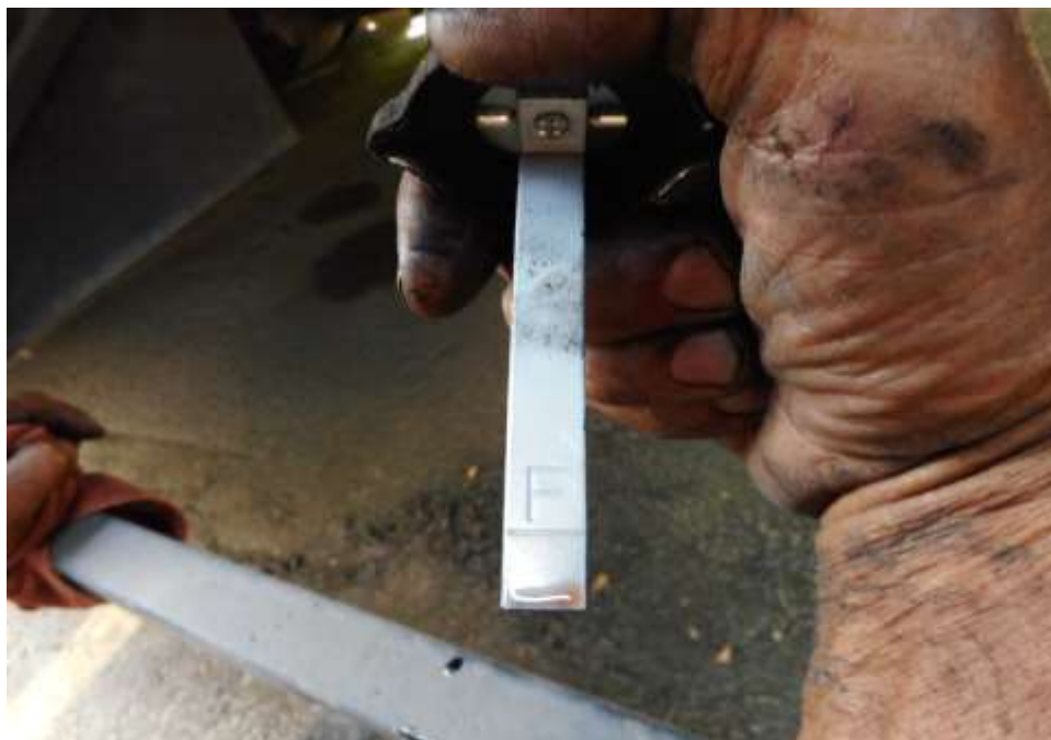
Photo 14 shows the power steering fluid reservoir of the Motor Bus at the time of my inspection. The power steering fluid was observed to be of sufficient level and without any visible contamination.
