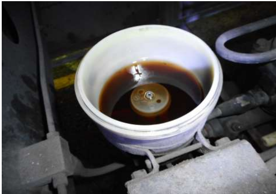
Photo 12 shows the brake reservoir of the Motor Bus at the time of my inspection. The brake fluid was observed to be of sufficient level & serviceable at the time of the accident.
