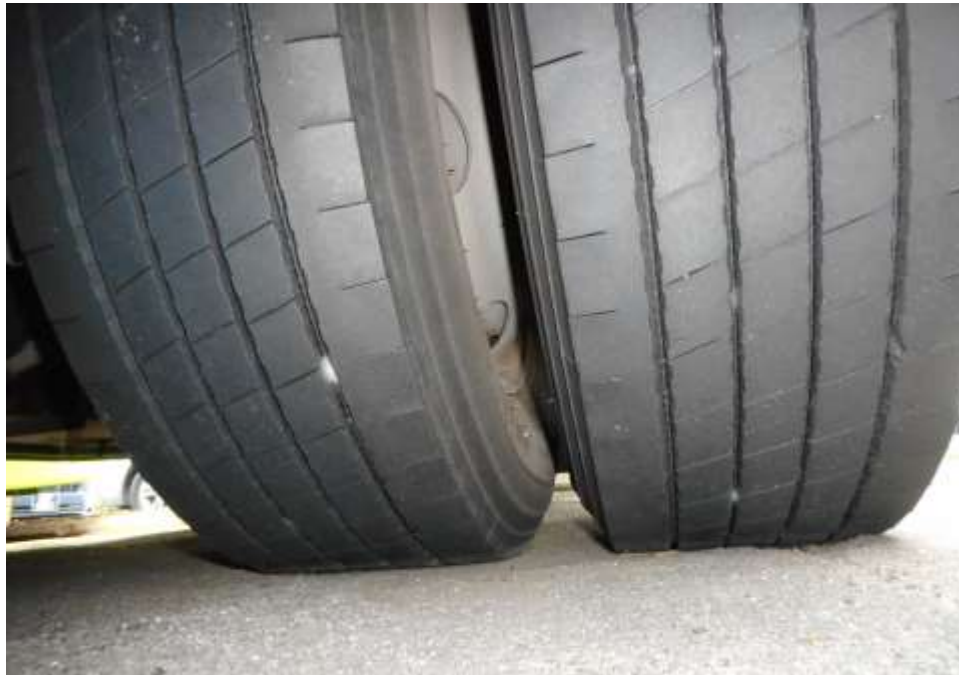
Photo 8 shows the condition of the rear left tyres of the Motor Bus, which was observed to be in serviceable condition with remaining tread depth of approximately 5.6mm. The tyres, which were wrapped around standard steel wheel rim, were also observed to be sufficiently inflated for vehicular operation. There was also no damage found on all 6 steel wheel rims of the Motor Bus.
