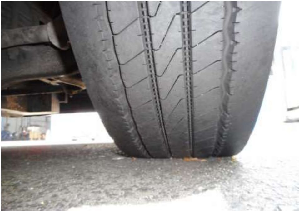
Photo 6 shows the condition of the front right tyre of the Motor Bus, which was observed to be in serviceable condition with remaining tread depth of approximately 9.5mm. The tyre, which was wrapped around standard steel wheel rim, was also observed to be sufficiently inflated for vehicular operation. There was no tear, cut or burst mark(s) on the outer and the inner sidewalls as well as across the tread of the 6 tyres that were fitted on the Motor Bus.
