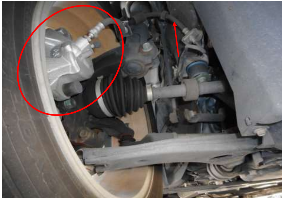
Photo 17 shows the brake hose/pipe (arrowed) at the front right wheel of the Motor Car. No leakage of brake fluid was observed. Visual examination of the various components of the braking system like the brake caliper (circled), brake booster, brake pedal etc had revealed all to be intact and without visible damage.
