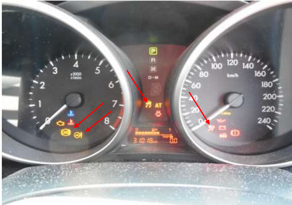
Photo 21 shows the warning light for Anti-Lock Brake System (ABS), Traction Control (TC) and Supplemental Restraint System (SRS) appearing on the instrument panel of the Motor Car during the self-test of its various electronic operating systems when its engine was cranked.
