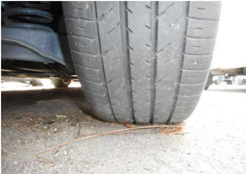
Photo 7 shows the condition of the rear right tyre of the Motor Car, which was observed to be in serviceable condition with remaining tread depth of approximately 5.3mm. The tyre was also observed to be sufficiently inflated for vehicular operation with no tear, cut or burst mark(s).
