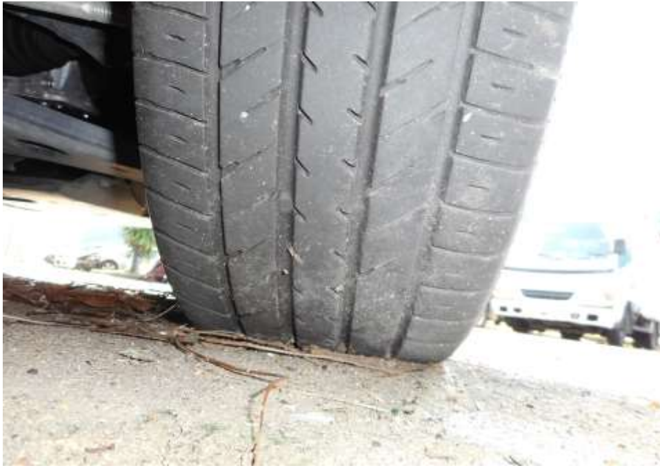
Photo 6 shows the condition of the front right tyre of the Motor Car, which was observed to be in serviceable condition with remaining tread depth of approximately 6mm. The tyre was sufficiently inflated for vehicular operation with no tear, cut or burst mark(s) on the outer and the inner sidewalls as well as across the tread. The 4 tyres of the Motor Car were wrapped around standard alloy wheel rims without any damage.
