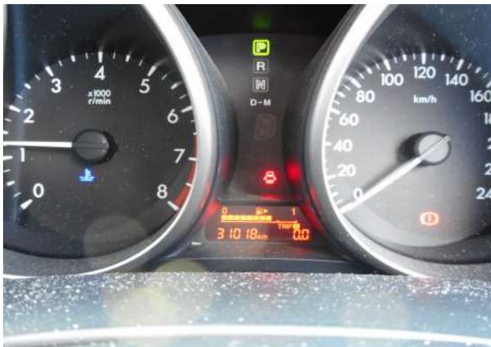
Photo 22 shows no warning lights illuminated on the instrument panel of the Motor Car after the engine was cranked. This would suggest that there was no abnormality to the various electronic operating systems of the Motor Car, like the ABS, TC and SRS etc.
