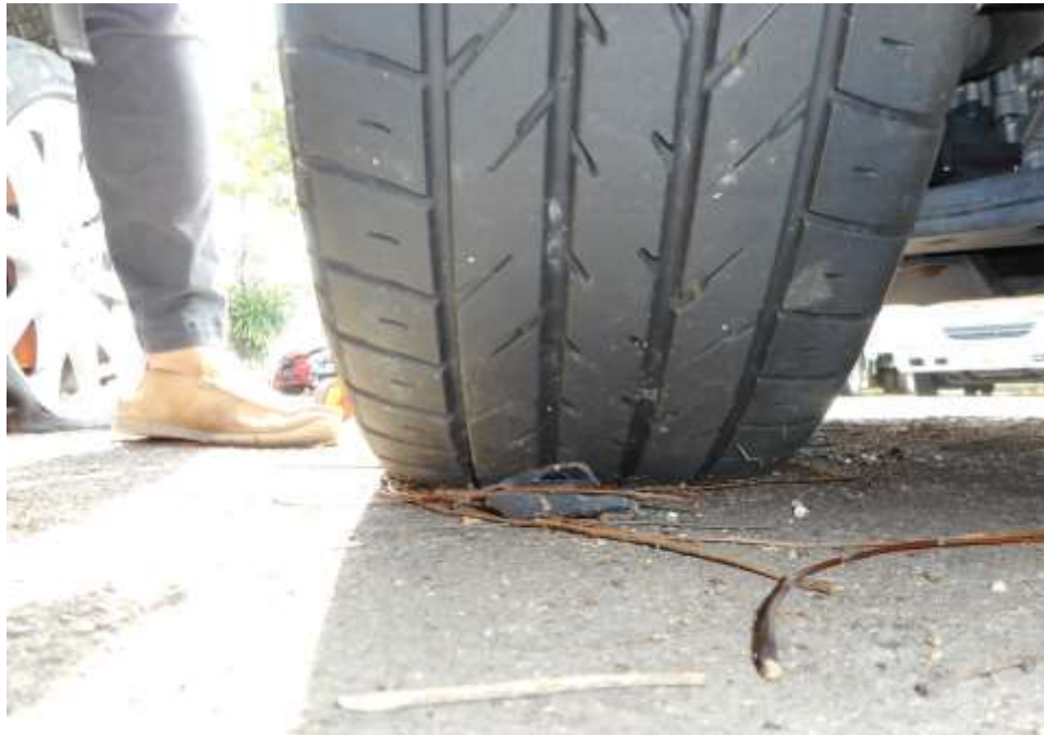
Photo 8 shows the condition of the front left tyre of the Motor Car, which was observed to be in serviceable condition with remaining tread depth of approximately 5.5mm. The tyre was sufficiently inflated for vehicular operation with no tear, cut or burst mark(s) on the outer and the inner sidewalls as well as across the tread. The 4 tyres of the Motor Car were wrapped around standard alloy wheel rims without any damage.
