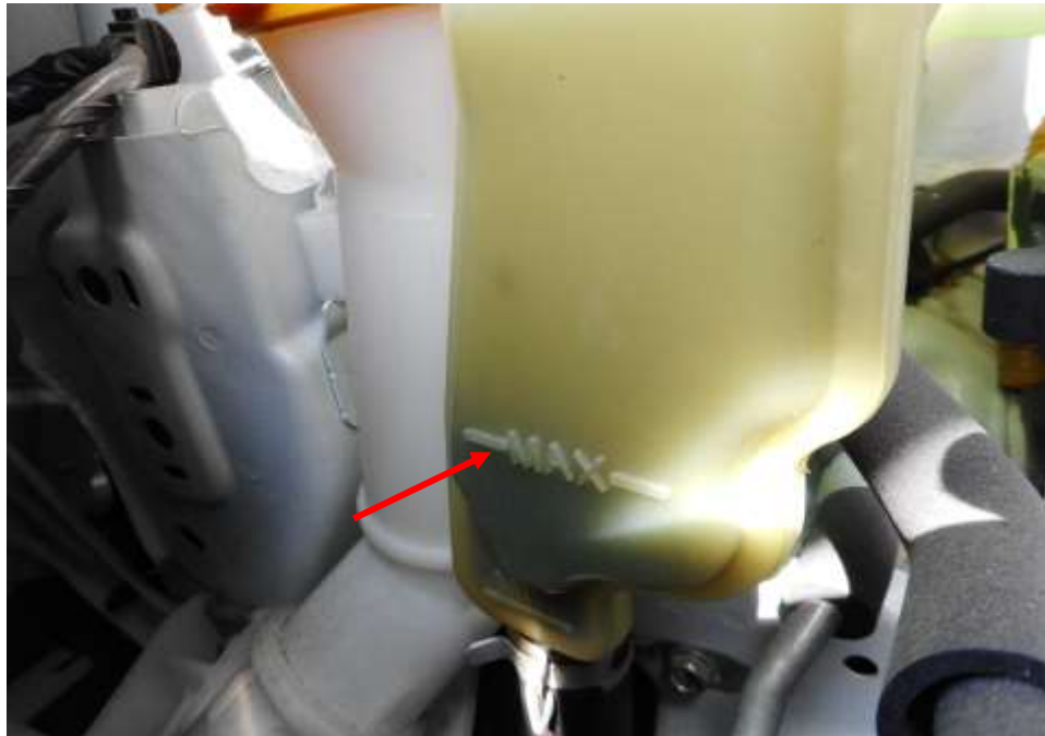
Photo 13 shows checks being carried out to the power steering fluid reservoir of the Motor Car at the time of my inspection. The steering fluid was observed to be of sufficient level (arrowed) and without any visible contamination.
