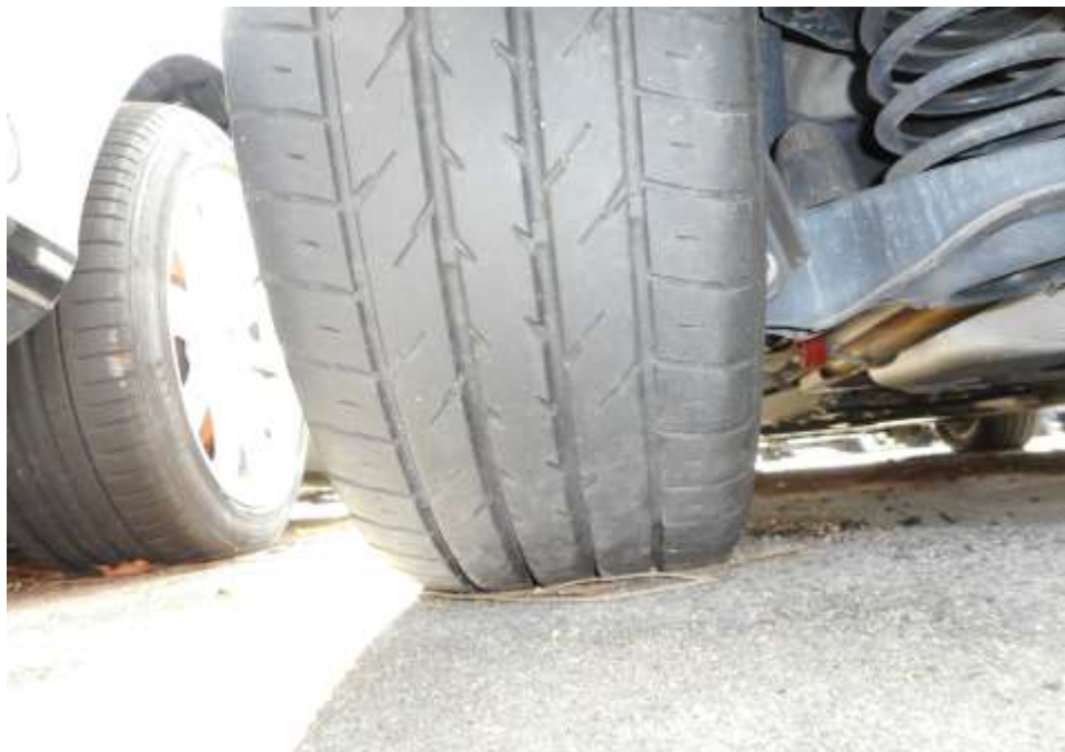
Photo 9 shows the condition of the rear left tyre of the Motor Car, which was observed to be in serviceable condition with remaining tread depth of approximately 5mm. There was also no tear, cut or burst mark(s) on the outer and the inner sidewalls as well as across the tread of the Motor Car's 4 tyres.
