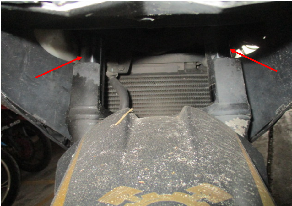
Photo 16 shows the front fork (arrowed) of the Motorcycle. The front fork and fork bracket of the Motorcycle were both found to be intact and undamaged. Turning the Motorcycle's handle bar towards the left and right did not produce any abnormal free play and/or resistance. The steering system of the Motorcycle was in serviceable condition at the time of our inspection.
