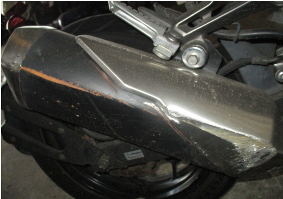
Photo 9 shows the exhaust muffler and exhaust muffler heat shield which were amongst the body parts of the Motorcycle that had sustained damage as a result of the accident.
