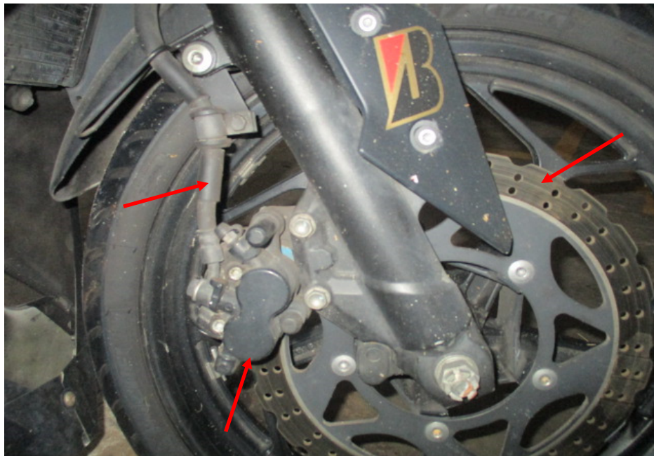
Photo 19 shows a close up view of the front brake caliper, front brake disc and front brake hose (arrowed) of the Motorcycle, which are all part of the components in the hydraulic front brake system of the Motorcycle. Our visual checks of these various components had revealed all to be intact with no visible damage. No leakage of brake fluid was also observed.
