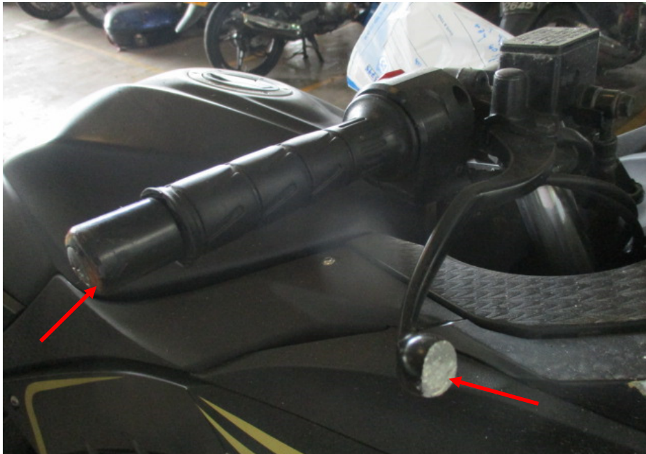
Photo 7 shows a closer view of the front brake lever and left handlebar end (arrowed) which were amongst the body parts of the Motorcycle that had sustained damage as a result of the accident.
