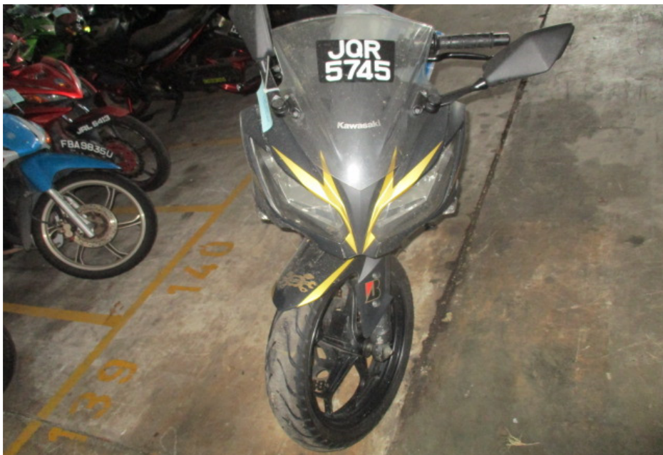
Photo 17 shows the front wheel of the Motorcycle turned towards its full right. Turning the Motorcycle's handle bar towards the left and right did not produce any abnormal free play and/or resistance. This would indicate that the steering system of the Motorcycle was in serviceable condition at the time of our inspection.
