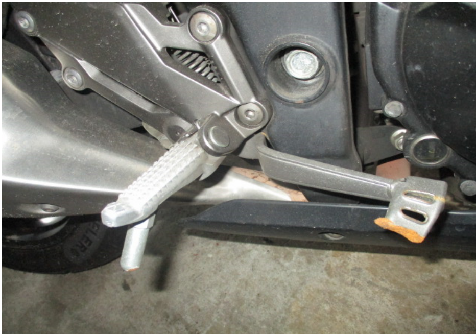
Photo 8 shows a closer view of the rear brake pedal and right front footrest, which were amongst the body parts of the Motorcycle that had sustained damage as a result of the accident.
