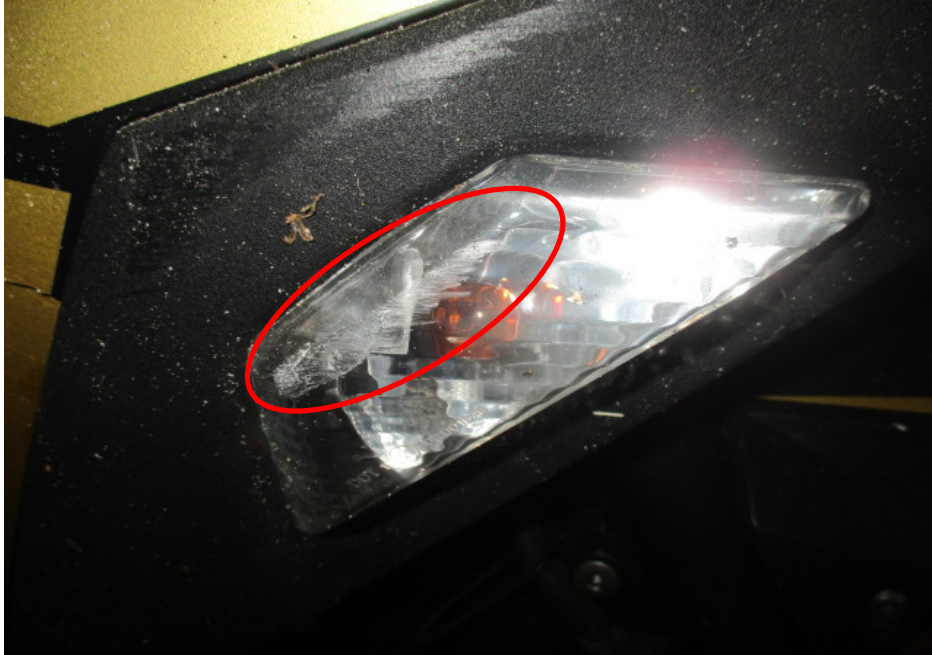
Photo 5 shows a close up view of the right front signal lamp (circled) which was amongst the body parts of the Motorcycle that had sustained damage as a result of the accident.
