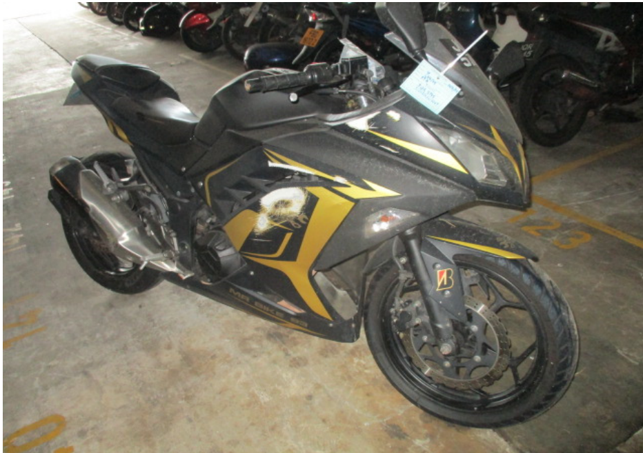
Photo 3 shows a general view of the right front body of the Motorcycle at the time of our inspection. The Motorcycle was observed to have sustained damages along its frontal and right portion. Amongst the body parts that were found to have been damaged include its head cowling, right side cowling, front brake lever, right front signal lamp, rear brake pedal, right front footrest, exhaust muffler and exhaust muffler heat shield, amongst others.
