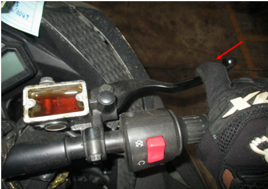
Photo 21 shows the front brake lever being depressed. There was some resistance felt (spongy like feel) upon pressing the front brake lever (arrowed). This would indicate that there is no leakage of pressure/vacuum in the brake system.
