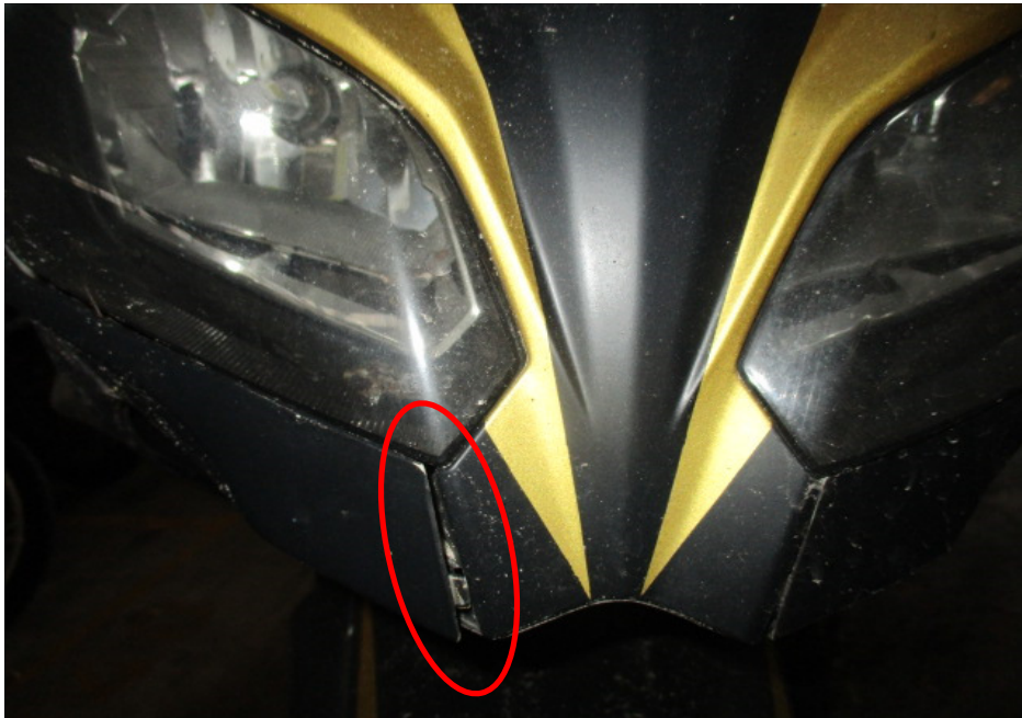
Photo 4 shows a closer view of the head cowling which was amongst the body parts at the front body of the Motorcycle that had sustained damage as a result of the accident (circled).
