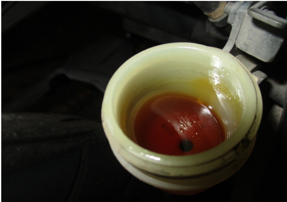
Photo 23 shows the brake fluid reservoir for the rear brake of the Motorcycle. The brake fluid was observed to be of sufficient level and without contamination for operational purposes.
