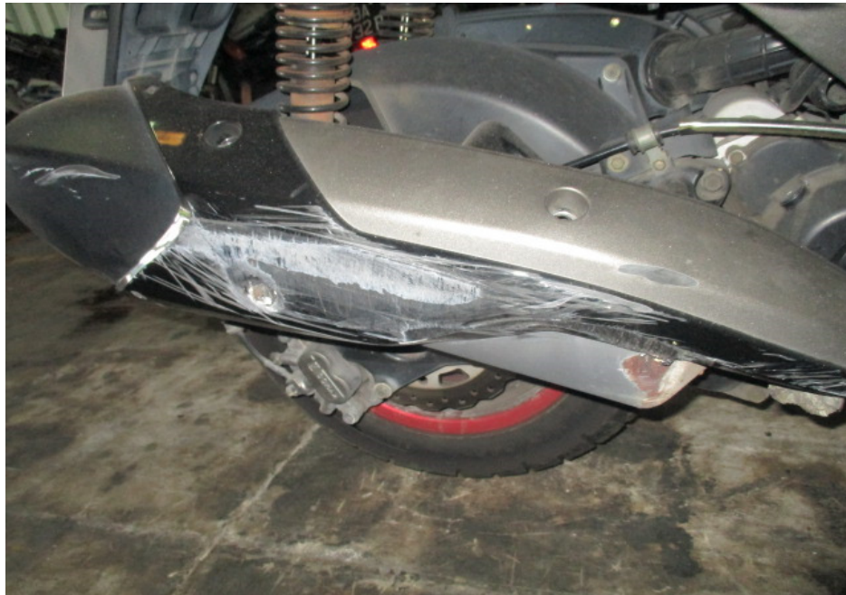
Photo 9 shows a closer view of the exhaust muffler and exhaust muffler heat shield of the Motorcycle which had sustained damage due to the accident.
