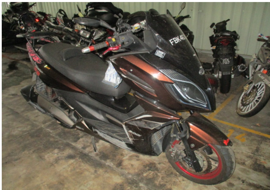
Photo 3 shows a general view of the right front body of the Motorcycle at the time of our inspection. The Motorcycle was observed to have sustained minor damages at the frontal and right portion. The body parts that were found to have been damaged include its front mudguard, front brake lever, right side mirror, right cowling, right pillion foot rest, exhaust muffler, exhaust muffler heat shield and top box rack, amongst others as a result of the accident.
