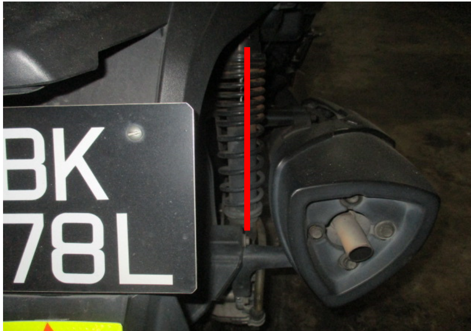
Photo 16 shows the right shock absorber of the motorcycle was found to be intact without any misalignment.
