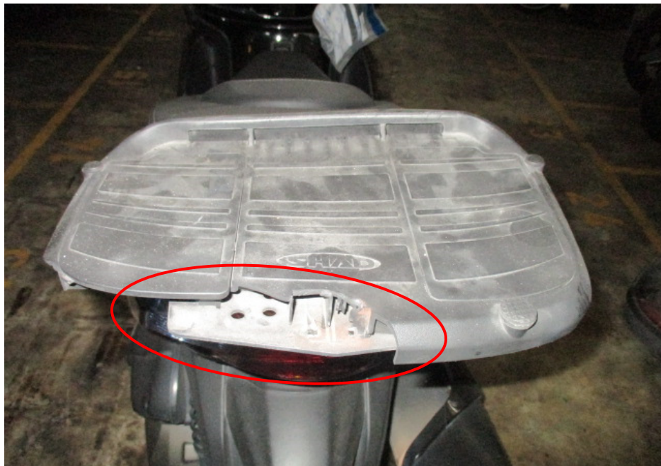
Photo 10 shows the broken top box rack of the Motorcycle (circled).
