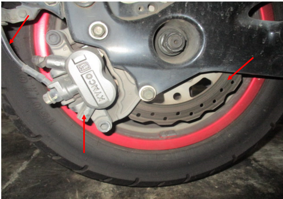
Photo 25 shows a close up view of the rear brake caliper, rear brake disc and rear brake hose (arrowed) of the Motorcycle, which are all part of the components in the hydraulic rear brake system of the Motorcycle. Our visual checks of these various components revealed all to be intact with no visible damage. No leakage of brake fluid was also observed.
