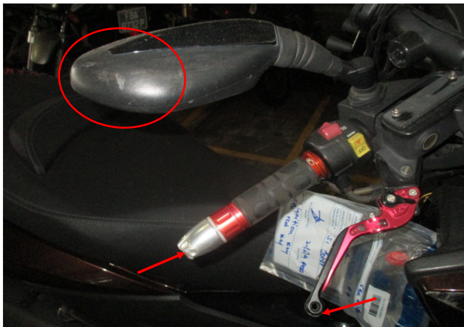
Photo 7 shows a closer view of the front brake lever and right handlebar end (arrowed) as well as the right side mirror (circled) of the Motorcycle which were observed to be damaged due to the accident
