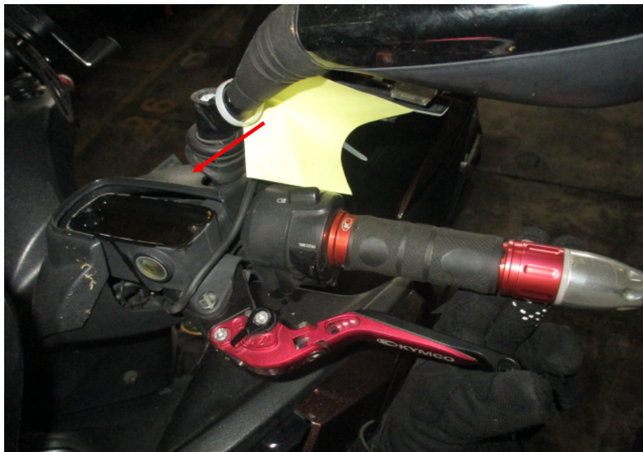
Photo 23 shows the rear brake lever being depressed. There was some resistance felt (spongy like feel) upon pressing the rear brake lever (arrowed). This would indicate that there is no leakage of pressure/vacuum in the brake system.
