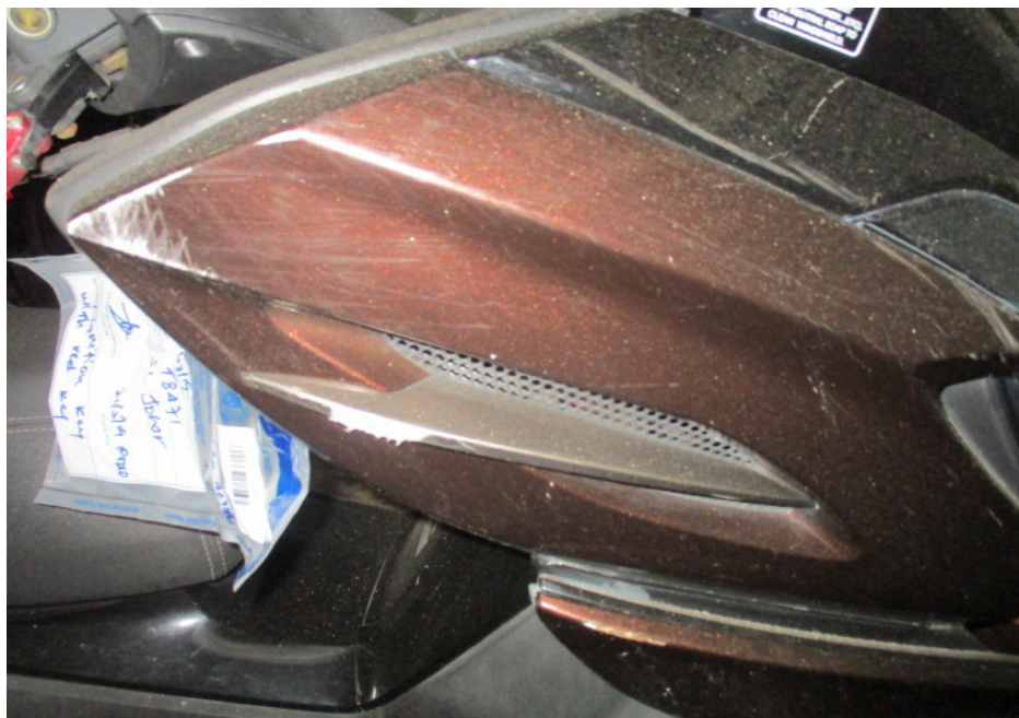
Photo 5 shows a closer view of the right cowling which was amongst the body parts at the front body of the Motorcycle that had sustained damage as a result of the accident.
