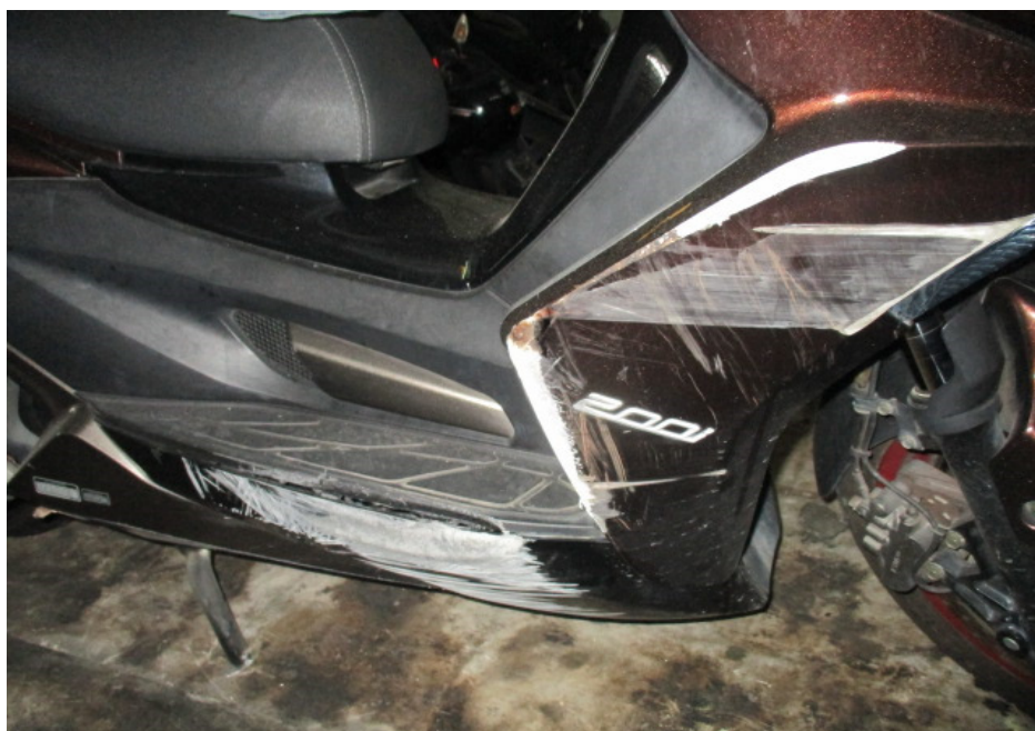
Photo 6 shows a closer view of the right bottom cowling of the Motorcycle which was observed to be damaged due to the accident.
