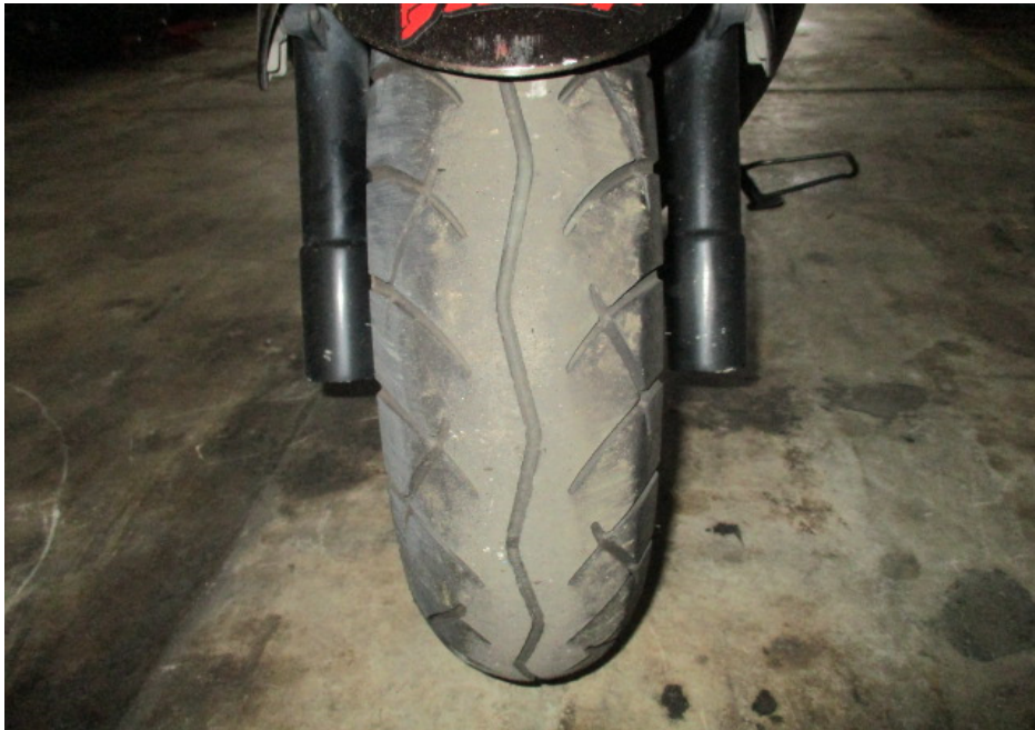
Photo 11 shows the condition of the Motorcycle's front tyre. The front tyre was observed to be in serviceable condition with remaining tread depth of approximately 3mm. There was no tear, burst mark(s) and/or punctured hole(s) on the sidewalls as well as across the tread of the front tyre.
