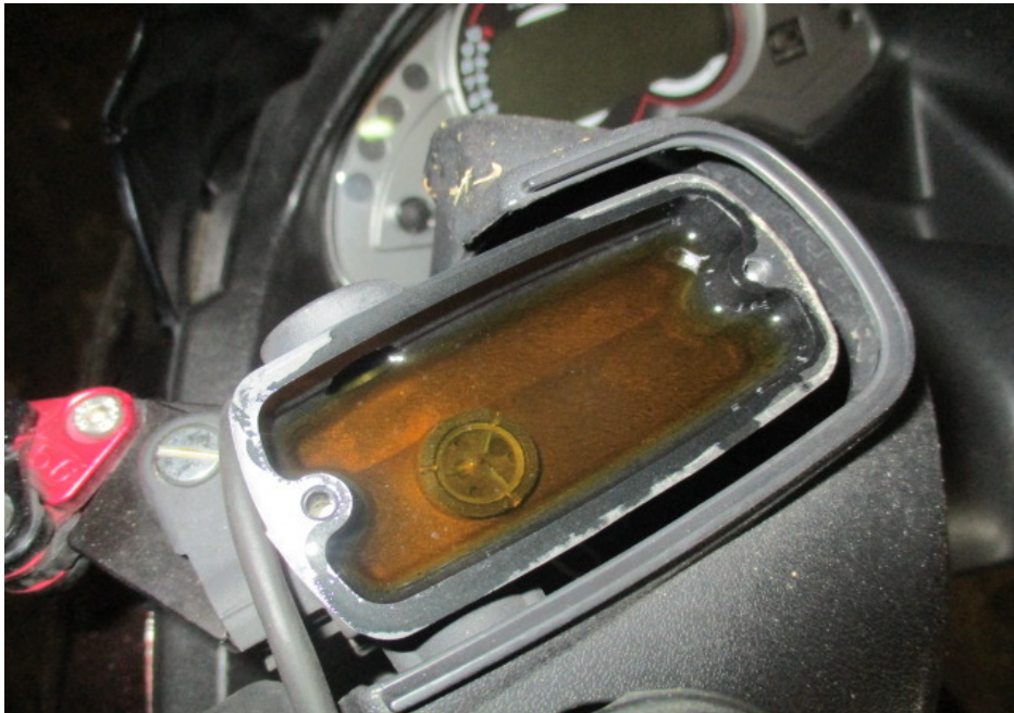
Photo 24 shows a close up view of the brake fluid reservoir for the rear brake of the Motorcycle. The brake fluid was observed to be of sufficient level and without contamination for operational purposes.
