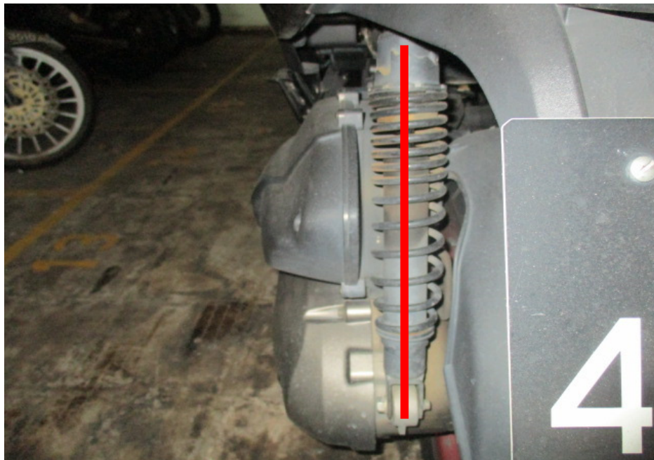
Photo 15 shows the left shock absorber of the motorcycle was found to be intact without any misalignment.
