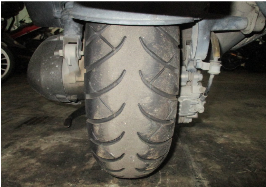
Photo 12 shows the condition of the Motorcycle's rear tyre. The rear tyre was observed to be in serviceable condition with remaining tread depth of approximately 5mm. The tyre was also observed to be sufficiently inflated for vehicular operation. We did not observe any tear, burst mark(s) and/or punctured hole(s) on the sidewalls as well as across the tread of the rear tyre.
