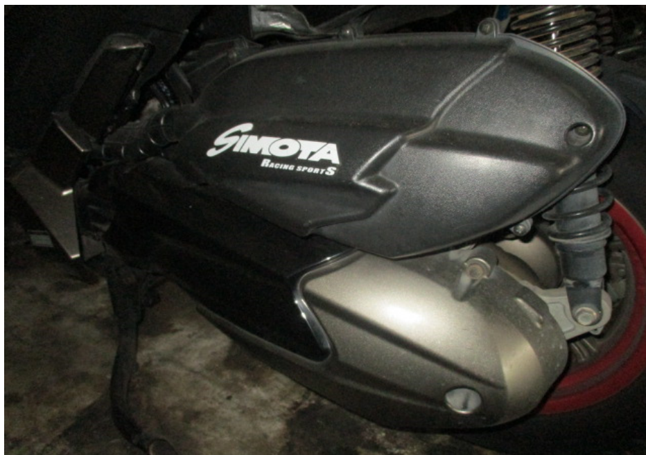
Photo 14 shows the drive train of the Motorcycle which was found to be intact without any misalignment.
