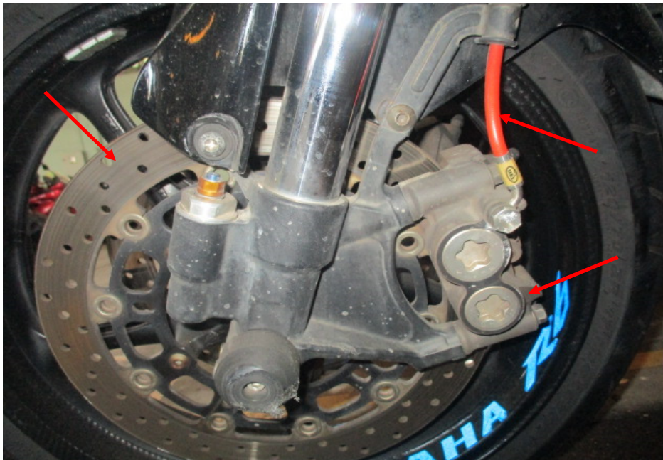
Photo 26 shows a close up view of the front brake caliper, front brake disc and front brake hose (arrowed) at the left side of the Motorcycle's front wheel, which are all part of the components in the hydraulic front brake system of the Motorcycle. Our visual checks of these various components had revealed all to be intact with no visible damage. No leakage of brake fluid was also observed.
