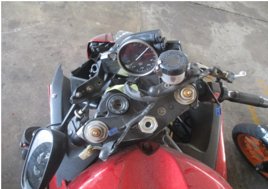
Photo 6 shows a close up view of the front brake lever, front brake fluid reservoir, side mirrors, clutch lever, handlebars and handlebar ends of the Motorcycle. These parts were amongst the body parts of the Motorcycle which were damaged as a result of the accident.
