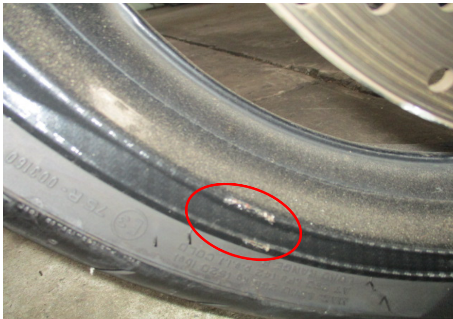
Photo 14 shows the front wheel rim of the Motorcycle at the time of our inspection. Some relatively minor marks of grazing nature were observed on the edges of the front wheel rim (circled), at the left side of the Motorcycle.
