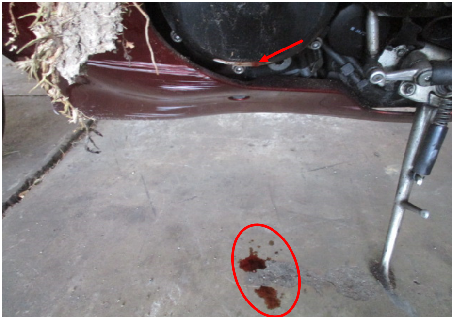
Photo 19 shows wet fluid stains observed on the ground (circled) directly below the damaged left engine cover of the Motorcycle (arrowed), indicating that a fluid leak had occurred as a result of the accident.
