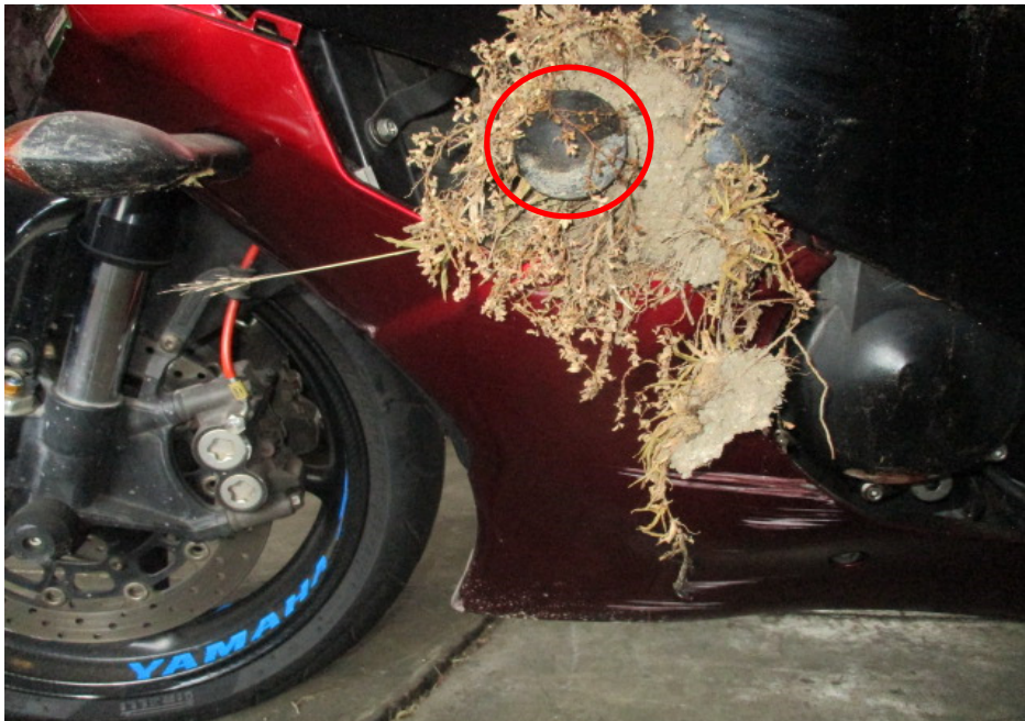
Photo 10 shows a closer view of the left side cowling and left front frame slider (circled), which were amongst the body parts of the Motorcycle that had sustained damage as a result of the accident.
