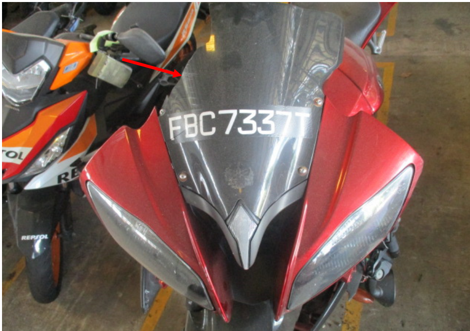
Photo 4 shows a closer view of the head cowling and windshield (arrowed) of the Motorcycle which had sustained damages as a result of the accident.
