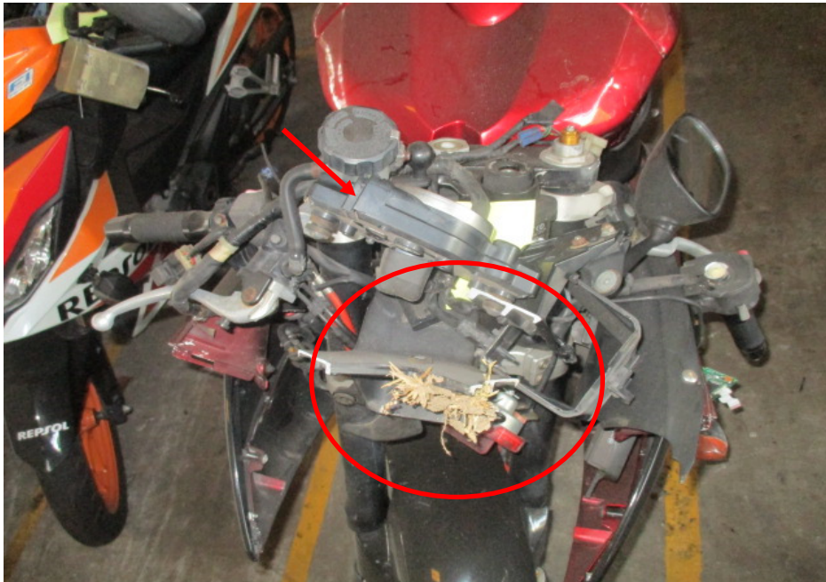
Photo 5 shows a closer view of the headlamp assembly (circled) and speedometer gauge (arrowed) which were amongst the body parts at the front body of the Motorcycle that had sustained damage as a result of the accident.
