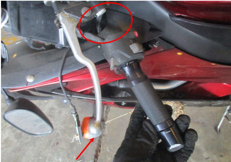
Photo 7 shows a closer view of the clutch lever (arrowed) and broken left handlebar (circled) which were amongst the body parts at the front body of the Motorcycle that had sustained damage as a result of the accident.
