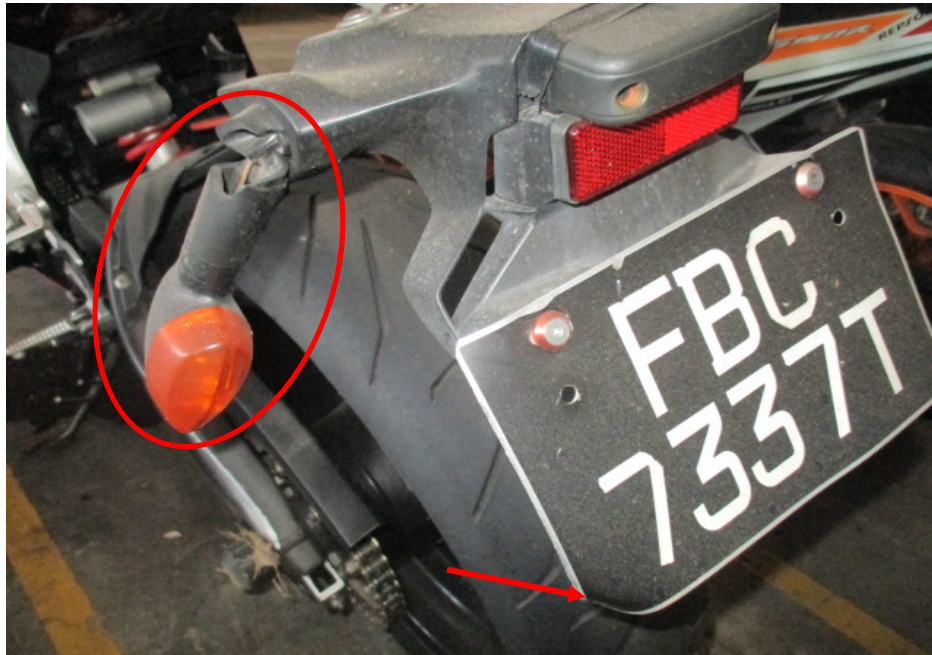
Photo 13 shows the dislodged left rear signal lamp (circled) and dented rear number plate of the Motorcycle as a result of the accident.
