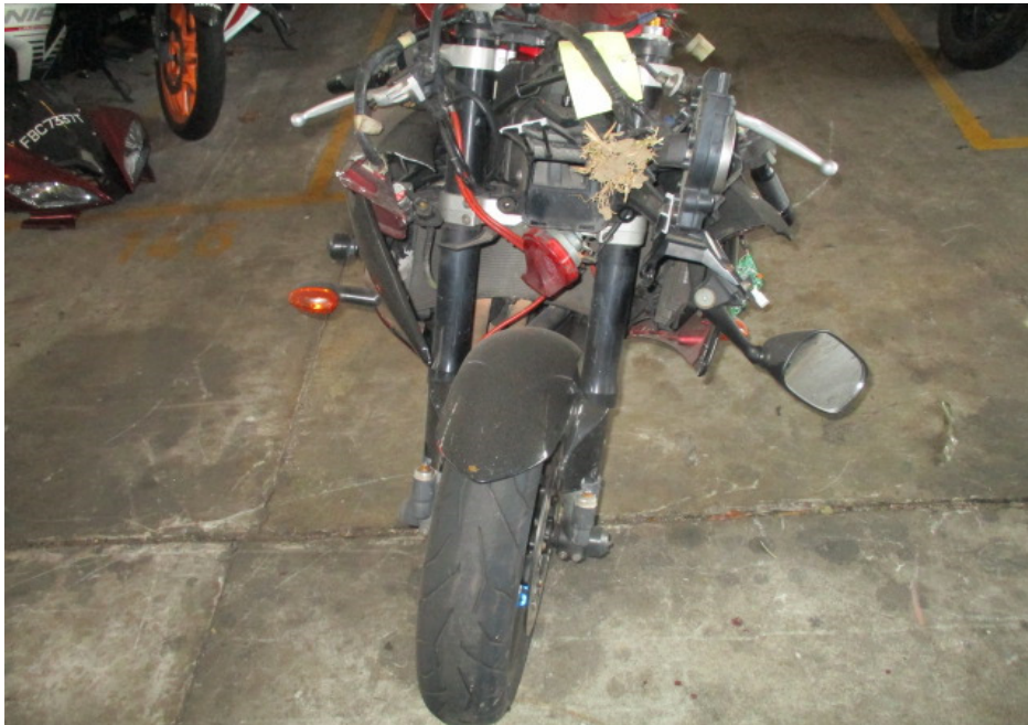
Photo 23 shows the front wheel of the Motorcycle turned slightly towards the right. We were unable to fully turn the handle bar towards the right due to the resistance from the broken components of the head cowl which were found to be pushed inwards as a result of the accident.
