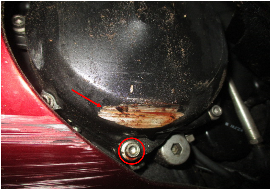
Photo 18 shows the left side of the engine of the Motorcycle at the time of our inspection. The various left engine components had sustained damage of grazing nature as a result of the accident (arrowed). Wet fluid stains were observed on the underside of the damaged left engine cover of the Motorcycle (circled).
