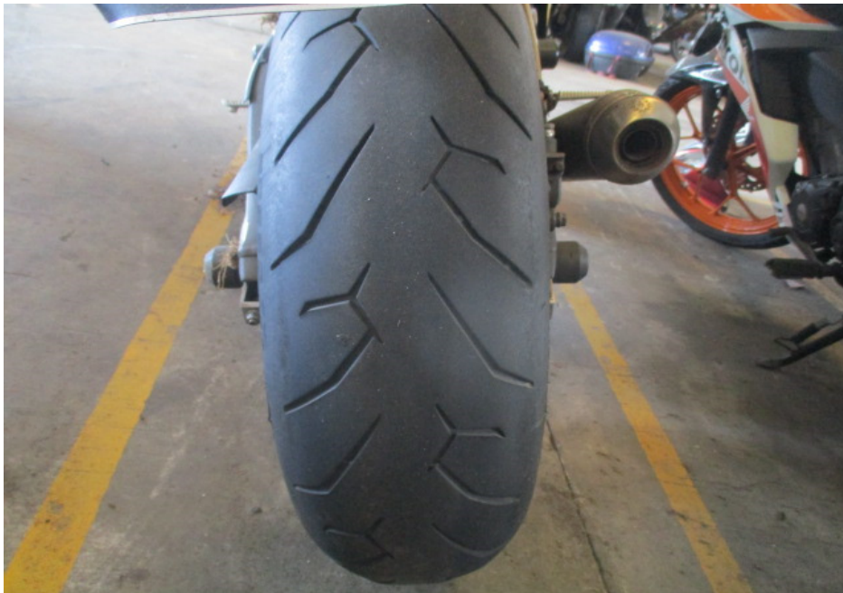
Photo 16 shows the condition of the Motorcycle's rear tyre. The rear tyre was observed to be in serviceable condition with remaining tread depth of approximately 3mm. The tyre was also observed to be sufficiently inflated for vehicular operation. We did not observe any tear, burst mark(s) and/or punctured hole(s) on the sidewalls as well as across the tread of the rear tyre.
