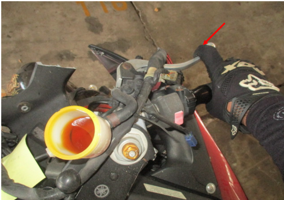
Photo 28 shows the front brake lever being depressed. There was some resistance felt (spongy like feel) upon pressing the front brake lever (arrowed). This would indicate that there is no leakage of pressure/vacuum in the brake system.
