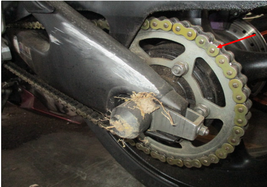
Photo 20 shows the gear chain (arrowed) of the Motorcycle, which was observed to be intact with no misalignment. It was also adequately lubricated for operating purposes. The gear chain rotates the rear wheel of the Motorcycle.
