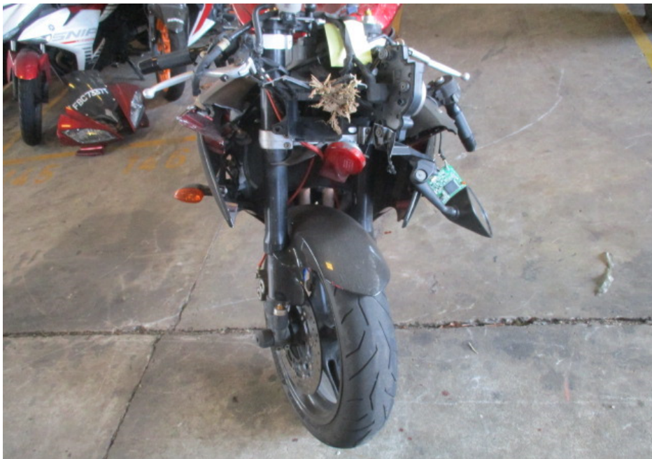
Photo 24 shows the front wheel of the Motorcycle turned towards its full left. Turning the Motorcycle's handle bar towards the left did not produce any abnormal free play and/or resistance. This would indicate that the steering system of the Motorcycle was in serviceable condition at the time of our inspection.
