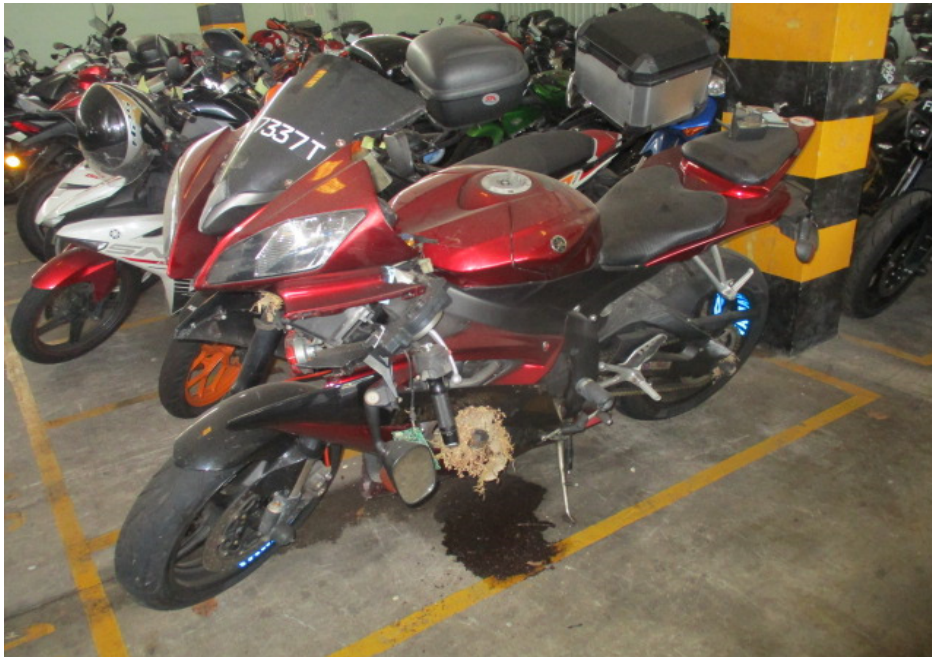
Photo 3 shows a general view of the left front body of the Motorcycle at the time of our inspection. The Motorcycle was observed to have sustained damages at its frontal and left portion. The body parts that were found to have been damaged include its headlamp assembly, head cowling, speedometer gauge, side mirrors, handlebars, petrol tank, left side cowling, frame sliders, gear shift pedal, left signal lamps and rear number plate, amongst others.
