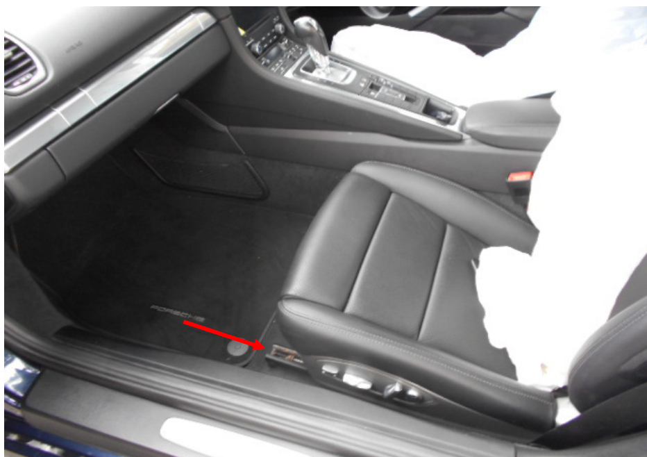
Photo 6 shows the front left seat of the Motor Car. The Motor Car is a 2-seater type of Motor Car. The 2 seats were secured via seat rails (arrowed) to the floor board. The seats were also fitted with a retractable seat belt reel and pretensioner. The seat belts were tested and able to be fastened into the respective pretensioners that were fitted on the side of each individual seat.
