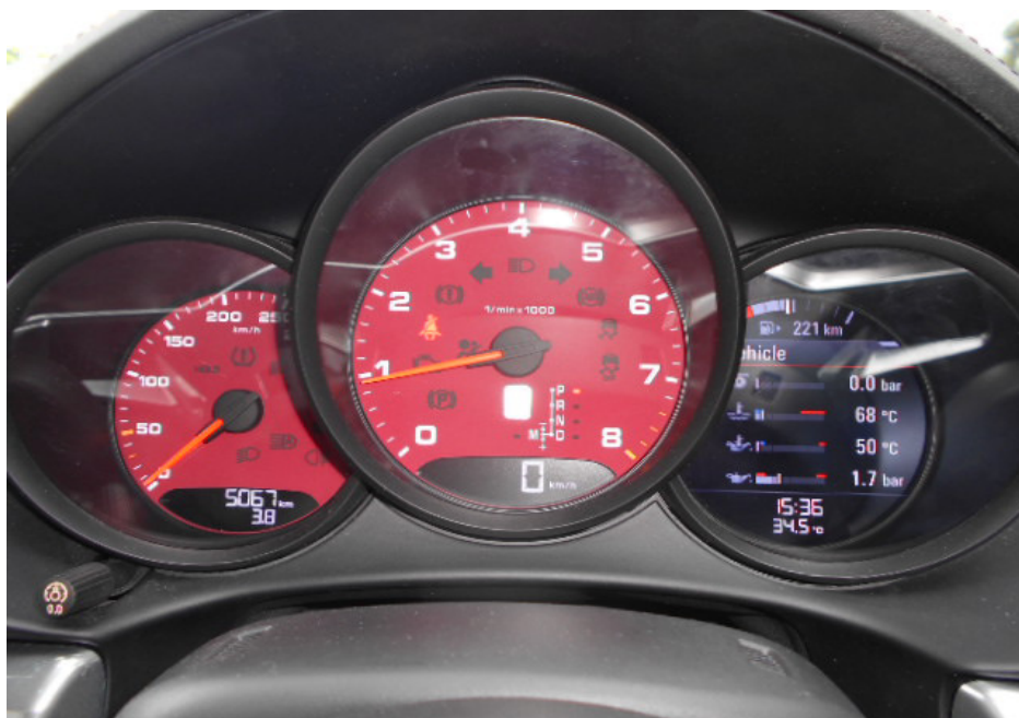
Photo 8 shows the respective warning lights no longer illuminated, indicating that there is no fault detected to the ABS, TPM and TCS systems of the Motor Car during the self-test. These electronic systems were hence in working condition at the time of my inspection.
