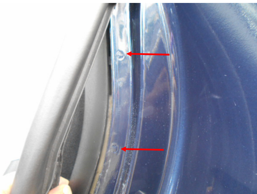
Photo 17 shows the rear left "C" pillar of the Motor Car. I did not find any weld marks other than original spot weld marks (arrowed) on the body panels of the Motor Car, indicating that there was no re-welding works carried out; and that the body panels of the Motor Car were originally fitted.
