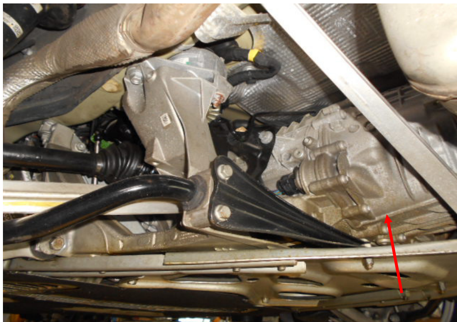
Photo 5 shows a general view of the transmission assembly (arrowed) of the Motor Car. My visual observations of the engine assembly and transmission assembly of the Motor Car revealed both to be fitted securely and not mounted onto the chassis body of the Motor Car.
