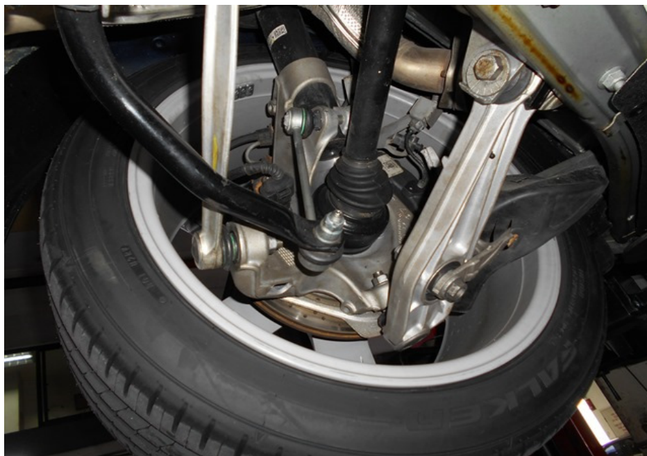
Photo 11 shows the various undercarriage components at the rear left wheel of the Motor Car. The mechanical components, control arms and linkages were all found to be intact and secured in an appropriate manner.
