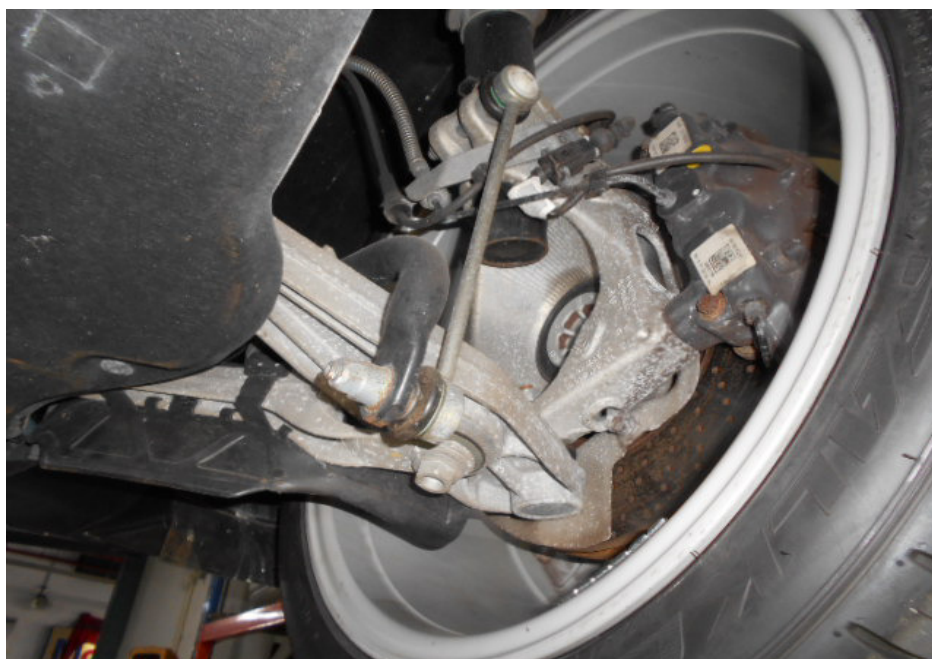
Photo 12 shows the various undercarriage components at the front right wheel of the Motor Car. The mechanical components, control arms and linkages were all found to be intact and secured in an appropriate manner. I did not observe any fluid leak and/or fluid stain on the underside of the Motor Car.
