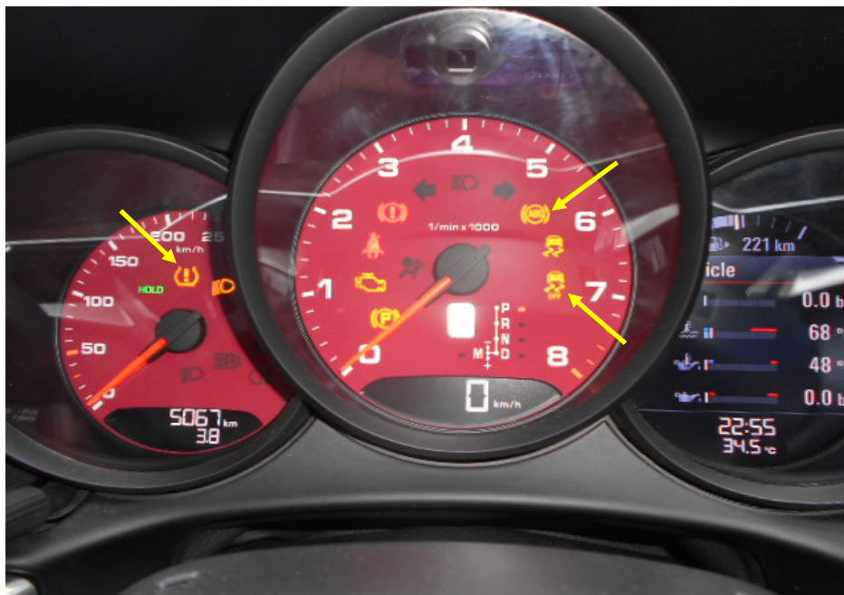
Photo 7 shows the warning lights for the various electronic safety features appearing on the instrument panel of the Motor Car during its self-test when the engine is cranked, in particular the ABS, TPM and TCS lights (arrowed).
