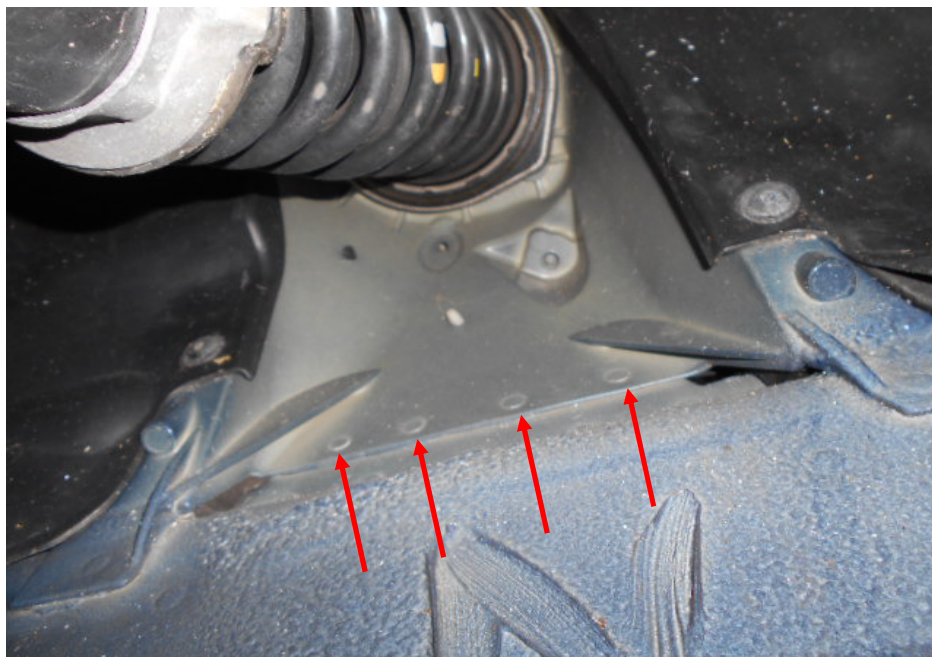
Photo 13 shows the structural body at the front left chassis of the Motor Car. Visually, I did not find any weld marks other than original spot weld marks (arrowed) at the joints along the chassis. This would indicate that no work was done on the chassis body of the Motor Car and that the chassis body was originally fitted.
