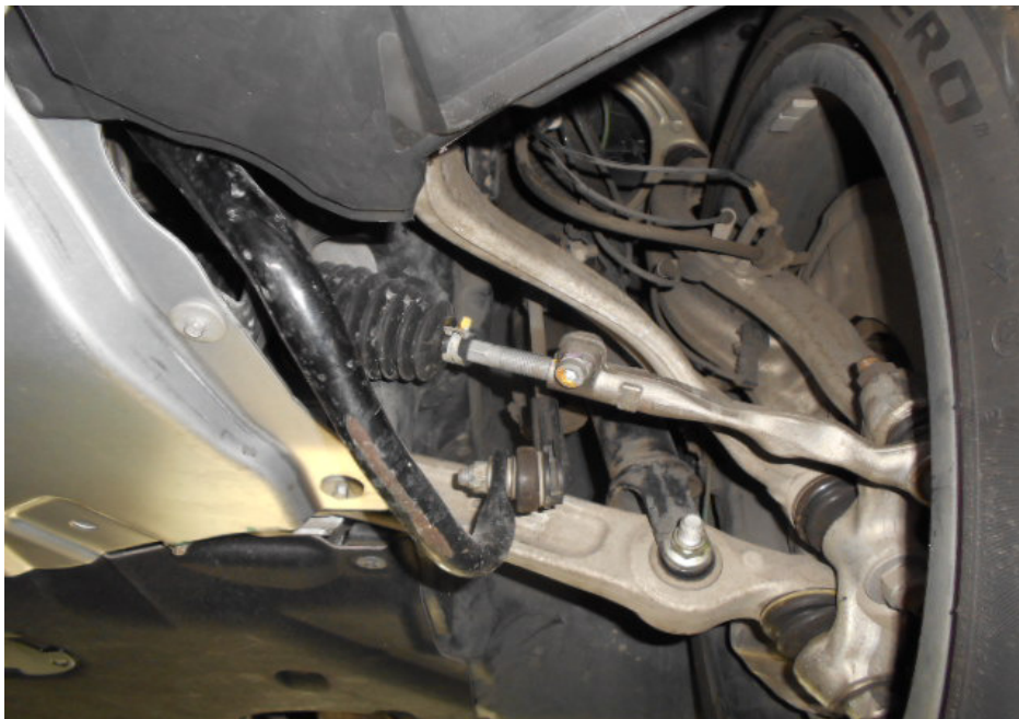
Photo 10 shows the various undercarriage components at the front left wheel of the Motor Car. The mechanical components, control arms and linkages were all found to be intact and secured in an appropriate manner.
