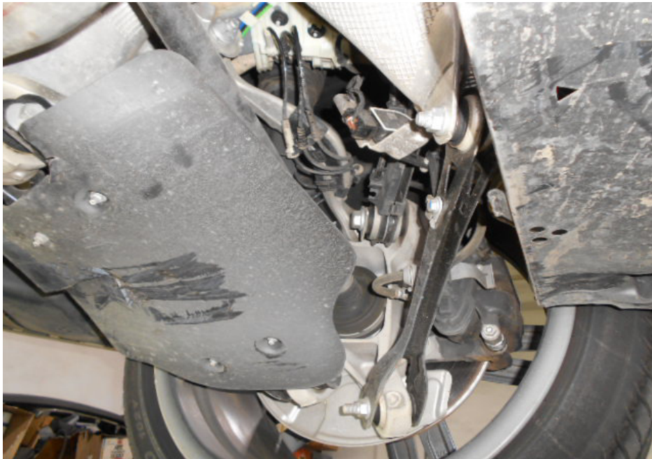
Photo 9 shows a general view of the control arms and linkages at the rear left wheel of the Motor Car. I did not observe any fluid leak and/or fluid stain on the underside of the Motor Car. All of the Motor Car's undercarriage components were observed to be intact and secured in an appropriate manner.
