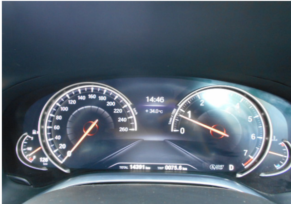
Photo 7 shows the respective warning lights no longer illuminated, indicating that there is no fault detected to the ABS, SRS, IAS, TPM and DSC systems of the Motor Car during the self-test. These electronic systems were hence in working condition at the time of my inspection.
