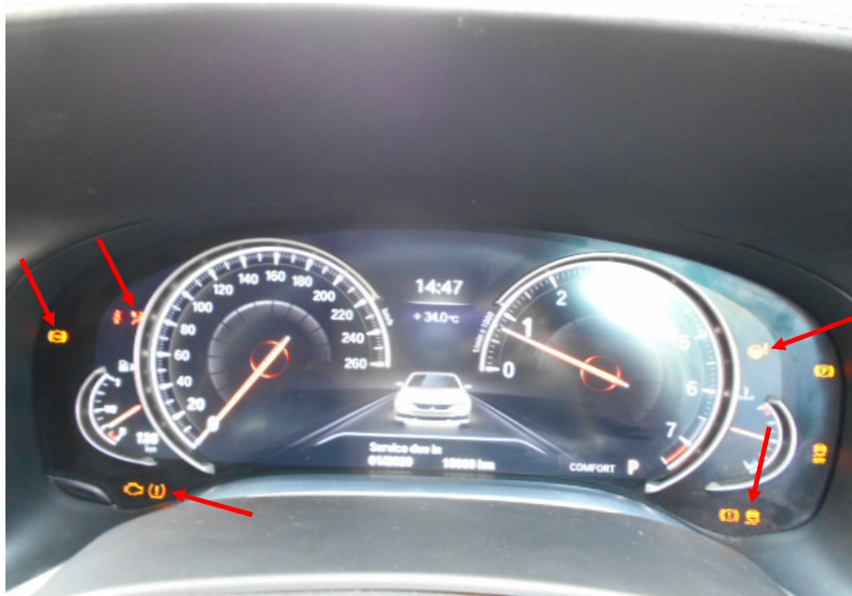
Photo 6 shows the warning lights for the various electronic safety features appearing on the instrument panel of the Motor Car during its self-test when the engine is cranked, in particular the ABS, SRS, IAS, TPM and DSC lights (arrowed).
