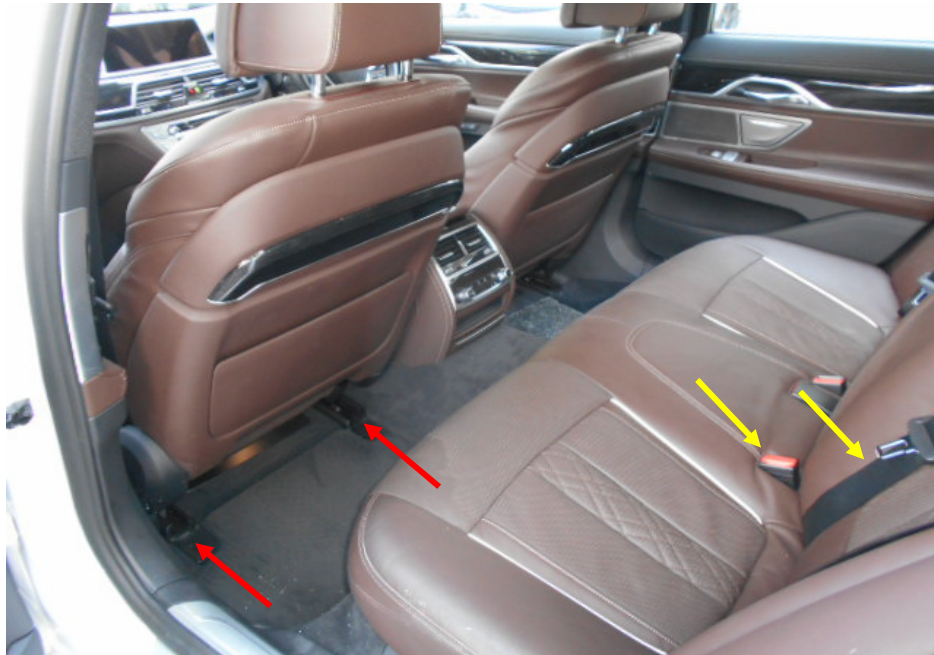
Photo 5 shows the seats of the Motor Car, which were secured via seat rails (red arrows) to the floor board. All the seats of the Motor Car were fitted with a retractable seat belt reel and pre-tensioner (yellow arrows). The seat belts were also able to be fastened into the respective pretensions that were fitted on the side of each individual seat.
