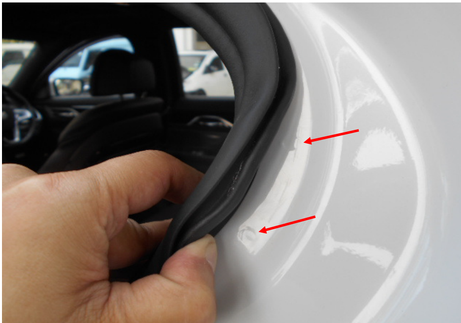
Photo 16 shows the rear left "C" pillar of the Motor Car. I did not find any weld marks other than original spot weld marks (arrowed) on the body panels of the Motor Car, indicating that there was no re-welding works carried out; and that the body panels of the Motor Car were originally fitted.
