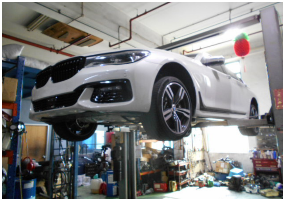
Photo 8 shows the Motor Car hoisted up for checks on its undercarriage. There was no sign(s) or indication(s) of fluid leakage and/or fluid stain(s) on the underside of the Motor Car. The undercarriage components of the Motor Car were also all observed to be intact and secured in an appropriate manner.
