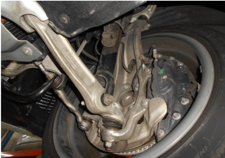
Photo 11 shows the various undercarriage components at the front right wheel of the Motor Car. The mechanical components, control arms and linkages were all found to be intact and secured in an appropriate manner.
