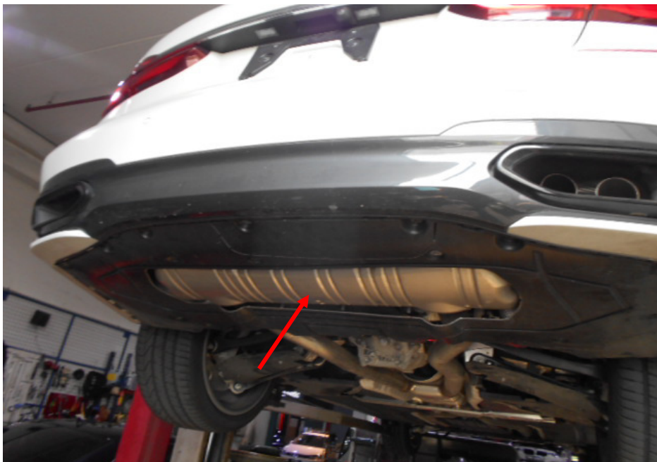
Photo 12 shows the Motor Car's rear exhaust muffler (arrowed). My examination of the Motor Car's exhaust system revealed no sign(s) or indication(s) of any cut or weld marks along its exhaust pipes and on its rear mufflers.
