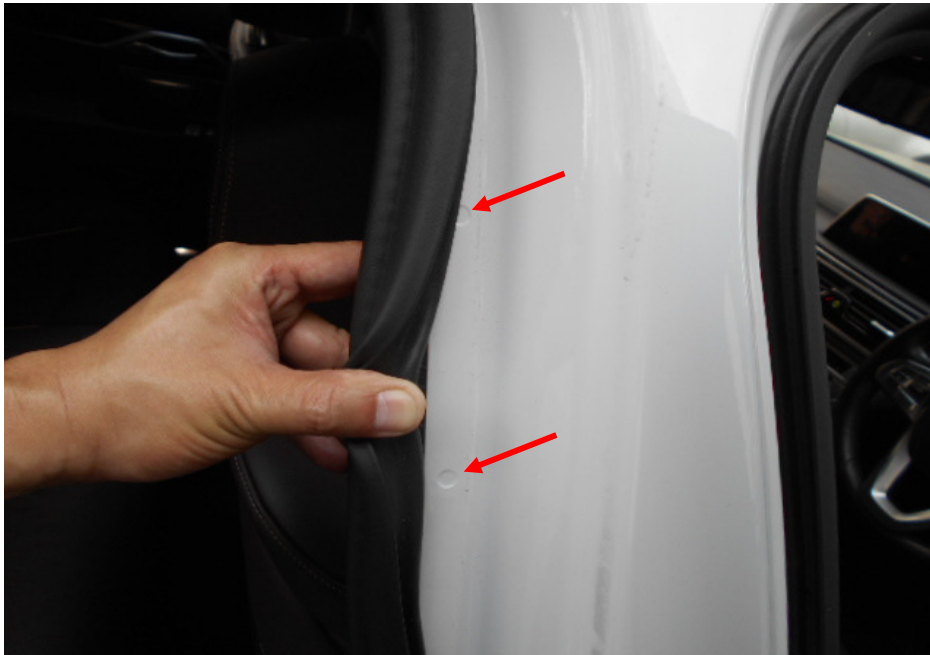
Photo 17 shows the right “B” pillar of the Motor Car. I did not find any weld marks other than original spot weld marks (arrowed) on the body panels of the Motor Car, indicating that there was no re-welding works carried out; and that the body panels of the Motor Car were originally fitted.
