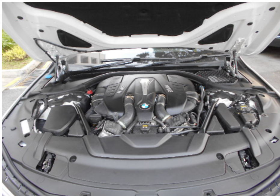
Photo 4 shows a general view of the engine compartment of the Motor Car at the time of my inspection. The various parts and components inside the engine compartment were all observed to be intact and properly fitted. There was also no sign(s) or indication(s) of fluid leak and/or fluid stain found inside the engine compartment.
