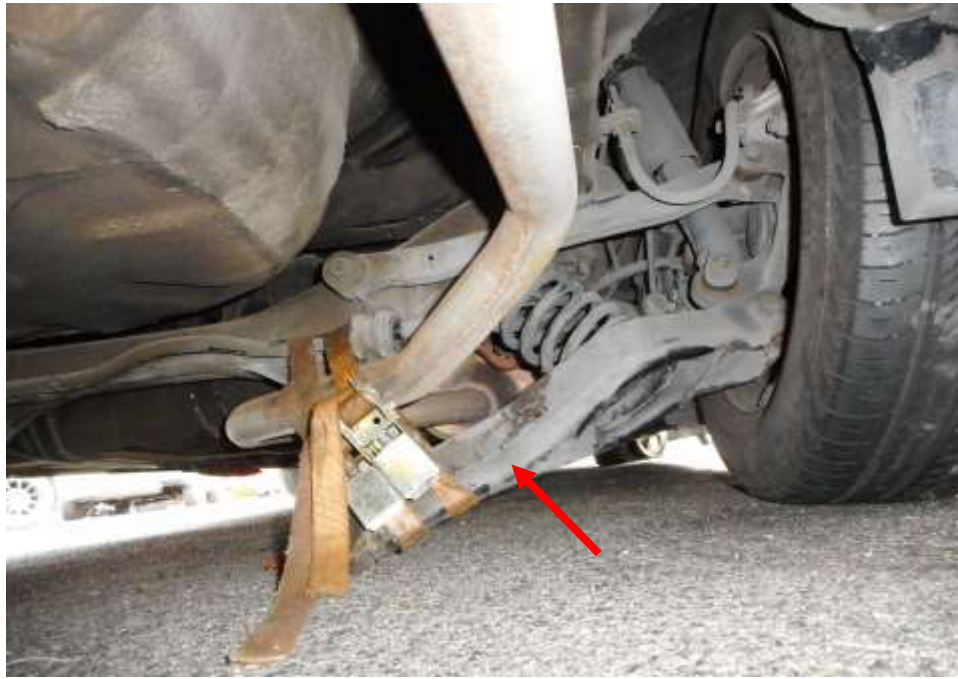
Photo 11 shows the close up view of the rear right suspension system of the Motor Car at the time of my inspection. The rear right lower arm (arrowed) of the Motor Car was observed to have been damaged as a result of the accident.
