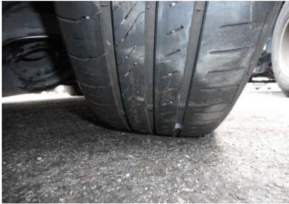
Photo 15 shows the condition of the rear right tyre of the Motor Car, which was observed to be in serviceable condition with remaining tread depth of approximately 4.3mm. There was no tear, cut or burst mark(s) on the outer and the inner sidewalls as well as across the tread of this tyre, however observed to sustained minor scratches to the rim as a result of the accident.
