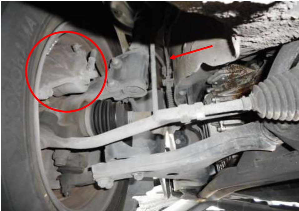
Photo 22 shows the brake hose (arrowed) at the front left wheel of the Motor Car. I did not observe any leakage of brake fluid at the 4 wheels of the Motor Car. My visual inspection of the various mechanical components of the Motor Car's braking system, including its brake caliper (circled), revealed all to be intact and without visible damage.
