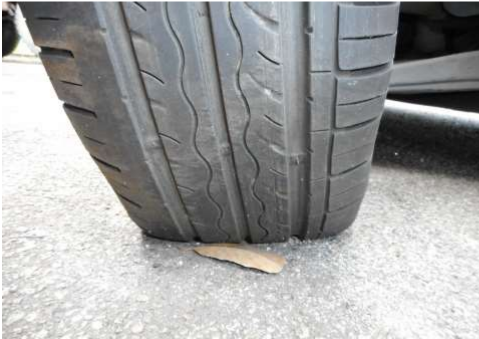
Photo 13 shows the condition of the rear left tyre of the Motor Car, which was observed to be in serviceable condition with remaining tread depth of approximately 4.6mm. There was no tear, cut or burst mark(s) on the outer and the inner sidewalls as well as across the tread of this tyre, however observed to be deflated due to damage to the rims.
