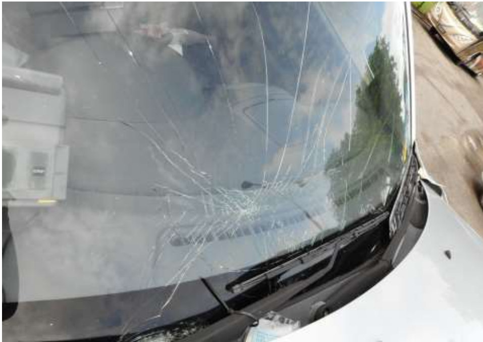
Photo 3 shows a close up view of the front windscreen of the Motor Car at the time of my inspection. The front windscreen of the Motor Car was observed to have been damaged as a result of the accident
