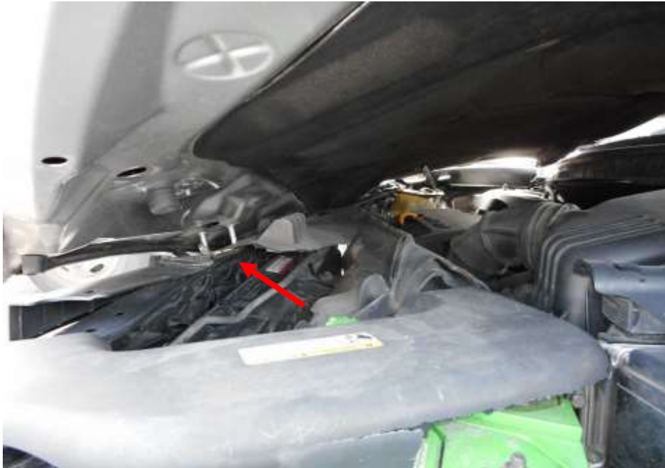
Photo 18 shows the damage to the locking mechanism (arrowed) Motor Car's front bonnet, rendering it unable to be unlocked and lifted up to carry out examination of the Motor Car's engine compartment as a result of the accident.
