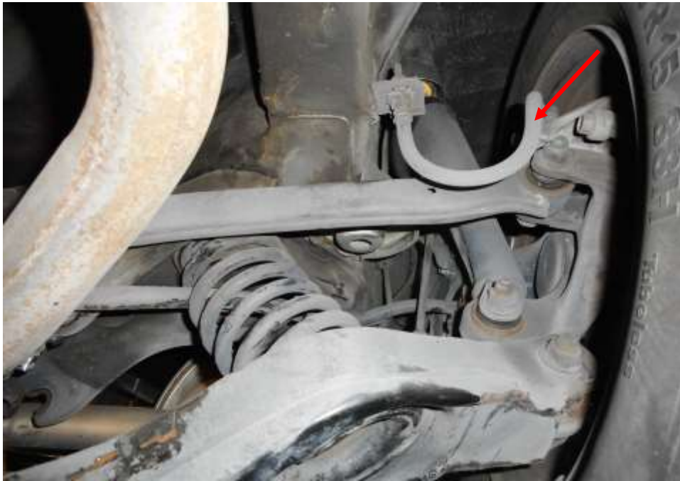
Photo 23 shows the various undercarriage components at the rear right wheel of the Motor Car, in particular the brake hose (arrowed). I did not observe any leakage of brake fluid at the 4 wheels of the Motor Car. My visual inspection of the various mechanical components of the Motor Car's braking system revealed all to be intact and without visible damage.
