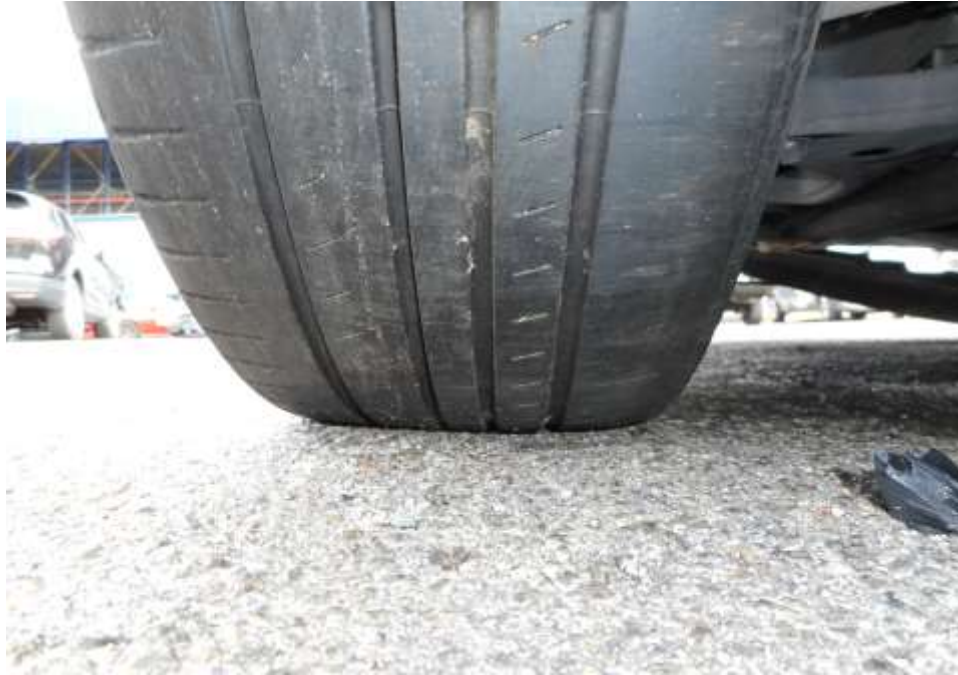
Photo 17 shows the condition of the front left tyre of the Motor Car, which was observed to be in serviceable condition with remaining tread depth of approximately 3.6mm. There was no tear, cut or burst mark(s) on the outer and the inner sidewalls as well as across the tread of this tyre, however observed to be deflated due to damage to the rims.
