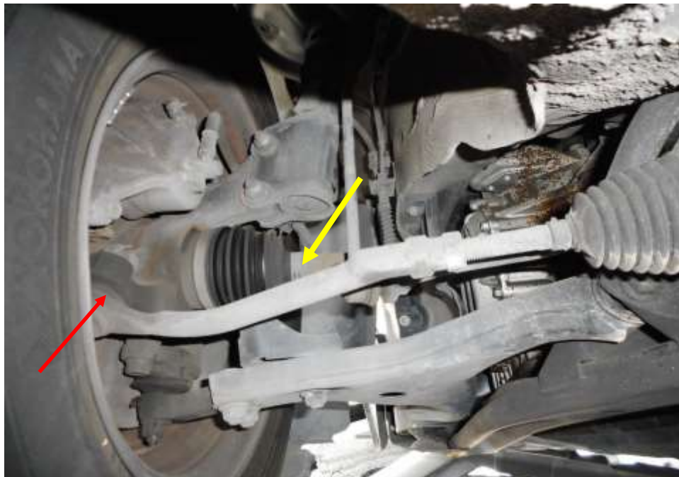
Photo 20 shows the various undercarriage components at the front left wheel of the Motor Car, which had included the steering tie rod (red arrow) and front left drive shaft (yellow arrow). The various undercarriage components of the Motor Car were all found to be intact without any visible damage.
