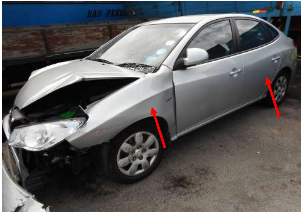
Photo 9 shows a general view of the front left portion of the Motor Car at the time of my inspection. The front left fender and the rear left body panel (arrowed) of the Motor Car was observed to have been damaged as a result of the accident.
