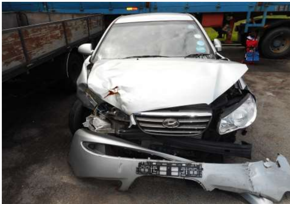
Photo 2 shows a general view of the front portion of the Motor Car at the time of my inspection. The Motor Car was also observed to have sustained extensive impact damage at its frontal and undercarriage portion, damaged parts had included its front windscreen, front bonnet, both front bonnet hinges, bonnet lock mechanism, front bumper, front number plate, left and right fenders, rear left body panel, engine system, radiator, front right headlamp and its undercarriage rear right lower arm were amongst the body parts that were observed to have been damaged as a result of the accident.
