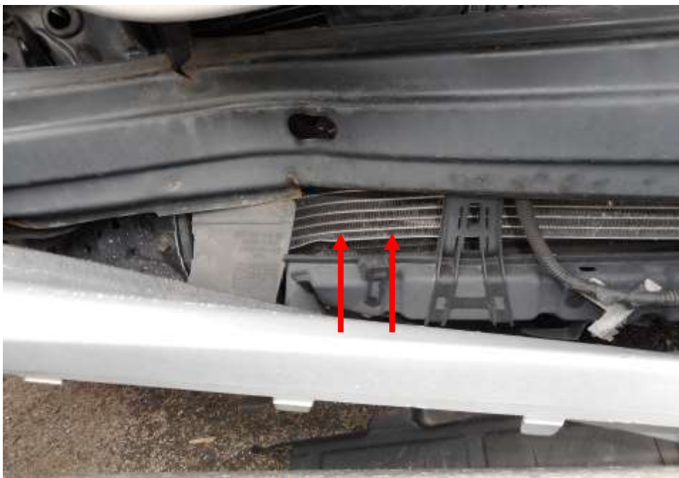
Photo 6 shows a close up view of the front portion of the Motor Car at the time of my inspection. The radiator of the Motor Car was observed to have been damaged by an induced impact as a result of the accident
