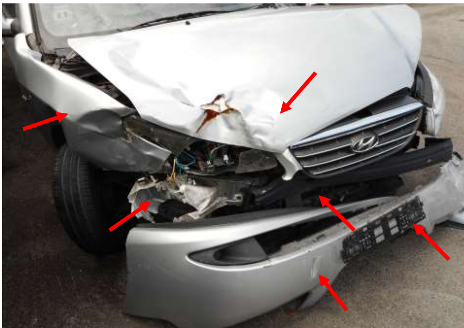
Photo 4 shows a general view of the front right portion of the Motor Car at the time of my inspection. The Motor Car was also observed to have sustained extensive impact damage at its frontal portal, damaged parts had included its, front bonnet, front bumper, right fender, engine system, radiator, front right headlamp (arrowed) were amongst the body parts that were observed to have been damaged as a result of the accident.
