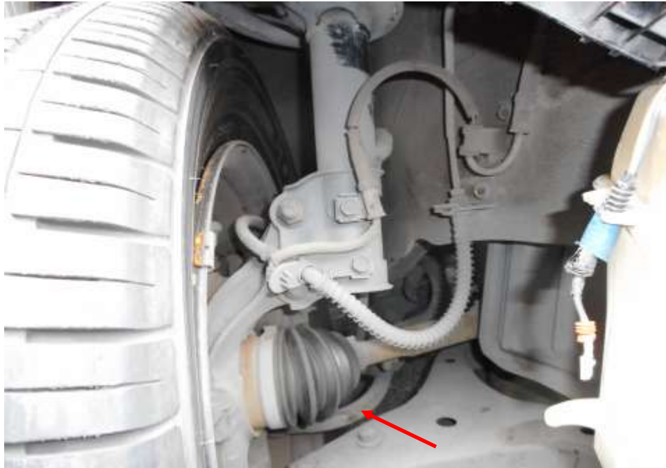
Photo 19 shows the undercarriage components at the front right wheel of the Motor Car. My checks on the underside of the Motor Car revealed damage to the various undercarriage components, the steering rack and pinion, tie rods, tie rod ends and ball joints (arrowed) revealed that these components were all generally in good condition.
