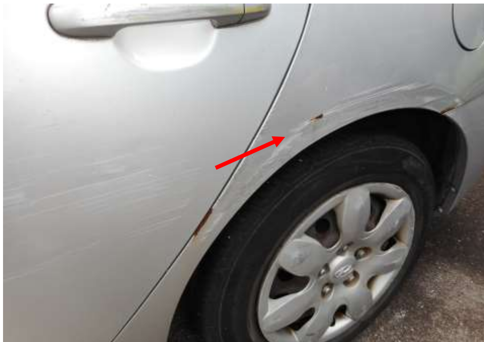
Photo 10 shows the close up view of the rear left panel portion of the Motor Car at the time of my inspection. The rear left body panel (arrowed) of the Motor Car was observed to have been damaged as a result of the accident.
