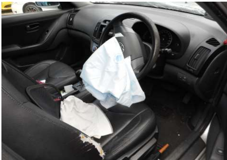
Photo 12 shows a general view of the Motor Car's interior compartment. The driver's air bag, were also deployed as a result of the accident.
