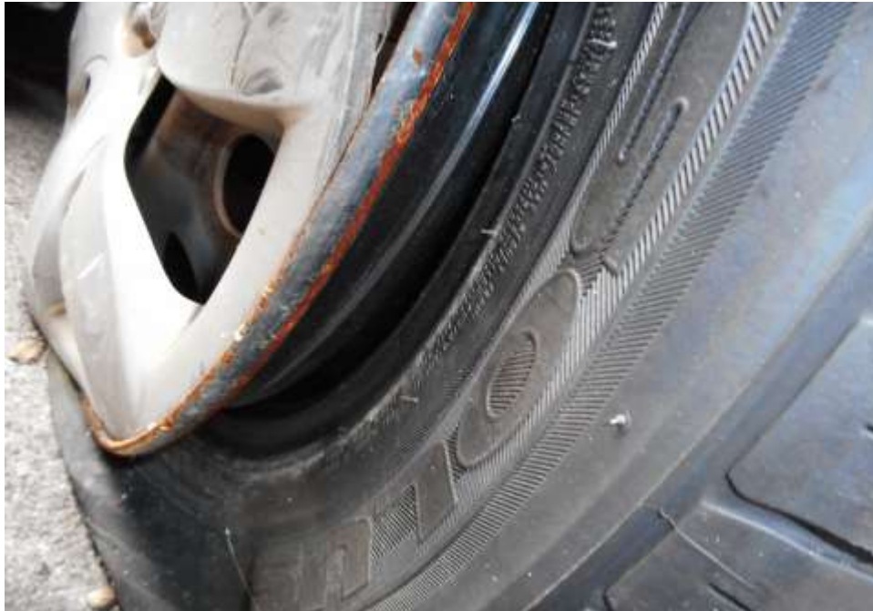
Photo 14 shows the condition of the front right wheel rim of the Motor Car. The tyre was observed to be sustained damage, dislodged from the rim and deflated as a result of the accident.
