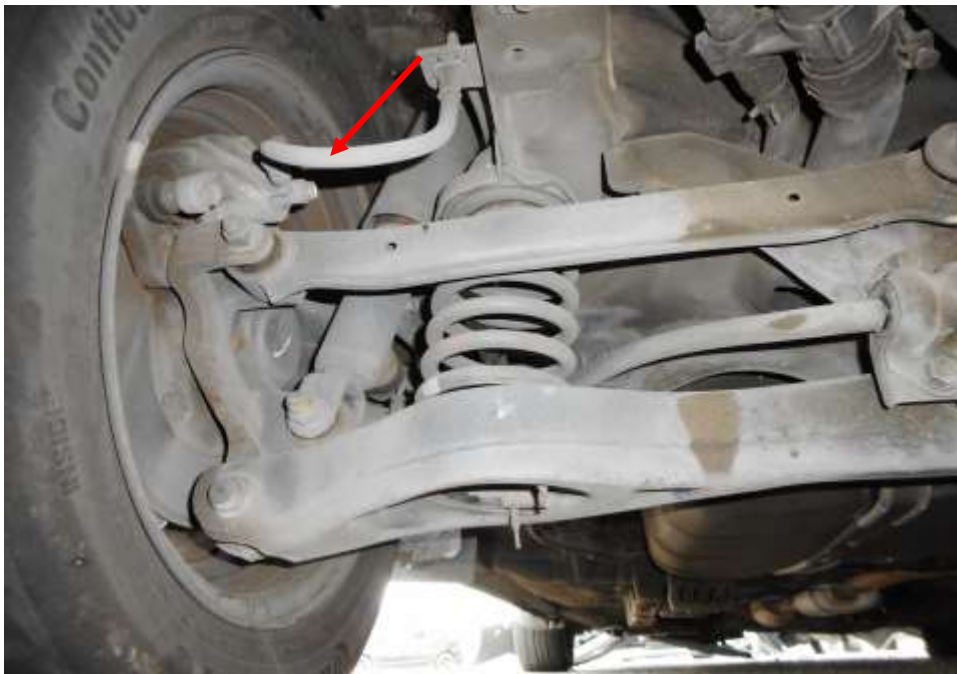
Photo 24 shows the various undercarriage components at the rear left wheel of the Motor Car, in particular the brake hose (arrowed). I did not observe any leakage of brake fluid at the 4 wheels of the Motor Car. My visual inspection of the various mechanical components of the Motor Car's braking system revealed all to be intact and without visible damage.
