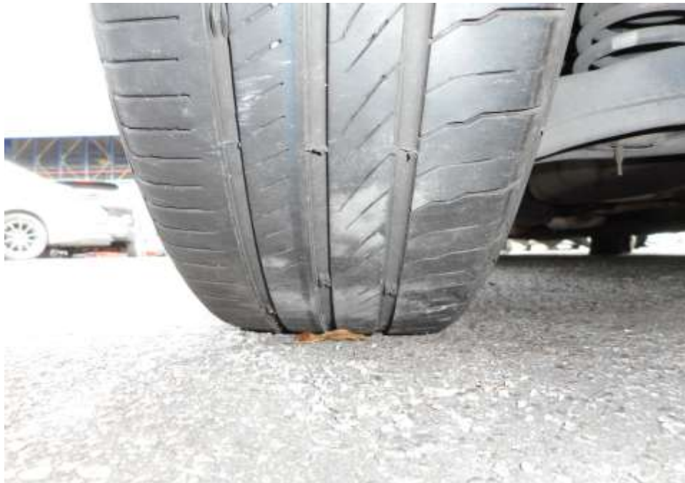
Photo 16 shows the condition of the rear left tyre of the Motor Car, which was observed to be in serviceable condition with remaining tread depth of approximately 4.5mm. There was no tear, cut or burst mark(s) on the outer and the inner sidewalls as well as across the tread of this tyre.
