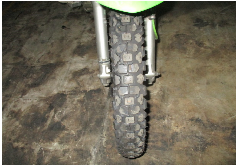
Photo 10 shows the front tyre of the Motorcycle at the time of our inspection. The front tyre was observed to be in serviceable condition with remaining tread depth of approximately 5mm. The pattern of the tread was also clearly visible. There was no tear, burst mark(s) and/or punctured hole(s) on the sidewalls as well as across the tread of the front tyre.
