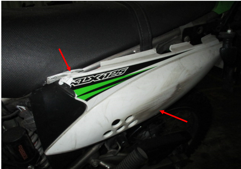
Photo 7 shows a closer view of the left rear side cover (arrowed) which was amongst the body parts of the Motorcycle that had sustained damage as a result of the accident.
