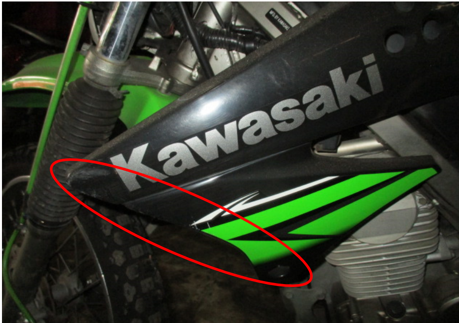
Photo 5 shows the left side cowling of the Motorcycle (circled) that had sustained damage as a result of the accident.
