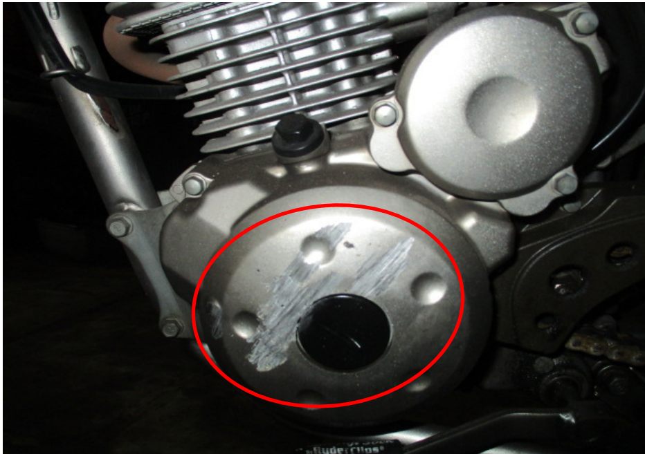
Photo 12 shows the left side of the engine of the Motorcycle at the time of our inspection. The various left engine components had sustained damage of grazing nature as a result of the accident (circled) however the engine components were still intact. There was also no fluid leak and/or fluid stain found around the left engine area of the Motorcycle.
