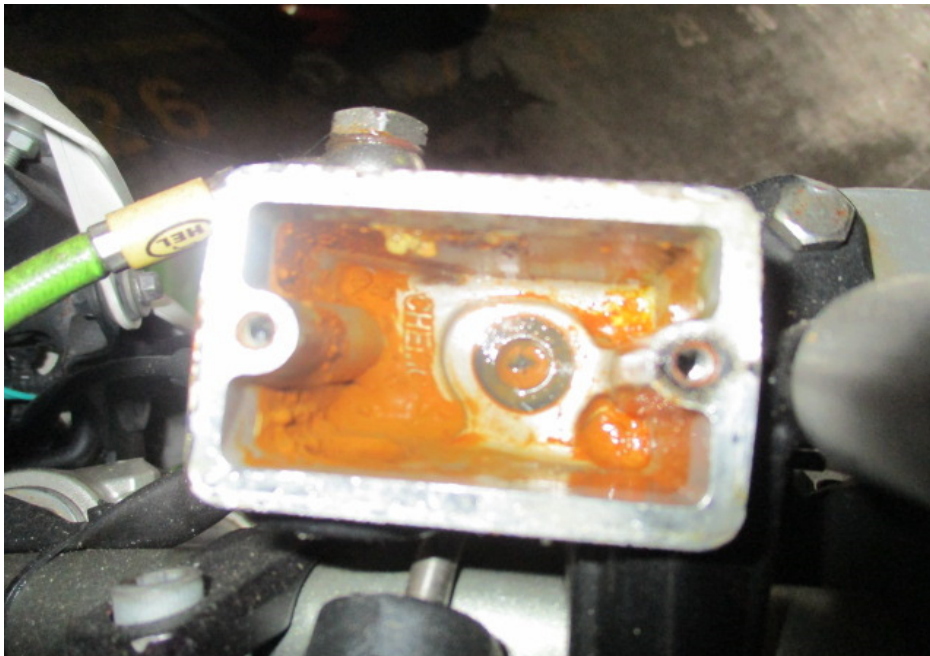
Photo 22 shows the brake fluid reservoir for the front brake of the Motorcycle. The brake fluid was observed to be of insufficient level for operational purposes, which is most likely due to the leakage from the brake fluid reservoir. The brake fluid reservoir was also observed to be corroded.
