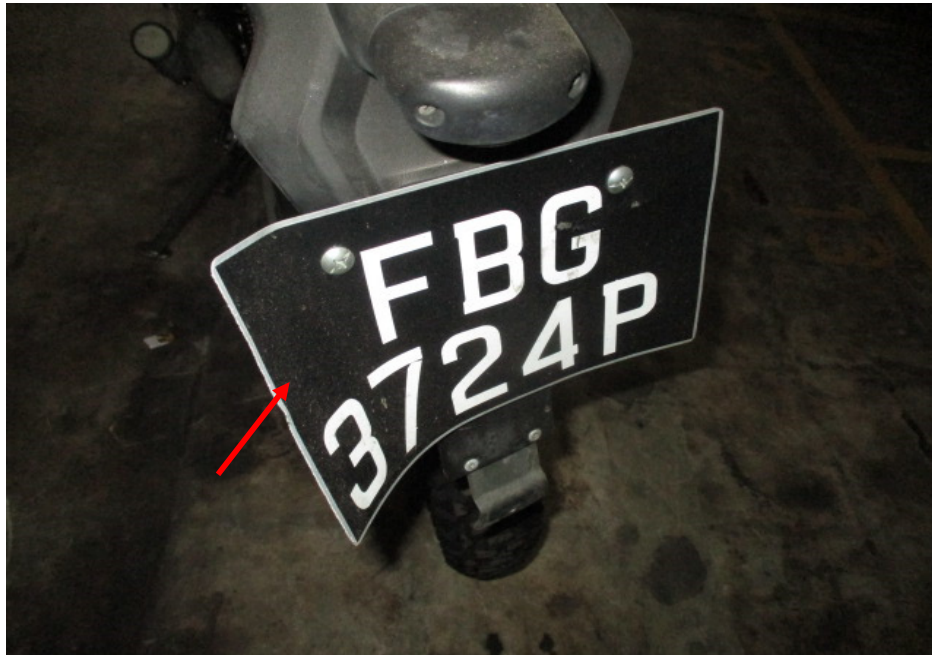
Photo 9 shows a closer view of the rear number plate (arrowed) which was amongst the body parts of the Motorcycle that had sustained damage as a result of the accident.
