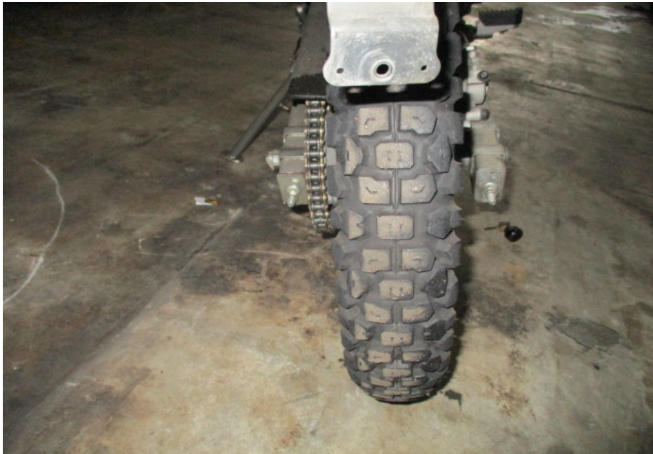
Photo 11 shows the condition of the Motorcycle's rear tyre. The rear tyre was observed to be in serviceable condition with remaining tread depth of approximately 8mm. The tyre was also observed to be sufficiently inflated for vehicular operation. We did not observe any tear, burst mark(s) and/or punctured hole(s) on the sidewalls as well as across the tread of the rear tyre.
