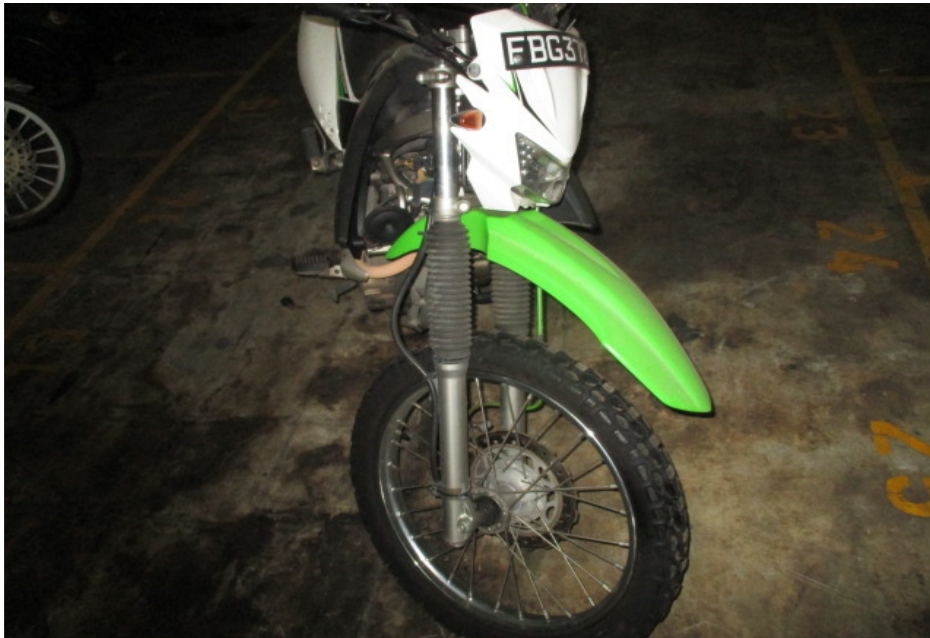
Photo 18 shows the front wheel of the Motorcycle turned towards its full left. Turning the Motorcycle's handle bar towards the left and right did not produce any abnormal free play and/or resistance. This would indicate that the steering system of the Motorcycle was in serviceable condition at the time of our inspection.
