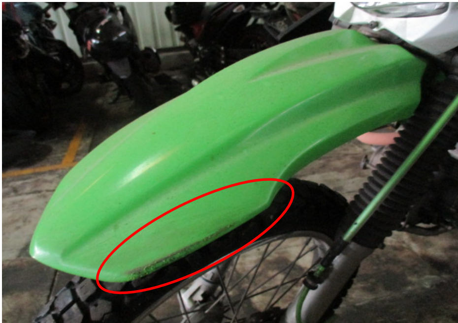
Photo 3 shows a closer view of the front mudguard (circled) which was amongst the body parts at the front body of the Motorcycle that had sustained damage as a result of the accident.
