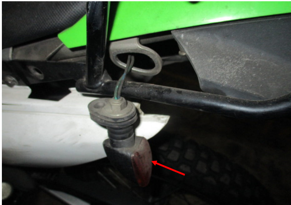
Photo 8 shows the left rear signal lamp (arrowed) which were amongst the body parts of the Motorcycle that had sustained damage as a result of the accident.
