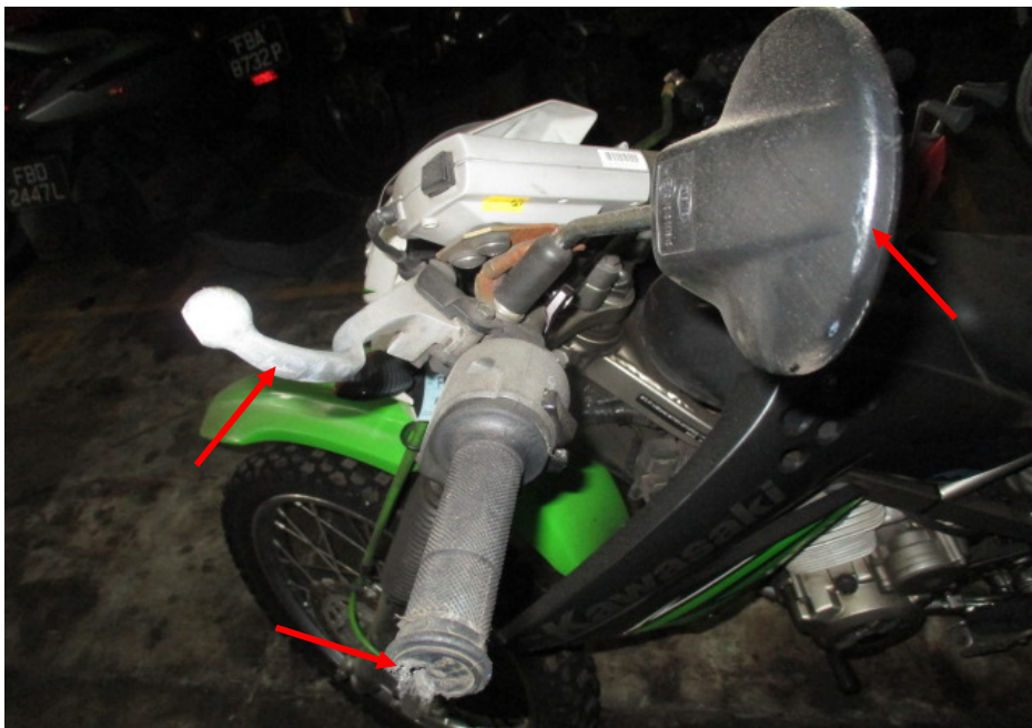
Photo 4 shows a closer view of the clutch lever, left side mirror and left handlebar end (arrowed) which were amongst the body parts of the Motorcycle that had sustained damage as a result of the accident.
