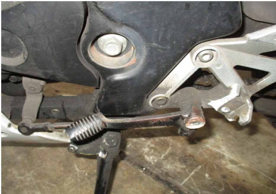
Photo 7 shows a closer view of the gear shift rod, gear shift pedal, left front footrest and left front footrest bracket, which were amongst the body parts of the Motorcycle that had sustained damage as a result of the accident.
