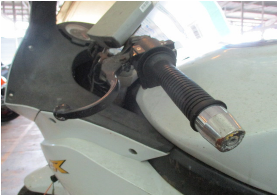
Photo 6 shows a closer view of the clutch lever, left handlebar grip and left handlebar end which were amongst the body parts of the Motorcycle that had sustained damage as a result of the accident.
