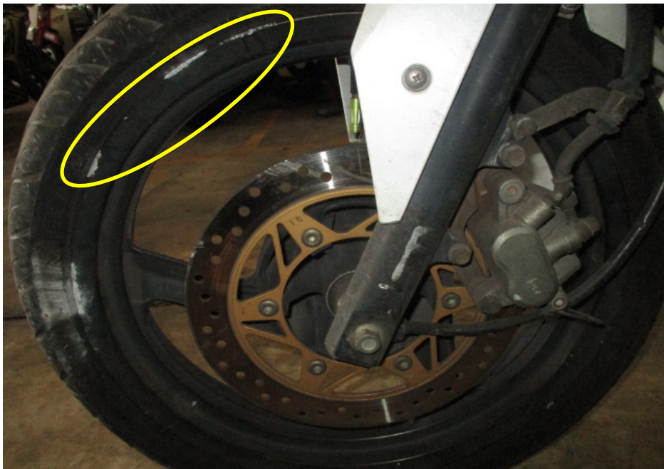
Photo 9 shows the front wheel rim and front tyre of the Motorcycle at the time of our inspection. The front tyre was observed to be in serviceable condition with remaining tread depth of approximately 3mm. The tyre was also observed to be sufficiently inflated for vehicular operation. Some relatively minor marks of grazing nature were observed on the edges of the front wheel rim (circled), at the left side of the Motorcycle.
