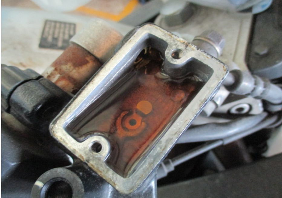
Photo 19 shows the brake fluid reservoir for the front brake of the Motorcycle. The brake fluid was observed to be of sufficient level and without contamination for operational purposes.
