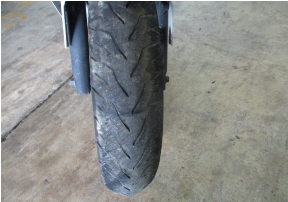
Photo 10 shows the front tyre of the Motorcycle at the time of our inspection. The front tyre was observed to be in serviceable condition. The pattern of the tread was also clearly visible. There was no tear, burst mark(s) and/or punctured hole(s) on the sidewalls as well as across the tread of the front tyre.
