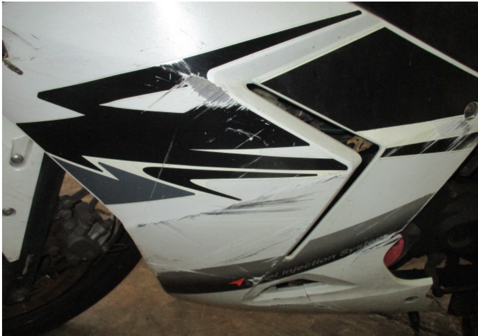
Photo 5 shows a closer view of the left side cowling of the Motorcycle that had sustained damage as a result of the accident.
