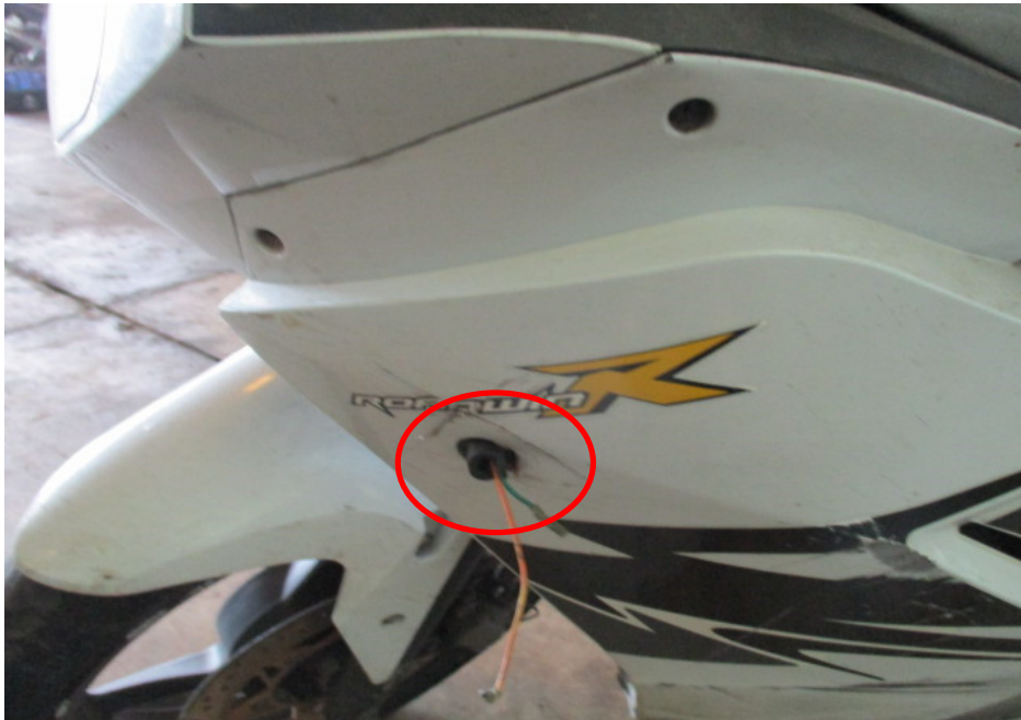
Photo 4 shows a close up view of the left front signal lamp (circled) which was amongst the body parts of the Motorcycle that had sustained damage as a result of the accident.
