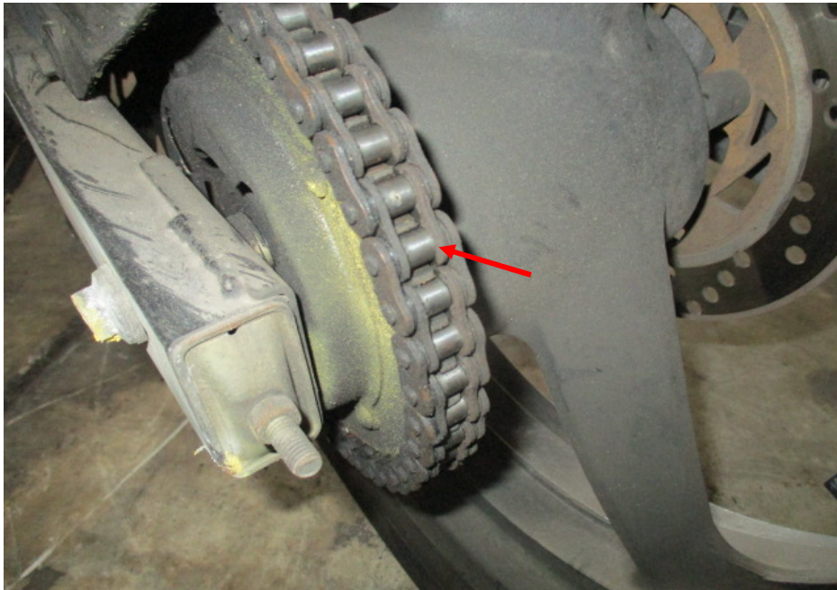
Photo 15 shows a closer view of the gear train (arrowed) of the Motorcycle, which was observed to be intact with no misalignment. It was also adequately lubricated for operating purposes.
