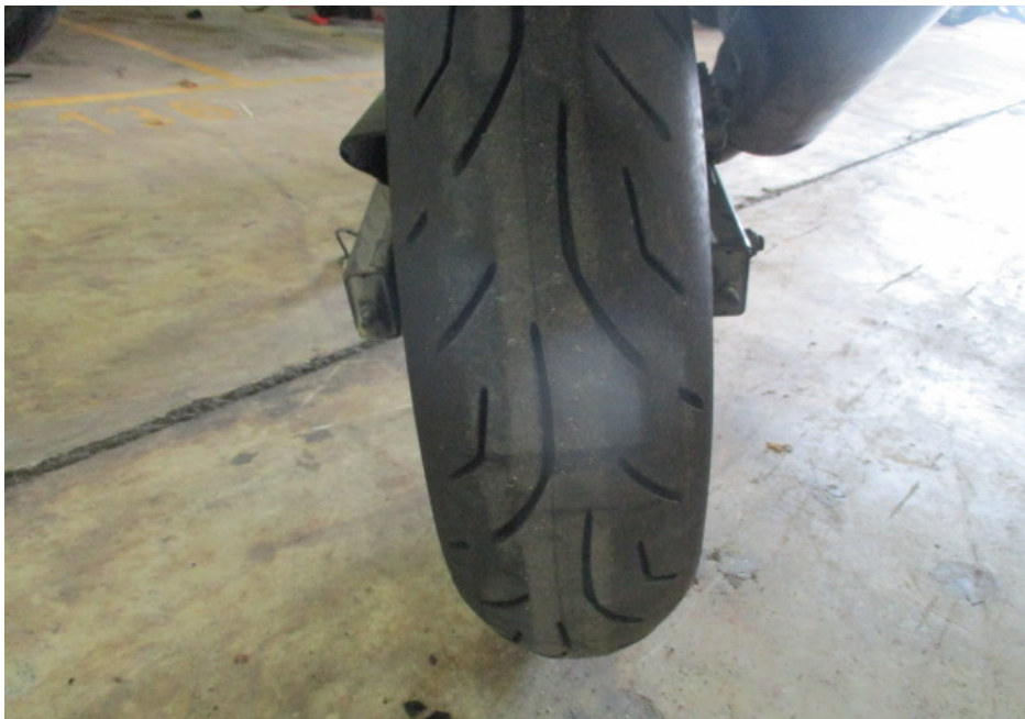
Photo 11 shows the condition of the Motorcycle's rear tyre. The rear tyre was observed to be in serviceable condition with remaining tread depth of approximately 4mm. The tyre was also observed to be sufficiently inflated for vehicular operation. We did not observe any tear, burst mark(s) and/or punctured hole(s) on the sidewalls as well as across the tread of the rear tyre.
