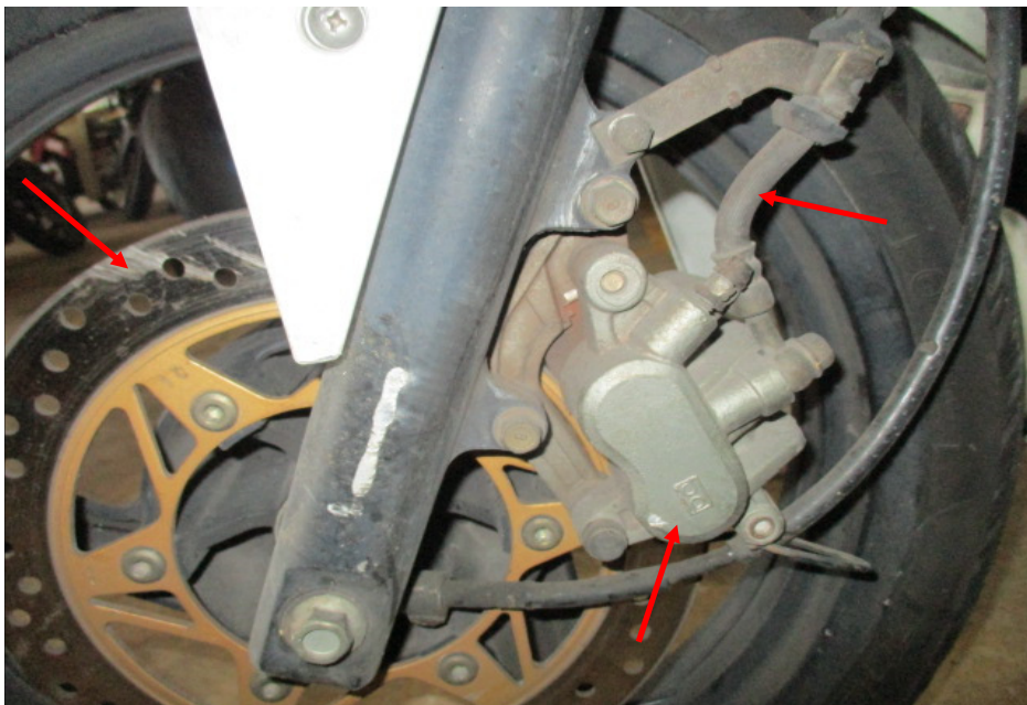
Photo 18 shows a close up view of the front brake caliper, front brake disc and front brake hose (arrowed) of the Motorcycle, which are all part of the components in the hydraulic front brake system of the Motorcycle. Our visual checks of these various components had revealed all to be intact with no visible damage. No leakage of brake fluid was also observed.
