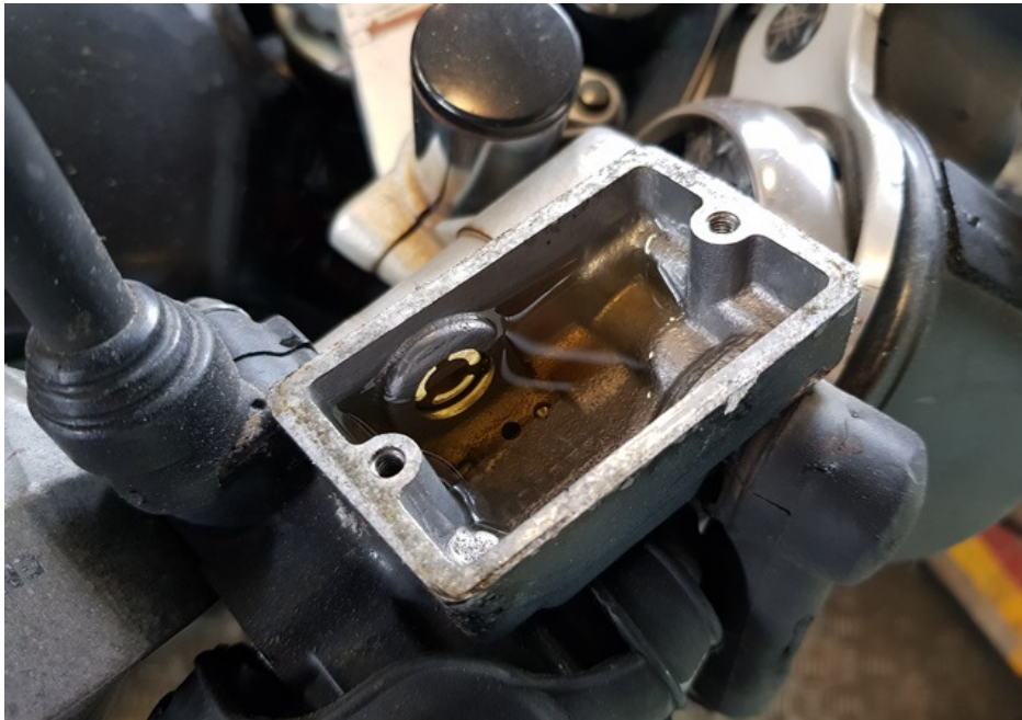
Photo 20 shows the brake fluid reservoir for the front brake of the Motorcycle. The brake fluid was observed to be at an insufficient level for operating purposes due to the brake fluid leak caused by the cut front brake hose as a result of the accident.
