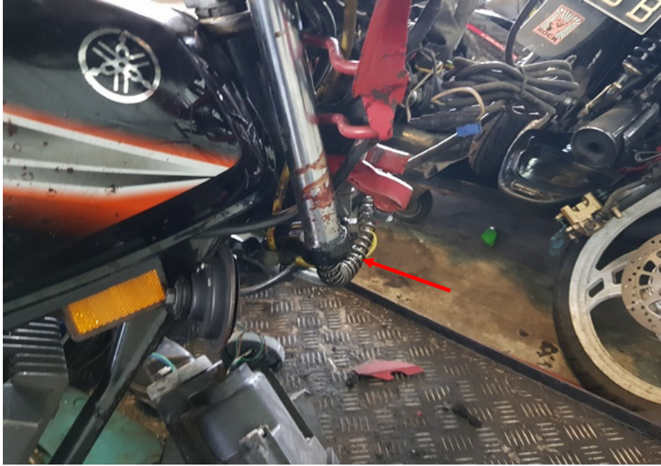
Photo 17 shows the front right fork of the Motorcycle. The front right fork (arrowed) was observed to be dislodged as a result of the accident. We were hence not able to conduct any tests on the steering system of the Motorcycle.
