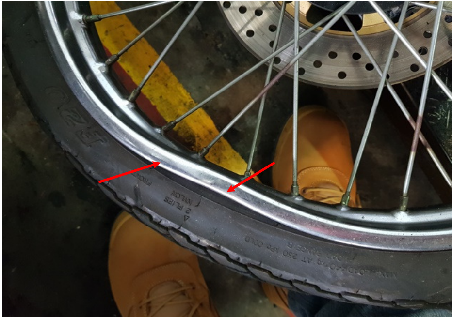
Photo 11 shows the bent front wheel rim of the Motorcycle at the time of our inspection (arrowed).
