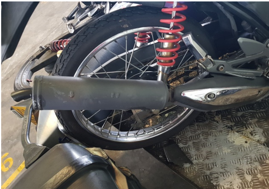
Photo 8 shows a closer view of the exhaust muffler, which was amongst the body parts of the Motorcycle that had sustained damage as a result of the accident.
