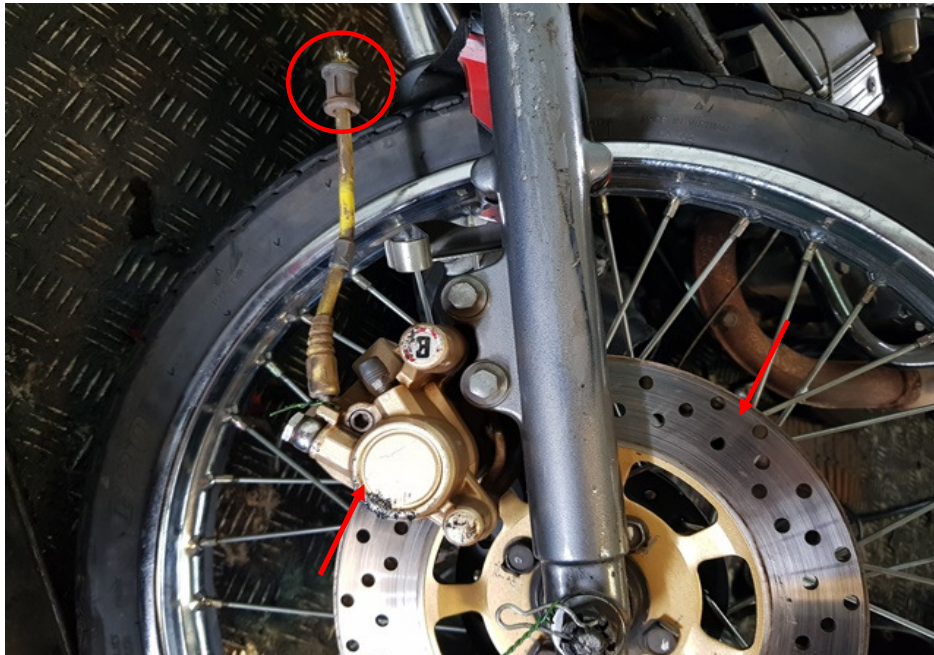
Photo 18 shows a close up view of the front brake caliper, front brake disc (arrowed) and front brake hose of the Motorcycle, which are all part of the components in the hydraulic front brake system of the Motorcycle. Our visual checks of the front brake caliper and front brake disc had revealed all to be intact with no visible damage. However we did observe that the front brake hose had been cut as a result of the accident (circled).
