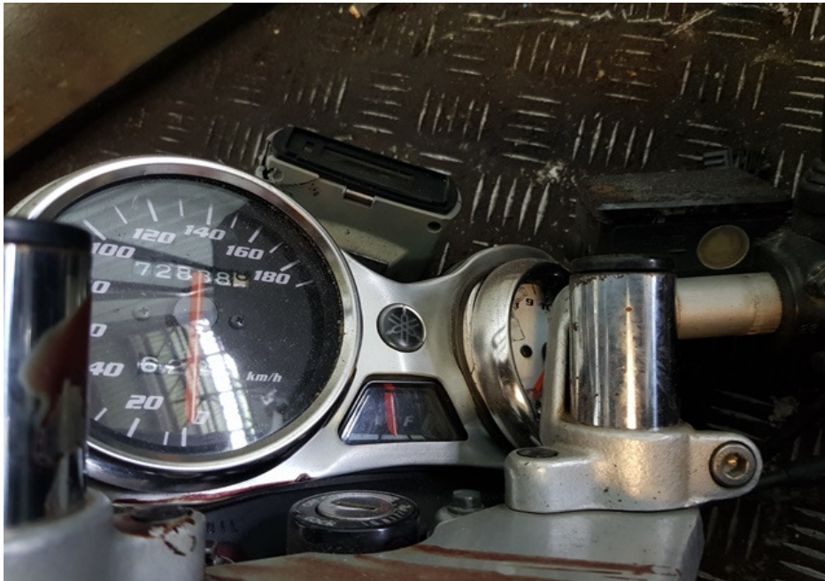
Photo 5 shows a closer view of the speedometer gauge which was amongst the body parts at the front body of the Motorcycle that had sustained damage as a result of the accident.
