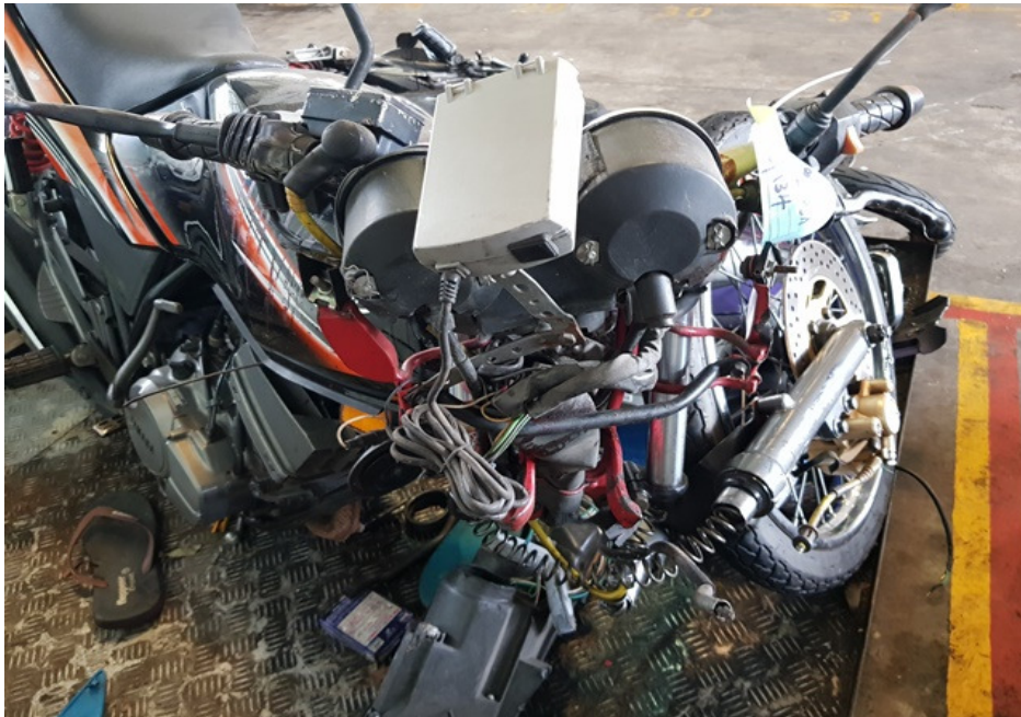
Photo 3 shows a general view of the front body of the Motorcycle at the time of our inspection. Body parts that were found to have been damaged include its headlamp assembly, fork assembly, speedometer gauge, side mirrors, clutch lever, front brake lever and petrol tank amongst others.
