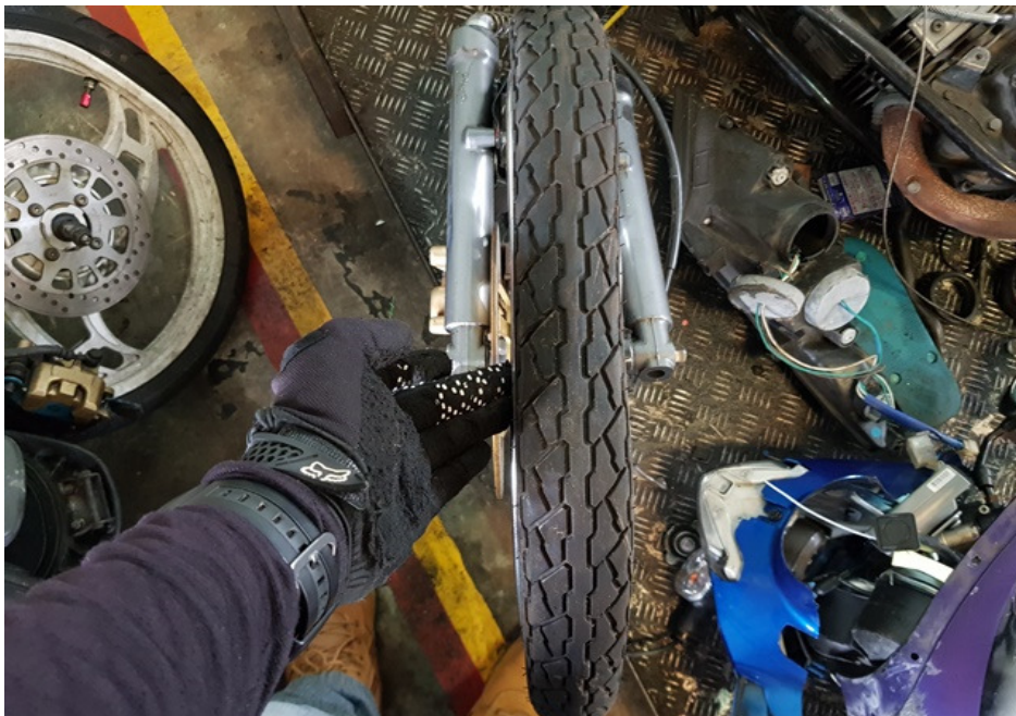
Photo 10 shows the condition of the Motorcycle's front tyre. The front tyre was observed to be in serviceable condition with remaining tread depth of approximately 3mm. The tyre was also observed to be sufficiently inflated for vehicular operation. We did not observe any tear, burst mark(s) and/or punctured hole(s) on the sidewalls as well as across the tread of the front tyre.
