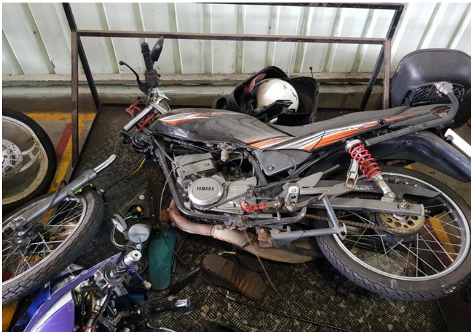
Photo 2 shows a general view of the left body of the Motorcycle at the time of our inspection. Body parts that were found to have been damaged include its headlamp assembly, front fork assembly, front wheel rim, side mirrors, clutch lever, front brake lever, fuel tank, exhaust muffler and rear side covers amongst others.
