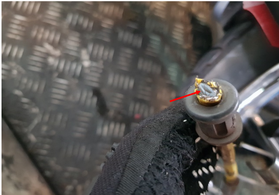
Photo 19 shows a close up view of the front brake hose which was observed to be cut as a result of the accident (arrowed).
