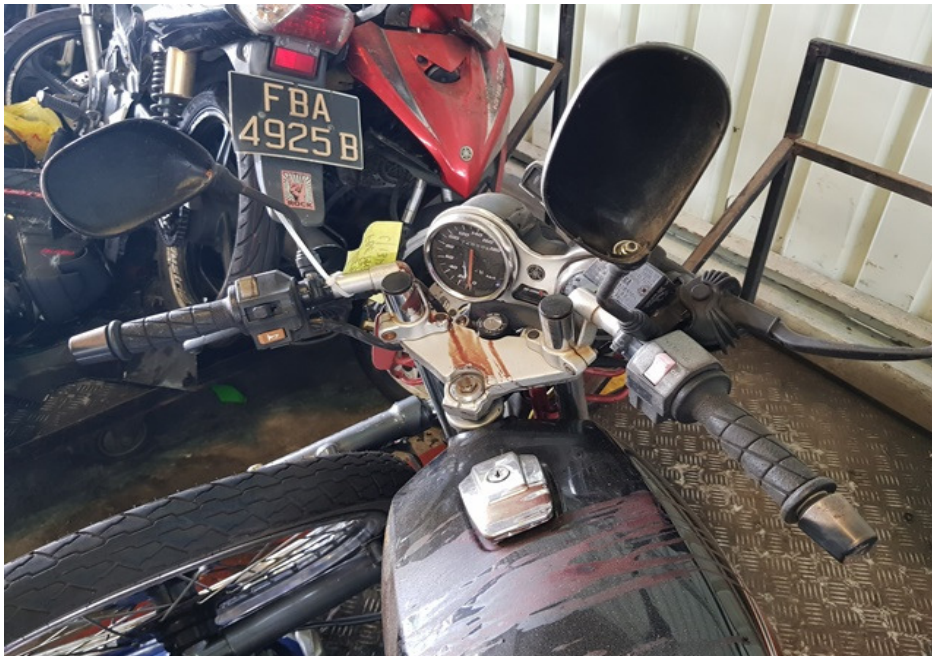
Photo 6 shows a closer view of the side mirrors, clutch lever, front brake lever, handlebars, handlebar grips and handlebar ends of the Motorcycle. These parts were amongst the body parts of the Motorcycle which were damaged as a result of the accident.
