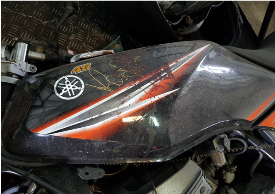
Photo 7 shows a closer view of the petrol tank, which was amongst the body parts of the Motorcycle that had sustained damage as a result of the accident.
