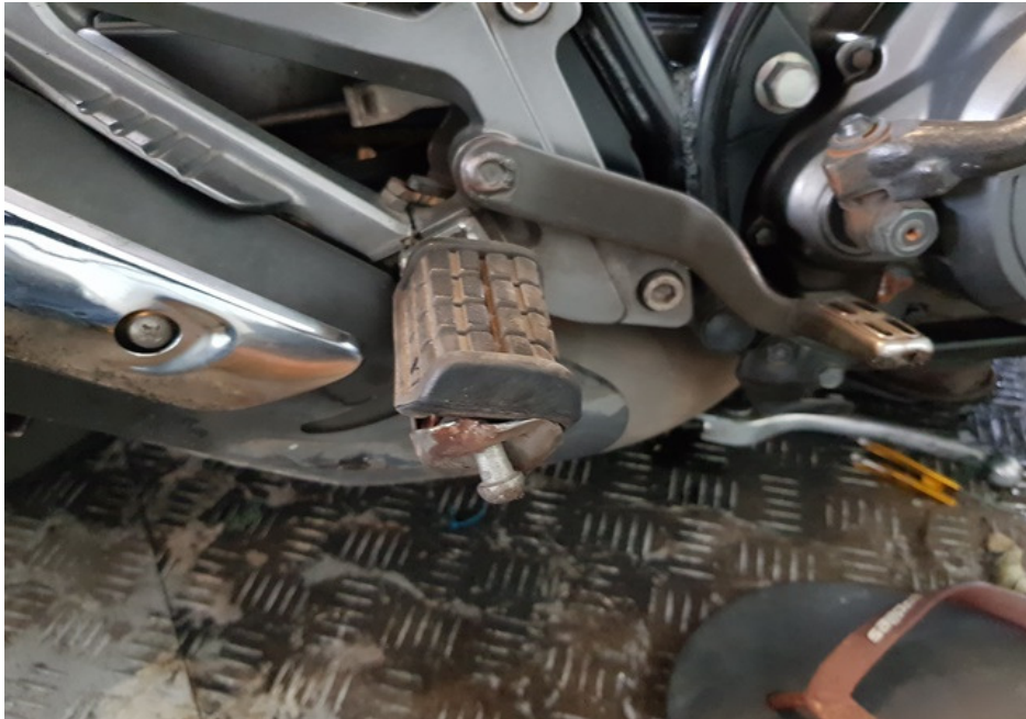
Photo 9 shows a closer view of the rear brake pedal, right front footrest and right front footrest bracket, which were amongst the body parts of the Motorcycle that had sustained damage as a result of the accident.
