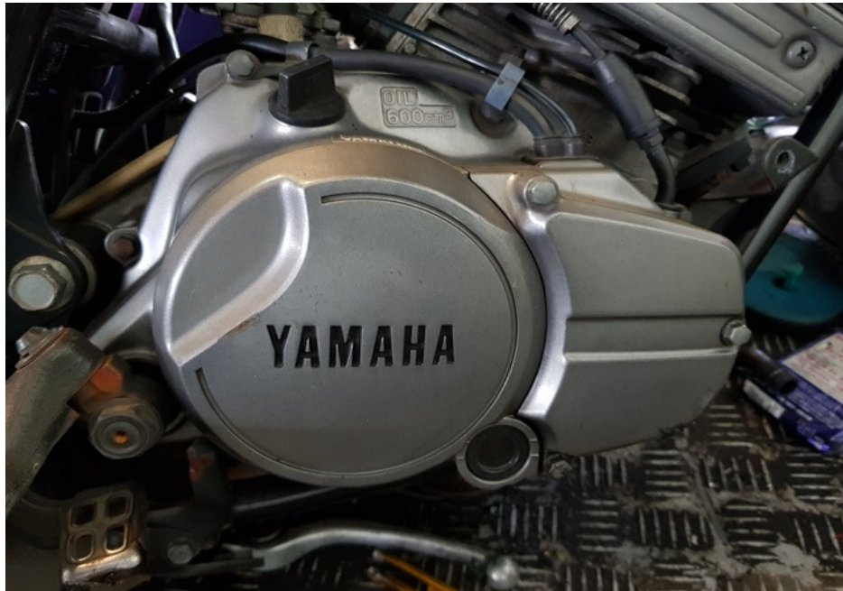
Photo 14 shows the right side of the engine of the Motorcycle at the time of our inspection. The various engine related parts and components were found to be intact with no visible damage. There was also no sign(s) or indication(s) of fluid leak observed around the right engine area of the Motorcycle.
