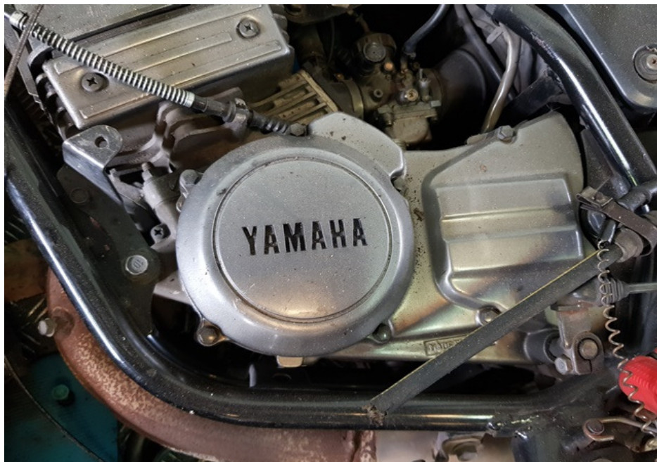
Photo 13 shows the left side of the engine of the Motorcycle at the time of our inspection. The various engine related parts and components were found to be intact with no visible damage. There was also no sign(s) or indication(s) of fluid leak observed around the left engine area of the Motorcycle.
