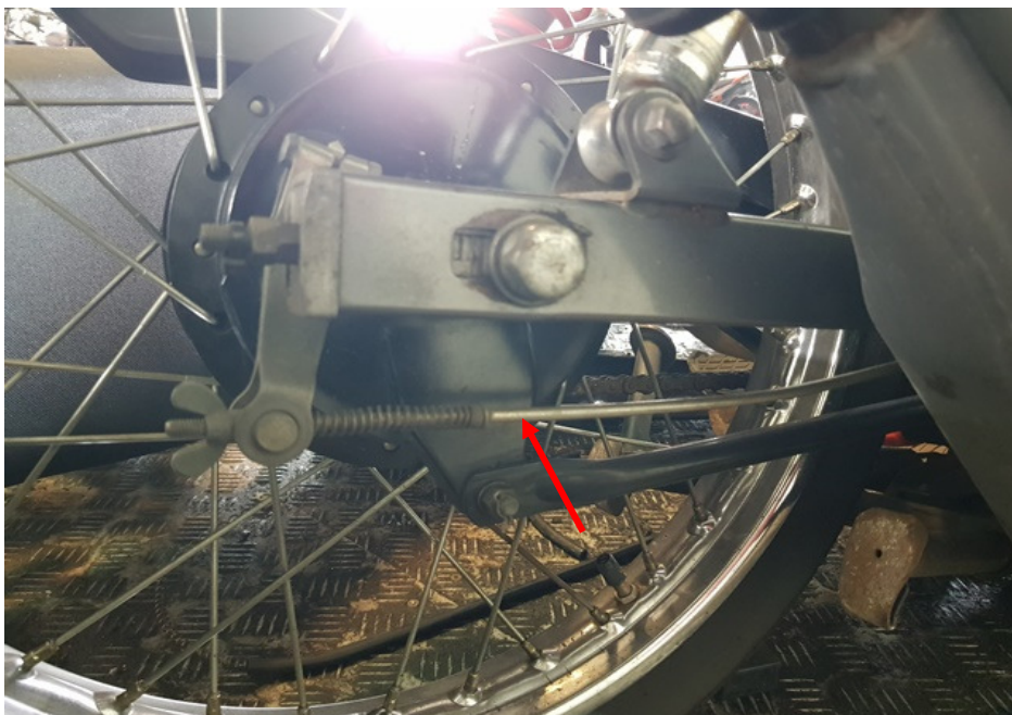
Photo 21 shows the rear wheel of the Motorcycle. The type of brake system for the rear wheel was of a mechanical type, controlled by the brake foot pedal of the Motorcycle. Our checks of the cable (arrowed), spring and drum which are all part of the components in the rear brake system of the Motorcycle reveal all to be intact and without damage.
