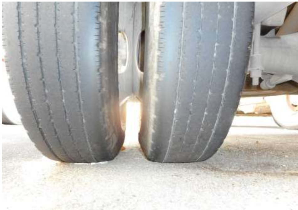
Photo 7 shows the condition of the rear right tyre of the Motor Lorry, which was observed to be in serviceable condition with remaining tread depth of approximately 3mm. The tyre, which was wrapped around standard steel wheel rim, was also observed to be sufficiently inflated for vehicular operation.
