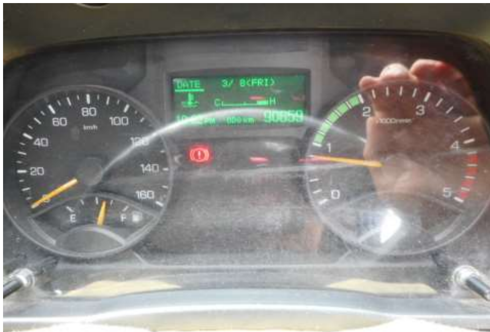
Photo 24 shows no warning lights illuminated on the instrument panel of the Motor Lorry after the engine was cranked. This would suggest that there was no abnormality to the electronic operating system of the Motor Lorry, like the ABS.
