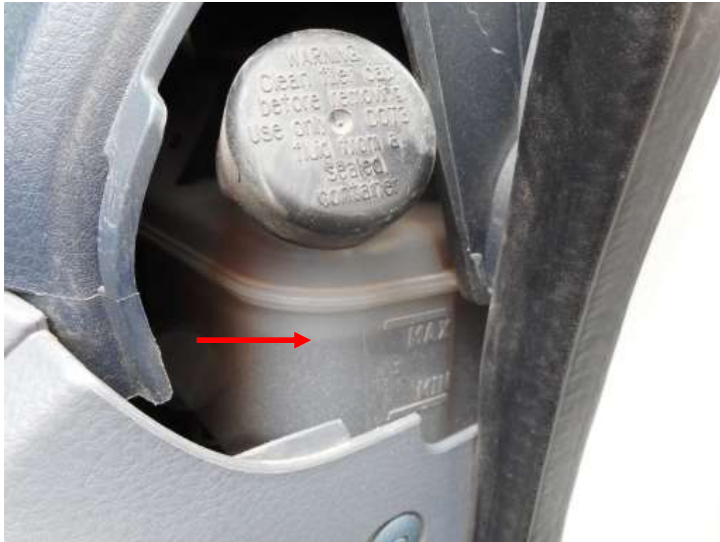
Photo 11 shows the brake fluid reservoir of the Motor Lorry at the time of my inspection. The brake fluid was observed to be of sufficient level (arrowed) and without any visible contamination.
