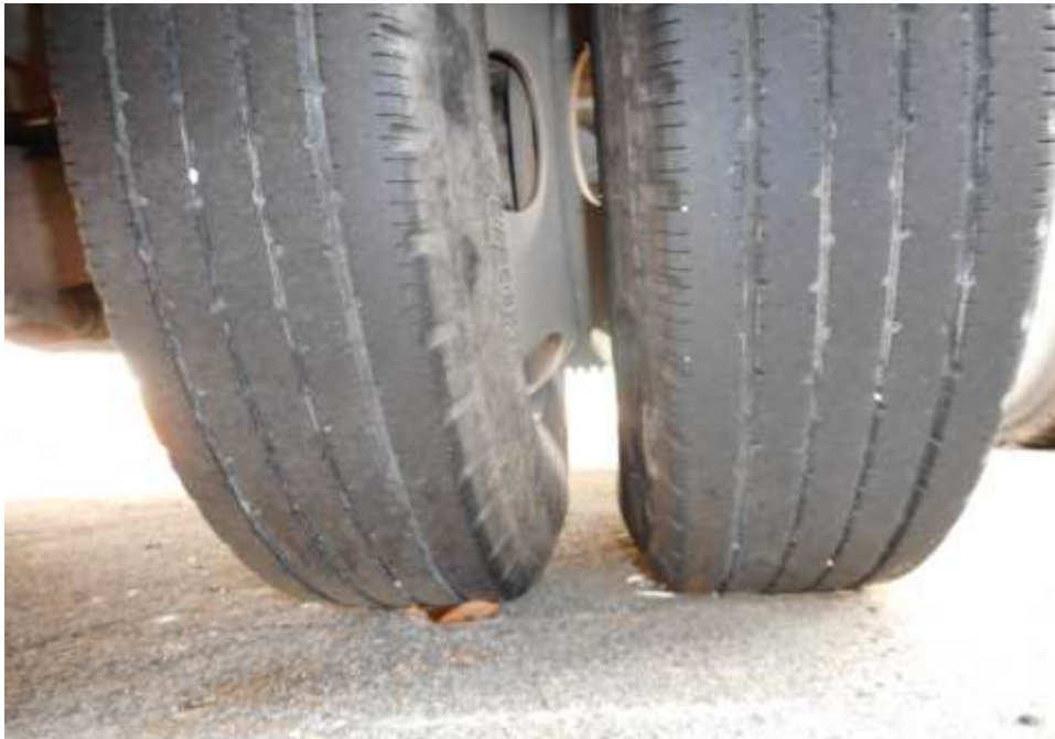
Photo 8 shows the condition of the rear left tyres of the Motor Lorry, which was observed to be in serviceable condition with remaining tread depth of approximately 3.5mm. The tyres, which were wrapped around standard steel wheel rim, were also observed to be sufficiently inflated for vehicular operation. There was also no damage found on all 6 steel wheel rims of the Motor Lorry.
