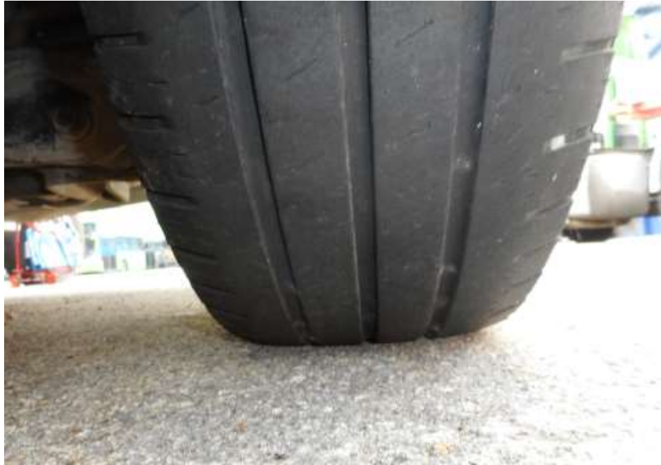
Photo 6 shows the condition of the front right tyre of the Motor Lorry, which was observed to be in serviceable condition with remaining tread depth of approximately 4mm. The tyre, which was wrapped around standard steel wheel rim, was also observed to be sufficiently inflated for vehicular operation. There was no tear, cut or burst mark(s) on the outer and the inner sidewalls as well as across the tread of the 6 tyres that were fitted on the Motor Lorry.
