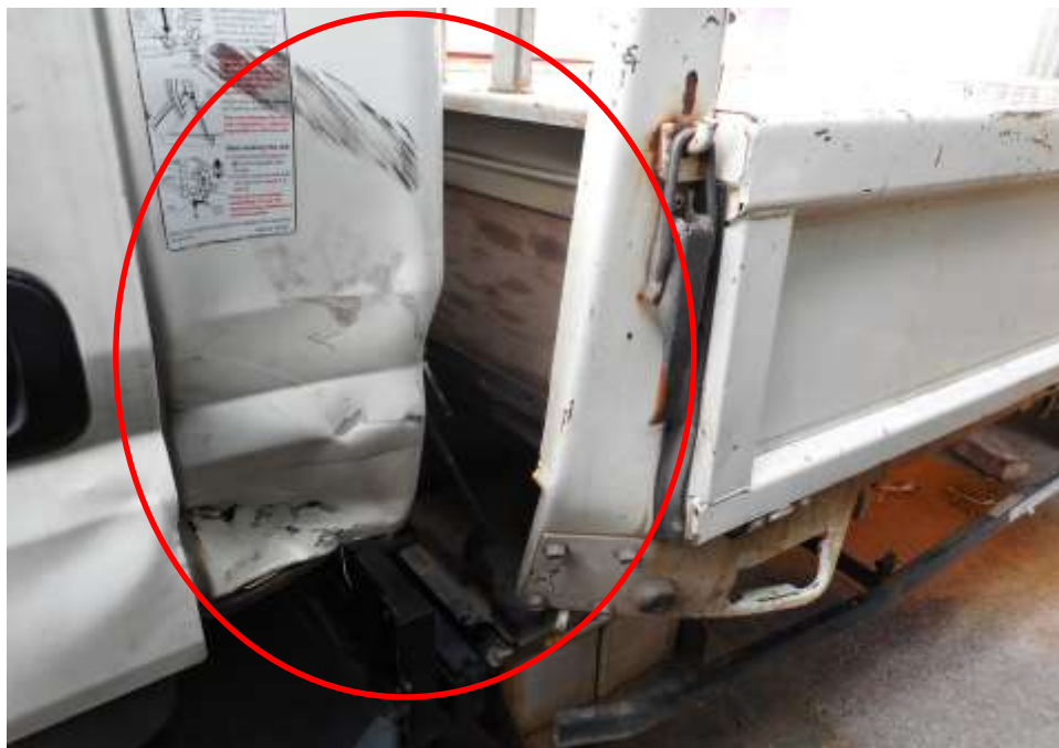
Photo 3 shows a close up view of the Motor Lorry's frontal portion at the time of my inspection. There was minor damage found to the front body panel of the Motor Lorry. Its left cabin panel (circled) were damage as a result of the accident.
