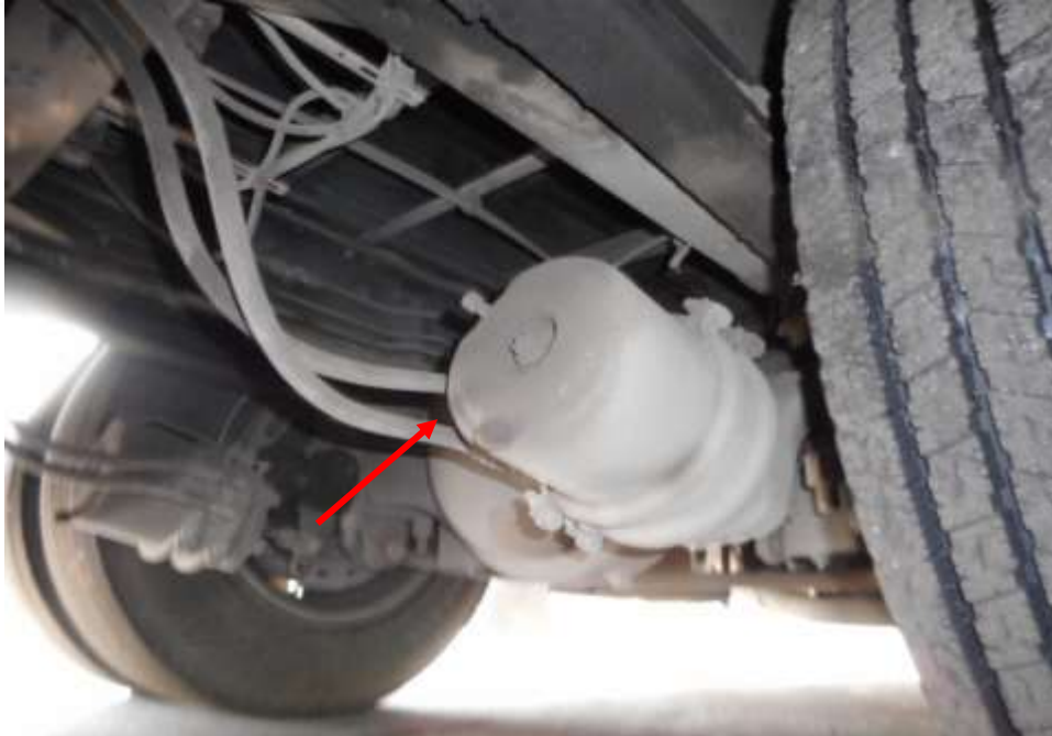
Photo 18 shows the brake pipe (arrowed) at the rear left wheel of the Motor Bus. I did not observe any leakage of brake fluid at the time of my inspection of the Motor Bus. My static tests of the Motor Bus's braking system, along with my visual examination of the various mechanical components in the braking system, had indicated that there was no internal leakage of pressure/vacuum. Hence the braking system of the Motor Bus was likely to be in serviceable condition at the material time of accident.
