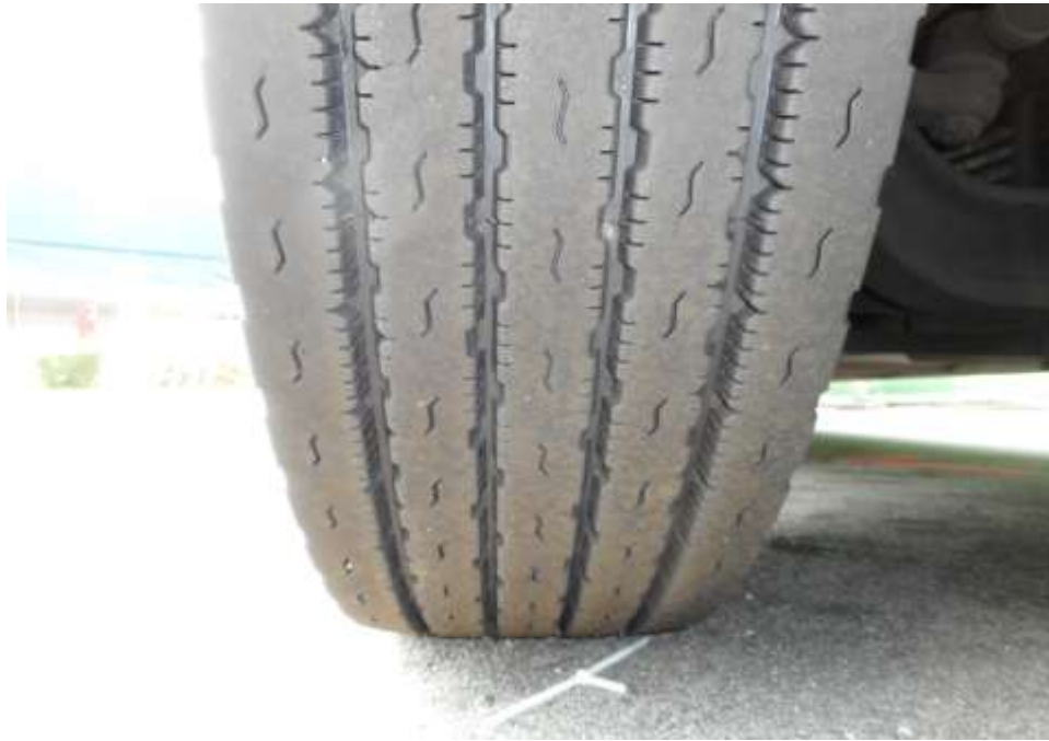
Photo 8 shows the condition of the front right tyre of the Motor Bus, which was observed to be in serviceable condition with remaining tread depth of approximately 8.9mm. The tyre, which was wrapped around standard steel wheel rim, was also observed to be sufficiently inflated for vehicular operation. There was no tear, cut or burst mark(s) on the outer and the inner sidewalls as well as across the tread of the 6 tyres that were fitted on the Motor Bus.
