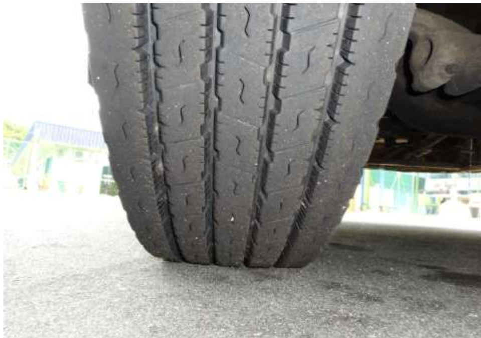
Photo 11 shows the condition of the front left tyres of the Motor Bus, which were observed to be in serviceable condition with remaining tread depth of approximately 8.7mm. There was also no tear, cut or burst mark(s) on the outer and the inner sidewalls as well as across the tread of the 6 tyres that were fitted on the Motor Bus.
