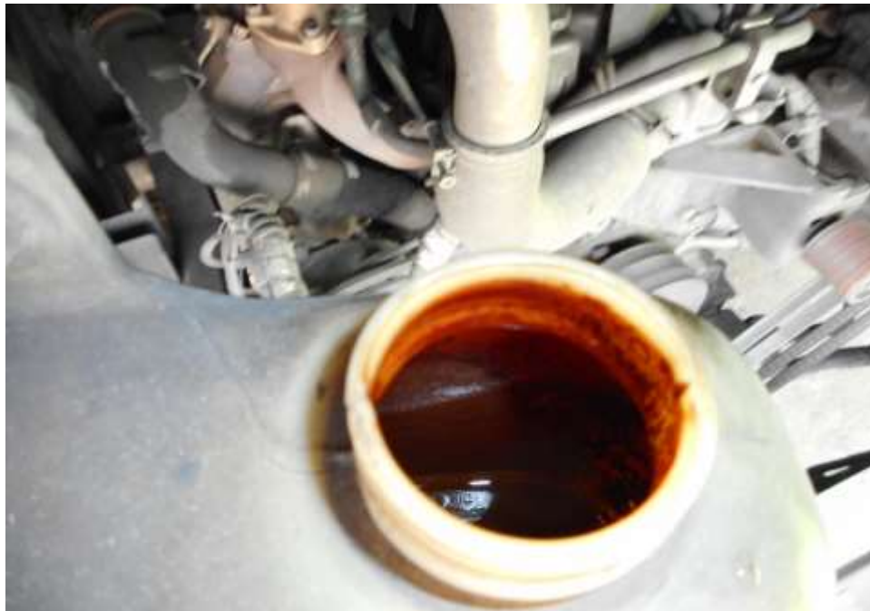
Photo 14 shows the engine coolant reservoir of the Motor Bus at the time of my inspection. The engine coolant was observed to be of sufficient level and without any visible contamination.
