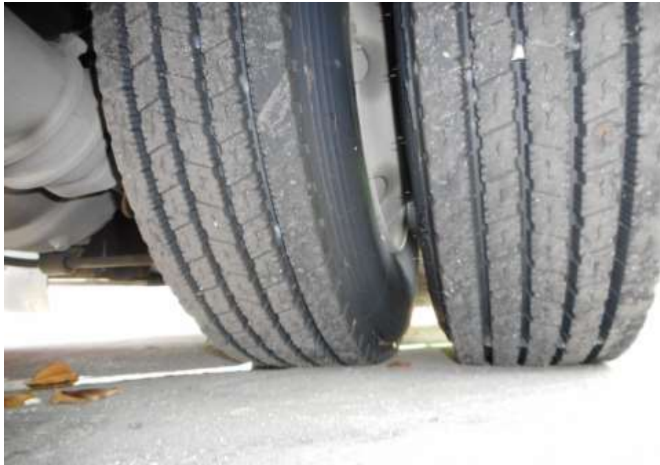
Photo 10 shows the condition of the rear left tyres of the Motor Bus, which was observed to be in serviceable condition with remaining tread depth of approximately 11.5mm. The tyres, which were wrapped around standard steel wheel rim, were also observed to be sufficiently inflated for vehicular operation. There was also no damage found on all 6 steel wheel rims of the Motor Bus.
