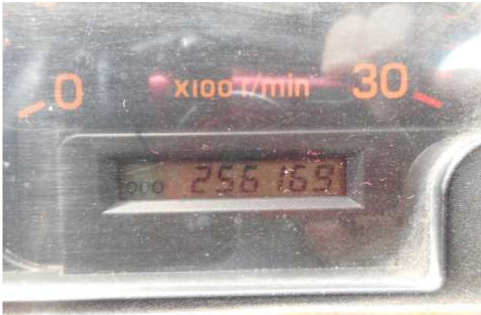
Photo 1 shows a general view of the instrument cluster of the Motor Bus at the time of my inspection. The mileage of the Motor Bus was 256,169km
