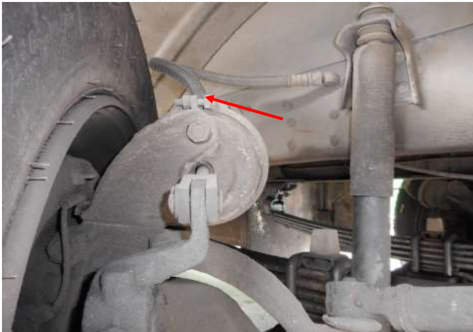
Photo 19 shows the brake pipe (arrowed) at the front right wheel of the Motor Bus. I did not observe any leakage of brake fluid at the time of my inspection of the Motor Bus. My static tests of the Motor Bus's braking system, along with my visual examination of the various mechanical components in the braking system, had indicated that there was no internal leakage of pressure/vacuum. Hence the braking system of the Motor Bus was likely to be in serviceable condition at the material time of accident.
