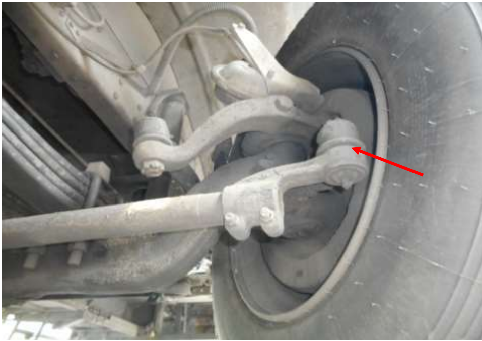
Photo 22 shows the various undercarriage components at the front right wheel of the Motor Bus, in particular the steering tie rod end (arrowed). The various steering components were all found to be intact, suggesting that the steering system of the Motor Bus was likely to be in serviceable condition at the material time of accident. There was also no sign of fluid stain(s) observed on the various undercarriage components.
