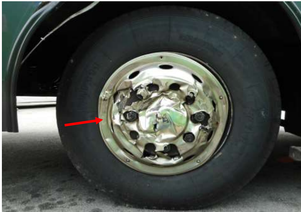
Photo 4 shows a close up view of the front left wheel of the Motor Bus at the time of my inspection. The Motor Bus was observed to have sustained minor damages at its front left wheel portion. Its front left wheel cover (arrowed) was damaged as a result of the accident at the time of my inspection.
