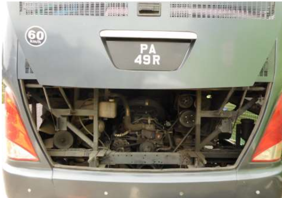
Photo 12 shows a general view of the Motor Bus's engine compartment, which was accessed by lifting the front cabin of the Motor Bus. The various parts and components inside the engine compartment were unaffected by the accident. There was also no sign(s) or indication(s) of fresh fluid leakage and/or fluid stain within the engine compartment
