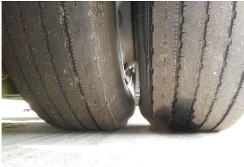
Photo 9 shows the condition of the rear right tyre of the Motor Bus, which was observed to be in serviceable condition with remaining tread depth of approximately 12mm. The tyre, which was wrapped around standard steel wheel rim, was also observed to be sufficiently inflated for vehicular operation.
