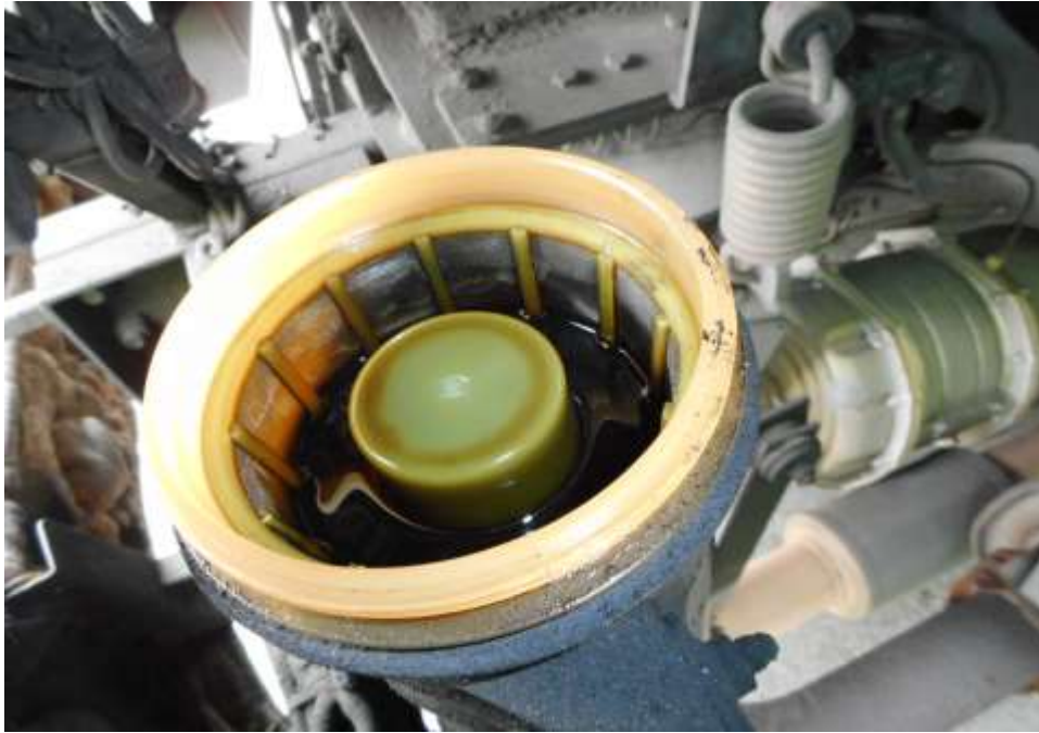
Photo 15 shows the power steering fluid reservoir of the Motor Bus at the time of my inspection. The power steering fluid was observed to be of sufficient level and without any visible contamination.
