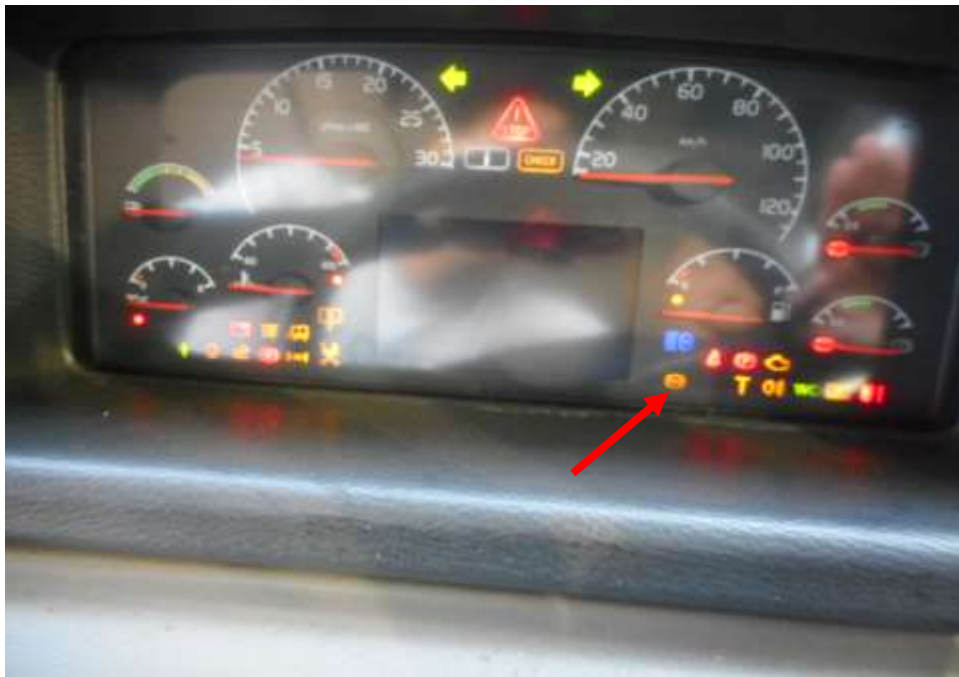
Photo 23 shows the warning light for Anti-Lock Brake System (ABS) appearing on the instrument panel of the Motor Bus during the self-test of its various electronic operating systems when its engine was cranked.
