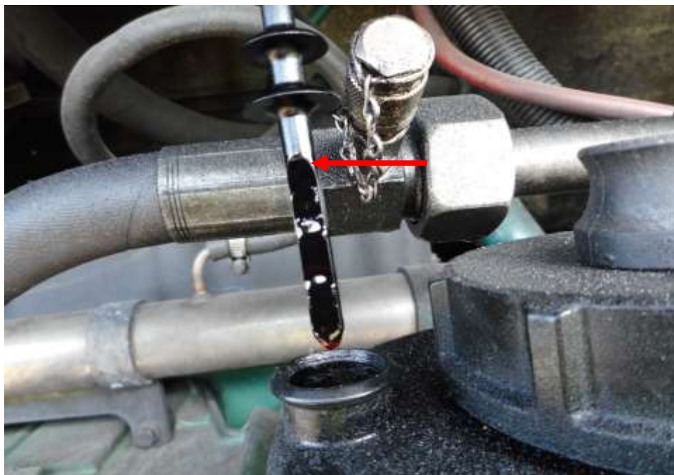
Photo 16 shows the power steering fluid reservoir of the Motor Bus at the time of my inspection. The power steering fluid was observed to be of sufficient level (arrowed) and without any visible contamination.
