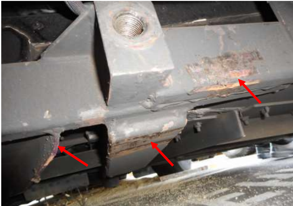
Photo 13 shows undercarriage of the Motor Bus at the time of my inspection. The undercarriage components of Motor Bus (arrowed) was observed to have received impact marks and damaged at the time of my inspection due to the towing process of the Motor Bus.
