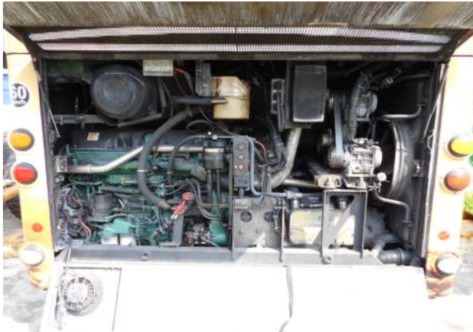
Photo 10 shows a general view of the Motor Bus's engine compartment, which was accessed by lifting the front cabin of the Motor Bus. The various parts and components inside the engine compartment were unaffected by the accident. There was also no sign(s) or indication(s) of fresh fluid leakage and/or fluid stain within the engine compartment.
