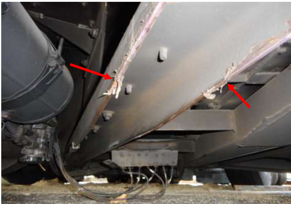
Photo 14 shows undercarriage of the Motor Bus at the time of my inspection. The undercarriage components of Motor Bus (arrowed) was observed to have received impact marks and damaged at the time of my inspection due to the towing process of the Motor Bus.
