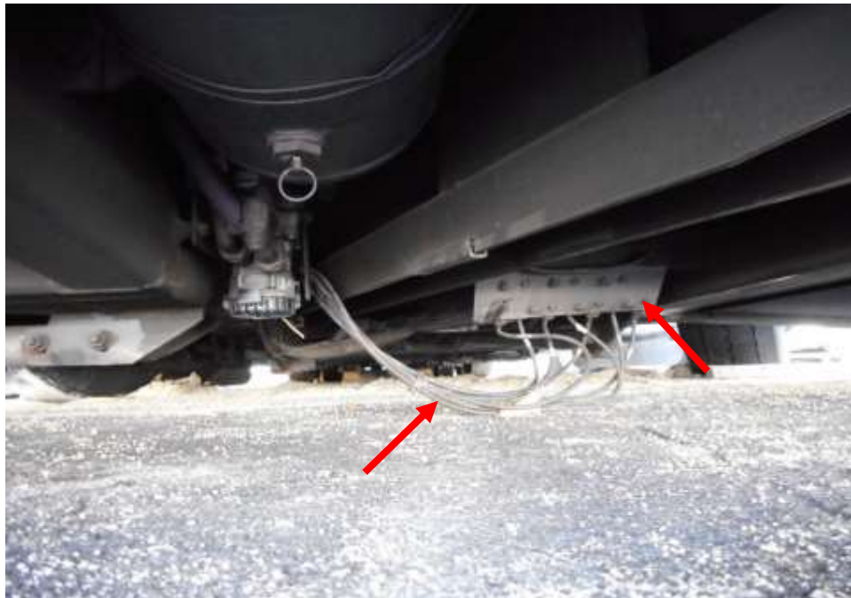
Photo 12 shows undercarriage of the Motor Bus at the time of my inspection. The hoses and the components of the air brakes (arrowed) were observed to be damaged and dislodged from the Motor Bus at the time of my inspection due to the towing process of the Motor Bus.
