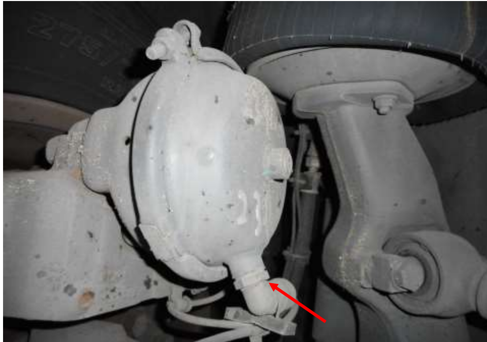
Photo 18 shows the brake pipe (arrowed) at the front right wheel of the Motor Bus was observed to be intact at the time of my inspection.
