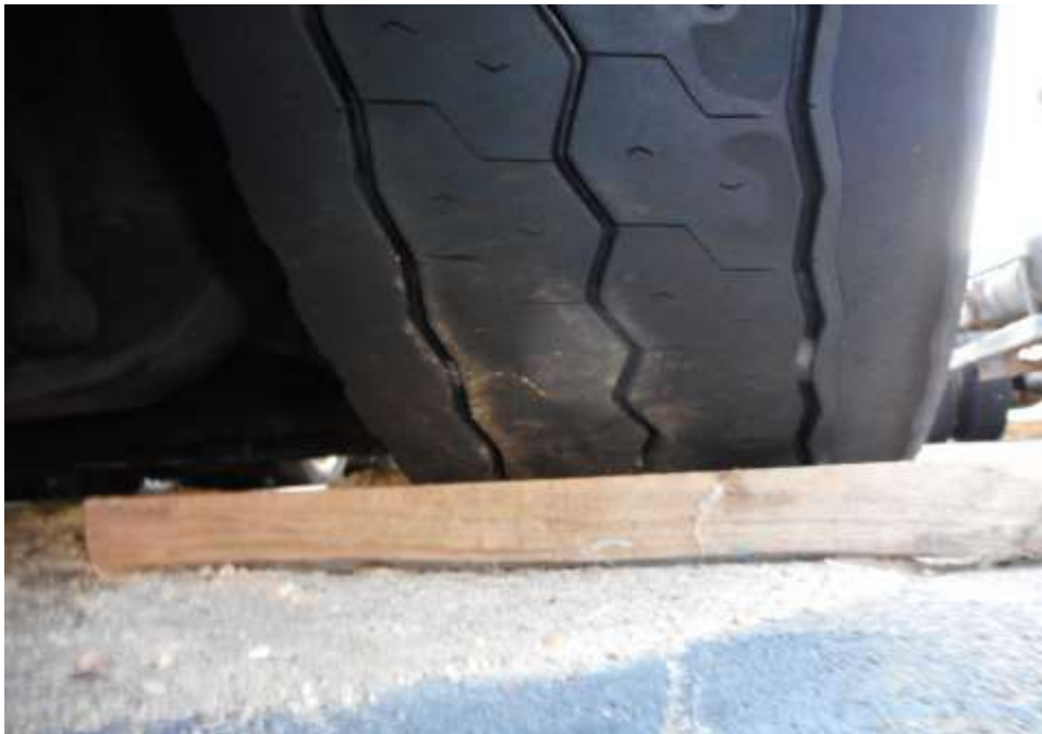
Photo 9 shows the condition of the front left tyres of the Motor Bus, which were observed to be in serviceable condition with remaining tread depth of approximately 8.6mm. There was also no tear, cut or burst mark(s) on the outer and the inner sidewalls as well as across the tread of the 6 tyres that were fitted on the Motor Bus.
