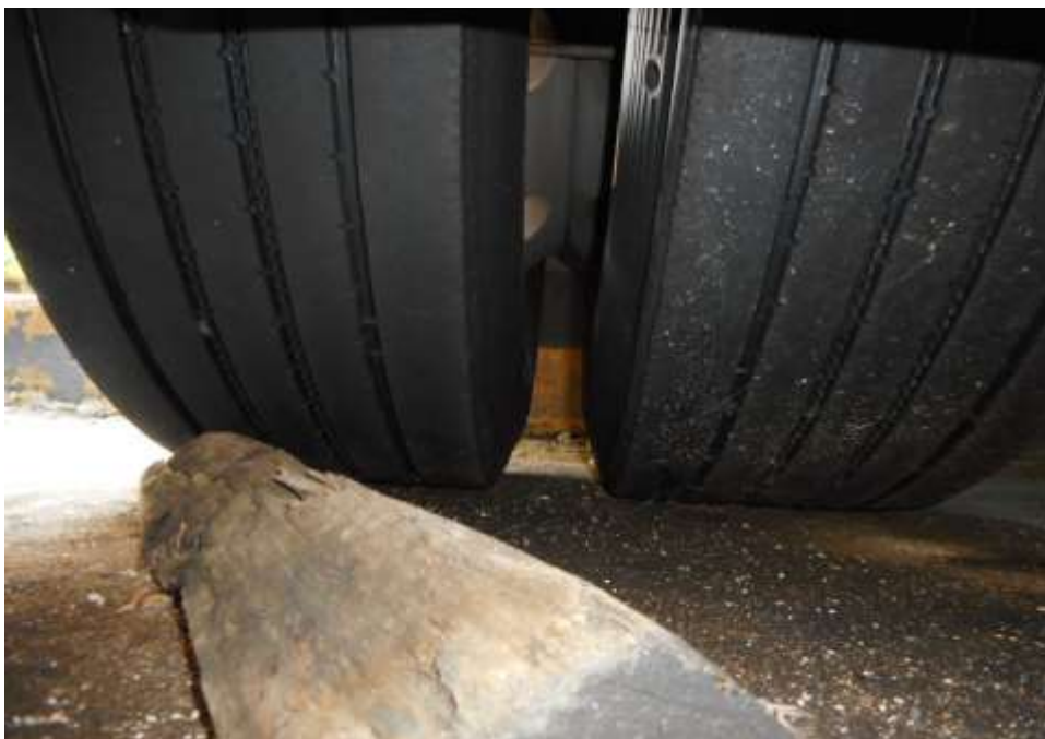
Photo 7 shows the condition of the rear right tyre of the Motor Bus, which was observed to be in serviceable condition with remaining tread depth of approximately 6.6mm. The tyre, which was wrapped around standard steel wheel rim, was also observed to be sufficiently inflated for vehicular operation.
