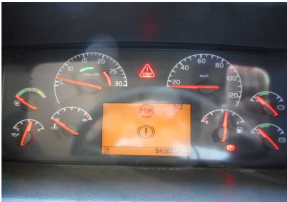
Photo 24 shows no warning lights illuminated on the instrument panel of the Motor Bus after the engine was cranked. This would suggest that there was no abnormality to the various electronic operating systems of the Motor Bus, like the ABS.
