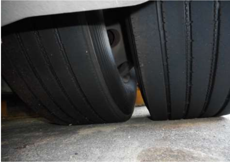
Photo 8 shows the condition of the rear left tyres of the Motor Bus, which was observed to be in serviceable condition with remaining tread depth of approximately 6.4mm. The tyres, which were wrapped around standard steel wheel rim, were also observed to be sufficiently inflated for vehicular operation. There was also no damage found on all 6 steel wheel rims of the Motor Bus.
