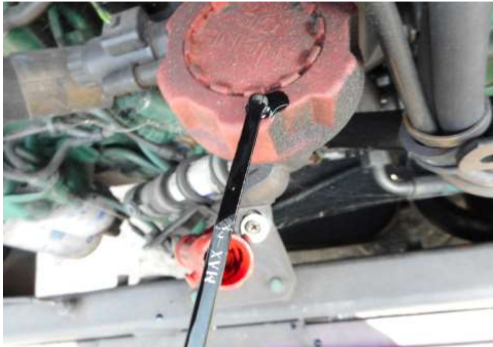
Photo 17 shows the engine oil dip stick of the Motor Bus at the time of my inspection. The engine oil was observed to be of sufficient level and without any visible contamination.
