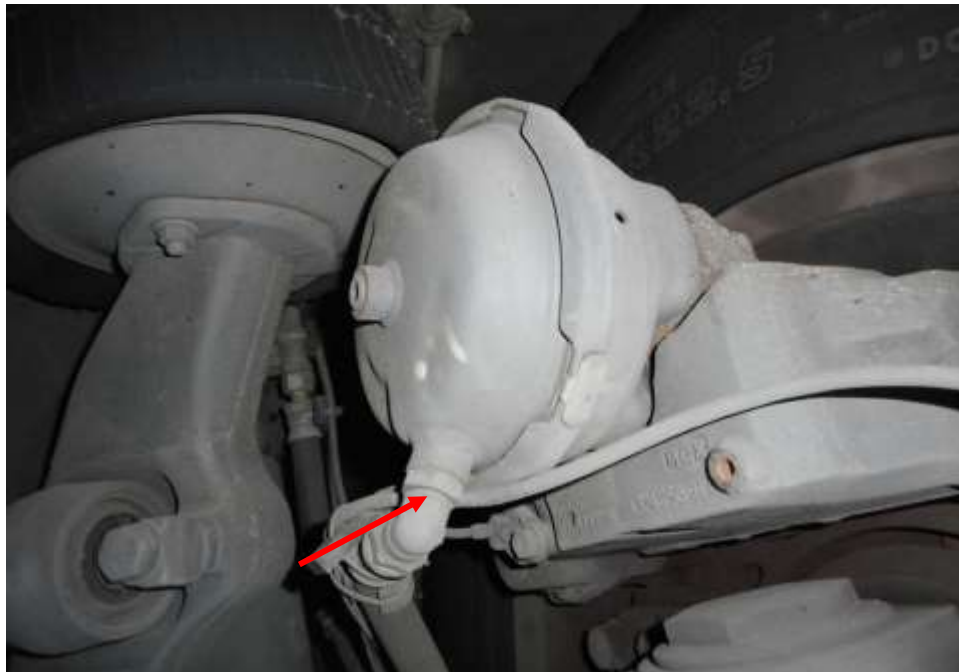
Photo 19 shows the brake pipe (arrowed) at the front left wheel of the Motor Bus was observed to be intact at the time of my inspection.
