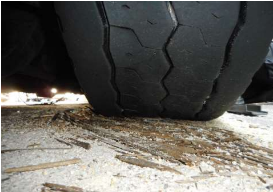
Photo 6 shows the condition of the front right tyre of the Motor Bus, which was observed to be in serviceable condition with remaining tread depth of approximately 10.2 mm. The tyre, which was wrapped around standard steel wheel rim, was also observed to be sufficiently inflated for vehicular operation. There was no tear, cut or burst mark(s) on the outer and the inner sidewalls as well as across the tread of the 6 tyres that were fitted on the Motor Bus.
