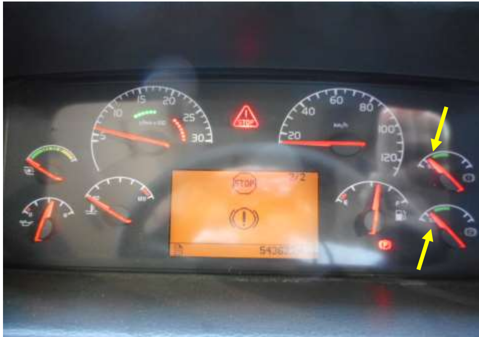
Photo 11 shows the air readings from the air brake cylinders of the Motor Bus at the time of my inspection. The air in the cylinder (arrowed) was observed to be of insufficient level at the time of my inspection as damage to the air brake hoses and as components was found which caused an air leak, due to the towing process of the Motor Bus.
