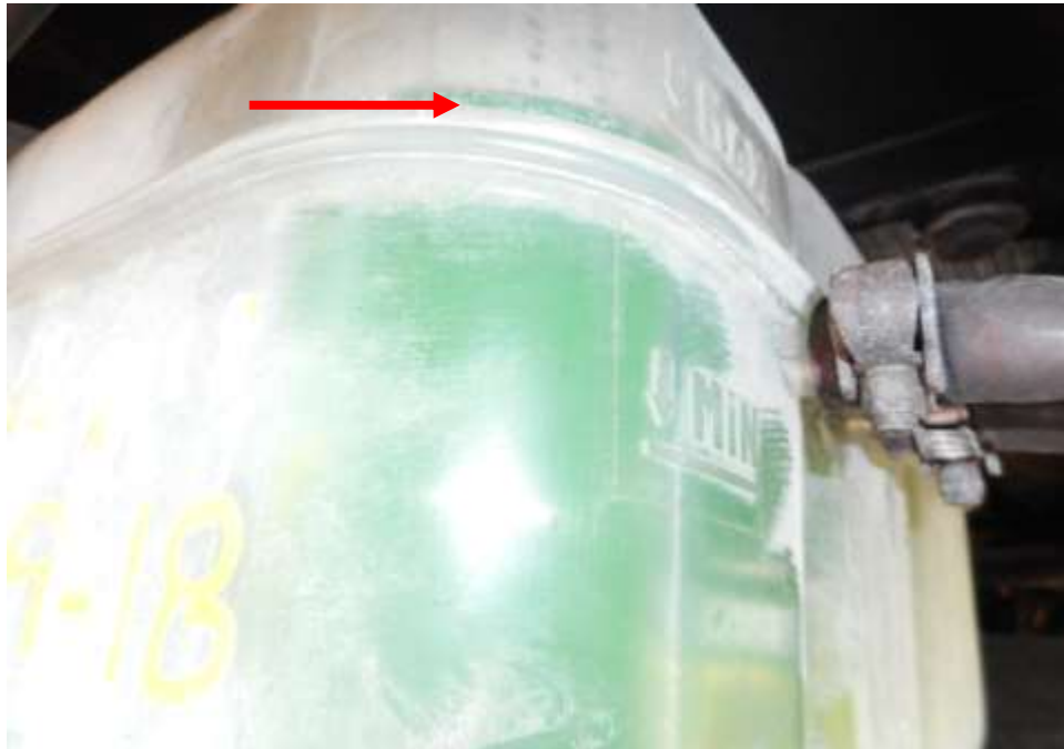
Photo 15 shows the engine coolant reservoir of the Motor Bus at the time of my inspection. The engine coolant was observed to be of sufficient level and without any visible contamination.
