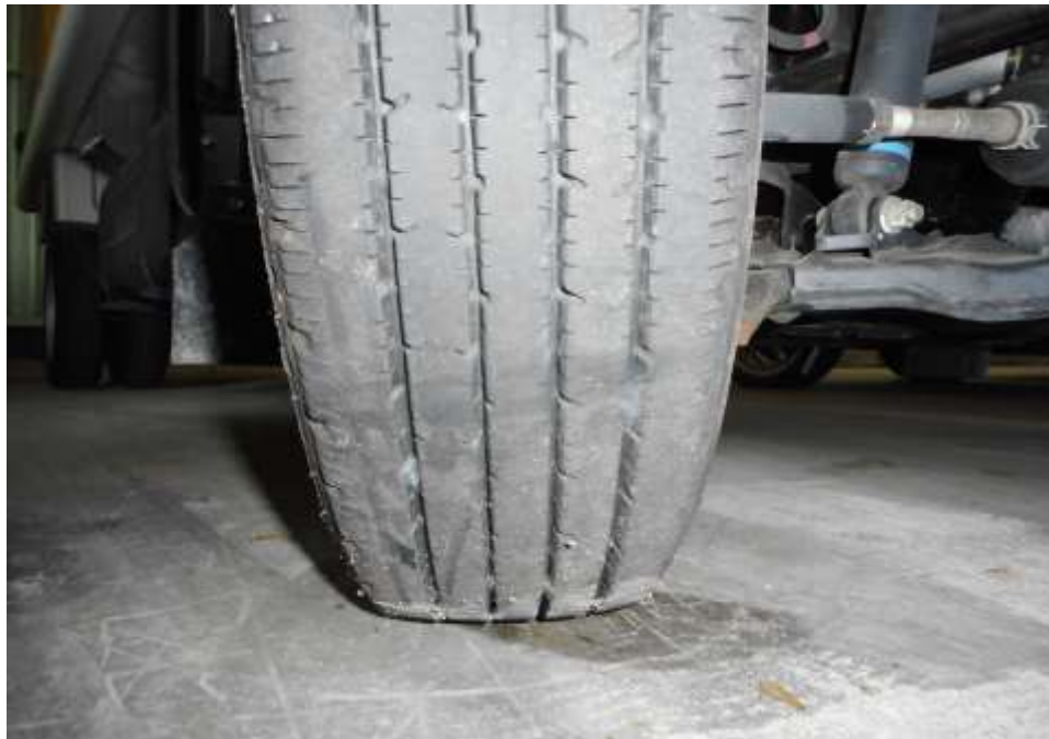
Photo 9 shows the condition of the front right tyre of the Motor Lorry, which was observed to be in serviceable condition with remaining tread depth of approximately 5.9mm. The tyre, which was wrapped around standard steel wheel rim, was also observed to be sufficiently inflated for vehicular operation. There was no tear, cut or burst mark(s) on the outer and the inner sidewalls as well as across the tread of the 6 tyres that were fitted on the Motor Lorry.
