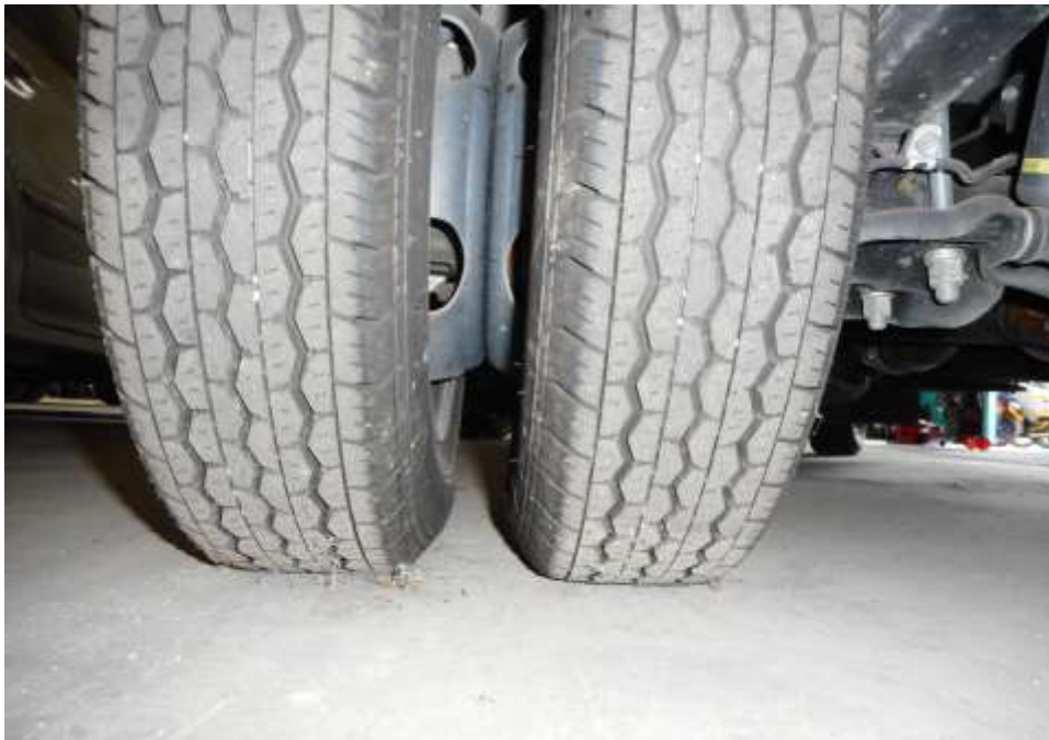
Photo 11 shows the condition of the rear left tyres of the Motor Lorry, which was observed to be in serviceable condition with remaining tread depth of approximately 4.7mm. The tyres, which were wrapped around standard steel wheel rim, were also observed to be sufficiently inflated for vehicular operation. There was also no damage found on all 6 steel wheel rims of the Motor Lorry.
