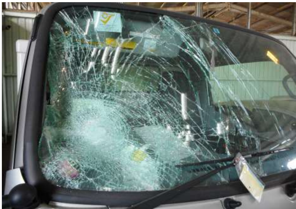
Photo 3 shows a close up view of the Motor Lorry's front body at the time of my inspection. It was observed to have sustained major damage at its frontal portion. Its front windscreen was damage as a result of the accident.
