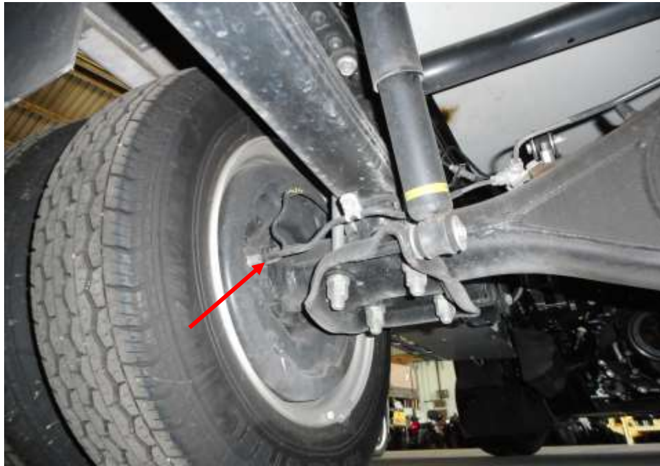
Photo 22 shows the brake pipe (arrowed) at the rear left wheel of the Motor Lorry. I did not observe any leakage of brake fluid at the time of my inspection of the Motor Lorry. My static tests of the Motor Lorry's braking system, along with my visual examination of the various mechanical components in the braking System had indicated that there was no internal leakage of pressure/vacuum. Hence the braking system of the Motor Lorry was likely to be in serviceable condition at the material time of accident.
