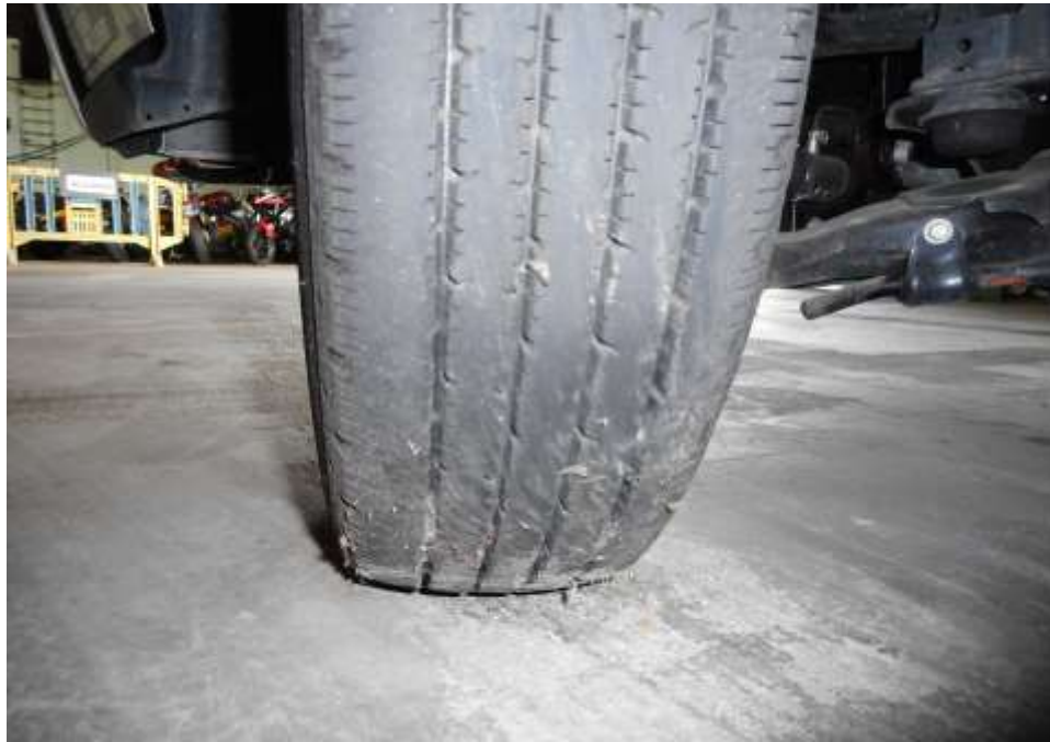
Photo 12 shows the condition of the front left tyres of the Motor Lorry, which were observed to be in serviceable condition with remaining, tread depth of approximately 7.2mm. There was also no tear, cut or burst mark(s) on the outer and the inner sidewalls as well as across the tread of the 6 tyres that were fitted on the Motor Lorry.
