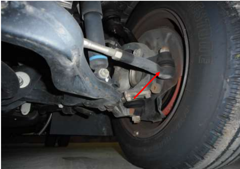
Photo 20 shows the various undercarriage components at the front left wheel of the Motor Lorry, in particular the steering tie rod end (arrowed). The various steering components were all found to be intact, suggesting that the steering system of the Motor Lorry was likely to be in serviceable condition at the material time of accident. There was also no sign of fluid stain(s) observed on the various undercarriage components.
