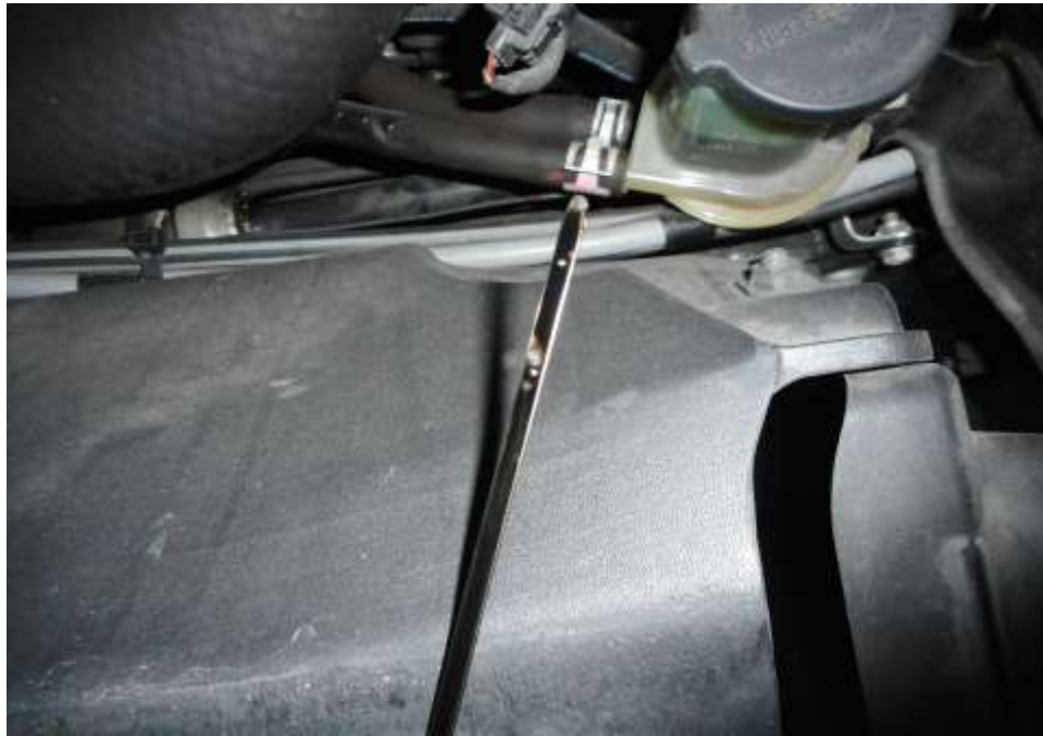
Photo 17 shows the engine dip stick of the Motor Lorry at the time of my inspection. The engine oil was observed to be of sufficient level and without any visible contamination.
