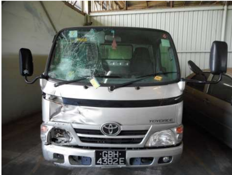
Photo 2 shows a general view of the Motor Lorry's front body at the time of my inspection. It was observed to have sustained major damage at its frontal portion. Its front windscreen, right side mirrors, front panel body panel, right headlamp, fog lights, front bumper, right side undercarriage wheel arch panel and mud flap were damage as a result of the accident.
