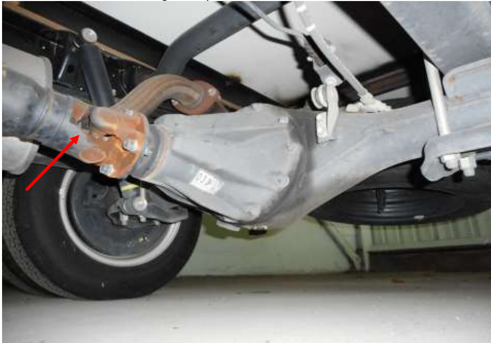
Photo 25 shows the various undercarriage components at the drive shaft of the Motor Lorry, in particular the rear drive shaft and the rear differential (arrowed). The various steering components were all found to be intact and there was also no sign of fluid stain(s) observed, suggesting that the steering system of the Motor Lorry was likely to be in serviceable condition at the material time of accident. There was also no sign of fluid stain(s) observed on the various undercarriage components.
