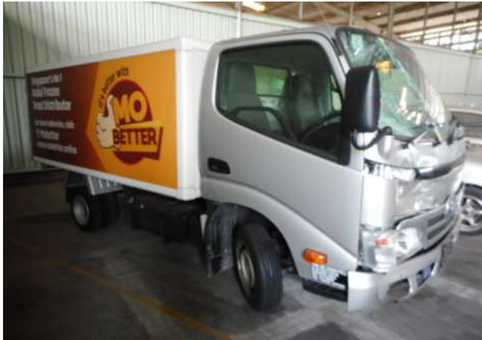
Photo 6 shows a general view of the front right body of the Motor Lorry at the time of my inspection. The Motor Lorry was observed to be in good general condition and unaffected from the accident.
