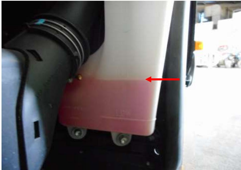
Photo 15 shows the engine coolant reservoir of the Motor Lorry at the time of my inspection. The engine coolant was observed to be of sufficient level and without any visible contamination.
