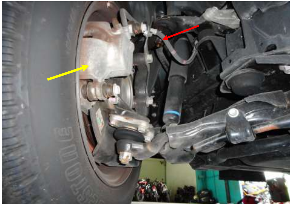
Photo 23 shows the brake hose/pipe (red arrow) at the front left wheel of the Motor Lorry. No leakage of brake fluid was observed. Visual examination of the various components of the braking system like the brake caliper (yellow arrow), brake booster, brake pedal etc had revealed all to be intact and without visible damage at the time of accident. There was also no sign of fluid stain(s) observed on the various undercarriage components.
