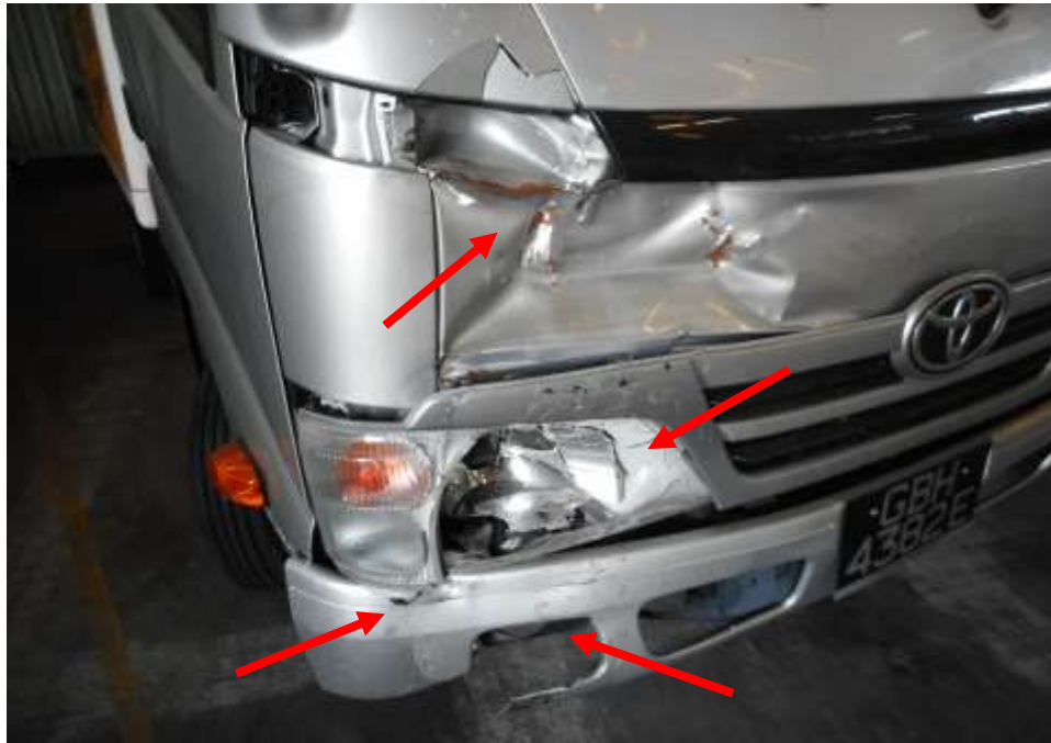
Photo 4 shows a close up view of the Motor Lorry's front body at the time of my inspection. It was observed to have sustained major damage at its frontal portion. Its front panel body panel, right headlamp, fog lights and front bumper (arrowed) were damage as a result of the accident.
