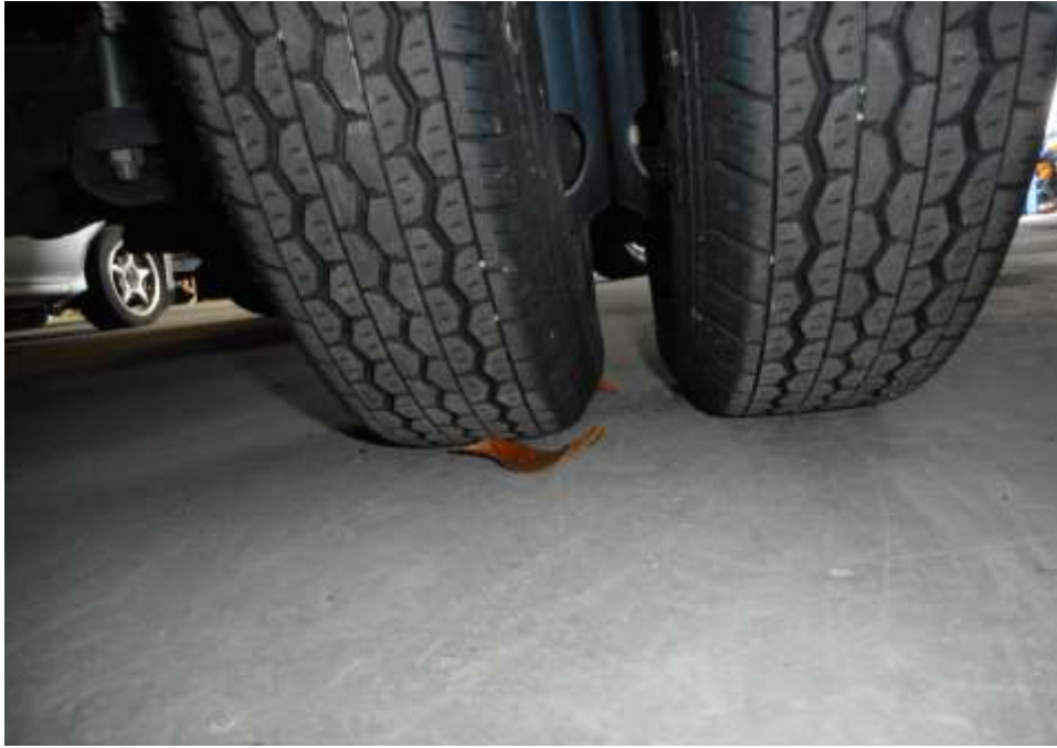
Photo 10 shows the condition of the rear right tyre of the Motor Lorry, which was observed to be in serviceable condition with remaining tread depth of approximately 4.7mm. The tyre, which was wrapped around standard steel wheel rim, was also observed to be sufficiently inflated for vehicular operation.
