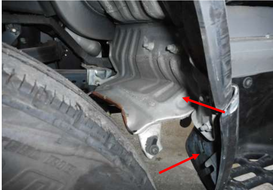
Photo 5 shows a close up view of the Motor Lorry's front body at the time of my inspection. It was observed to have sustained major damage at its frontal portion. Its right side undercarriage wheel arch panel and mud flap (arrowed) were damage as a result of the accident.
