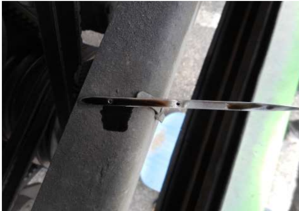
Photo 15 shows the engine oil dip stick system of the Motor Bus at the time of my inspection. The engine oil was observed to be of sufficient level and without any visible contamination.
