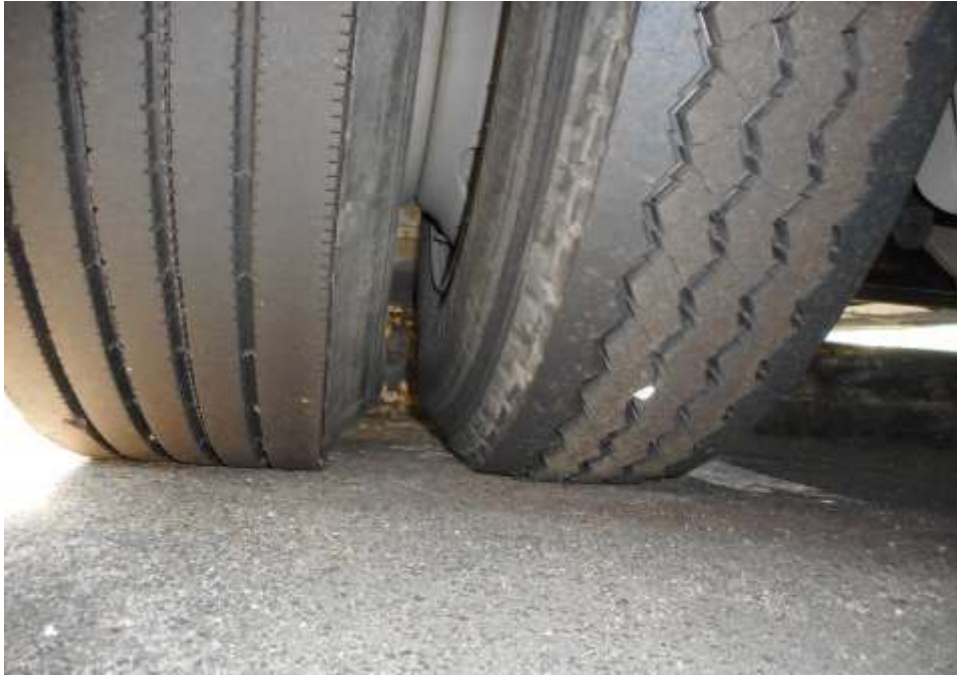
Photo 8 shows the condition of the rear right tyre of the Motor Bus, which was observed to be in serviceable condition with remaining tread depth of approximately 8.7mm. The tyre, which was wrapped around standard steel wheel rim, was also observed to be sufficiently inflated for vehicular operation.
