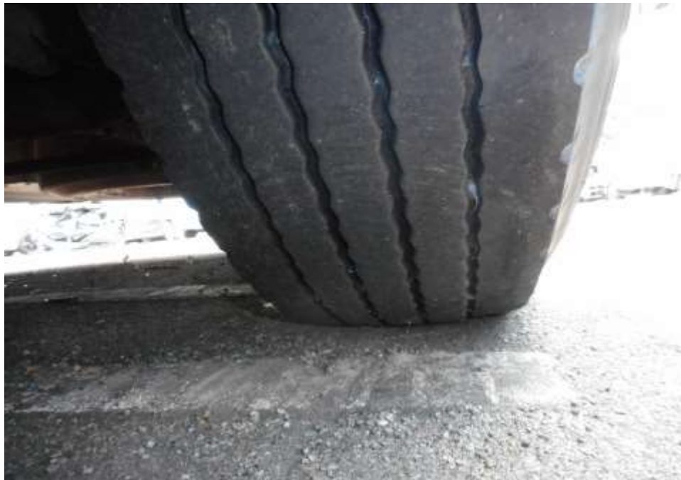
Photo 7 shows the condition of the front right tyre of the Motor Bus, which was observed to be in serviceable condition with remaining tread depth of approximately 7.2 mm. The tyre, which was wrapped around standard steel wheel rim, was also observed to be sufficiently inflated for vehicular operation. There was no tear, cut or burst mark(s) on the outer and the inner sidewalls as well as across the tread of the 6 tyres that were fitted on the Motor Bus.
