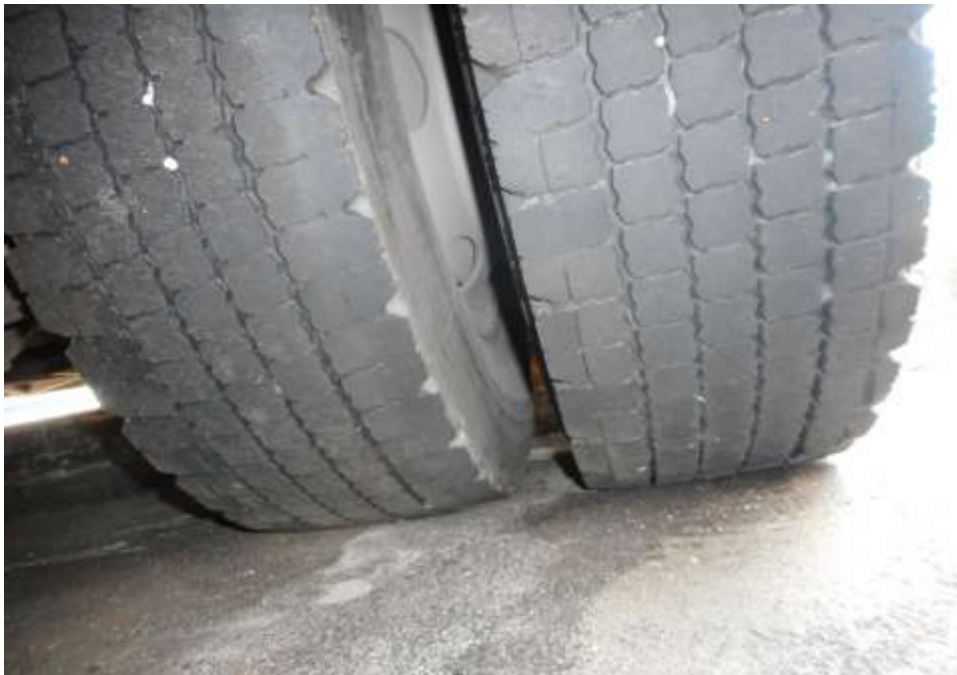
Photo 9 shows the condition of the rear left tyres of the Motor Bus, which was observed to be in serviceable condition with remaining tread depth of approximately 7mm. The tyres, which were wrapped around standard steel wheel rim, were also observed to be sufficiently inflated for vehicular operation. There was also no damage found on all 6 steel wheel rims of the Motor Bus.
