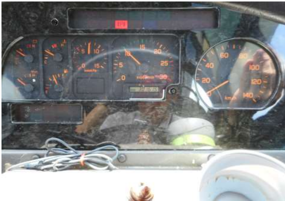
Photo 26 shows no warning lights illuminated on the instrument panel of the Motor Bus after the engine was cranked. This would suggest that there was no abnormality to the various electronic operating systems of the Motor Bus, like the ABS.
