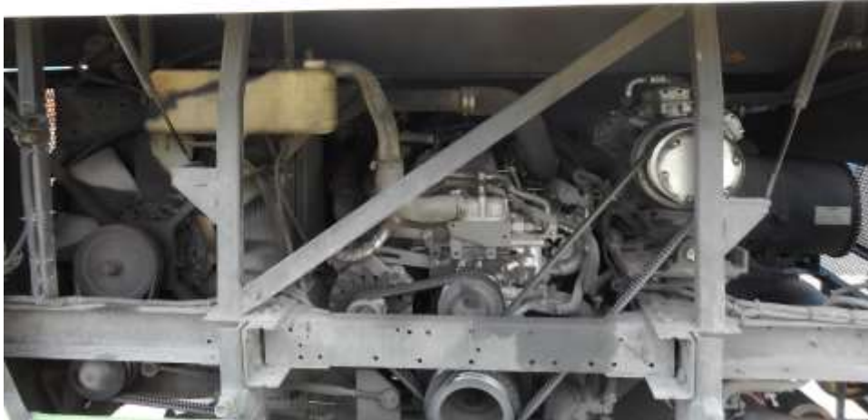
Photo 11 shows a general view of the Motor Bus's engine compartment, which was accessed by lifting the front cabin of the Motor Bus. The various parts and components inside the engine compartment were unaffected by the accident. There was also no sign(s) or indication(s) of fresh fluid leakage and/or fluid stain within the engine compartment (photograph shows the engine compartment as viewed from the right front side of the Motor Bus).
