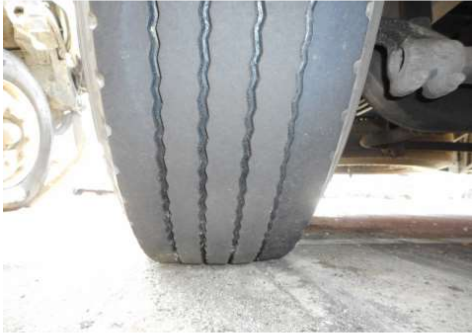
Photo 10 shows the condition of the front left tyres of the Motor Bus, which were observed to be in serviceable condition with remaining tread depth of approximately 7.7mm. There was also no tear, cut or burst mark(s) on the outer and the inner sidewalls as well as across the tread of the 6 tyres that were fitted on the Motor Bus.
