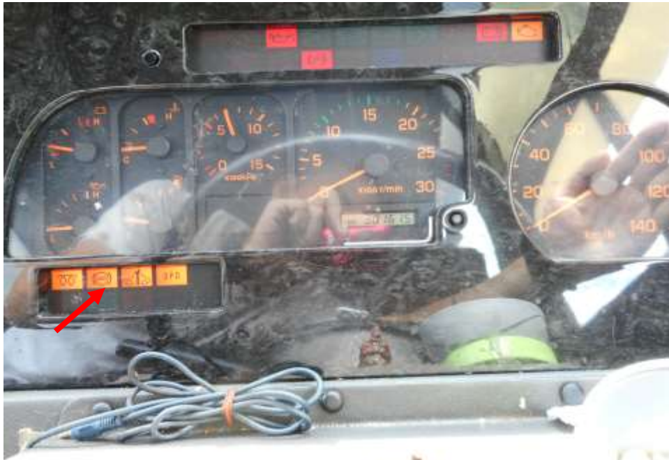
Photo 25 shows the warning light for Anti-Lock Brake System (ABS) appearing on the instrument panel of the Motor Bus during the self-test of its various electronic operating systems when its engine was cranked.
