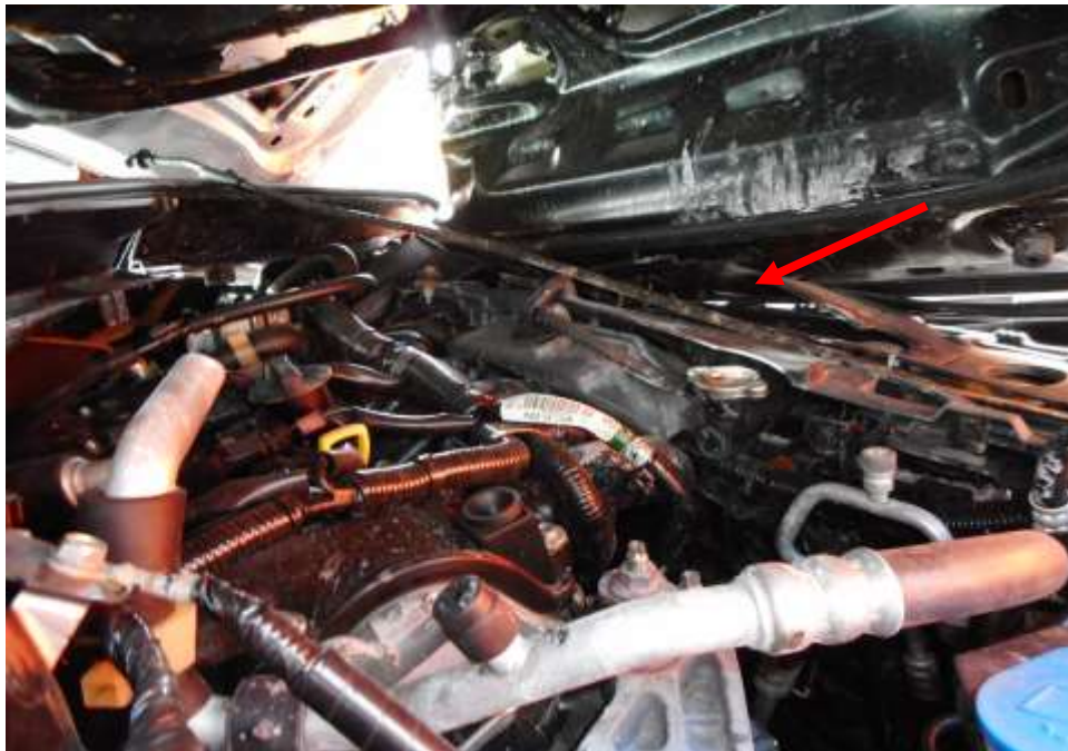
Photo 16 shows the damage to the bonnet locking mechanism (arrowed) Motor Car's front bonnet, rendering it unable to be unlocked and lifted up to carry out examination of the Motor Car's engine compartment as a result of the accident.
