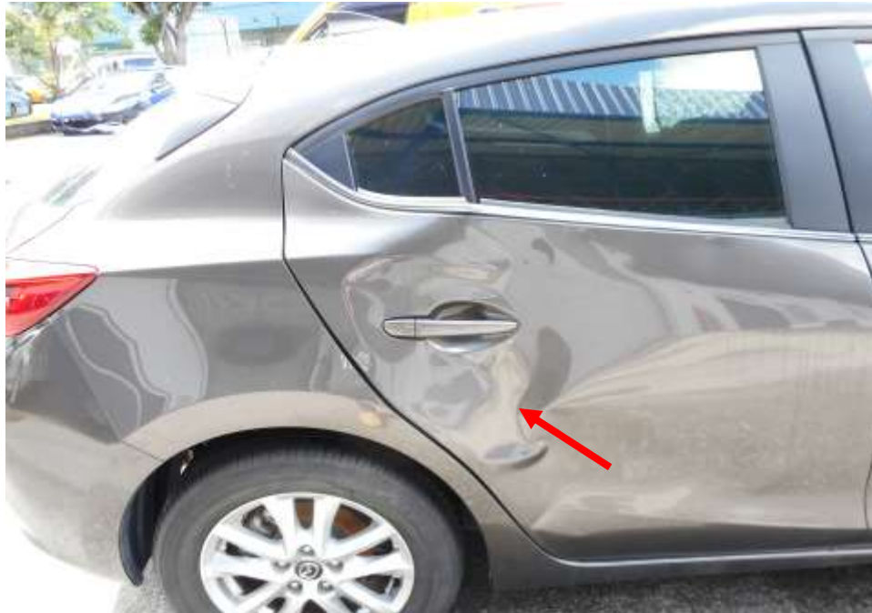
Photo 13 shows close up view of the left portion of the Motor Car at the time of my inspection. Its rear passenger door panel (arrowed) was damage as a result of the accident.
