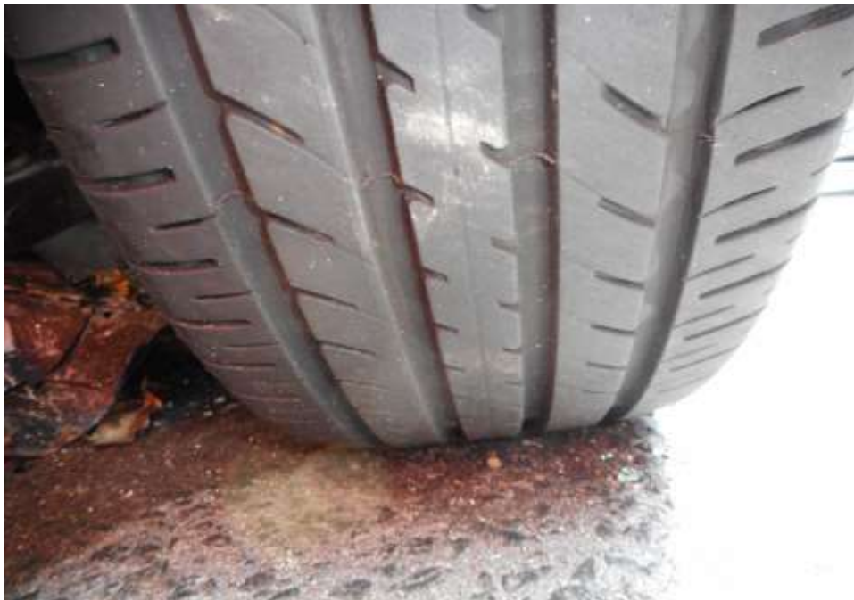
Photo 15 shows the condition of the front left tyre of the Motor Car, which was observed to be in serviceable condition with remaining tread depth of approximately 6.4mm. There was no tear, cut or burst mark(s) on the outer and the inner sidewalls as well as across the tread of this tyre.
