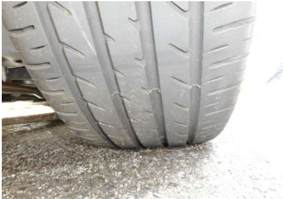
Photo 13 shows the condition of the rear right tyre of the Motor Car, which was observed to be in serviceable condition with remaining tread depth of approximately 5.1mm. There was no tear, cut or burst mark(s) on the outer and the inner sidewalls as well as across the tread of this tyre.
