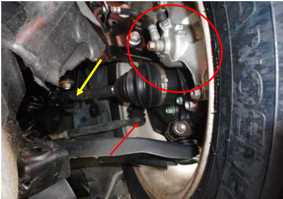
Photo 19 shows the various undercarriage components at the front left wheel of the Motor Car, which had included the steering tie rod (red arrow) and front left drive shaft (yellow arrow), its brake caliper and brake hoses (circled). The various undercarriage components of the Motor Car were all found to be intact without any visible damage.
