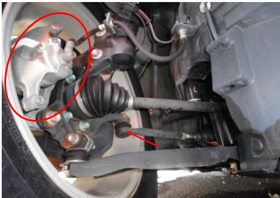
Photo 17 shows the undercarriage components at the front right wheel of the Motor Car. My checks on the underside of the Motor Car revealed damage to the various undercarriage components, the steering rack and pinion, tie rods, tie rod ends and ball joints (arrowed), the brake caliper and brake hoses (circled) revealed that these components were all generally intact.
