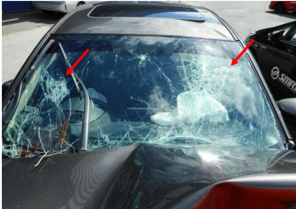
Photo 3 shows a close up view of the front windscreen of the Motor Car at the time of my inspection. The front windscreen (arrowed) of the Motor Car was observed to have been damaged as a result of the accident
