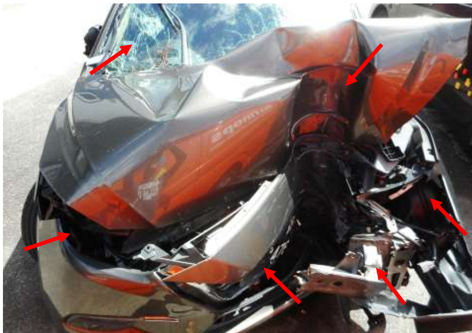
Photo 4 shows a general view of the front right portion of the Motor Car at the time of my inspection. its front windscreen, front bonnet, front bumper, front number plate, both front left and right headlamp (arrowed) were amongst the body parts that were observed to have been damaged as a result of the accident.
