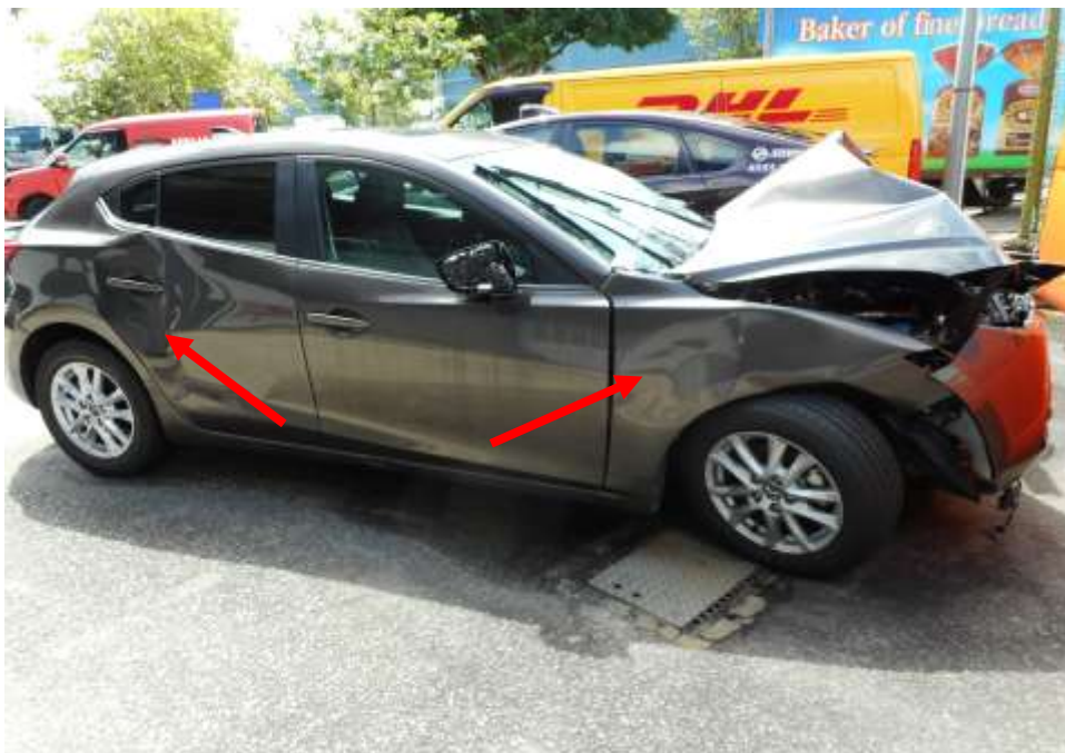
Photo 12 shows a general view of the left portion of the Motor Car at the time of my inspection. The left portion of the Motor Car was observed to have been affected by the accident. Its front fender and rear passenger door panel (arrowed) was damage as a result of the accident.
