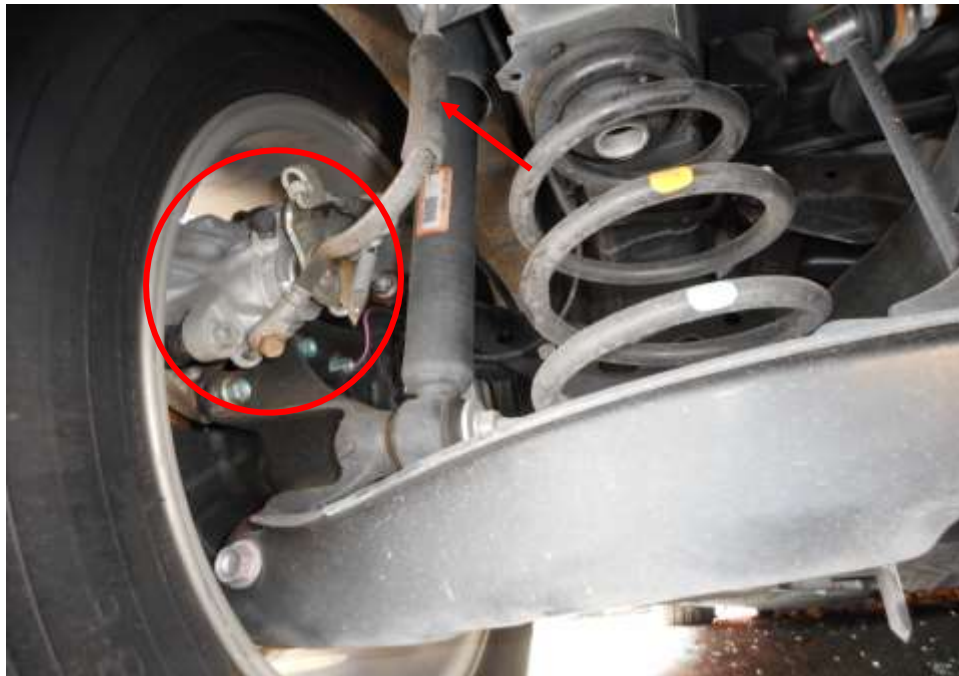
Photo 21 shows the various undercarriage components at the rear left wheel of the Motor Car, in particular the brake hose (arrowed) and brake caliper (circled). I did not observe any leakage of brake fluid at the 4 wheels of the Motor Car. My visual inspection of the various mechanical components of the Motor Car's braking system revealed all to be intact and without visible damage.
