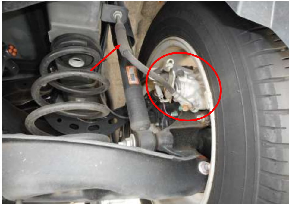
Photo 20 shows the various undercarriage components at the rear right wheel of the Motor Car, in particular the brake hose (arrowed) and brake caliper (circled). I did not observe any leakage of brake fluid at the 4 wheels of the Motor Car. My visual inspection of the various mechanical components of the Motor Car's braking system revealed all to be intact and without visible damage.
