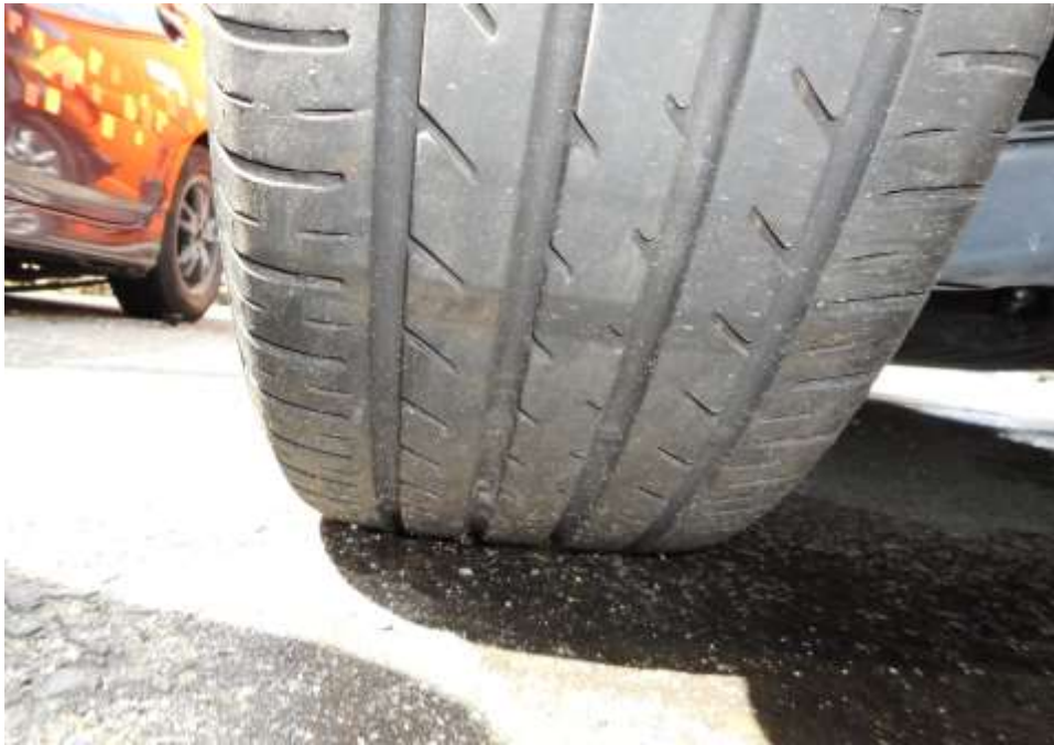
Photo 14 shows the condition of the rear left tyre of the Motor Car, which was observed to be in serviceable condition with remaining tread depth of approximately 5.7mm. There was no tear, cut or burst mark(s) on the outer and the inner sidewalls as well as across the tread of this tyre.
