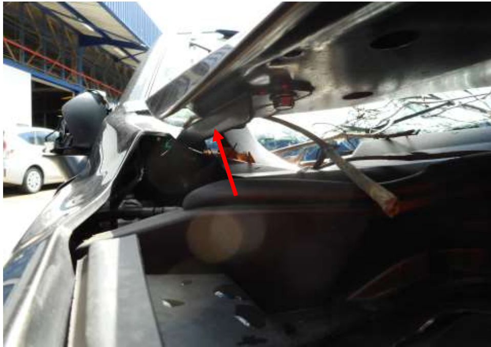
Photo 7 shows a close up view of the right bonnet hinge of the Motor Car at the time of my inspection. The right bonnet hinge of the Motor Car was observed to have been damaged as a result of the accident rendering the bonnet unable to be opened (arrowed)
