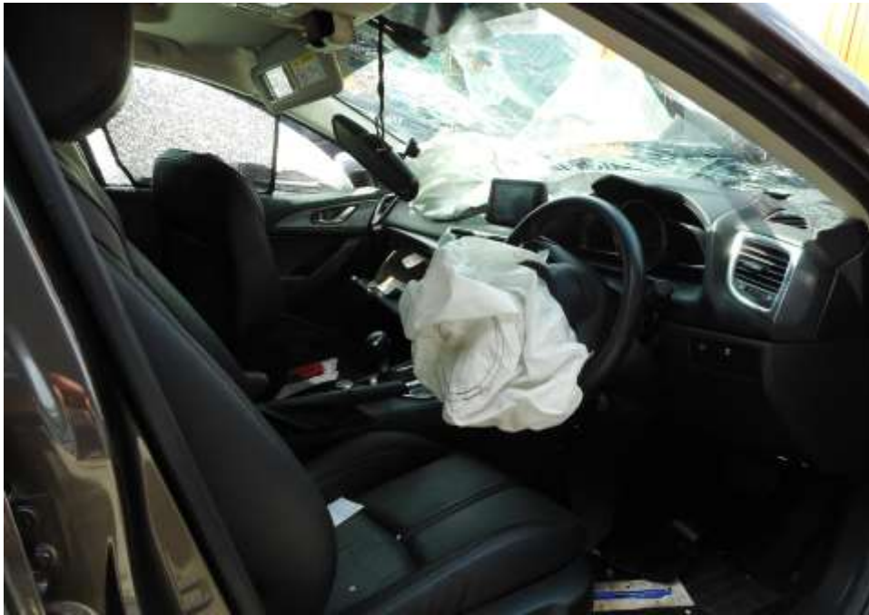
Photo 11 shows a general view of the Motor Car's interior compartment. Both the driver and front passenger air bags were also deployed as a result of the accident.
