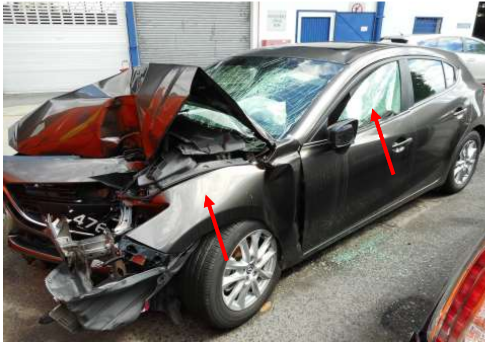
Photo 9 shows a general view of the front left portion of the Motor Car at the time of my inspection. The front left fender and the front left passenger windscreen panel (arrowed) of the Motor Car was observed to have been damaged as a result of the accident.
