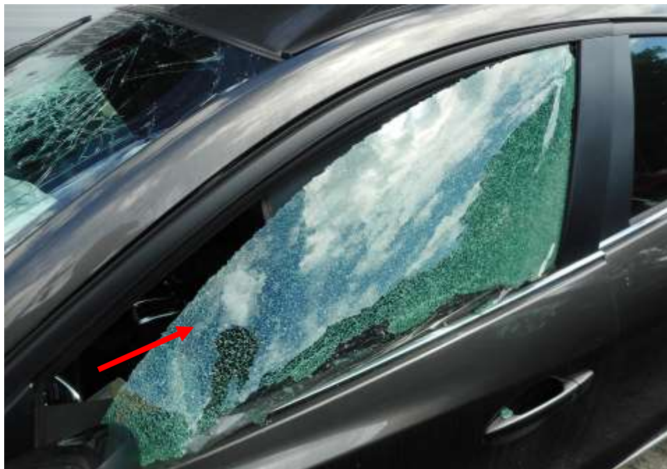
Photo 10 shows the close up view of the left panel portion of the Motor Car at the time of my inspection. The front left passenger windscreen (arrowed) of the Motor Car was observed to have been damaged as a result of the accident.
