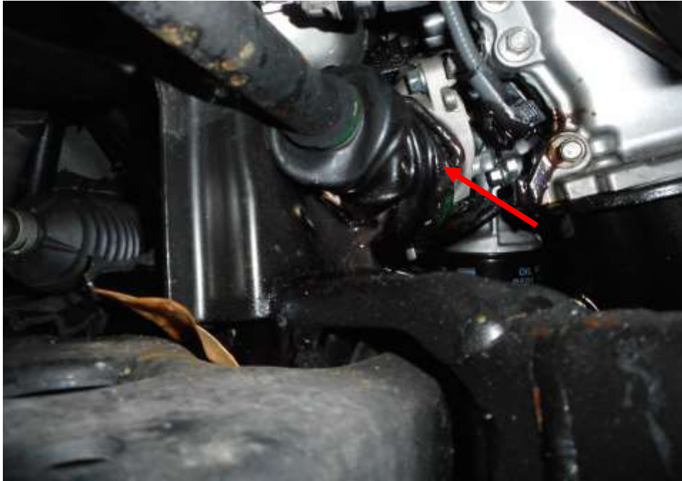
Photo 18 shows the undercarriage components at the front right wheel of the Motor Car. My checks on the underside of the Motor Car revealed damage to the various undercarriage components, the driveshaft inner rubber boot (arrowed) was found to be broken with fresh fluid leakage as a result of the accident. At the time of our inspection
