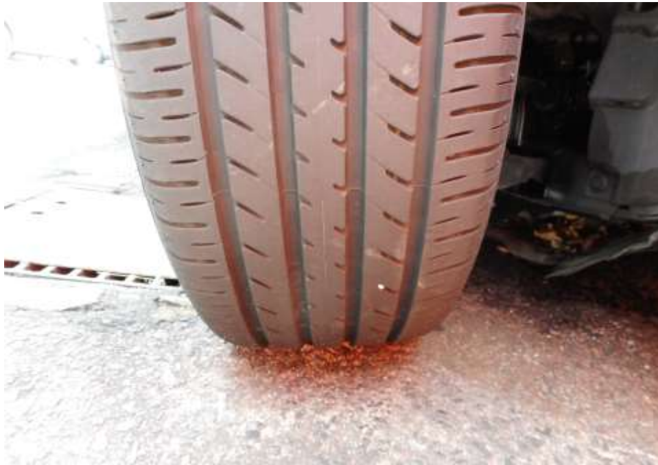
Photo 12 shows the condition of the front right tyre of the Motor Car, which was observed to be in serviceable condition with remaining tread depth of approximately 6.9mm. There was no tear, cut or burst mark(s) on the outer and the inner sidewalls as well as across the tread of this tyre.
