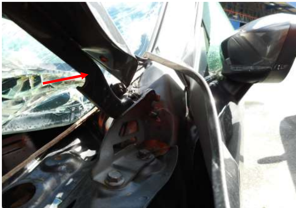
Photo 8 shows a close up view of the left bonnet hinge of the Motor Car at the time of my inspection. The left bonnet hinge of the Motor Car was observed to have been damaged as a result of the accident rendering the bonnet unable to be opened (arrowed)
