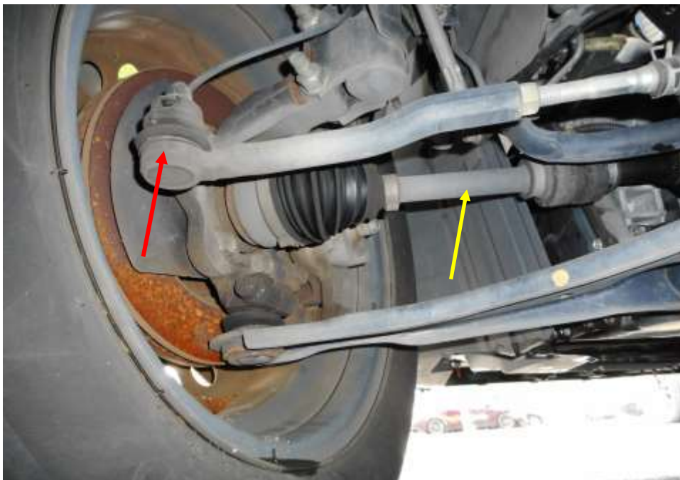
Photo 21 shows the various undercarriage components at the front left wheel of the Motor Car, which had included the steering tie rod (red arrow) and front left drive shaft (yellow arrow). The various undercarriage components of the Motor Car were all found to be intact without any visible damage.
