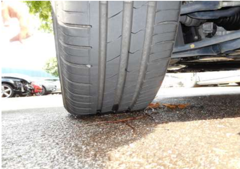
Photo 10 shows the condition of the front left tyre of the Motor Car, which was observed to be in serviceable condition with remaining tread depth of approximately 6.3mm. The tyre, which was wrapped around alloy wheel rim, was also observed to be sufficiently inflated for vehicular operation. The 4 tyres of the Motor Car were wrapped around standard alloy wheel rims that were without any significant damage apart for some relatively minor kerb grazing type of damage on the outer side of the wheel rims
