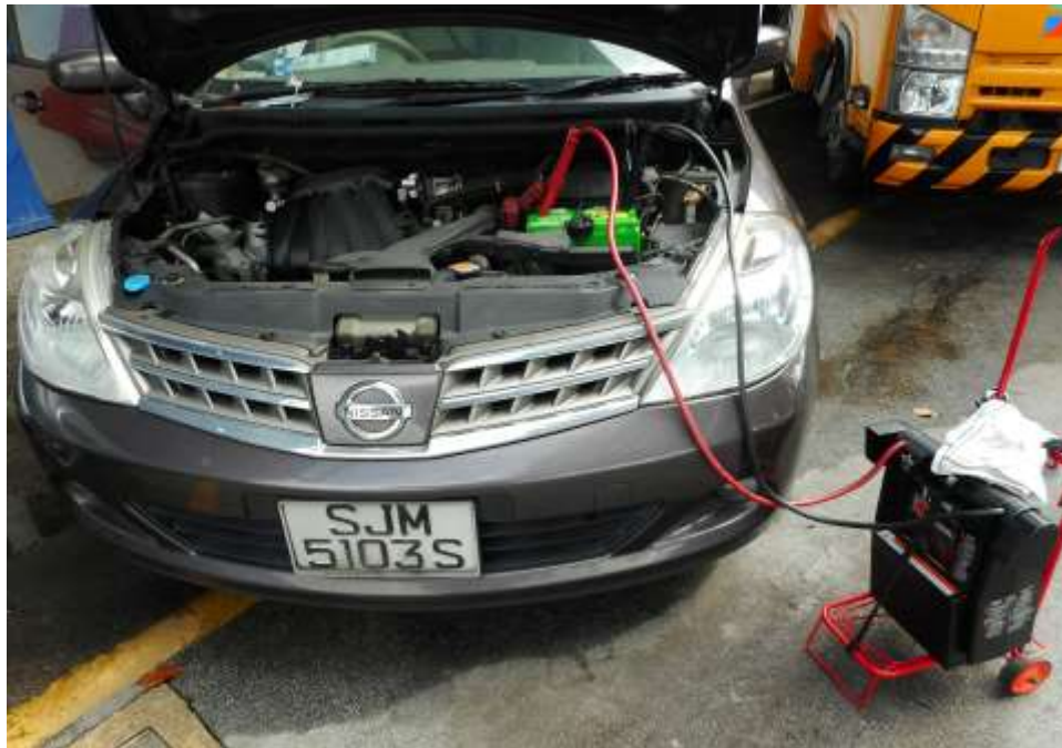
Photo 17 shows the jumpstarting process of the Motor Car with an external battery pack. The Motor Car was unable to be cranked due to a fault in the ignition system.
