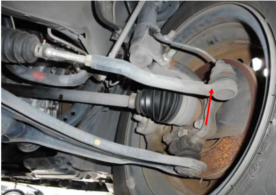
Photo 20 shows the various undercarriage components at the front right wheel of the Motor Car, in particular the steering tie rod (arrowed). The various steering components were all found to be intact; there was also no sign of fluid stain observed on the various undercarriage components at the front right wheel of the Motor Car.
