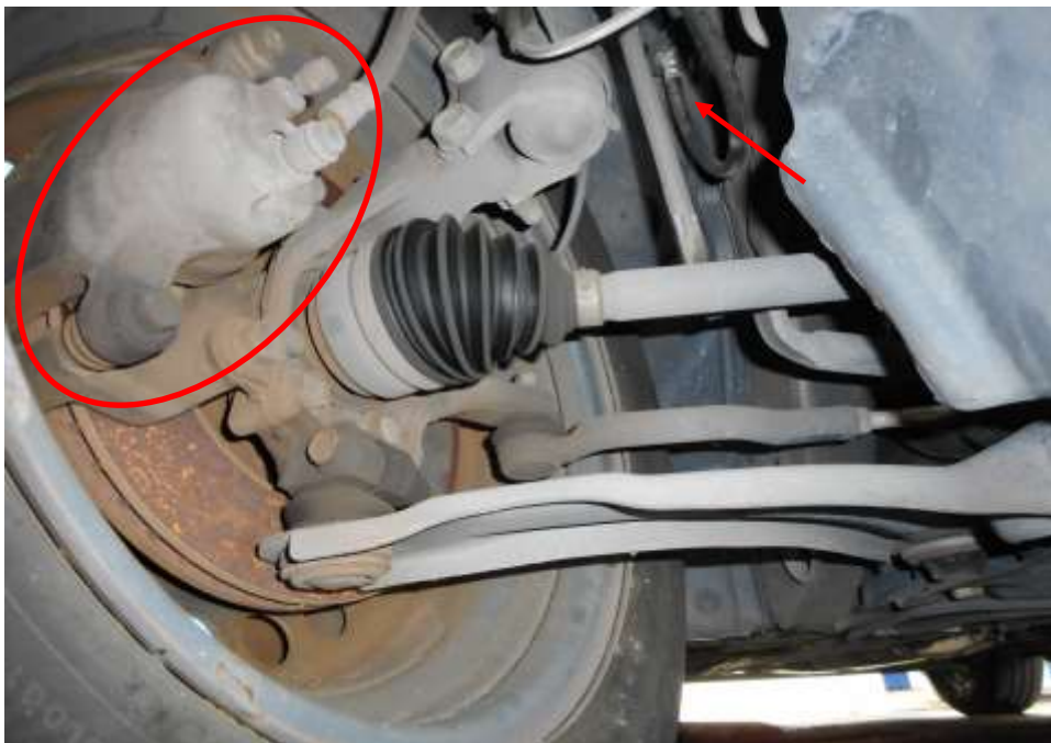
Photo 19 shows the brake hose/pipe (arrowed) at the front right wheel of the Motor Car. No leakage of brake fluid was observed. Visual examination of the various components of the braking system like the brake caliper (circled) revealed to be intact and without visible damage.
