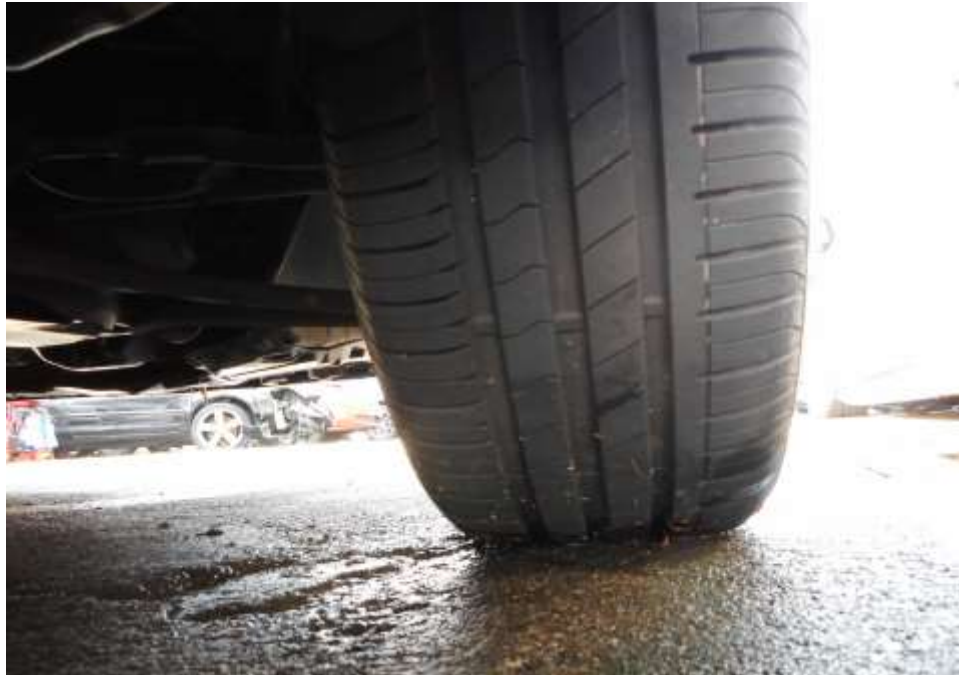
Photo 8 shows the condition of the front right tyre of the Motor Car, which was observed to be in serviceable condition with remaining tread depth of approximately 6.2mm. The tyre was sufficiently inflated for vehicular operation with no tear, cut or burst mark(s) on the outer and the inner sidewalls as well as across the tread. The 4 tyres of the Motor Car were wrapped around standard alloy wheel rims without any damage.
