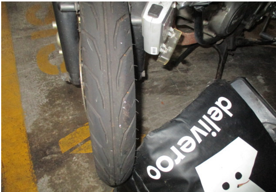
Photo 12 shows the front tyre of the Motorcycle at the time of our inspection. The front tyre was observed to be in serviceable condition with remaining tread depth of approximately 4mm. The tyre was also observed to be sufficiently inflated for vehicular operation. We did not observe any tear, burst mark(s) and/or punctured hole(s) on the sidewalls as well as across the tread of the front tyre.
