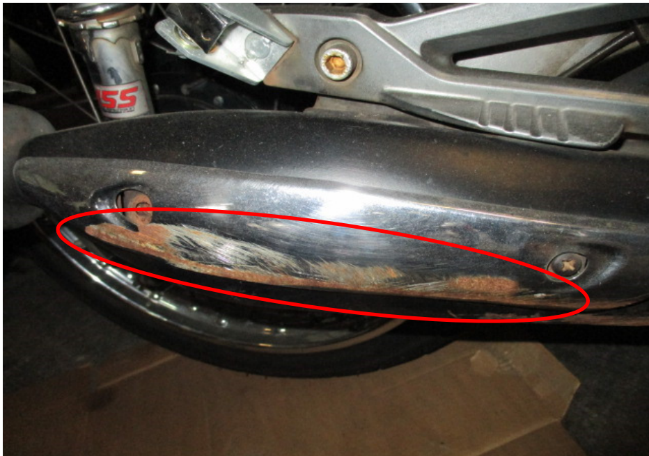
Photo 10 shows the exhaust muffler heat shield (circled) which was amongst the body parts of the Motorcycle that had sustained damage as a result of the accident.
