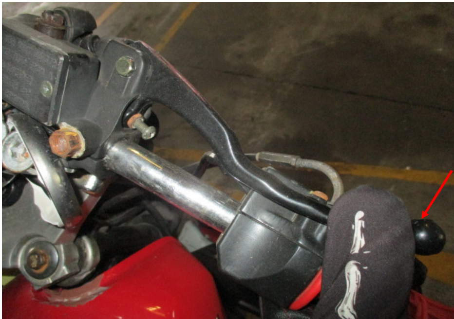
Photo 21 shows the front brake lever being depressed. There was no resistance felt (spongy like feel) upon pressing the front brake lever (arrowed). This would indicate that there is leakage of pressure/vacuum in the brake system.
