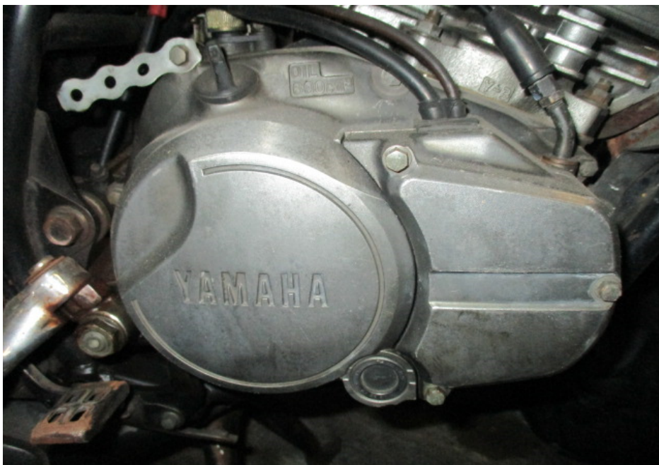
Photo 15 shows the right side of the engine of the Motorcycle at the time of our inspection. The various engine related parts and components were found to be intact with no visible damage. There was also no sign(s) or indication(s) of fluid leak observed around the right engine area of the Motorcycle.
