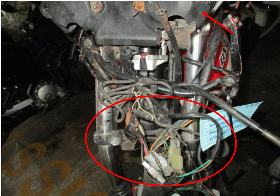
Photo 3 shows a closer view of the headlamp assembly (circled) and speedometer gauge (arrowed) which were amongst the body parts at the front body of the Motorcycle that had sustained damage as a result of the accident.
