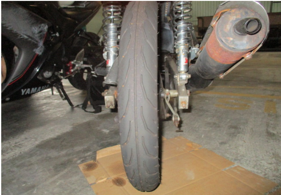
Photo 13 shows the condition of the Motorcycle's rear tyre. The rear tyre was observed to be in serviceable condition with remaining tread depth of approximately 3mm. The tyre was also observed to be sufficiently inflated for vehicular operation. We did not observe any tear, burst mark(s) and/or punctured hole(s) on the sidewalls as well as across the tread of the rear tyre.
