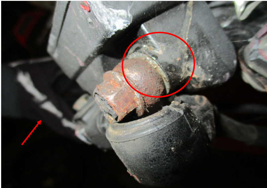
Photo 20 shows the brake fluid reservoir for the front brake of the Motorcycle. A leakage of brake fluid from the front brake fluid reservoir was observed (circled) when the front brake lever was depressed (arrowed).
