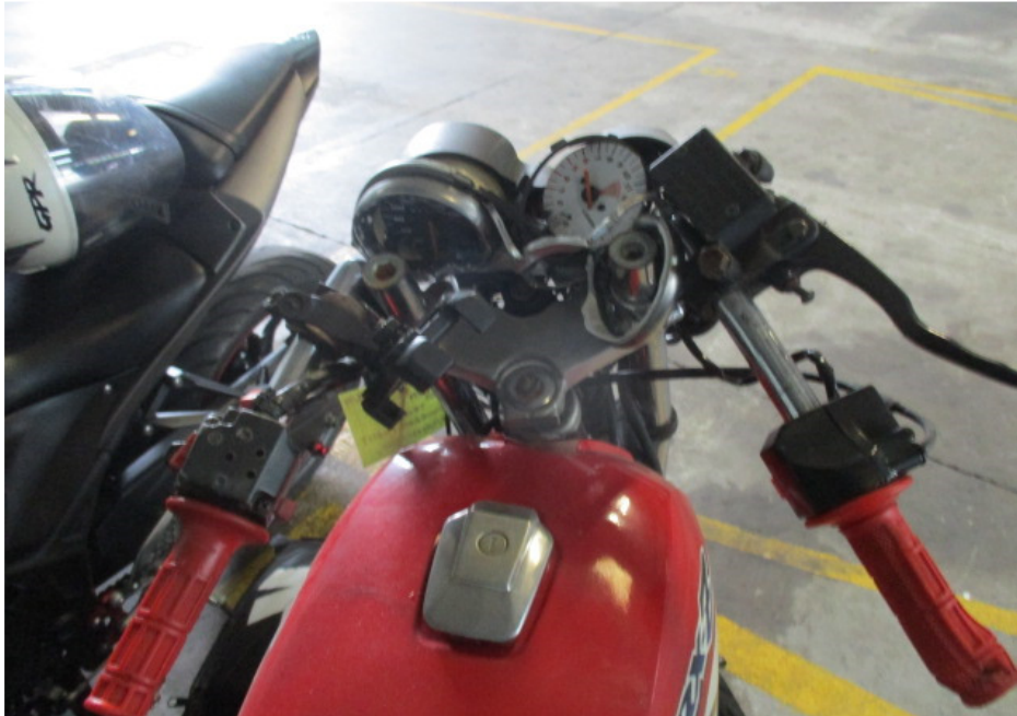
Photo 5 shows a close up view of the side mirrors, clutch lever, front brake lever, handlebars and right handlebar end of the Motorcycle. These parts were amongst the body parts of the Motorcycle which were damaged as a result of the accident.
