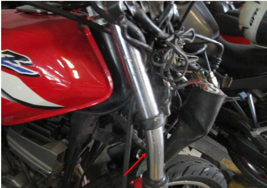
Photo 18 shows the front right fork of the Motorcycle. The front right fork (arrowed) was observed to be bent inwards as a result of the accident. We were hence not able to conduct any tests on the steering system of the Motorcycle.
