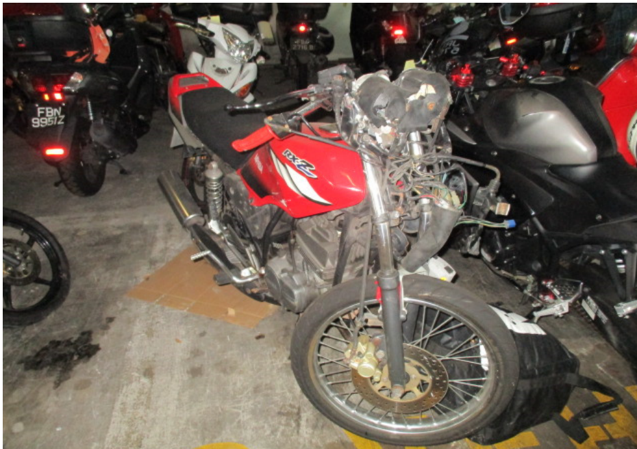
Photo 2 shows a general view of the right front body of the Motorcycle at the time of our inspection. The Motorcycle was observed to have sustained damages all around. The body parts that were found to have been damaged include its speedometer gauge, headlamp assembly, headlight, front mudguard, side mirrors, clutch lever, front brake lever, handlebars, petrol tank, right front footrest, exhaust muffler, exhaust muffler heat shield and rear side covers, amongst others.
