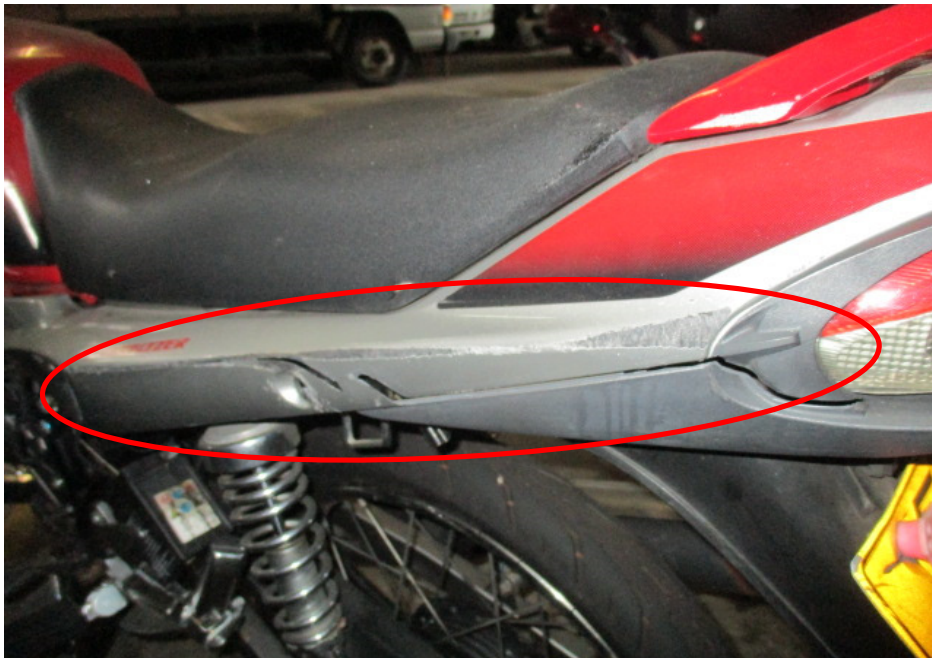
Photo 8 shows the damaged left rear side cover (circled) which was amongst the body parts of the Motorcycle that had sustained damage as a result of the accident.
