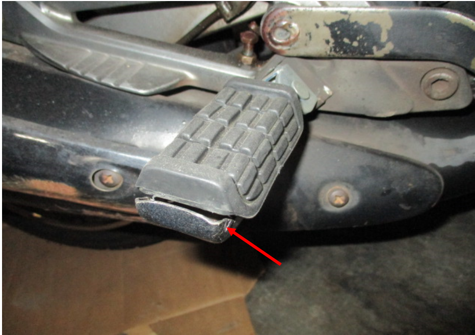
Photo 7 shows a closer view of the right front footrest (arrowed) which was amongst the body parts of the Motorcycle that had sustained damage as a result of the accident.
