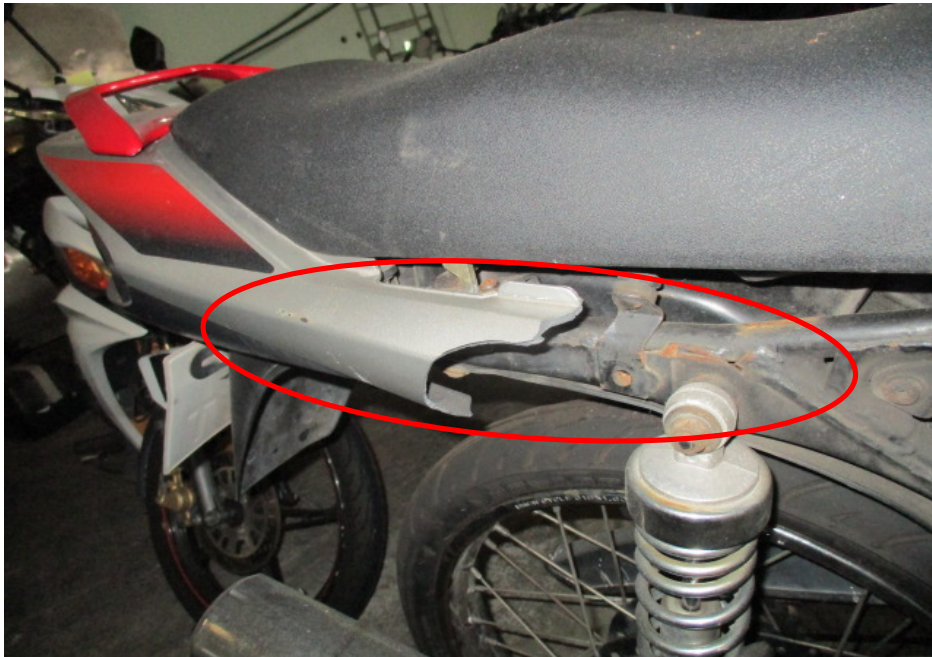
Photo 9 shows the damaged right rear side cover (circled) which was amongst the body parts of the Motorcycle that had sustained damage as a result of the accident.
