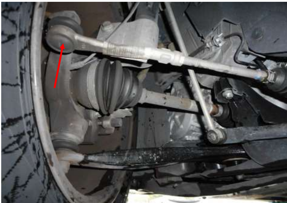
Photo 21 shows the various undercarriage components at the front left wheel of the Motor Car, which had included the steering tie rod (red arrow). The various undercarriage components of the Motor Car were all found to be intact without any visible damage.
