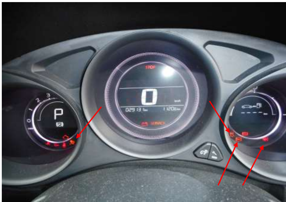
Photo 22 shows the warning light for Anti-Lock Brake System (ABS), Electric Power Steering System (EPS), Traction Control (TC) and Supplemental Restraint System (SRS) appearing on the instrument panel of the Motor Car during the self-test of its various electronic operating systems when its engine was cranked.
