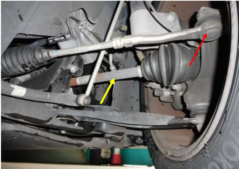
Photo 20 shows the various undercarriage components at the front right wheel of the Motor Car, in particular the steering tie rod (red arrow) and drive shaft (yellow arrow). The various steering components were all found to be intact, suggesting that the steering system of the Motor Car was likely to be in serviceable condition at the material time of accident. There was also no sign of fluid stain observed on the various undercarriage components at the front right wheel of the Motor Car.
