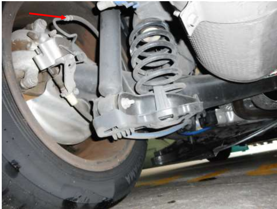
Photo 15 shows the brake hose/pipe (arrowed) at the rear left wheel of the Motor Car. I did not observe any leakage of brake fluid at the time of my inspection of the Motor Car. Static tests of the Motor Car's braking system had indicated that there was no internal leakage of pressure/vacuum. The undercarriage components of the Motor Car were also all found to be intact and without any visible damage.
