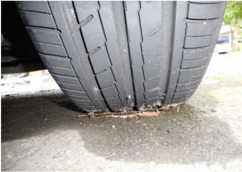
Photo 6 shows the condition of the front right tyre of the Motor Car, which was observed to be in serviceable condition with remaining tread depth of approximately 4.4mm. The tyre was sufficiently inflated for vehicular operation with no tear, cut or burst mark(s) on the outer and the inner sidewalls as well as across the tread. The 4 tyres of the Motor Car were wrapped around standard alloy wheel rims without any damage.
