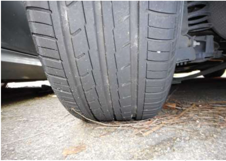
Photo 8 shows the condition of the rear left tyre of the Motor Car, which was observed to be in serviceable condition with remaining tread depth of approximately 6.5mm. The tyre, which was wrapped around alloy wheel rim, was also observed to be sufficiently inflated for vehicular operation. The 4 tyres of the Motor Car were wrapped around standard alloy wheel rims.
