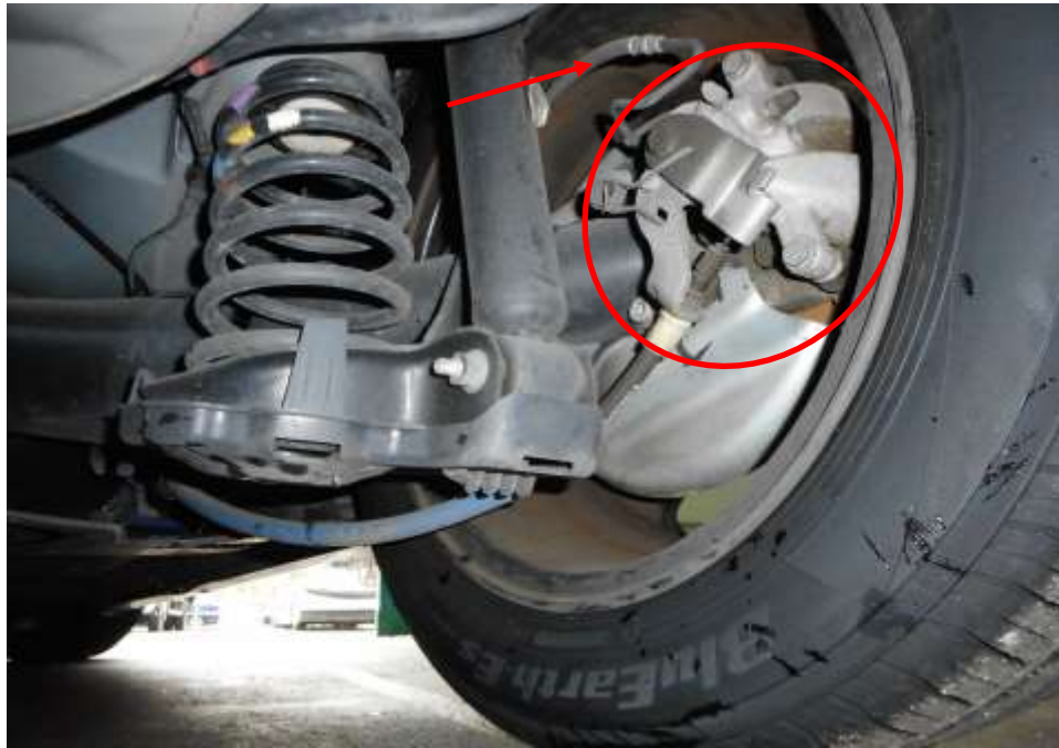
Photo 16 shows the brake hose/pipe (arrowed) at the rear right wheel of the Motor Car. No leakage of brake fluid was observed. Visual examination of the various components of the braking system like the brake caliper (circled), brake booster, brake pedal etc had revealed all to be intact and without visible damage.
