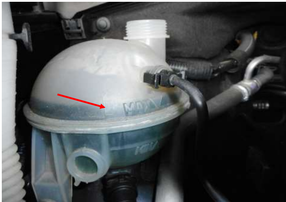
Photo 12 shows checks being carried out to the engine coolant of the Motor Car at the time of my inspection. The engine coolant was observed to be of sufficient level (arrowed) and without any visible contamination.
