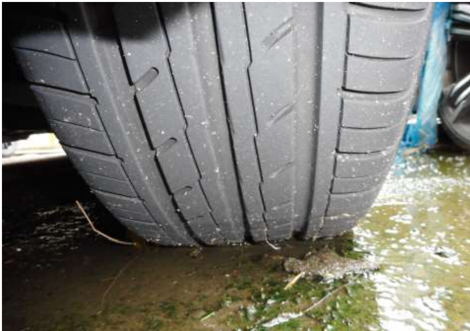
Photo 9 shows the condition of the rear right tyre of the Motor Car, which was observed to be in serviceable condition with remaining tread depth of approximately 6.7mm. There was also no tear, cut or burst mark(s) on the outer and the inner sidewalls as well as across the tread of the Motor Car's 4 tyres.
