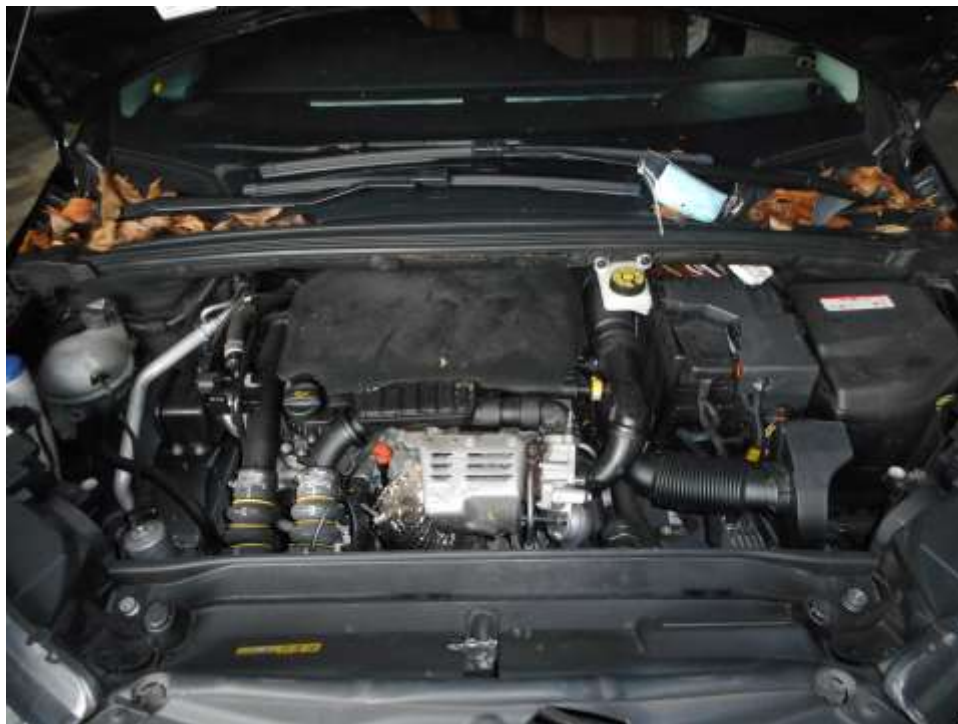
Photo 10 shows a general view of the Motor Car's engine compartment. The various parts and components inside the engine compartment were unaffected by the accident. There was also no sign(s) or indication(s) of fluid leakage and/or fluid stain within the engine compartment.
