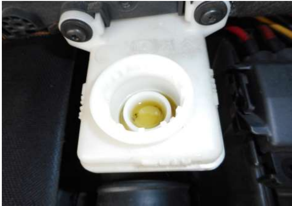
Photo 11 shows the brake fluid reservoir of the Motor Car at the time of my inspection. The brake fluid was observed to be of sufficient level and without any visible contamination.
