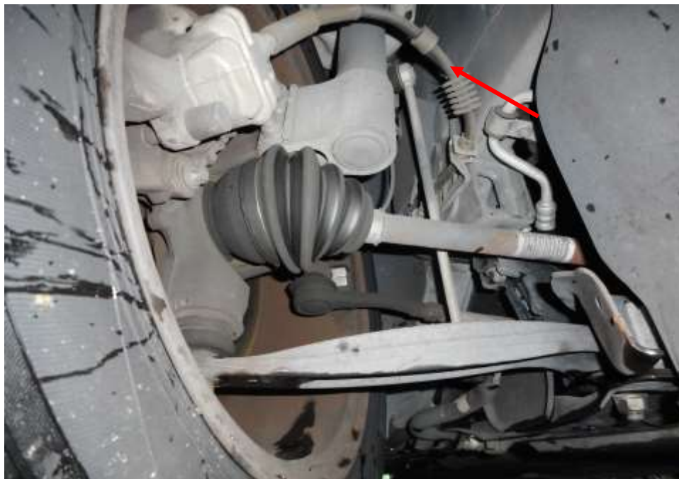
Photo 17 shows the brake hose/pipe (arrowed) at the front right wheel of the Motor Car. I did not observe any leakage of brake fluid at the time of my inspection of the Motor Car. Static tests of the Motor Car's braking system had indicated that there was no internal leakage of pressure/vacuum. The undercarriage components of the Motor Car were also all found to be intact and without any visible damage.
