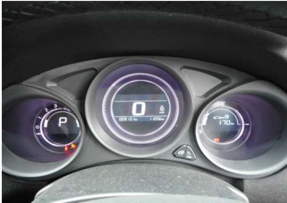
Photo 23 shows no warning lights illuminated on the instrument panel of the Motor Car after the engine was cranked. This would suggest that there was no abnormality to the various electronic operating systems of the Motor Car, like the ABS, EPS, TC and SRS etc.
