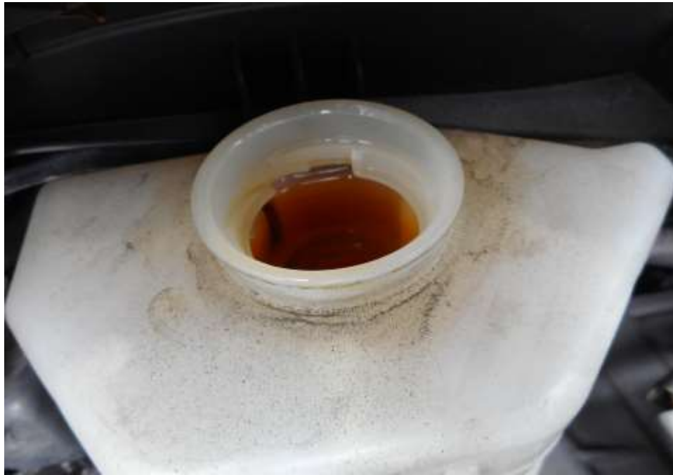
Photo 12 shows the brake fluid reservoir of the Motor Taxi at the time of my inspection. The brake fluid was observed to be of sufficient level and without any visible contamination.
