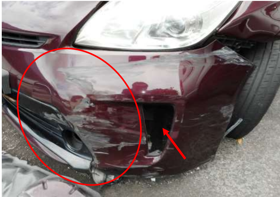
Photo 4 shows a close-up view of the front body of the Motor Taxi at the time of my inspection. The Motor Taxi was observed to have sustained relatively minor damage at its frontal portion. Its front bumper (circled) and fog lamp (arrowed) was damaged as a result of the accident.
