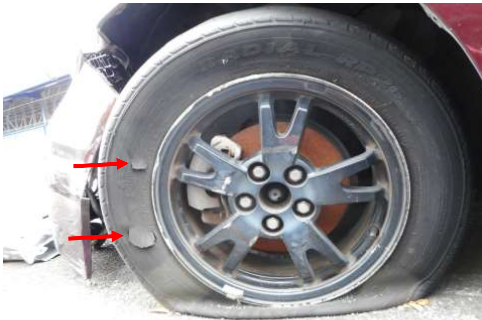
Photo 11 shows the condition of the front left tyre of the Motor Taxi, which was observed to have cut marks (arrowed) and delated as a result of the accident. The remaining tread depth of approximately 3.5mm.
