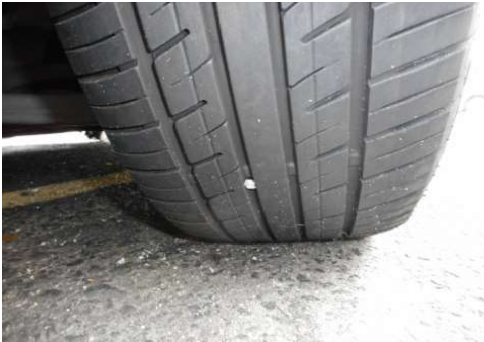
Photo 8 shows the condition of the front right tyre of the Motor Taxi, which was observed to be in serviceable condition with remaining tread depth of approximately 5.3mm. The tyre was sufficiently inflated for vehicular operation with no tear, cut or burst mark(s) on the outer and the inner sidewalls as well as across the tread. The 4 tyres of the Motor Taxi were wrapped around standard alloy wheel rims without any damage.
