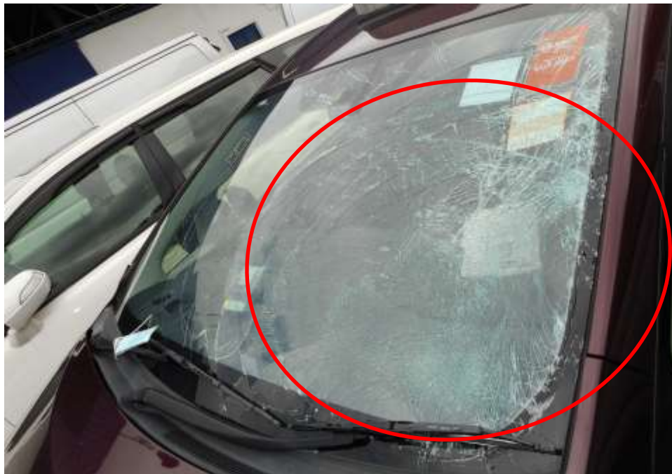
Photo 2 shows a close-up view of the damaged front windscreen (circled) of the Motor Taxi as a result of the accident.
