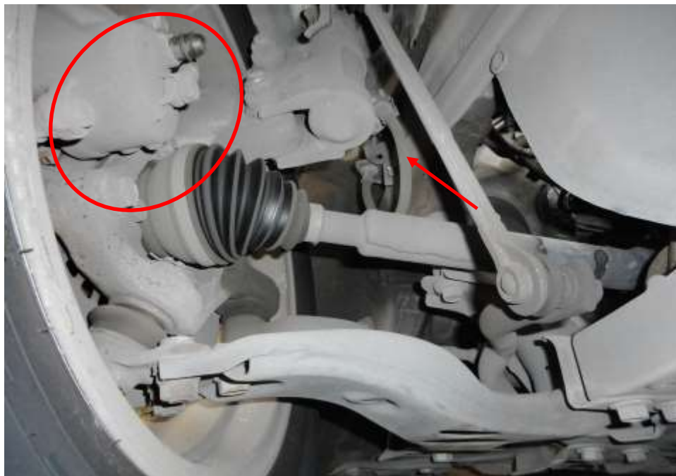
Photo 18 shows the brake hose/pipe (arrowed) at the front right wheel of the Motor Taxi. No leakage of brake fluid was observed. Visual examination of the various components of the braking system like the brake caliper (circled), brake booster, brake pedal etc had revealed all to be intact and without visible damage.
