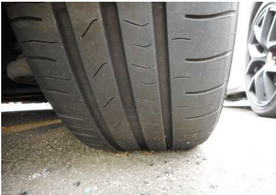
Photo 9 shows the condition of the rear right tyre of the Motor Taxi, which was observed to be in serviceable condition with remaining tread depth of approximately 5.5mm. The tyre was also observed to be sufficiently inflated for vehicular operation with no tear, cut or burst mark(s).
