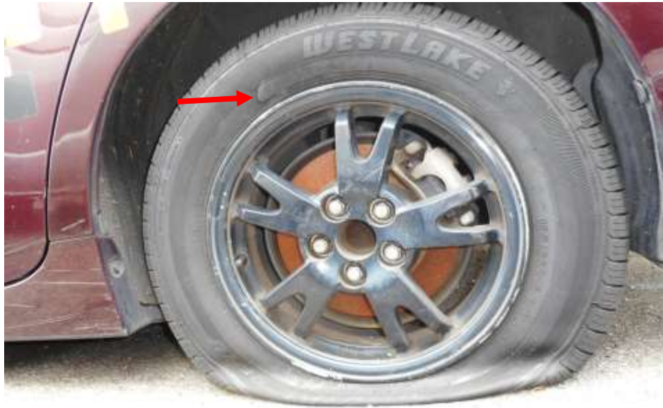
Photo 10 shows the condition of the rear left tyre of the Motor Taxi, which was observed to have cut marks (arrowed) and delated as a result of the accident. The remaining tread depth of approximately 6.5mm.
