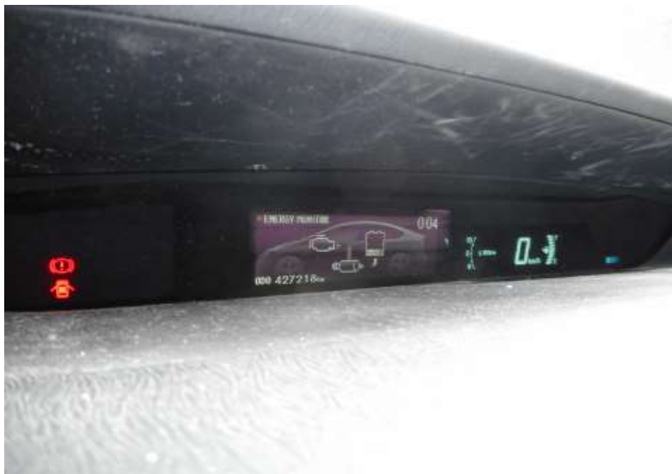
Photo 23 shows no warning lights illuminated on the instrument panel of the Motor Taxi after the engine was cranked. This would suggest that there was no abnormality to the various electronic operating systems of the Motor Taxi, like the ABS, EPS, TC and SRS etc.
