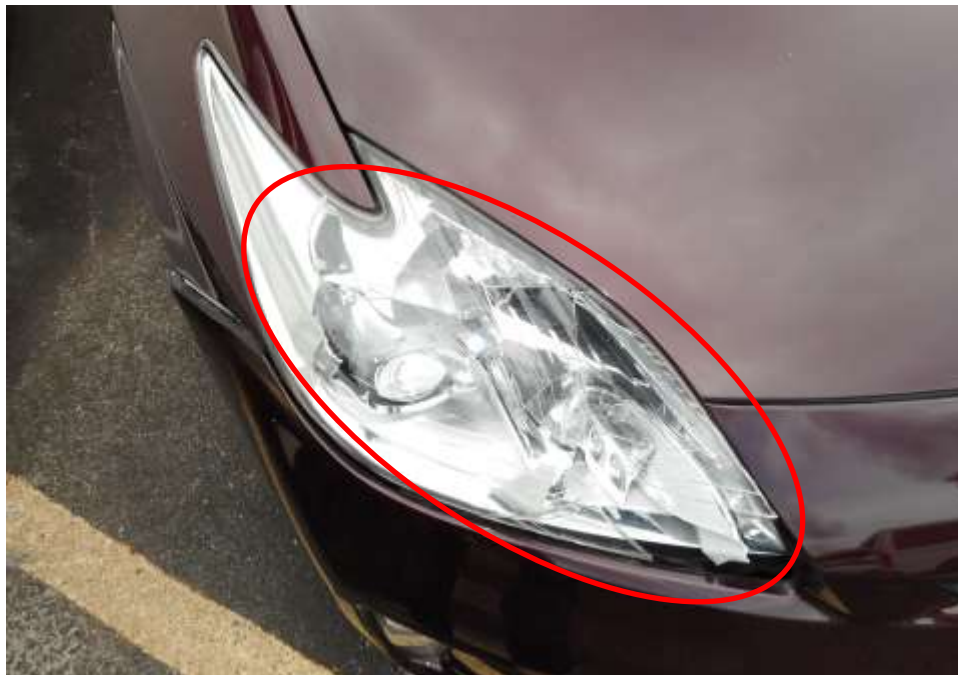
Photo 3 shows a close-up view of the Motor Taxi's right headlamp. Its front right headlamp (circled) was damaged as a result of the accident.
