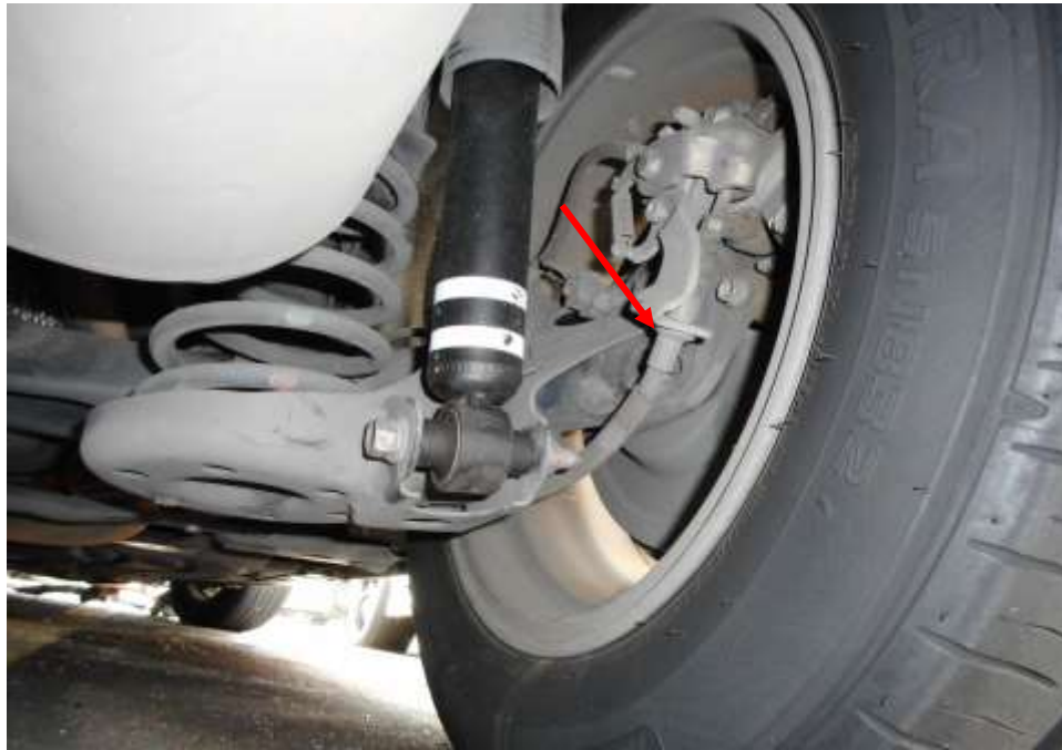
Photo 17 shows the brake hose/pipe (arrowed) at the rear right wheel of the Motor Taxi. I did not observe any leakage of brake fluid at the time of my inspection of the Motor Taxi. Static tests of the Motor Taxi's braking system had indicated that there was no internal leakage of pressure/vacuum. The undercarriage components of the Motor Taxi were also all found to be intact and without any visible damage.
