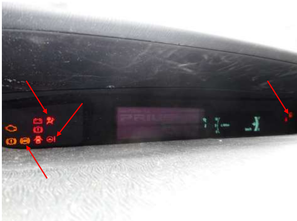
Photo 22 shows the warning light for Anti-Lock Brake System (ABS), Electric Power Steering System (EPS), Traction Control (TC) and Supplemental Restraint System (SRS) appearing on the instrument panel of the Motor Taxi during the self-test of its various electronic operating systems when its engine was cranked.
