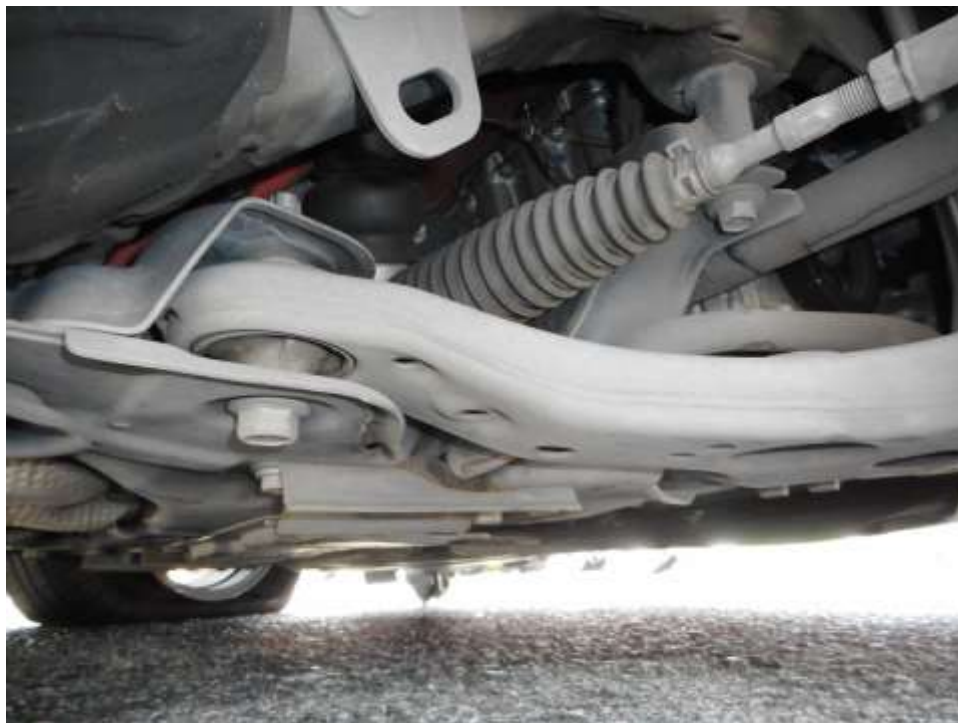
Photo 15 shows the undercarriage of the Motor Taxi, at the area where the engine housing and transmission housing are located. I did not find any sign(s) or indication(s) of fluid leak and/or fluid stain(s) on the underside of the Motor Taxi.
