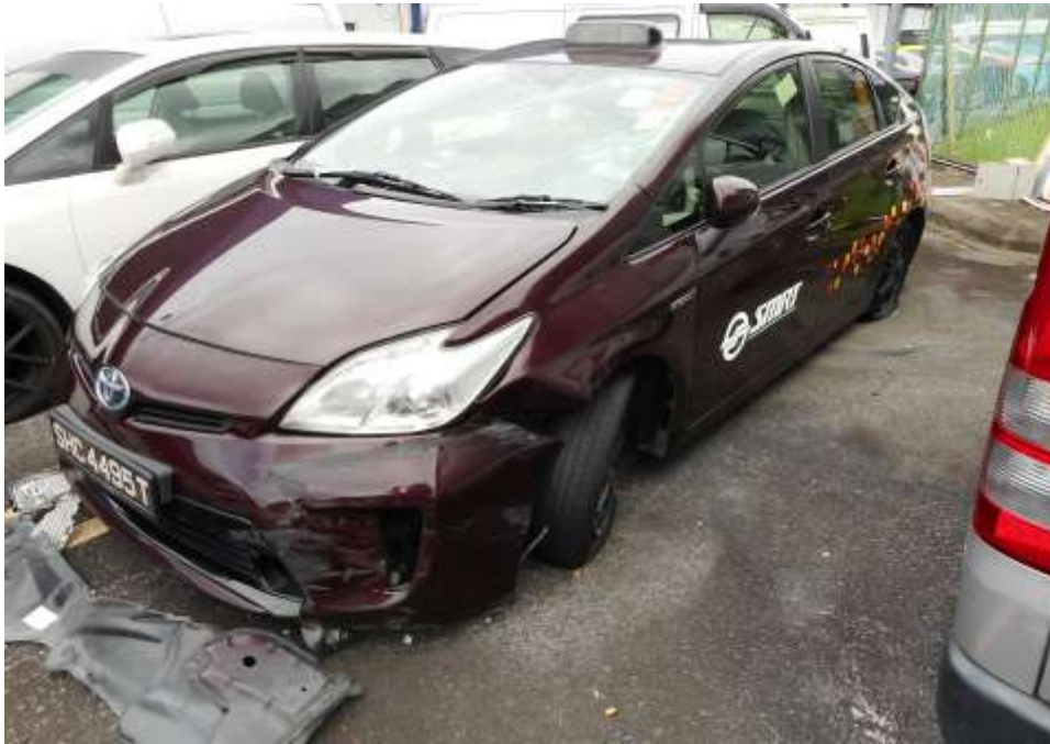
Photo 6 shows a general view of the Motor Taxi's left body panel at the time of my inspection. The left portion of the Motor Taxi was observed to have been unaffected by the accident.
