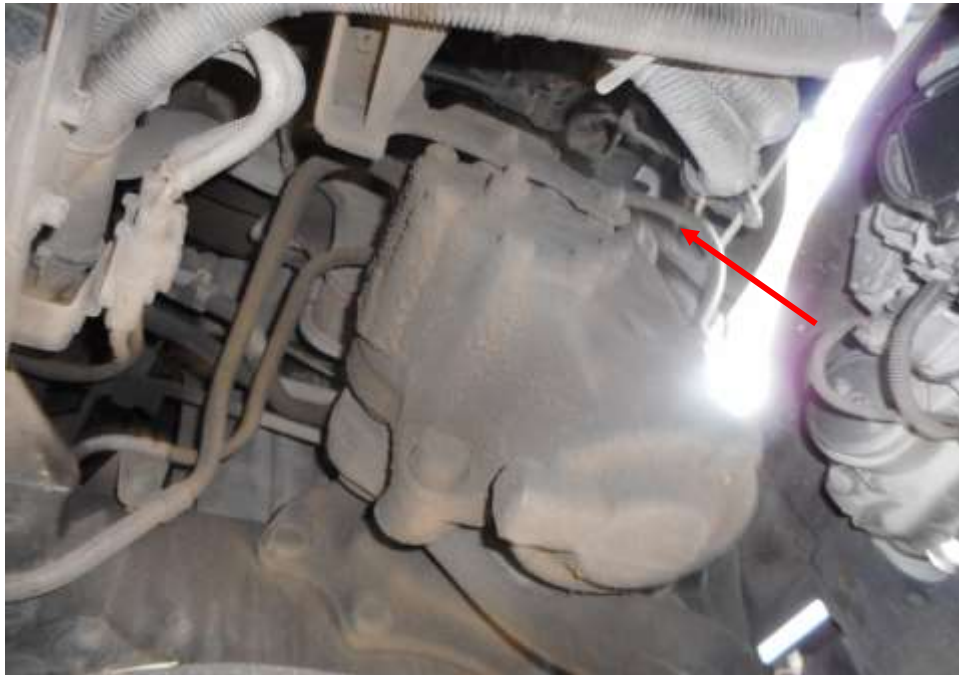
Photo 20 shows the steering box component (arrowed) at the undercarriage of the Motor Lorry was found to be intact without any visible damage. There was also no sign of fluid stain(s) observed on the various undercarriage components.
