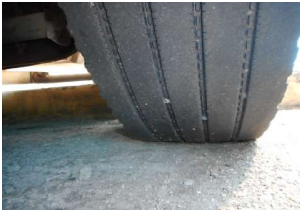
Photo 7 shows the condition of the front right tyre of the Motor Lorry, which was observed to be in serviceable condition with remaining tread depth of approximately 5 mm. The tyre, which was wrapped around standard steel wheel rim, was also observed to be sufficiently inflated for vehicular operation. There was no tear, cut or burst mark(s) on the outer and the inner sidewalls as well as across the tread of the 6 tyres that were fitted on the Motor Lorry.
