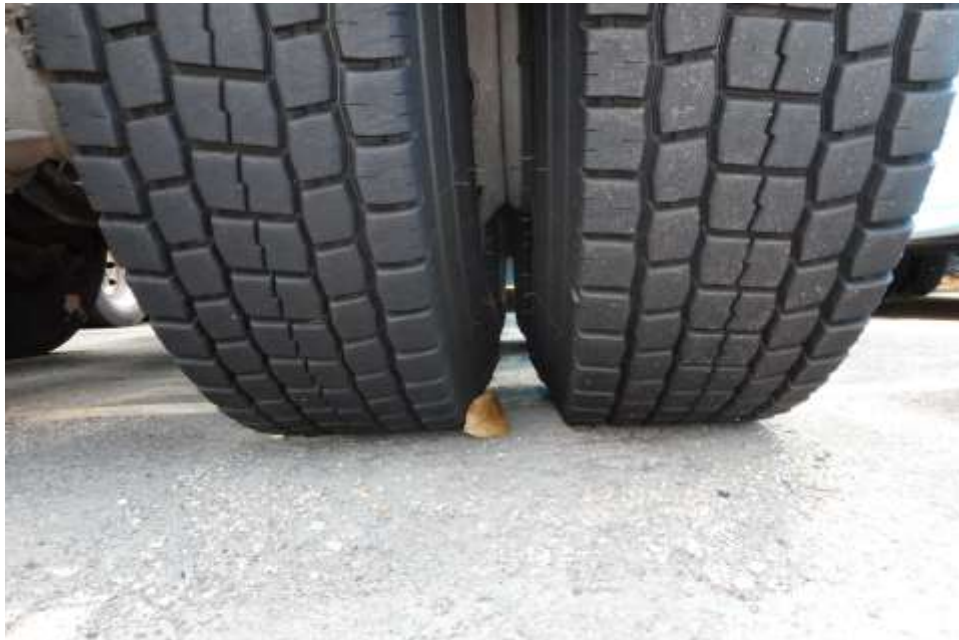
Photo 8 shows the condition of the rear right tyre of the Motor Lorry, which was observed to be in serviceable condition with remaining tread depth of approximately 10.6mm. The tyre, which was wrapped around standard steel wheel rim, was also observed to be sufficiently inflated for vehicular operation.
