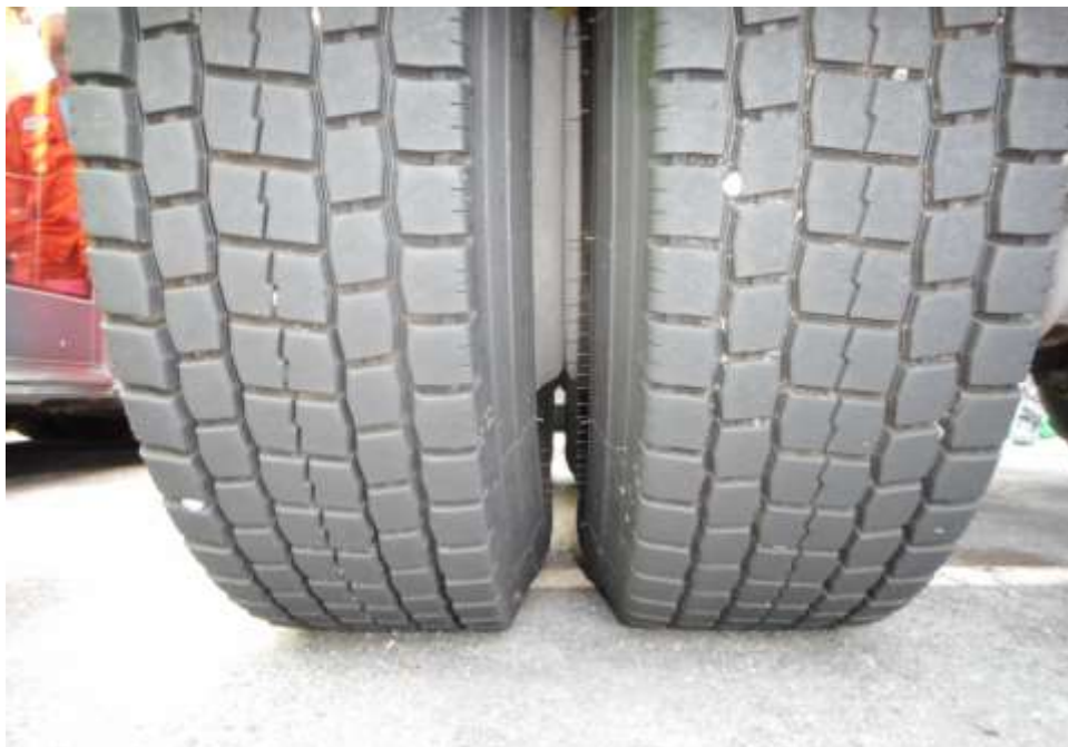
Photo 9 shows the condition of the rear left tyres of the Motor Lorry, which was observed to be in serviceable condition with remaining tread depth of approximately 10.3mm. The tyres, which were wrapped around standard steel wheel rim, were also observed to be sufficiently inflated for vehicular operation. There was also no damage found on all 6 steel wheel rims of the Motor Lorry.
