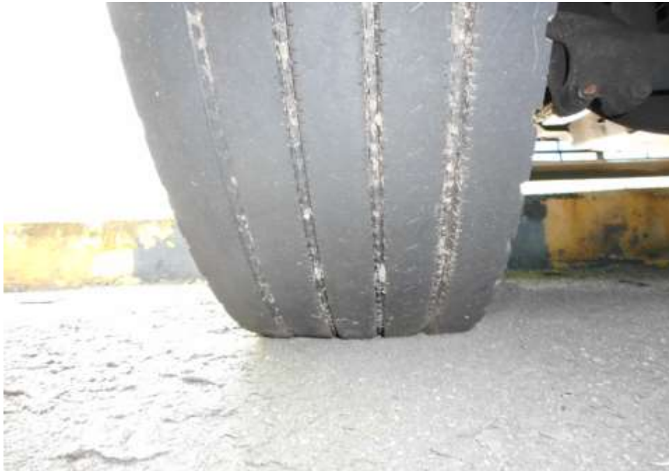
Photo 10 shows the condition of the front left tyres of the Motor Lorry, which were observed to be in serviceable condition with remaining tread depth of approximately 7.5mm. There was also no tear, cut or burst mark(s) on the outer and the inner sidewalls as well as across the tread of the 6 tyres that were fitted on the Motor Lorry.
