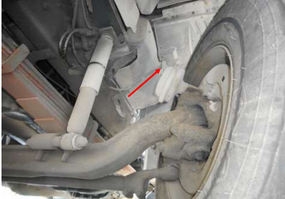
Photo 16 shows the brake pipe (arrowed) at the front left wheel of the Motor Lorry. I did not observe any leakage of brake fluid at the time of my inspection of the Motor Lorry. My static tests of the Motor Lorry's braking system, along with my visual examination of the various mechanical components in the braking system had indicated that there was no internal leakage of pressure/vacuum. Hence the braking system of the Motor Lorry was likely to be in serviceable condition at the material time of accident.
