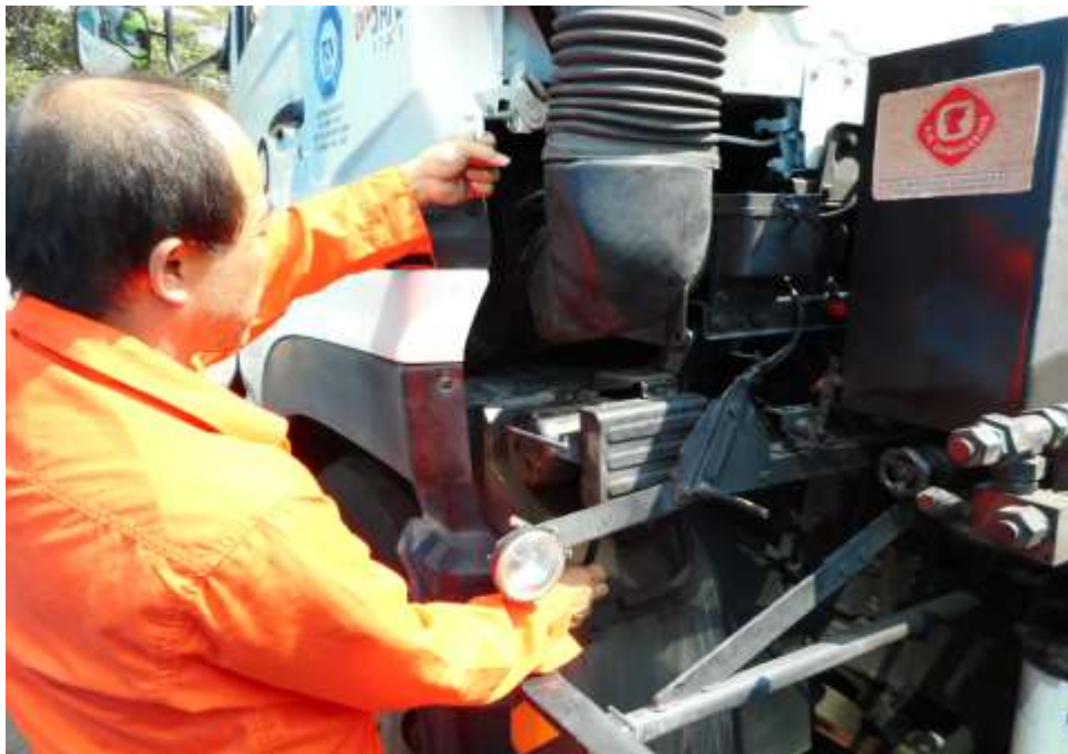
Photo 11 shows the mechanic attempting to operate the Motor Lorry's cabin lifter mechanism by the Motor Lorry. There was no movement to the cabin lifter despite multiple attempts to operate it. (Unable to operate)
