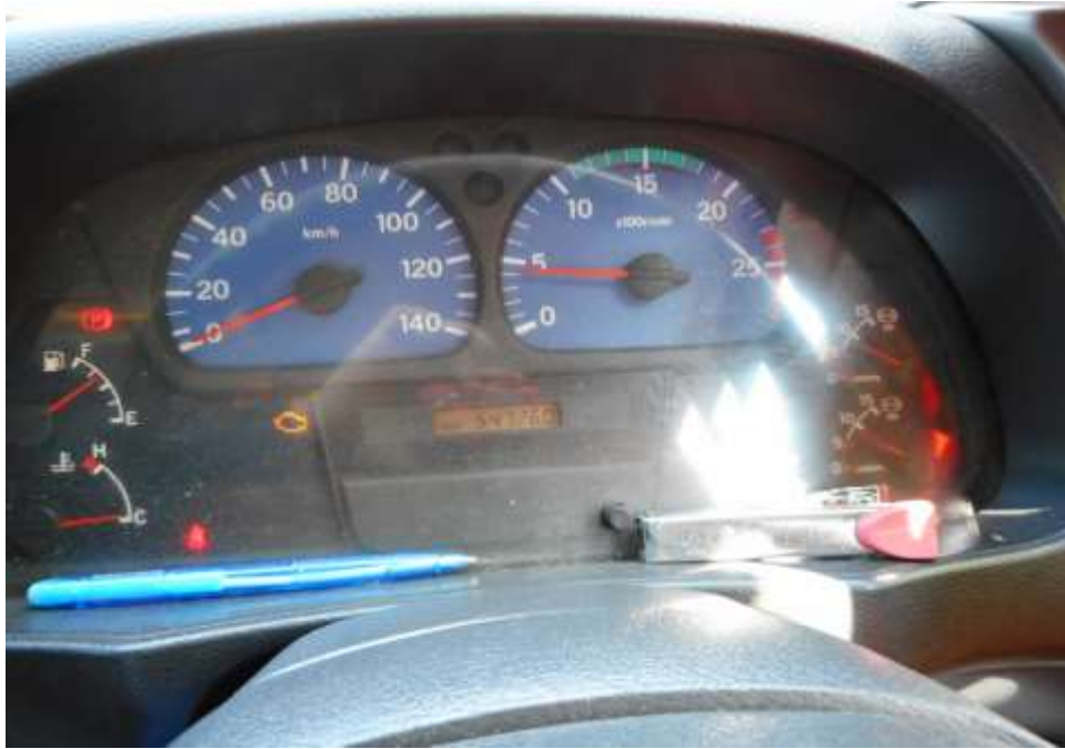
Photo 23 shows no warning lights illuminated on the instrument panel of the Motor Lorry after the engine was cranked. This would suggest that there was no abnormality to the various electronic operating systems of the Motor Lorry, like the ABS etc.
