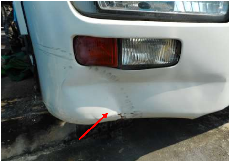
Photo 3 shows a close up view of the front body of the Motor Lorry at the time of my inspection. The Motor Lorry was observed to have sustained minor damage to its frontal portion; its front bumper was damaged (arrowed) as a result of the accident.
