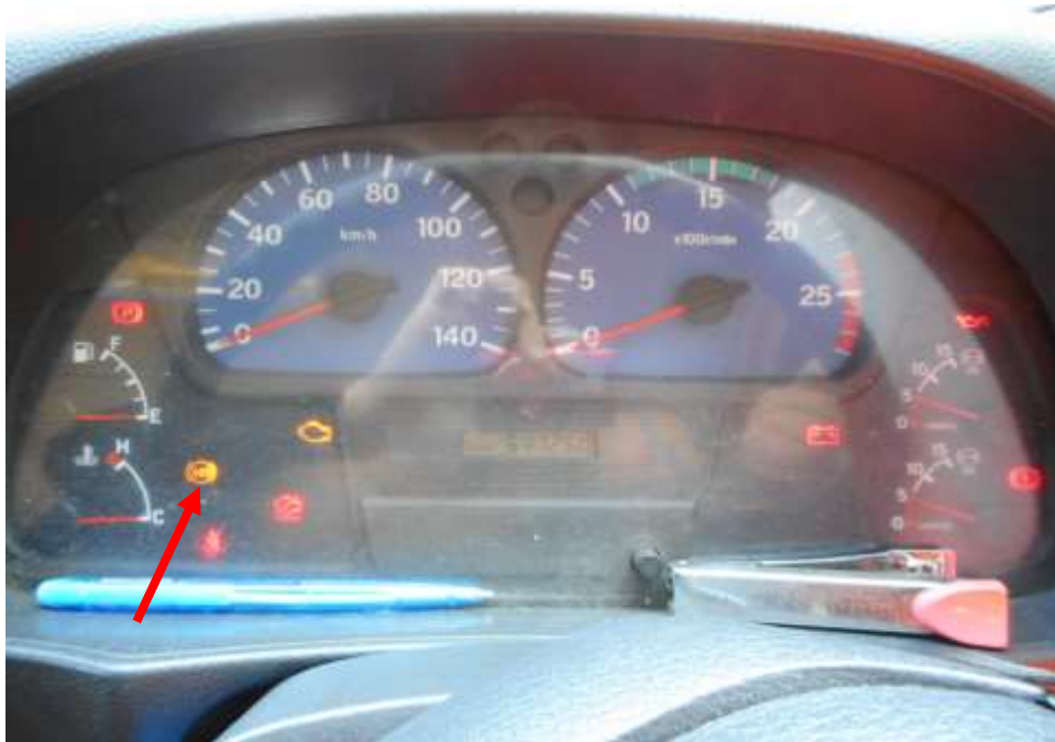
Photo 22 shows the warning light for Anti-Lock Brake System (ABS) (arrowed) appearing on the instrument panel of the Motor Lorry during the self-test of its various electronic operating systems when its engine was cranked.
