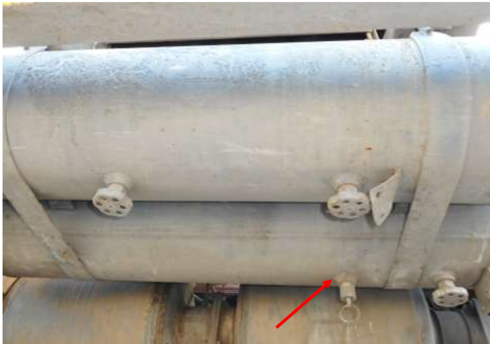
Photo 17 shows the air brake cylinder (arrowed) at the undercarriage of the Motor Lorry. I did not observe any leakage of air brake fluid at the time of my inspection of the Motor Lorry. My static tests of the Motor Lorry's braking system, along with my visual examination of the various mechanical components in the braking system had indicated that there was no internal leakage of pressure/vacuum. Hence the braking system of the Motor Lorry was likely to be in serviceable condition at the material time of accident.
