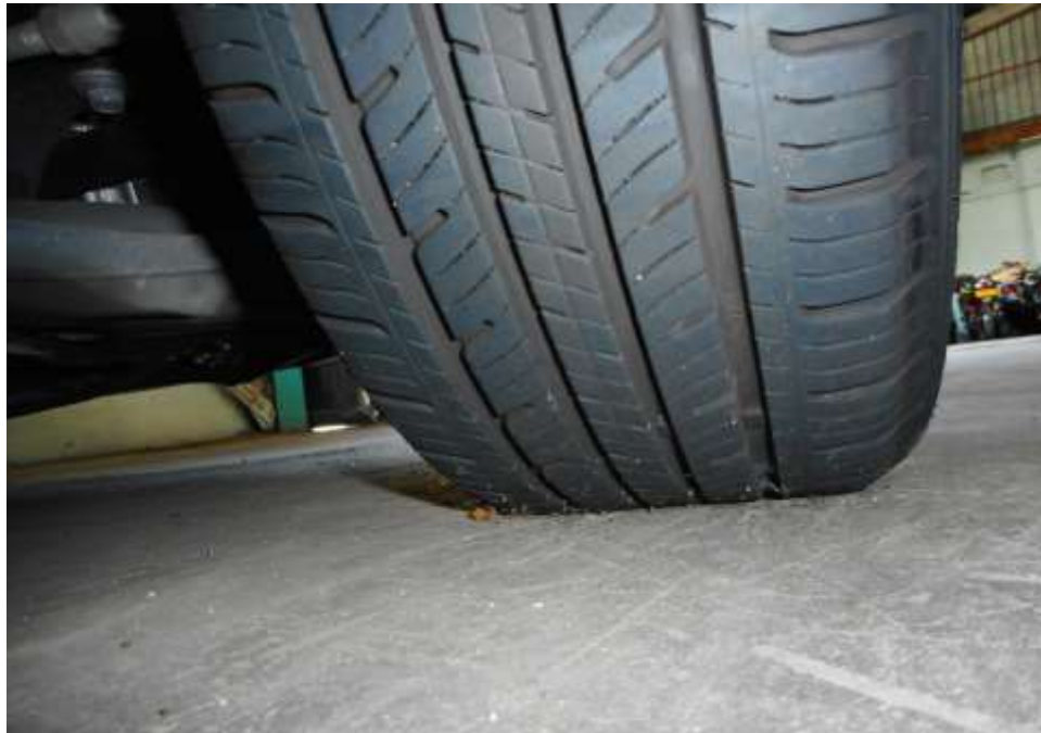
Photo 6 shows the condition of the front right tyre of the Motor Taxi, which was observed to be in serviceable condition with remaining tread depth of approximately 6.6mm. The tyre was sufficiently inflated for vehicular operation with no tear, cut or burst mark(s) on the outer and the inner sidewalls as well as across the tread. The 4 tyres of the Motor Taxi were wrapped around standard alloy wheel rims without any damage.
