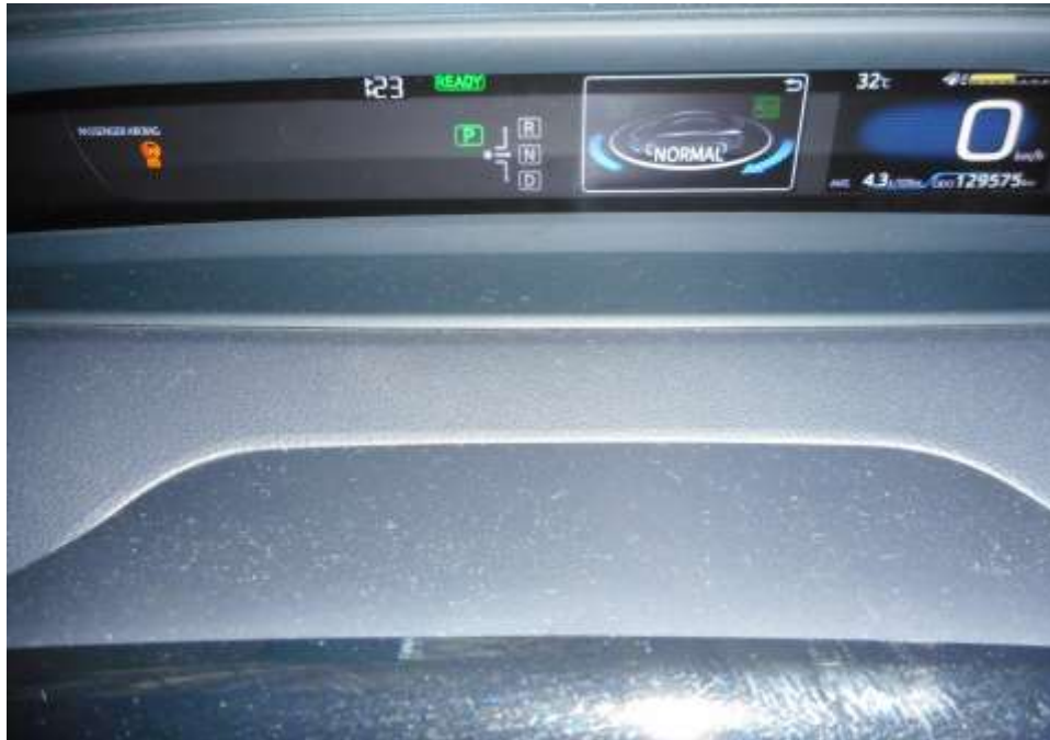
Photo 21 shows no warning lights illuminated on the instrument panel of the Motor Taxi after the engine was cranked. This would suggest that there was no abnormality to the various electronic operating systems of the Motor Taxi, like the ABS, EPS, TC and SRS etc.
