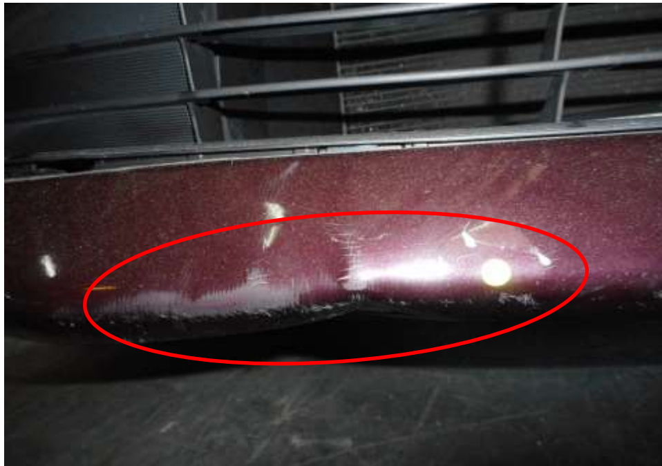
Photo 2 shows a close up view of the damaged front bumper (circled) of the Motor Taxi as a result of the accident
