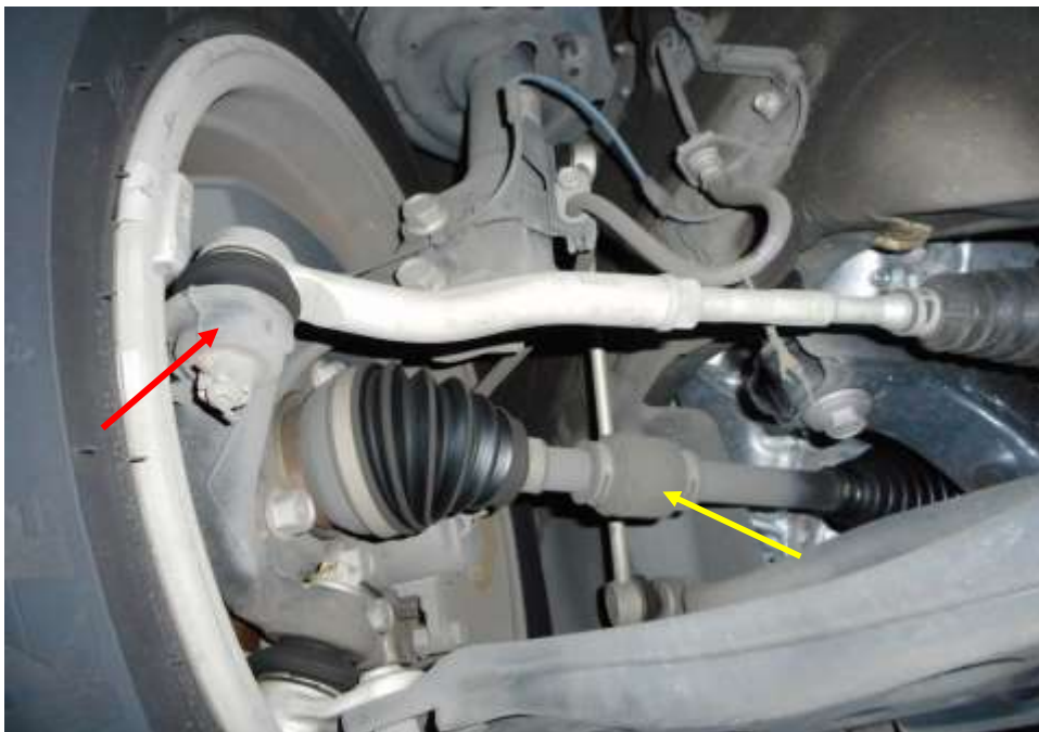
Photo 19 shows the various undercarriage components at the front left wheel of the Motor Taxi, which had included the steering tie rod (red arrow) and front left drive shaft (yellow arrow). The various undercarriage components of the Motor Taxi were all found to be intact without any visible damage.
