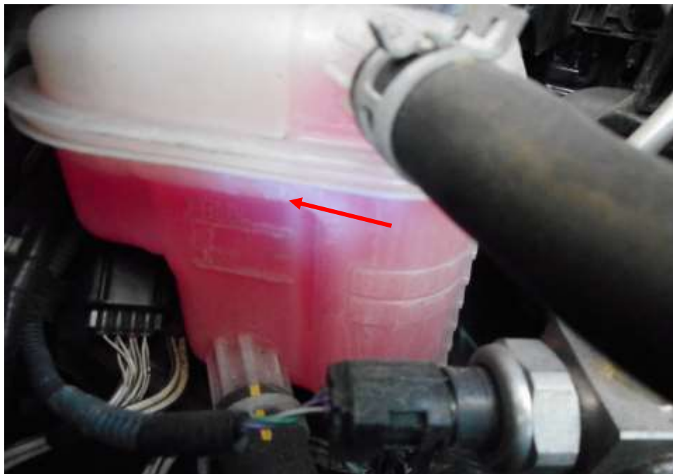
Photo 12 shows checks being carried out to the engine coolant of the Motor Taxi at the time of my inspection. The engine coolant was observed to be of sufficient level (arrowed) and without any visible contamination.
