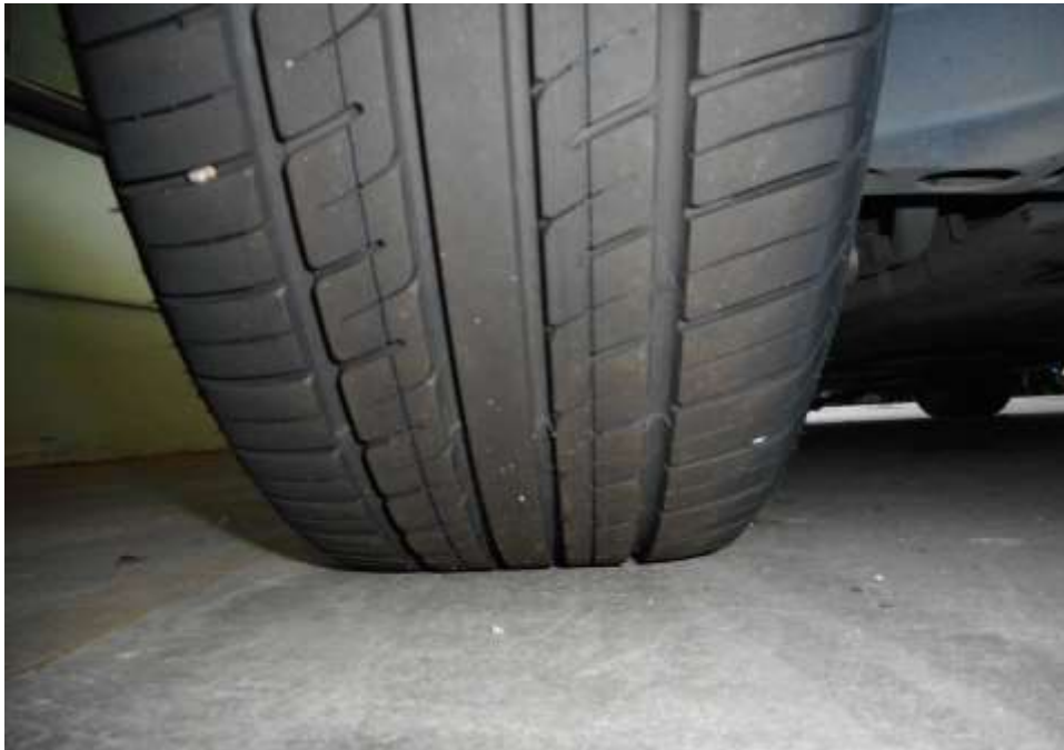
Photo 8 shows the condition of the rear left tyre of the Motor Taxi, which was observed to be in serviceable condition with remaining tread depth of approximately 6.3mm. The tyre, which was wrapped around alloy wheel rim, was also observed to be sufficiently inflated for vehicular operation. The 4 tyres of the Motor Taxi were wrapped around standard alloy wheel rims that were without any significant damage apart for some relatively minor kerb grazing type of damage on the outer side of the wheel rims
