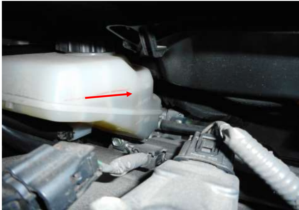
Photo 11 shows the brake fluid reservoir of the Motor Taxi at the time of my inspection. The brake fluid was observed to be of sufficient level (arrowed) and without any visible contamination.
