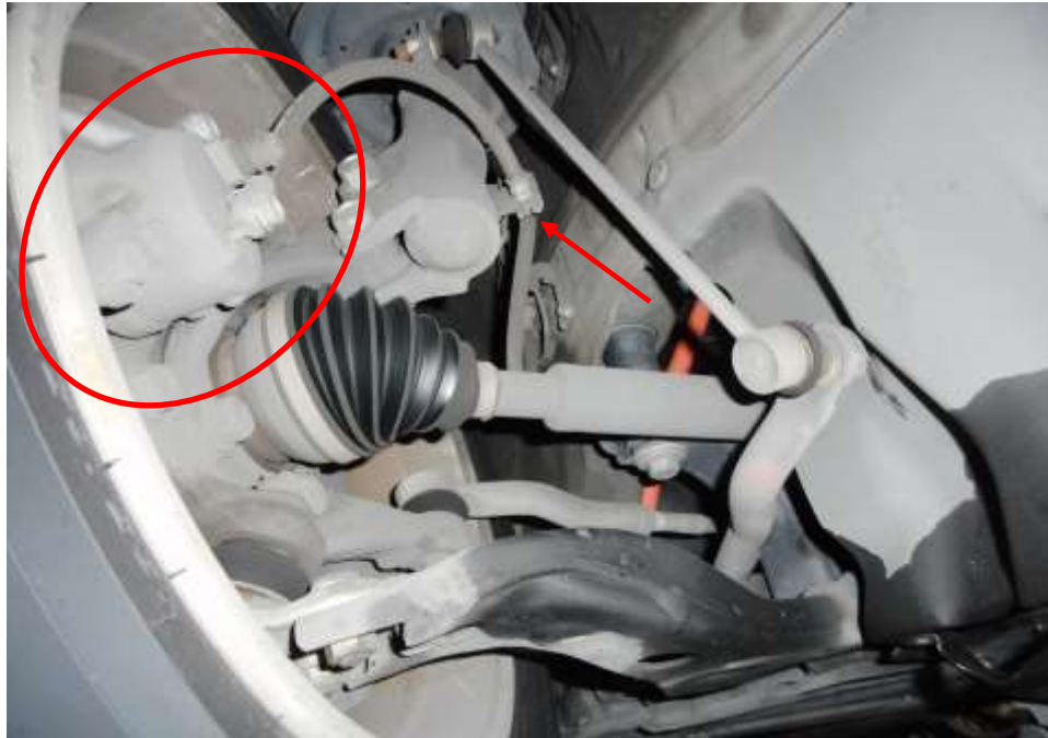
Photo 16 shows the brake hose/pipe (arrowed) at the front right wheel of the Motor Taxi. No leakage of brake fluid was observed. Visual examination of the various components of the braking system like the brake caliper (circled), brake booster, brake pedal etc had revealed all to be intact and without visible damage.
