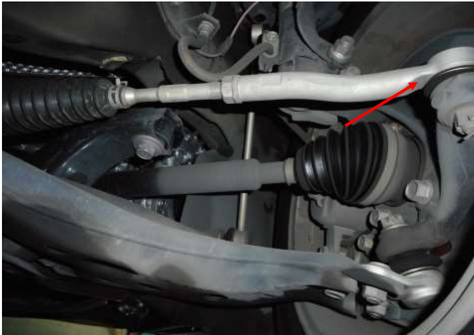
Photo 18 shows the various undercarriage components at the front right wheel of the Motor Taxi, in particular the steering tie rod (arrowed). The various steering components were all found to be intact, suggesting that the steering system of the Motor Taxi was likely to be in serviceable condition at the material time of accident. There was also no sign of fluid stain observed on the various undercarriage components at the front right wheel of the Motor Taxi.
