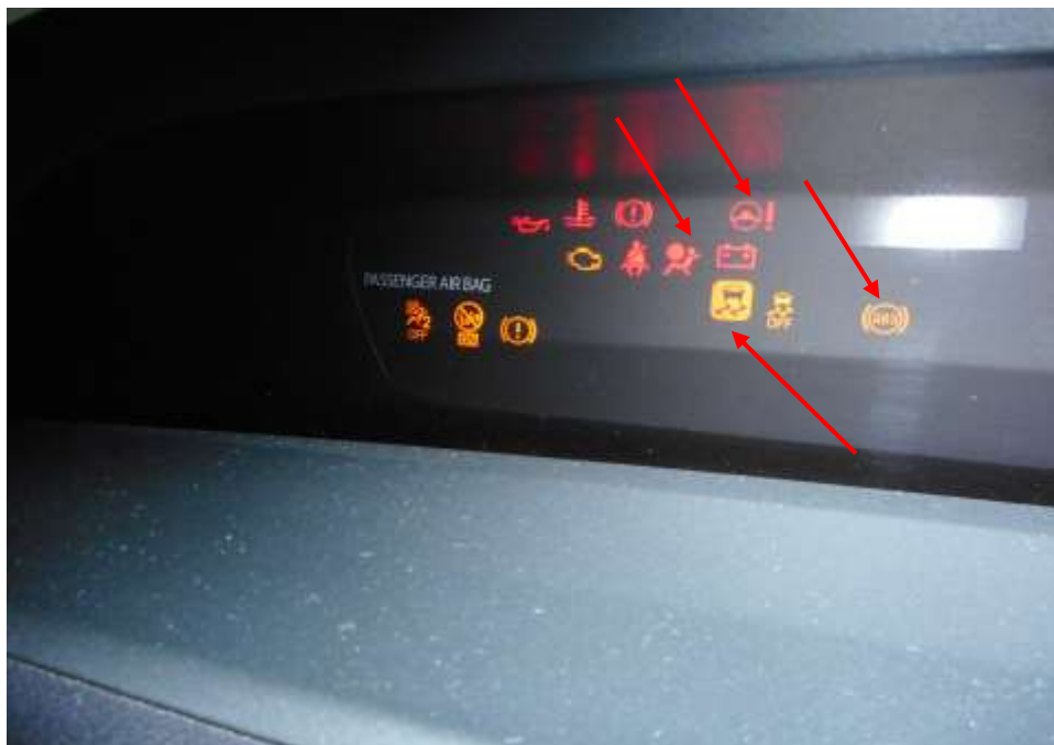
Photo 20 shows the warning light for Anti-Lock Brake System (ABS), Electric Power Steering System (EPS), Traction Control (TC) and Supplemental Restraint System (SRS) appearing on the instrument panel of the Motor Taxi during the self-test of its various electronic operating systems when its engine was cranked.
