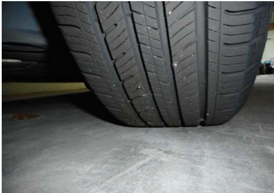
Photo 7 shows the condition of the rear right tyre of the Motor Taxi, which was observed to be in serviceable condition with remaining tread depth of approximately 6.7mm. The tyre was also observed to be sufficiently inflated for vehicular operation with no tear, cut or burst mark(s).
