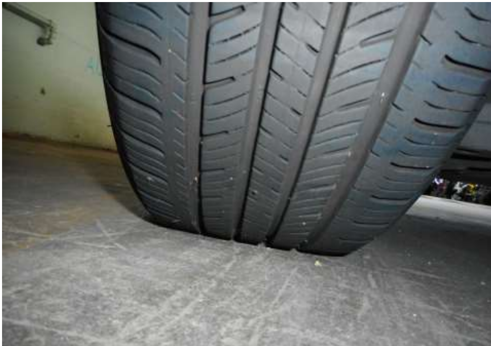
Photo 9 shows the condition of the front left tyre of the Motor Taxi, which was observed to be in serviceable condition with remaining tread depth of approximately 6.4mm. There was also no tear, cut or burst mark(s) on the outer and the inner sidewalls as well as across the tread of the Motor Taxi's 4 tyres.
