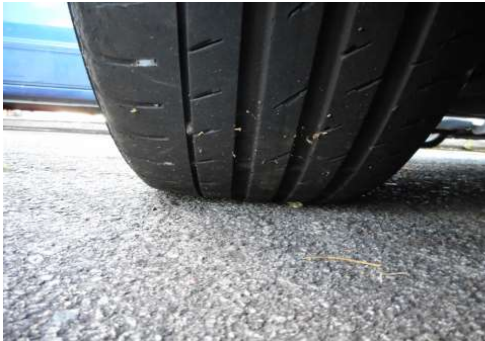
Photo 9 shows the condition of the rear right tyre of the Motor Car, which was observed to be in serviceable condition with remaining tread depth of approximately 4.4mm. There was also no tear, cut or burst mark(s) on the outer and the inner sidewalls as well as across the tread of the Motor Car's 4 tyres.
