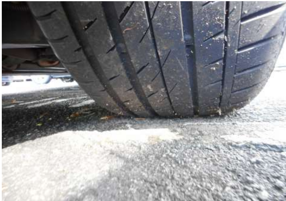
Photo 7 shows the condition of the rear right tyre of the Motor Car, which was observed to be in serviceable condition with remaining tread depth of approximately 6.1mm. The tyre was also observed to be sufficiently inflated for vehicular operation with no tear, cut or burst mark(s).
