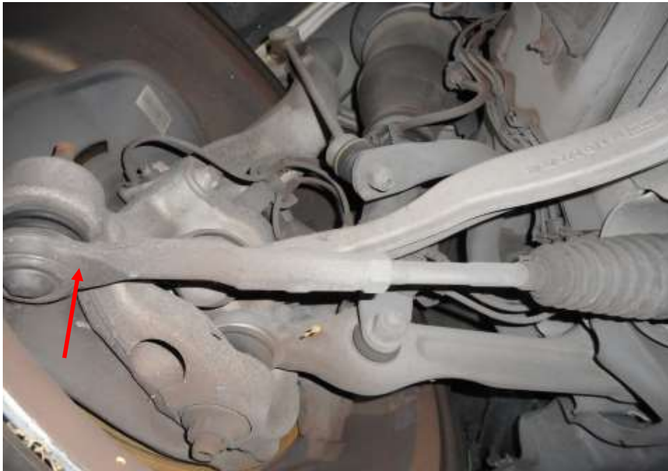
Photo 18 shows the various undercarriage components at the front right wheel of the Motor Car, in particular the steering tie rod (arrowed). The various steering components were all found to be intact, suggesting that the steering system of the Motor Car was likely to be in serviceable condition at the material time of accident. There was also no sign of fluid stain observed on the various undercarriage components at the front right wheel of the Motor Car.
