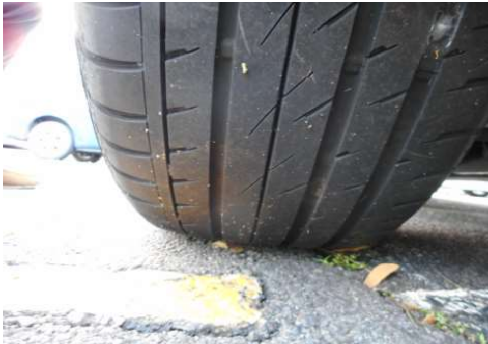
Photo 8 shows the condition of the rear left tyre of the Motor Car, which was observed to be in serviceable condition with remaining tread depth of approximately 6.3mm. The tyre, which was wrapped around alloy wheel rim, was also observed to be sufficiently inflated for vehicular operation. The 4 tyres of the Motor Car were wrapped around standard alloy wheel rims that were without any significant damage apart for some relatively minor kerb grazing type of damage on the outer side of the wheel rims
