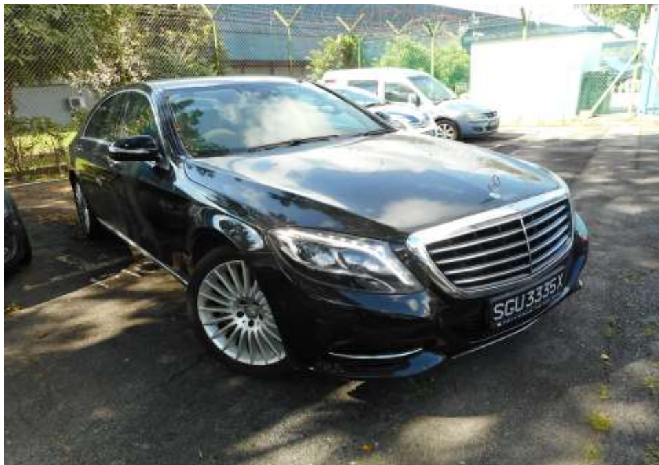
Photo 17 shows the front right wheel of the Motor Car turned to its full left. During my steering system test, I did not experience any abnormal free play and/or resistance when I had turned the steering wheel towards the left and right. This would suggest that the steering system of the Motor Car was likely to be in serviceable condition at the material time of accident.
