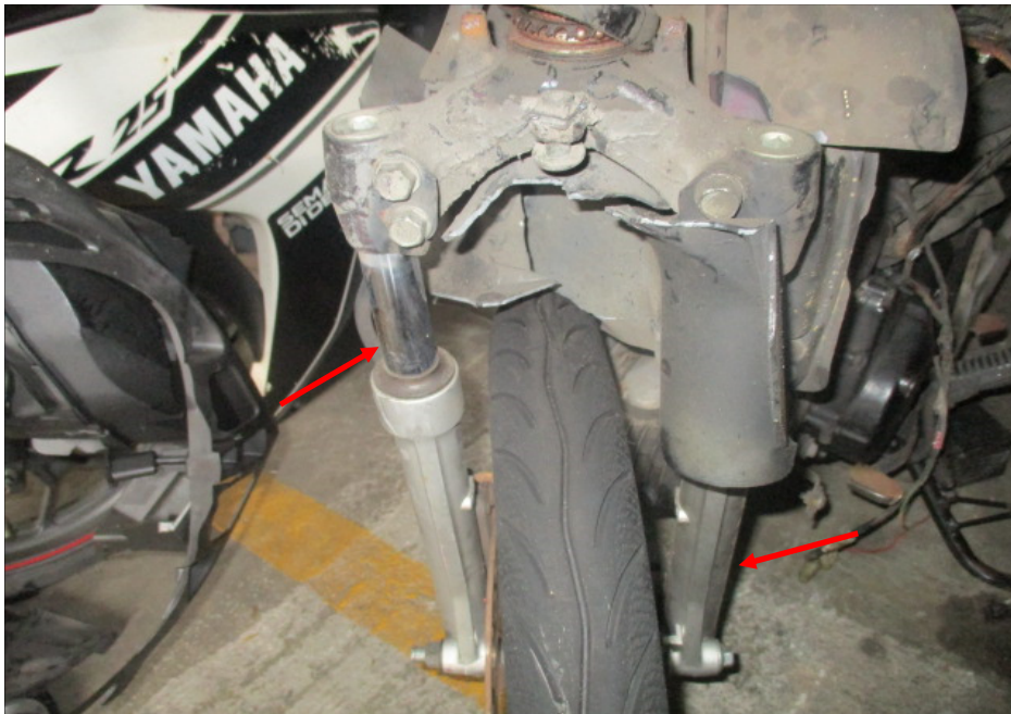
Photo 22 shows the front fork of the Motorcycle. The front fork (arrowed) was observed to be bent inwards as a result of the accident. We were hence not able to conduct any tests on the steering system of the Motorcycle.
