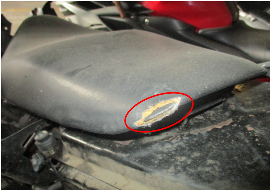
Photo 13 shows the seat of the Motorcycle which was observed to be torn as a result of the accident (circled).
