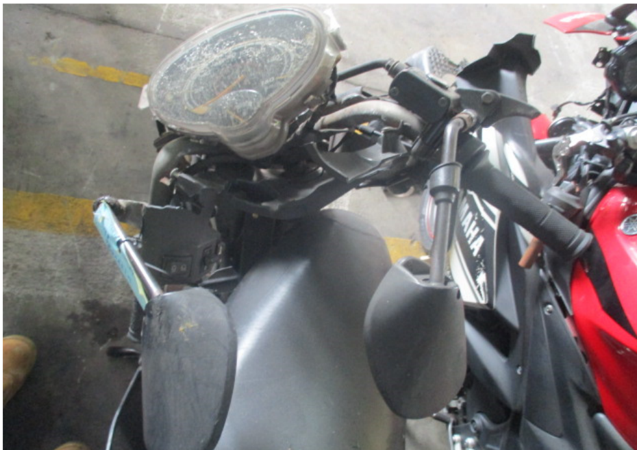
Photo 5 shows a closer view of the speedometer gauge, side mirrors and handlebars of the Motorcycle. These parts were amongst the body parts of the Motorcycle which were damaged as a result of the accident.
