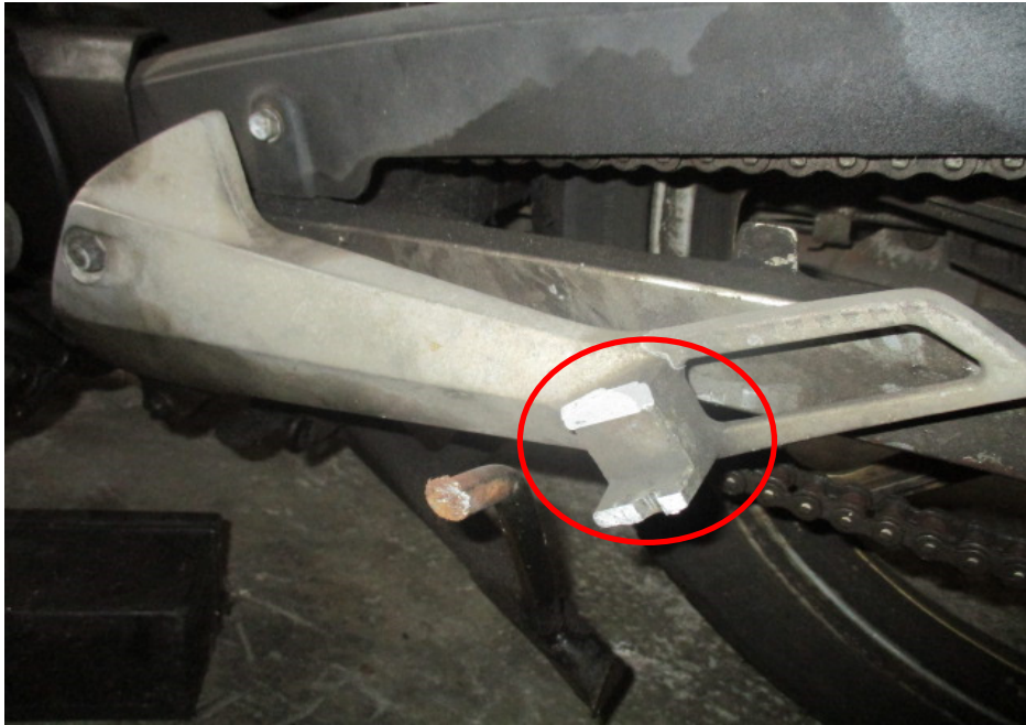
Photo 10 shows a closer view of the left pillion footrest bracket (circled), which was amongst the body parts of the Motorcycle that had sustained damage as a result of the accident.
