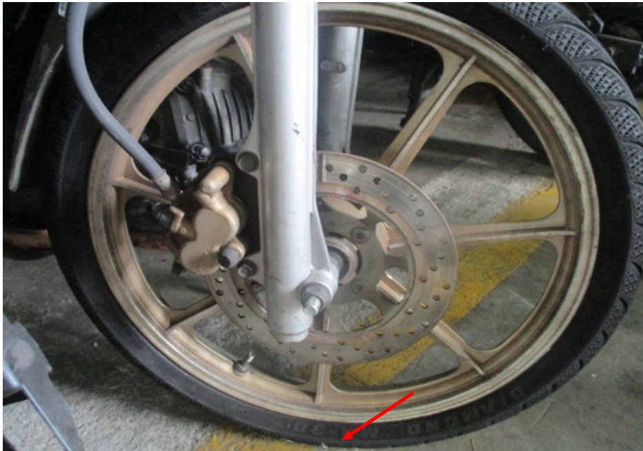
Photo 15 shows the front tyre of the Motorcycle at the time of our inspection. We observed that the front tyre was punctured (arrowed).
