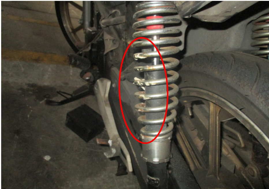
Photo 11 shows a close up view of the shock absorber on the left side of the Motorcycle which was amongst the body parts at the rear body of the Motorcycle damaged as a result of the accident (circled).
