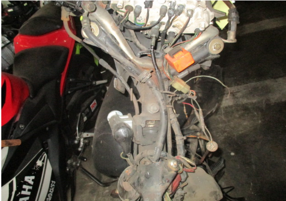
Photo 4 shows a closer view of the headlamp assembly of the Motorcycle. These parts were amongst the body parts of the Motorcycle which were damaged as a result of the accident.
