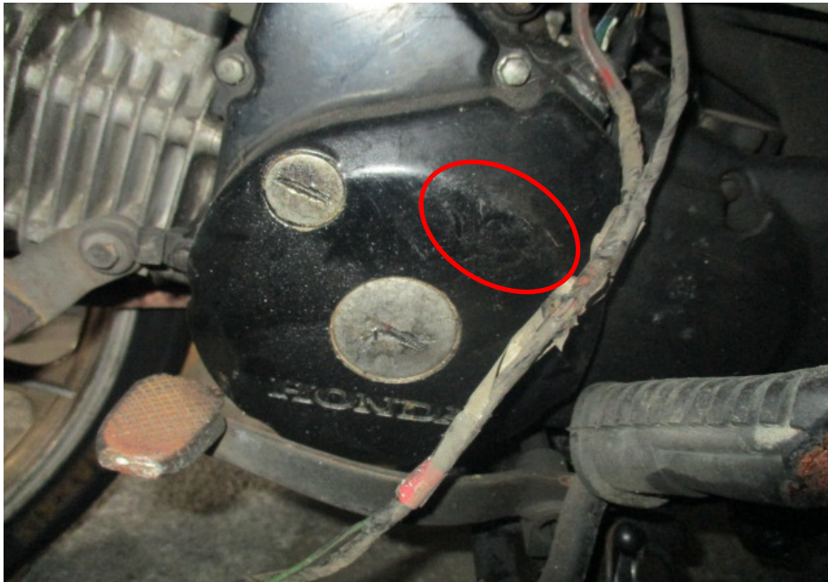
Photo 19 shows the left side of the engine of the Motorcycle at the time of our inspection. The various left engine components had sustained damage of grazing nature as a result of the accident (circled) however the engine components were still intact. There was also no fluid leak and/or fluid stain found around the left engine area of the Motorcycle.
