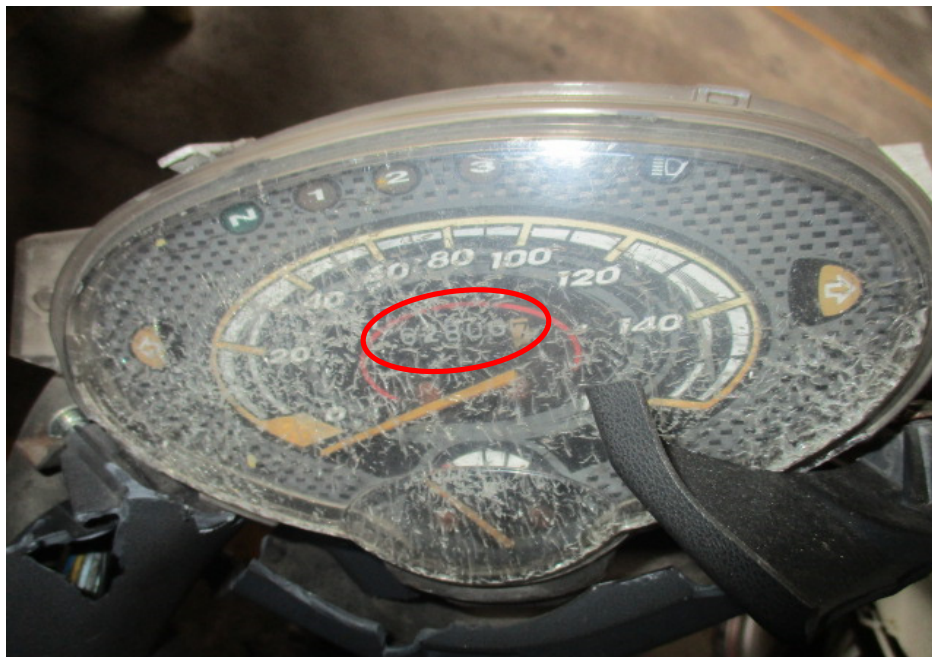
Photo 1 shows a closer view of the speedometer gauge of the Motorcycle which was damaged as a result of the accident. The mileage of the Motorcycle at the time of our inspection was 62, 800 (circled).
