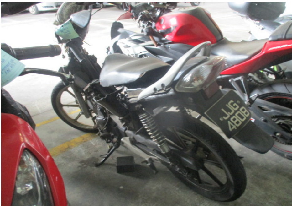
Photo 3 shows a general view of the left rear body of the Motorcycle at the time of our inspection. Body parts that were found to have been damaged include its front fork assembly, headlight assembly, speedometer gauge, front mudguard, front wheel rim, side mirrors, front brake lever, handlebars, left side cowling, left front footrest, left pillion footrest bracket, left pillion grab rail and seat, amongst others.
