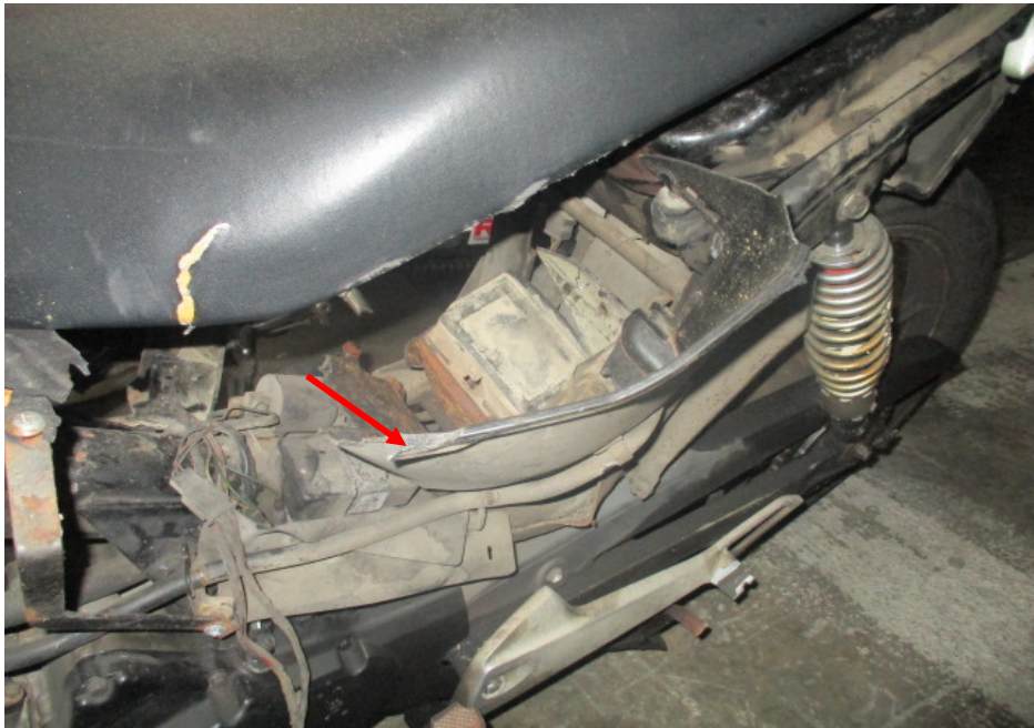
Photo 7 shows the left side cowling (arrowed) which was amongst the body parts of the Motorcycle damaged as a result of the accident.
