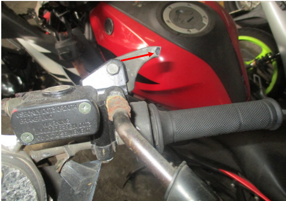
Photo 8 shows a close up view of the broken front brake lever (arrowed) of the Motorcycle which was amongst the body parts of the Motorcycle damaged as a result of the accident.
