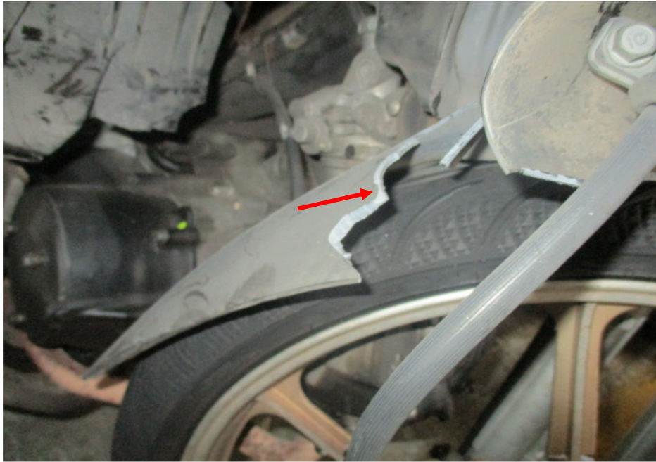
Photo 6 shows a close up view of the broken front mudguard (arrowed) of the Motorcycle which was amongst the body parts at the front body of the Motorcycle that had sustained damage as a result of the accident.
