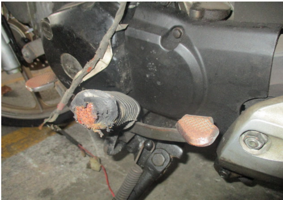
Photo 9 shows the damaged gear shift pedal, left front footrest and left front footrest bracket, which were amongst the body parts of the Motorcycle that had sustained damage as a result of the accident.
