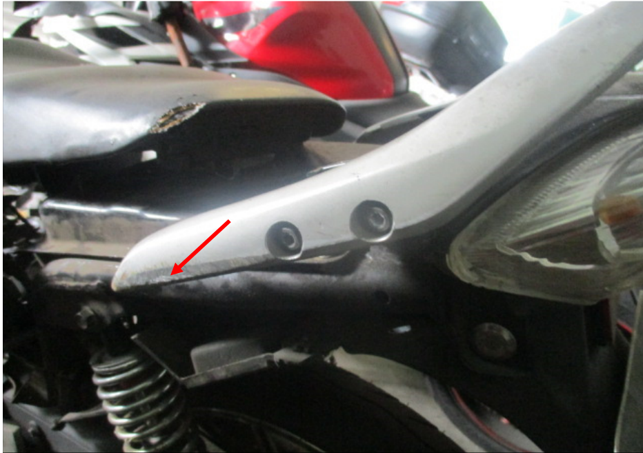
Photo 12 shows a closer view of the pillion grab rail of the Motorcycle which sustained damages of grazing nature (arrowed) as a result of the accident.
