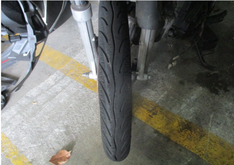
Photo 16 shows the condition of the Motorcycle's front tyre. The front tyre was observed to be in serviceable condition with remaining tread depth of approximately 3mm. The tyre was observed to be punctured. However we did not observe any tear and/or burst mark(s) on the sidewalls as well as across the tread of the front tyre.
