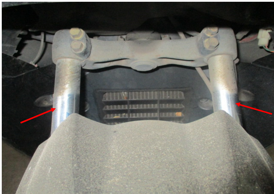
Photo 18 shows the front forks (arrowed) of the Motorcycle. The front forks and fork brackets of the Motorcycle were both found to be intact and undamaged. Turning the Motorcycle's handle bar towards the left and right did not produce any abnormal free play and/or resistance. The steering system of the Motorcycle was in serviceable condition at the time of our inspection.
