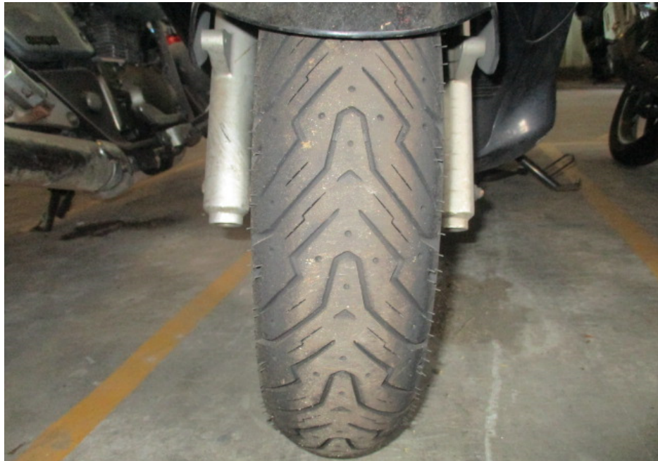
Photo 12 shows the condition of the Motorcycle's front tyre. The front tyre was observed to be in serviceable condition with remaining tread depth of approximately 3mm. There was no tear, burst mark(s) and/or punctured hole(s) on the sidewalls as well as across the tread of the front tyre.
