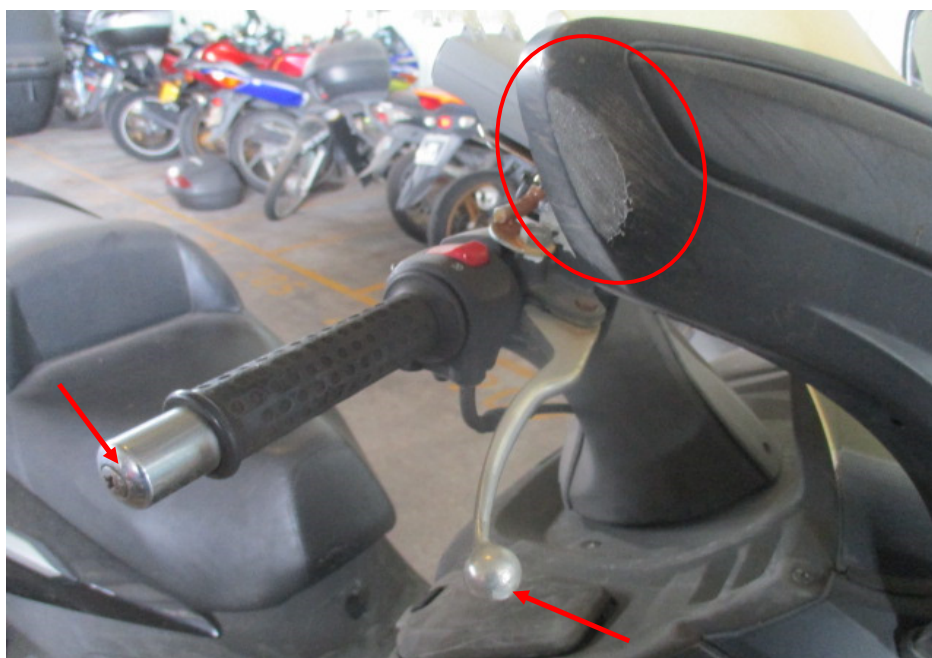
Photo 5 shows a closer view of the front brake lever and right handlebar end (arrowed) as well as the right side mirror (circled) of the Motorcycle which were observed to be damaged due to the accident
