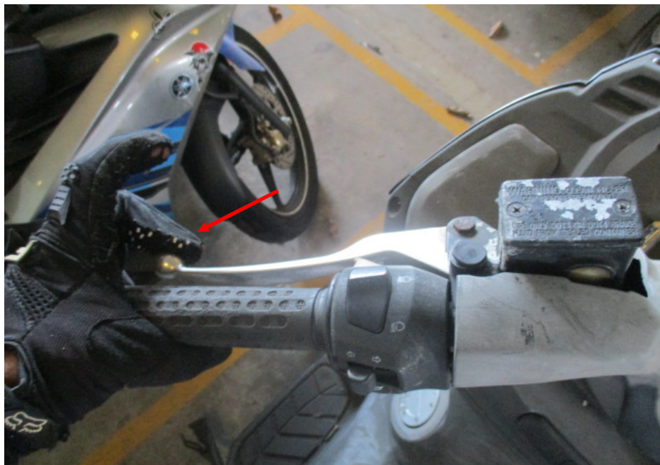
Photo 22 shows the rear brake lever being depressed. There was some resistance felt (spongy like feel) upon pressing the rear brake lever (arrowed). This would indicate that there is no leakage of pressure/vacuum in the brake system.
