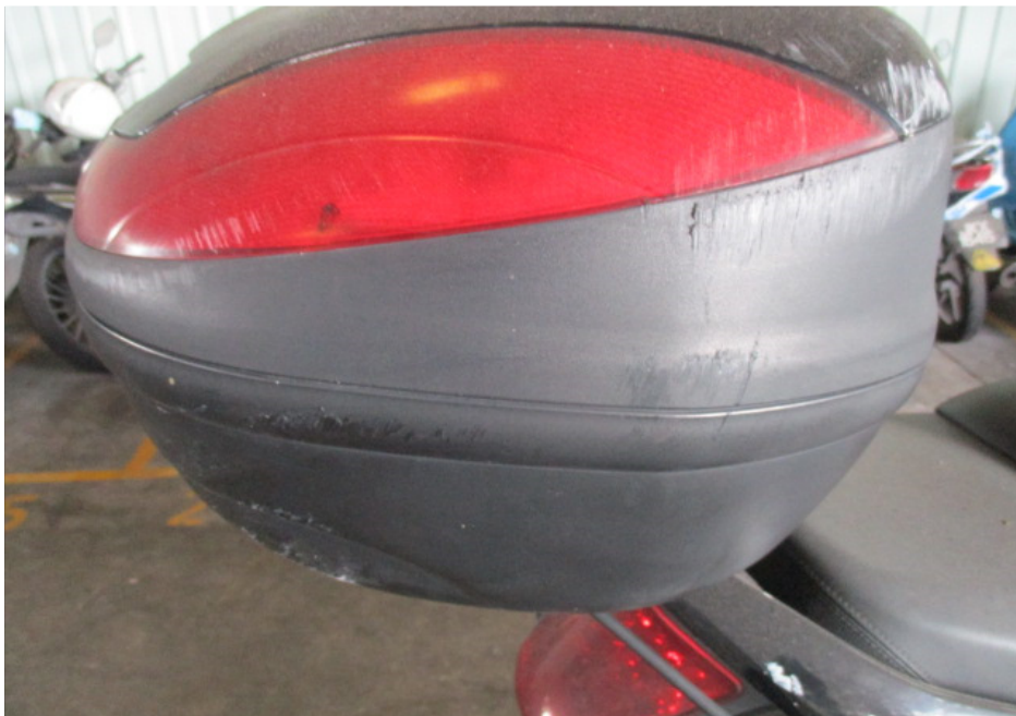
Photo 11 shows a closer view of the top box of the Motorcycle which was observed to have sustained scratches due to the accident.
