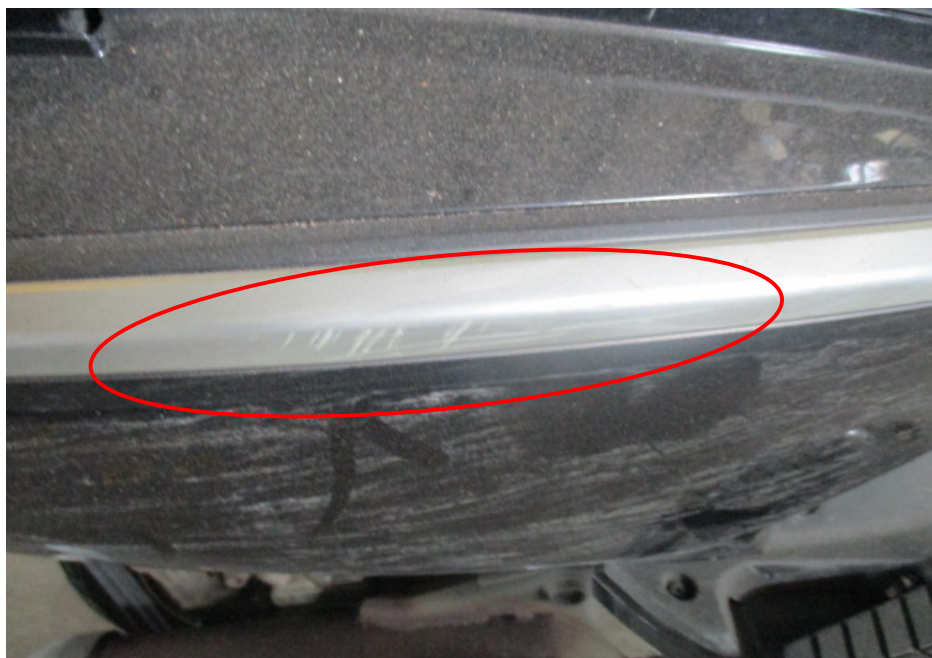
Photo 10 shows a closer view of the damaged right rear side cover of the Motorcycle which was observed to have sustained scratches due to the accident (circled).
