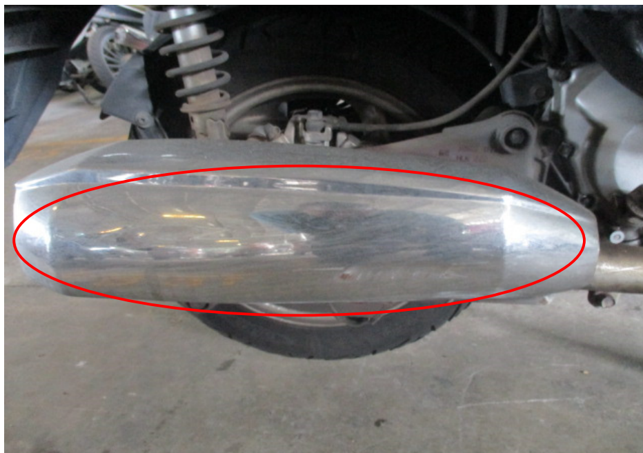
Photo 9 shows a closer view of the exhaust muffler of the Motorcycle which had sustained damage due to the accident (circled).
