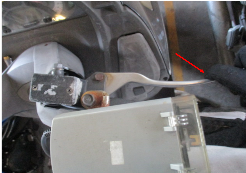
Photo 23 shows the front brake lever being depressed. There was some resistance felt (spongy like feel) upon pressing the front brake lever (arrowed). This would indicate that there is no leakage of pressure/vacuum in the brake system.
