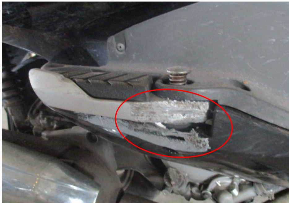
Photo 8 shows a closer view of the damaged right pillion footrest (circled) of the Motorcycle at the time of our inspection.
