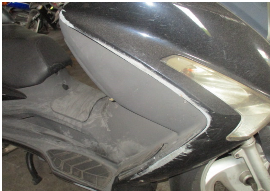
Photo 6 shows a closer view of the right cowling which was amongst the body parts at the front body of the Motorcycle that had sustained damage as a result of the accident.
