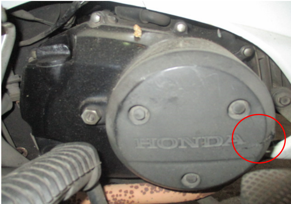
Photo 14 shows the right side of the engine of the Motorcycle at the time of our inspection. The outer engine cover had sustained a crack as a result of the accident (circled) however the engine components were still intact. There was also no fluid leak and/or fluid stain found around the right engine area of the Motorcycle.
