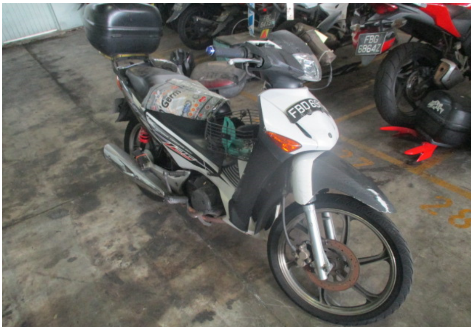
Photo 2 shows a general view of the right front body of the Motorcycle at the time of our inspection. The Motorcycle was observed to have sustained damages along its front and right side. Amongst the body parts that were found to have been damaged include its headlight assembly, front mudguard, right side mirror, front brake lever, right cowling, right front footrest, right rear side cover, exhaust muffler and top box, amongst others.
