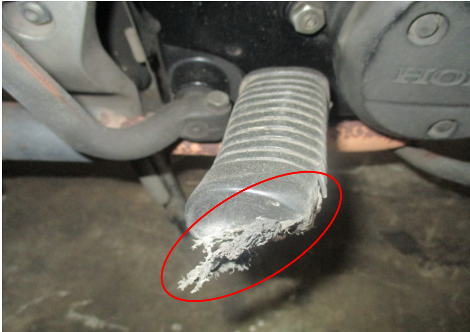
Photo 7 shows a closer view of the right front footrest (circled) which was amongst the body parts of the Motorcycle that had sustained damage as a result of the accident.
