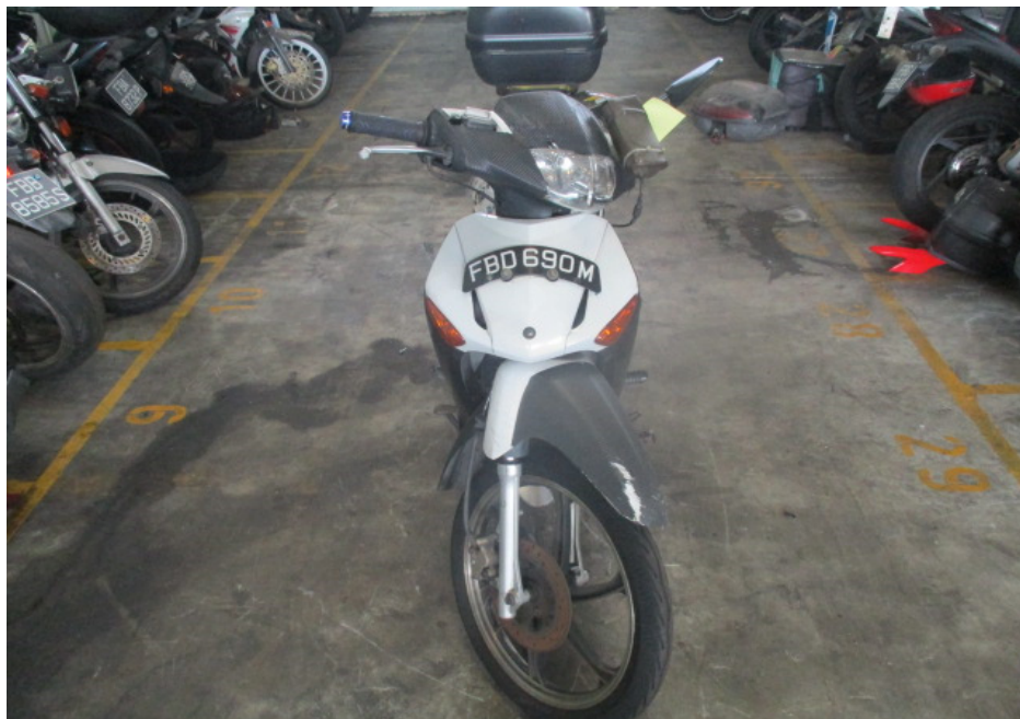
Photo 17 shows the front wheel of the Motorcycle turned towards its full left. Turning the Motorcycle's handle bar towards the left and right did not produce any abnormal free play and/or resistance. This would indicate that the steering system of the Motorcycle was in serviceable condition at the time of our inspection.
