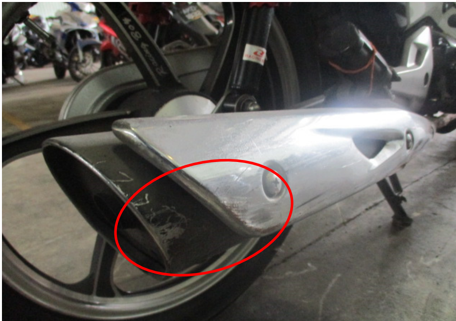
Photo 8 shows a close up view of the exhaust muffler and exhaust muffler heat shield (circled) which were amongst the body parts of the Motorcycle that had sustained damage as a result of the accident.
