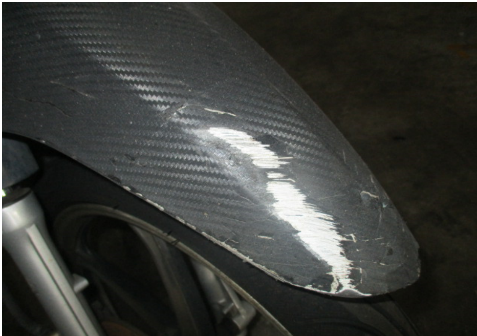
Photo 4 shows a closer view of the front mudguard which was amongst the body parts at the front body of the Motorcycle that had sustained damage as a result of the accident.
