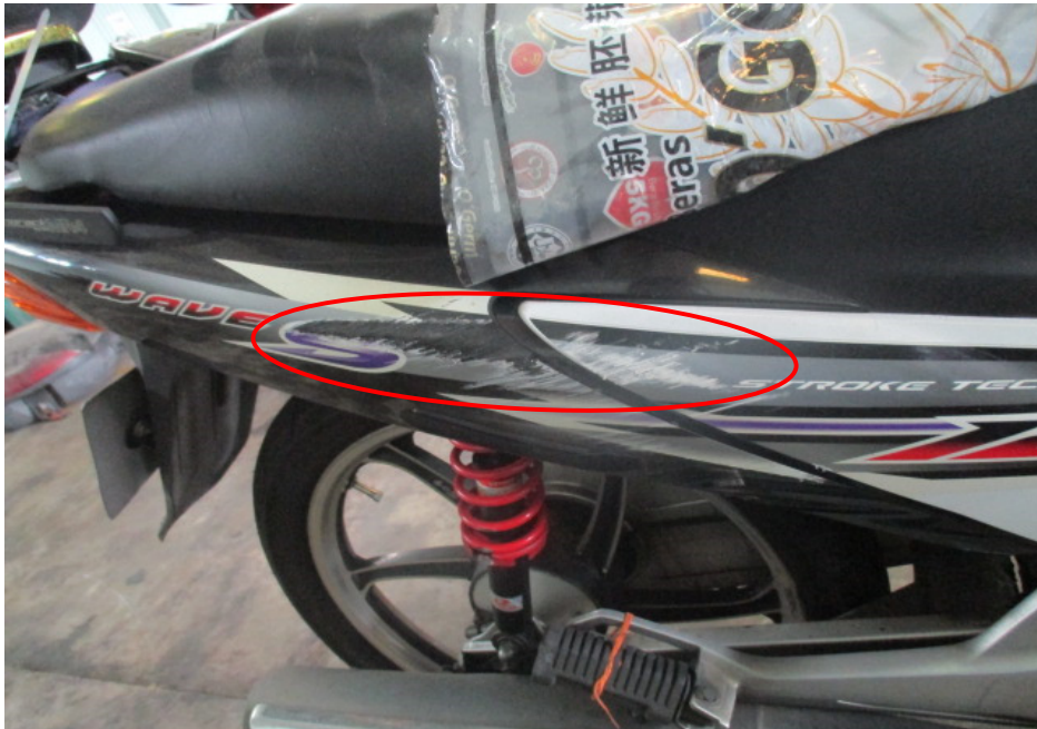
Photo 9 shows a close up view of the right rear side cover (circled) which was amongst the body parts of the Motorcycle that had sustained damage as a result of the accident.
