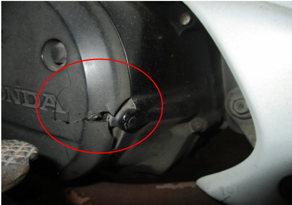
Photo 15 shows a close up of the crack sustained to the outer engine cover on the right side of the engine of the Motorcycle (circled). However we observed that the engine components were still intact. There was also no fluid leak and/or fluid stain found around the right engine area of the Motorcycle.
