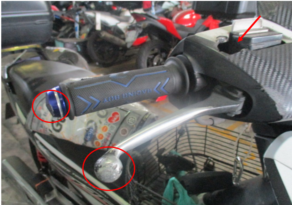
Photo 5 shows a closer view of the front brake lever and right handlebar end (circled) as well as the dislodged right side mirror (arrowed) which were amongst the body parts of the Motorcycle that had sustained damage as a result of the accident.
