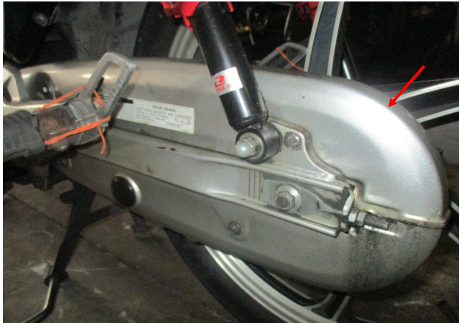
Photo 16 shows the general view of the gear train (arrowed) of the Motorcycle, which was observed to be intact with no misalignment.
