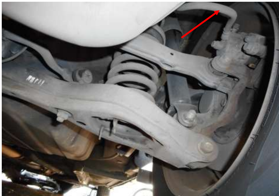
Photo 14 shows the various undercarriage components at the rear right wheel of the Motor Taxi, in particular the brake hose (arrowed). I did not observe any leakage of brake fluid at the 4 wheels of the Motor Taxi. My visual inspection of the Motor Taxi's various mechanical braking components revealed all to be intact without visible damage.
