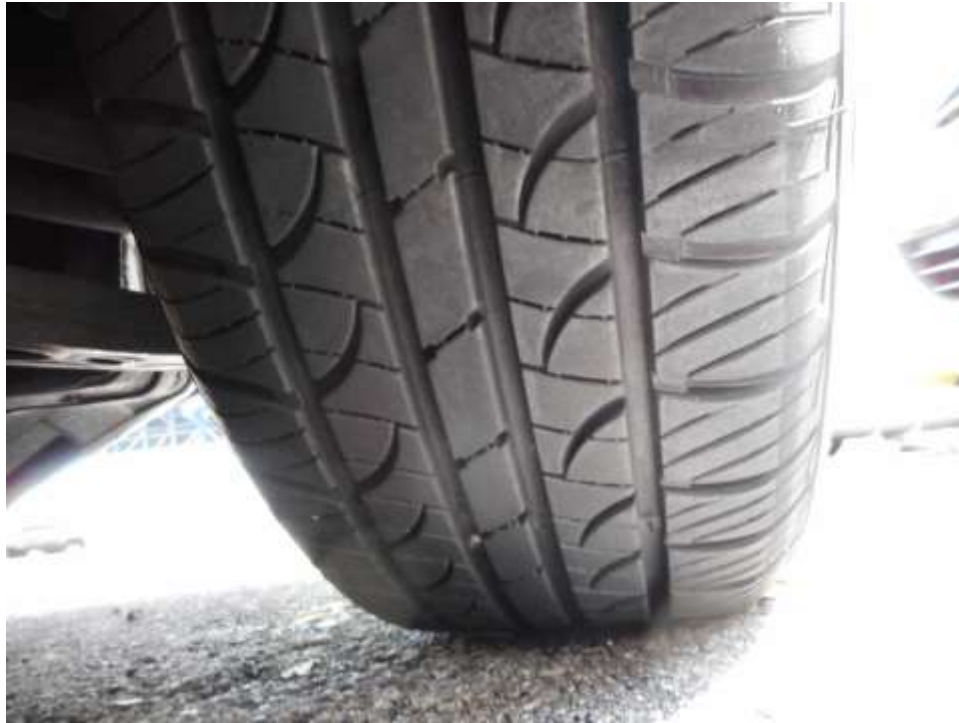
Photo 6 shows the condition of the front right tyre of the Motor Taxi, which was observed to be in serviceable condition with remaining tread depth of approximately 6.8mm. The tyre, which was wrapped around standard wheel rim, was also observed to be sufficiently inflated for vehicular operation.
