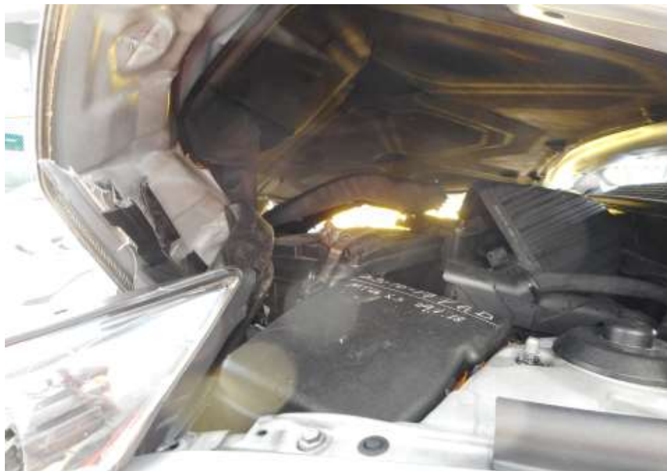
Photo 10 shows the close up view of the Motor Taxi's engine compartment. Parts that were mainly towards the front of the engine compartment were pushed inwards as a result of the impact force onto the frontal body of the Motor Taxi. The front support panel, front bumper reinforcement, cooling fan, air condenser, radiator and battery were all observed to have been damaged.
