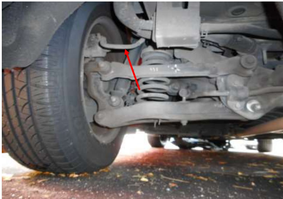
Photo 13 shows the various undercarriage components at the rear left wheel of the Motor Taxi, in particular the brake hose (arrowed). I did not observe any leakage of brake fluid at the 4 wheels of the Motor Taxi. My visual inspection of the various mechanical components of the Motor Taxi's braking system revealed all to be intact and without visible damage.
