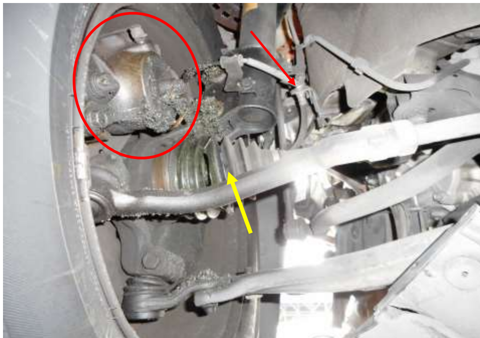
Photo 18 shows the brake hose/pipe (arrowed) at the front right wheel of the Motor Taxi. There was grease found on the brake caliper, it was caused by the broken boot of the drive shaft which splattered grease around the brake caliper (yellow arrow). However there was no brake fluid leak observed on and around the brake caliper itself. Visual examination of the various components of the braking system like the brake caliper (circled), had revealed all to be intact and without visible damage.
