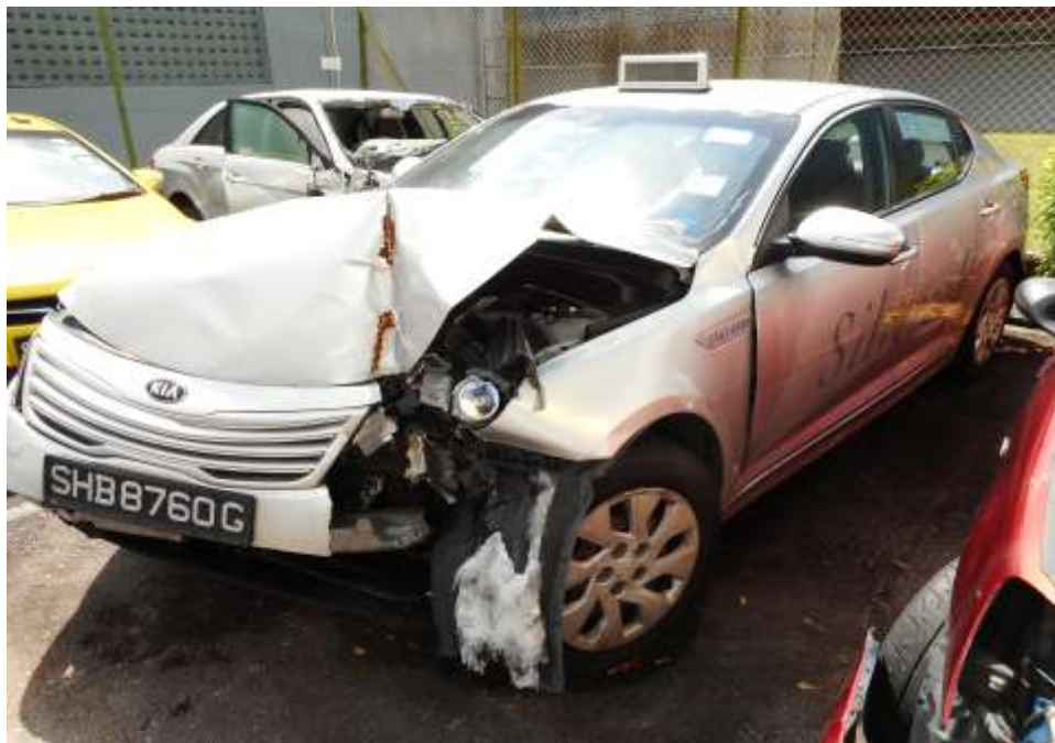
Photo 3 shows a general view of the front left body of the Motor Taxi at the time of my inspection. The Motor Taxi was observed to have sustained impact damage that was confined to its frontal body. Its front windscreen, front bumper, front bonnet, front left headlamp and front left fender were amongst the body parts that were damaged as a result of the accident
