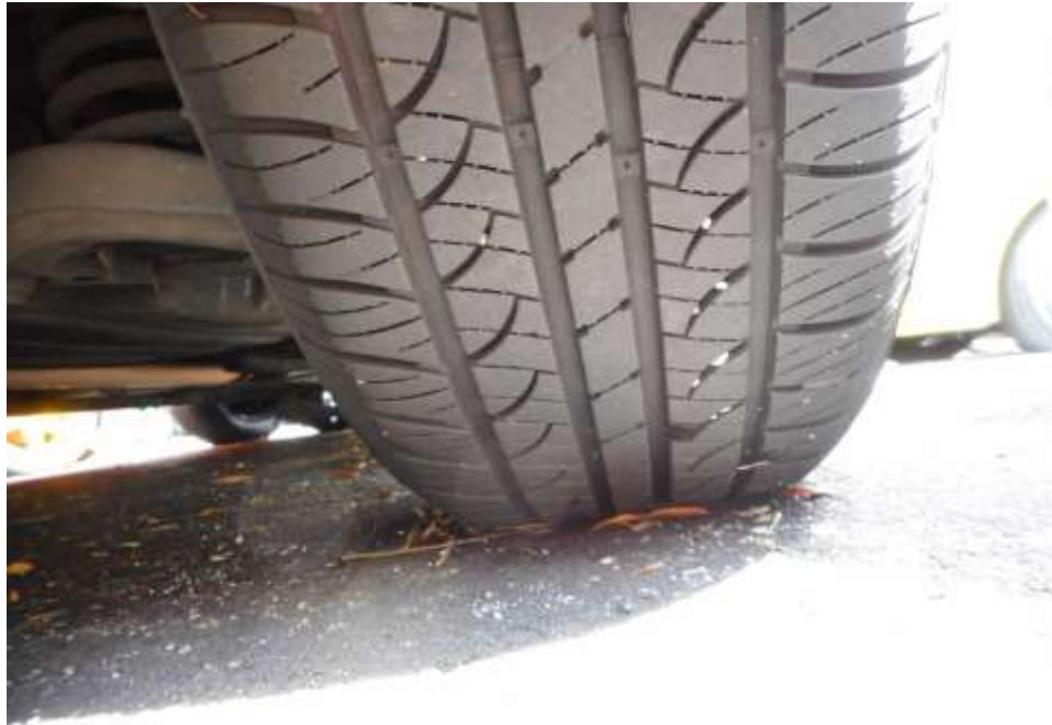
Photo 8 shows the condition of the rear right tyre of the Motor Taxi, which was observed to be in serviceable condition with remaining tread depth of approximately 7.8mm. There was no tear, cut or burst mark(s) on the outer and the inner sidewalls as well as across the tread of the tyre.
