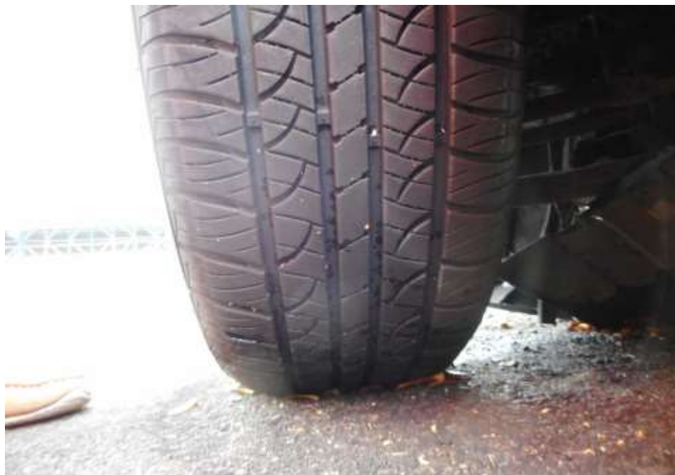
Photo 5 shows the condition of the front left tyre of the Motor Taxi, which was observed to be in serviceable condition with remaining tread depth of approximately 6.7mm. The tyre, which was wrapped around standard wheel rim, was also observed to be sufficiently inflated for vehicular operation. There was no tear, cut or burst mark(s) on the outer and the inner sidewalls as well as across the tread of the tyre.
