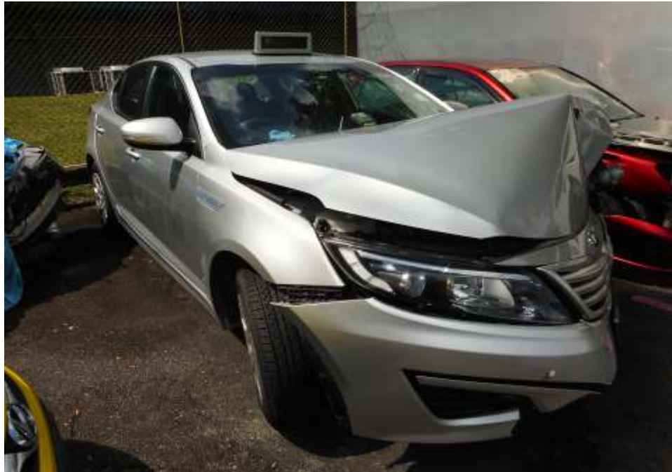
Photo 2 shows a general view of the front right body of the Motor Taxi at the time of my inspection. The Motor Taxi was observed to have sustained impact damage that was confined to its frontal body. Its front bumper and front bonnet were amongst the body parts that were damaged as a result of the accident. The mileage of the Motor Taxi was not recorded due to the extent of damage, which had affected the ignition system of the Motor Taxi.
