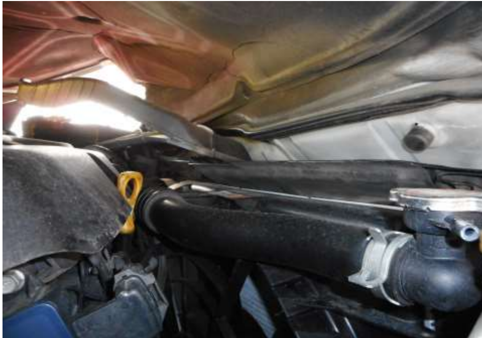
Photo 9 shows the close up view of the Motor Taxi's engine compartment. Parts towards the front of the engine compartment were observed to be damaged. The bonnet locking mechanism and the hinges of the Motor Taxi's front bonnet were damaged and unable to be opened as a result of the accident.
