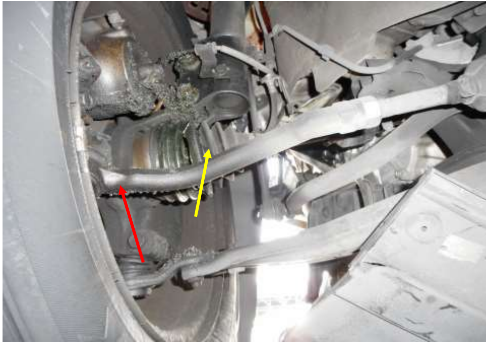
Photo 11 shows the various undercarriage components at the front left wheel of the Motor Taxi, in particular the steering tie rod (red arrow) and front left drive shaft (yellow arrow). There was a broken rubber boot found at the outer side of the drive shaft CV joint. However the various steering components were all found to be intact
