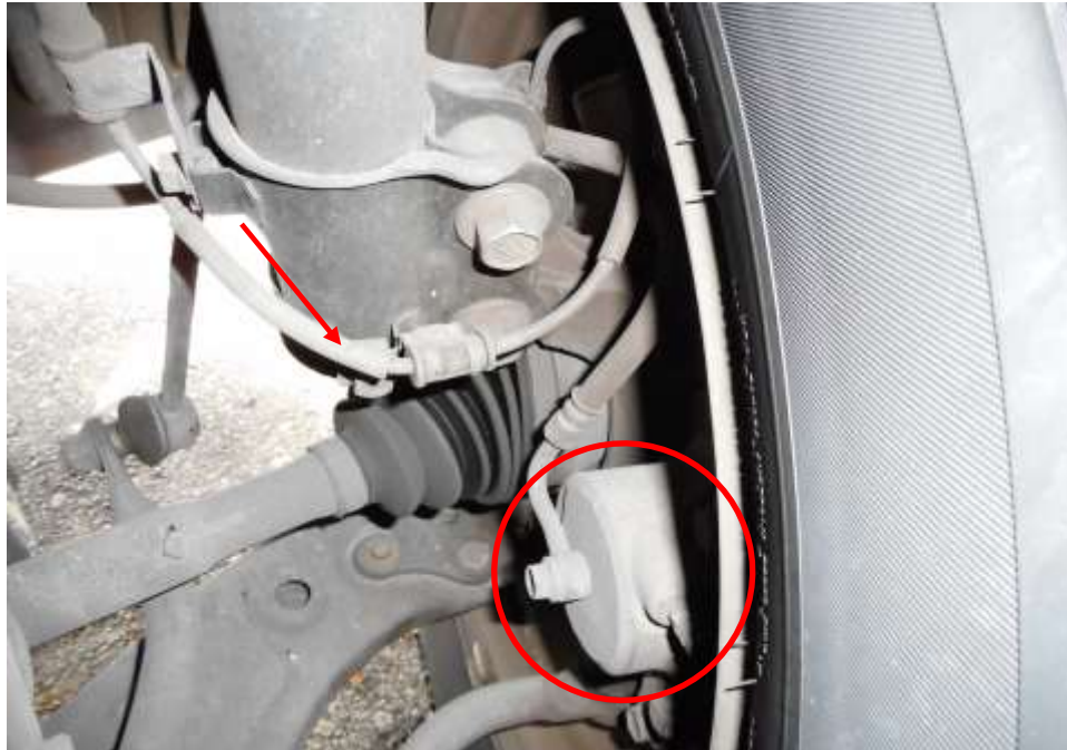
Photo 17 shows the brake hose/pipe (arrowed) at the front right wheel of the Motor Taxi. There was no brake fluid leak observed. Visual examination of the various components of the braking system like the brake caliper (circled), revealed all to be intact and without visible damage.
