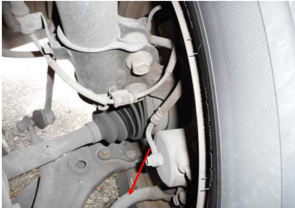
Photo 12 shows the various undercarriage components at the front right wheel of the Motor Taxi, in particular the steering tie rod (arrowed). The various steering components were all found to be intact
