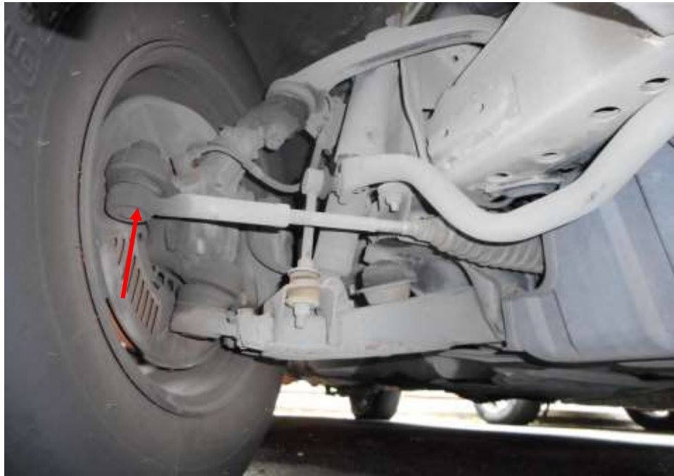
Photo 24 shows the various undercarriage components at the front right wheel of the Mini Bus, in particular the steering tie rod (arrowed). The various steering components were all found to be intact, suggesting that the steering system of the Mini Bus was likely to be in serviceable condition at the material time of accident. There was also no sign of fluid stain observed on the various undercarriage components at the front right wheel of the Mini Bus.
