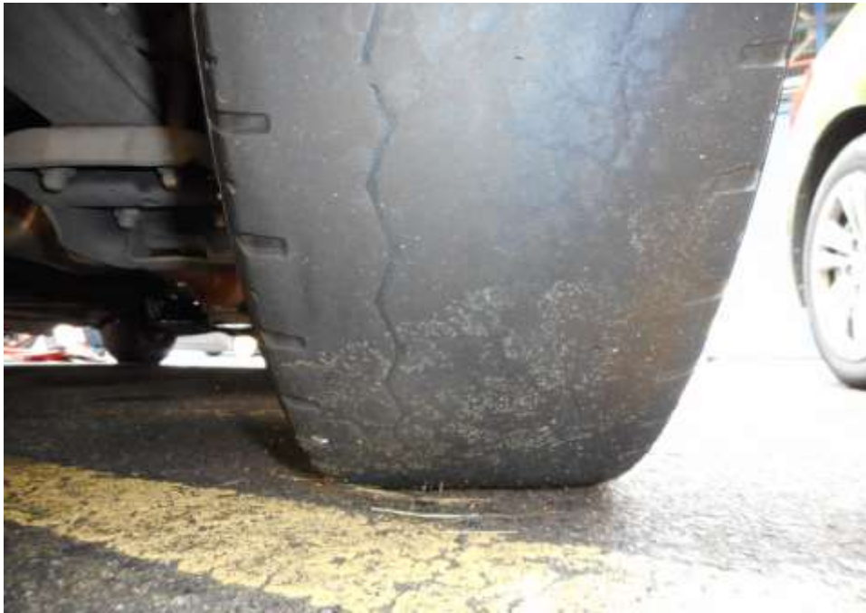
Photo 10 shows the condition of the rear right tyre of the Mini Bus. The tyre was observed to be sufficiently inflated for vehicular operation with no tear, cut or burst mark(s). However was observed to be in unserviceable condition with remaining tread depth of approximately 0.5mm.
