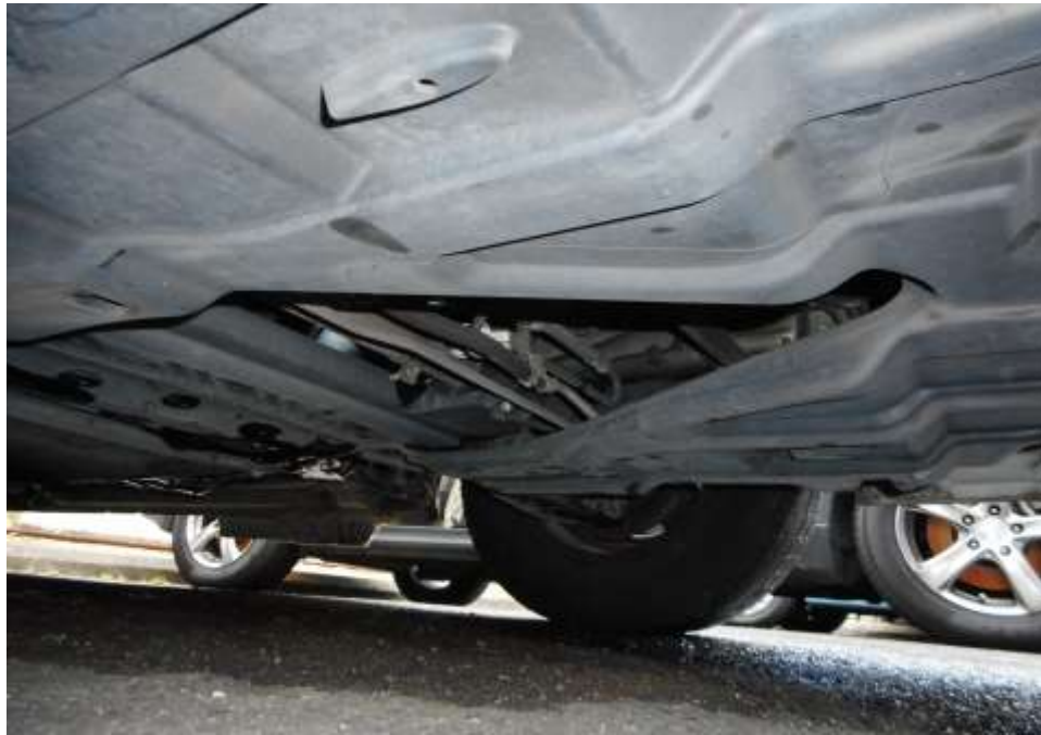
Photo 19 shows the undercarriage of the Mini Bus, at the area where the engine housing and transmission housing are located. I did not find any sign(s) or indication(s) of fluid leak and/or fluid stain(s) on the underside of the Mini Bus.
