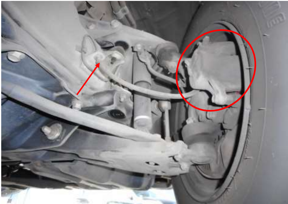
Photo 22 shows the brake hose/pipe (arrowed) at the front right wheel of the Mini Bus. No leakage of brake fluid was observed. Visual examination of the various components of the braking system like the brake caliper (circled), brake booster, brake pedal etc had revealed all to be intact and without visible damage.
