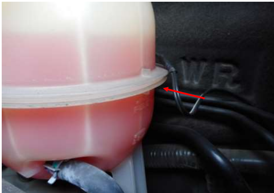
Photo 16 shows checks being carried out to the engine coolant of the Mini Bus at the time of my inspection. The engine coolant was observed to be of sufficient level (arrowed) and without any visible contamination.
