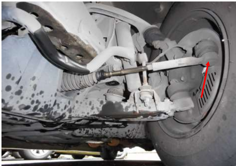
Photo 25 shows the various undercarriage components at the front left wheel of the Mini Bus, which had included the steering tie rod (red arrow) the various undercarriage components of the Mini Bus were all found to be intact without any visible damage.
