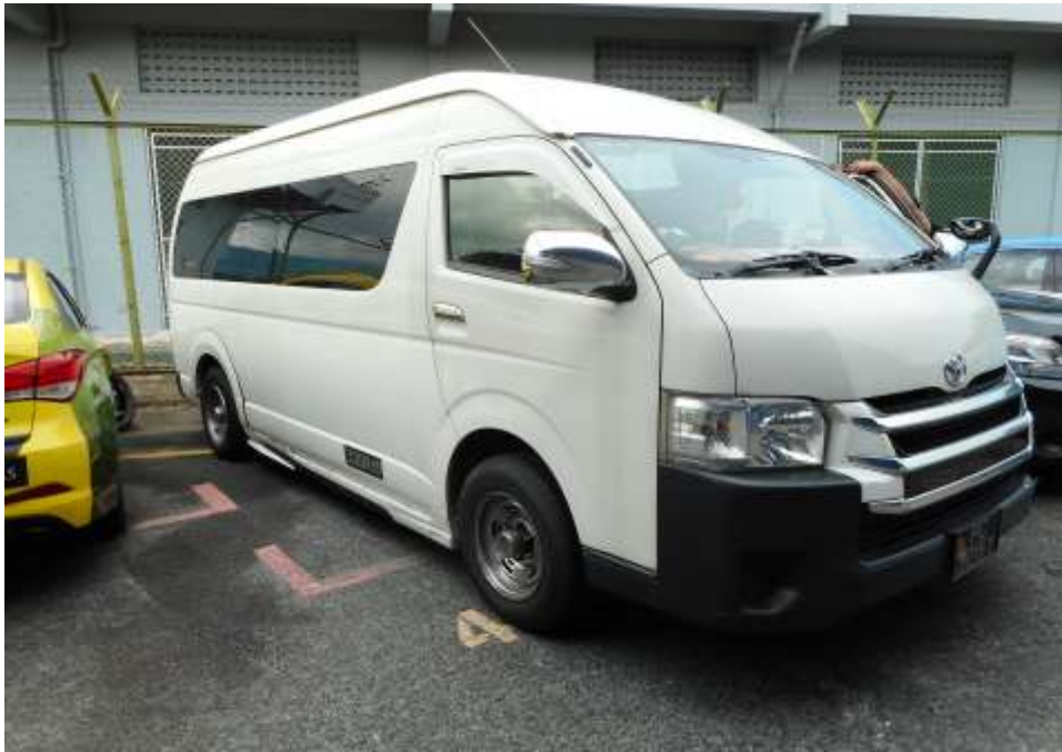
Photo 6 shows a general view of the Mini Bus's right body at the time of my inspection. The right portion of the Mini Bus was observed to have been unaffected by the accident.
