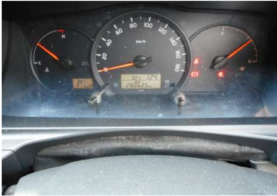
Photo 27 shows no warning lights illuminated on the instrument panel of the Mini Bus after the engine was cranked. This would suggest that there was no abnormality to the various electronic operating systems of the Mini Bus, like the ABS and SRS etc.
