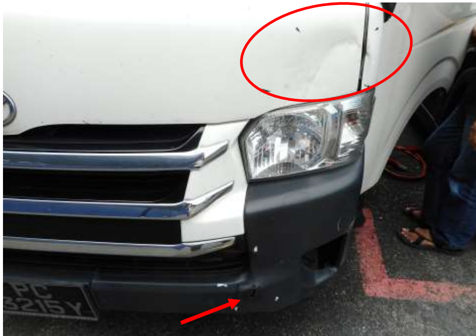
Photo 2 shows a close up view of the damaged front bonnet (circled) and bumper (arrowed) of the Mini Bus at the time of my inspection as a result of the accident.
