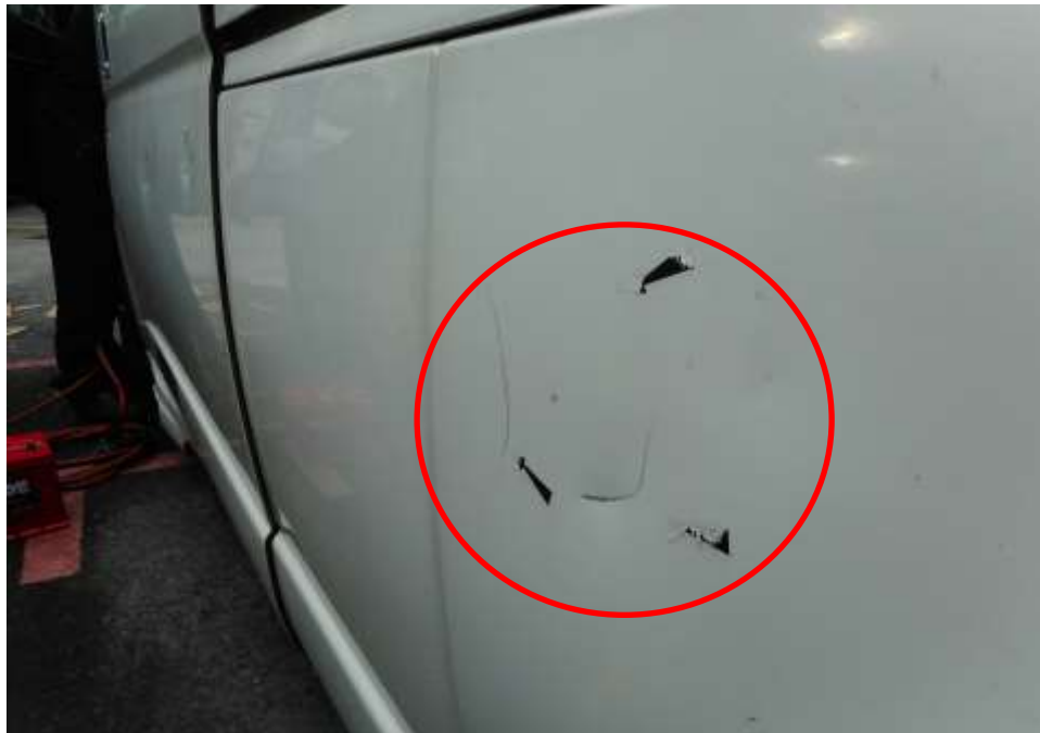
Photo 5 shows a close up view of the damaged left door panel (circled) of the Mini Bus at the time of my inspection as a result of the accident.
