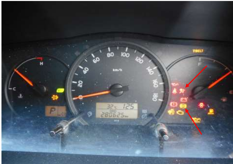
Photo 26 shows the warning light for Anti-Lock Brake System (ABS) and Supplemental Restraint System (SRS) appearing on the instrument panel of the Mini Bus during the self-test of its various electronic operating systems when its engine was cranked.
