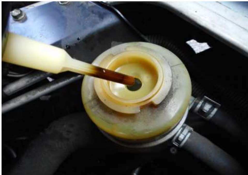
Photo 18 shows the power steering dip stick of the Mini Bus at the time of my inspection. The power steering fluid was observed to be of sufficient level and without any visible contamination.
