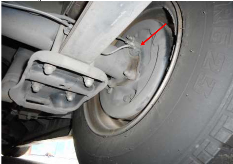
Photo 21 shows the brake hose/pipe (arrowed) at the rear right wheel of the Mini Bus. I did not observe any leakage of brake fluid at the time of my inspection of the Mini Bus. Static tests of the Mini Bus's braking system had indicated that there was no internal leakage of pressure/vacuum. The undercarriage components of the Mini Bus were also all found to be intact and without any visible damage.
