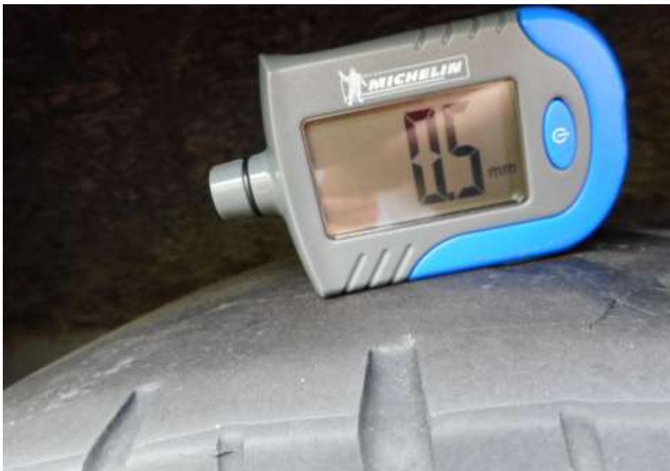
Photo 11 shows the tread depth measurement of the rear right tyre of the Mini Bus. The tyre was observed to be of unserviceable condition with remaining tread depth of approximately 0.5mm, at the time of inspection.
