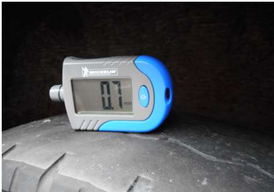
Photo 13 shows the tread depth measurement of the rear left tyre of the Mini Bus. The tyre was observed to be of unserviceable condition with remaining tread depth of approximately 0.7mm, at the time of inspection.
