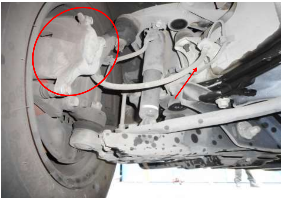
Photo 23 shows the brake hose/pipe (arrowed) at the front left wheel of the Mini Bus. No leakage of brake fluid was observed. Visual examination of the various components of the braking system like the brake caliper (circled), brake booster, brake pedal etc had revealed all to be intact and without visible damage.
