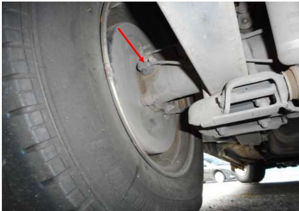
Photo 20 shows the brake hose/pipe (arrowed) at the rear left wheel of the Mini Bus. I did not observe any leakage of brake fluid at the time of my inspection of the Mini Bus. Static tests of the Mini Bus's braking system had indicated that there was no internal leakage of pressure/vacuum. The undercarriage components of the Mini Bus were also all found to be intact and without any visible damage.
