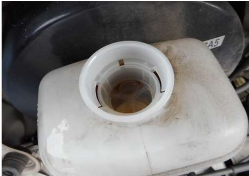
Photo 15 shows the brake fluid reservoir of the Mini Bus at the time of my inspection. The brake fluid was observed to be of sufficient level and without any visible contamination.
