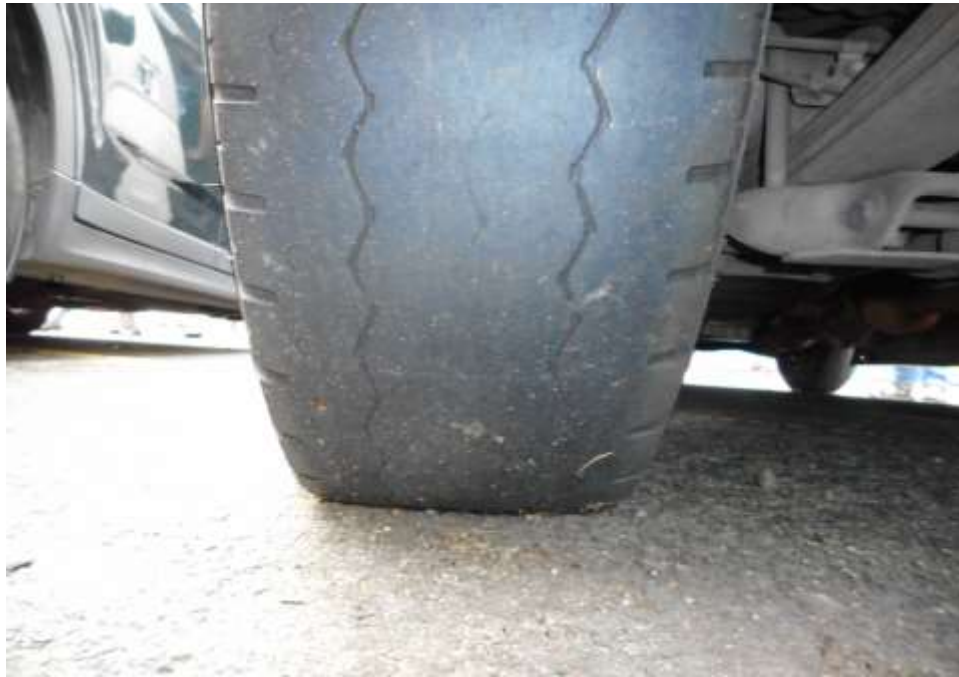
Photo 12 shows the condition of the rear left tyre of the Mini Bus. The tyre was observed to be sufficiently inflated for vehicular operation with no tear, cut or burst mark(s). However was observed to be in unserviceable condition with remaining tread depth of approximately 0.7mm.
