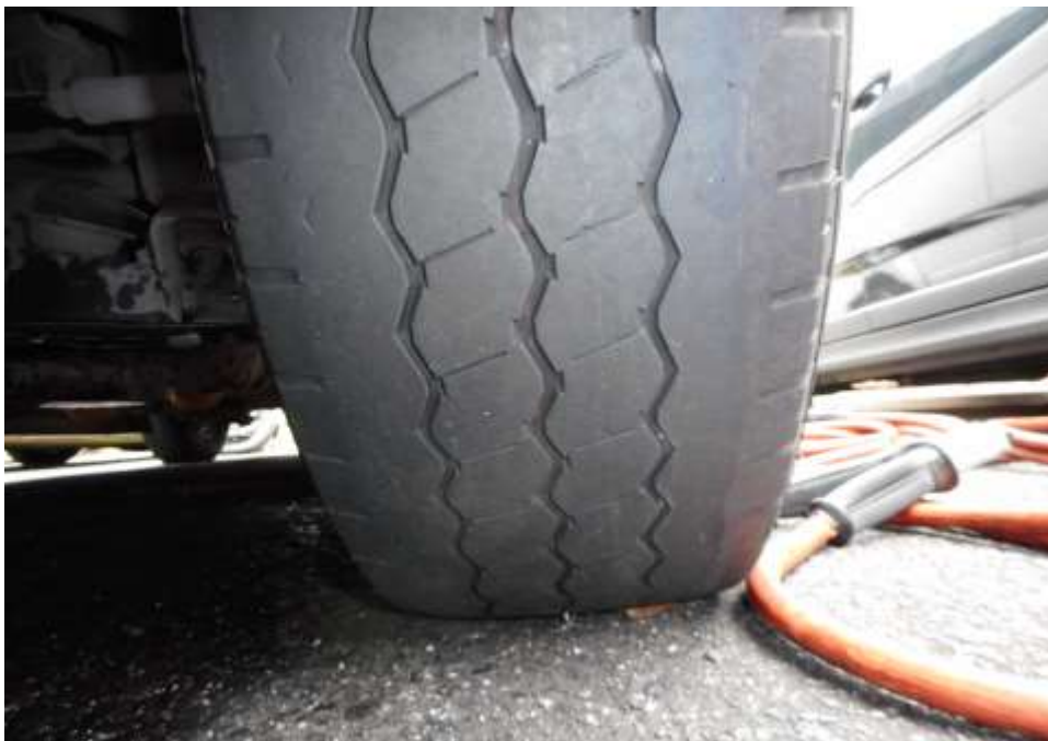
Photo 9 shows the condition of the front left tyre of the Mini Bus, which was observed to be in serviceable condition with remaining tread depth of approximately 2.7mm. There was also no tear, cut or burst mark(s) on the outer and the inner sidewalls as well as across the tread of the Mini Bus's 4 tyres.
