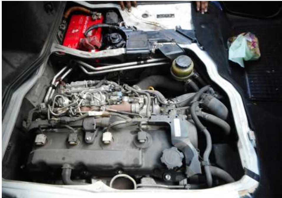
Photo 14 shows a general view of the Mini Bus's engine compartment. The various parts and components inside the engine compartment were unaffected by the accident. There was also no sign(s) or indication(s) of fluid leakage and/or fluid stain within the engine compartment.
