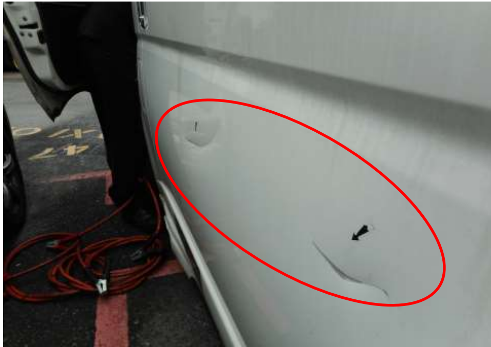
Photo 4 shows a close up view of the damaged left sliding door panel (circled) of the Mini Bus at the time of my inspection as a result of the accident.
