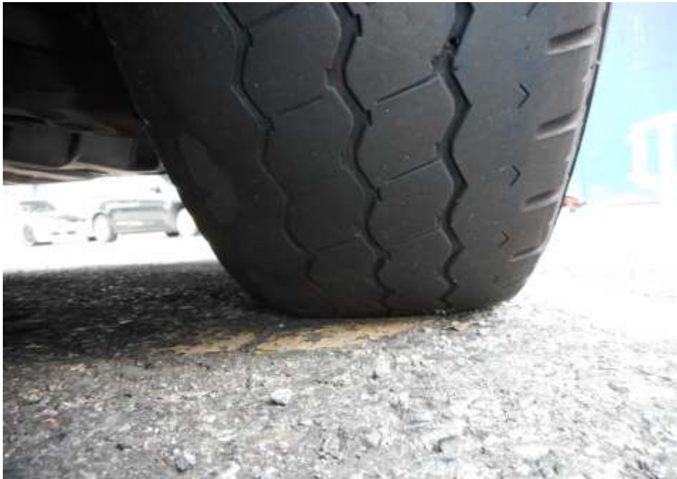
Photo 8 shows the condition of the front right tyre of the Mini Bus, which was observed to be in serviceable condition with remaining tread depth of approximately 2.8mm. The tyre was sufficiently inflated for vehicular operation with no tear, cut or burst mark(s) on the outer and the inner sidewalls as well as across the tread. The 4 tyres of the Mini Bus were wrapped around standard steel wheel rims without any damage.
