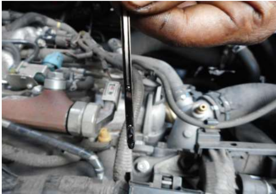
Photo 17 shows the engine oil dip stick of the Mini Bus at the time of my inspection. The engine oil was observed to be of sufficient level and without any visible contamination.
