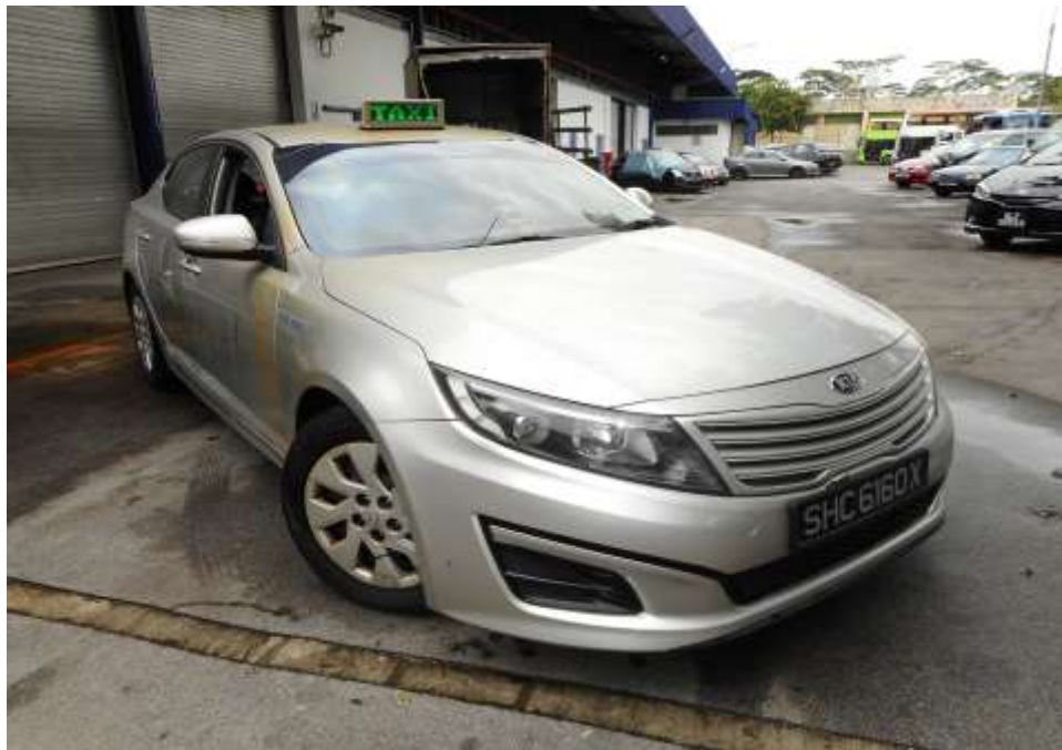
Photo 25 shows the front right wheel of the Motor Taxi turned to its full left. During my steering system test, I did not experience any abnormal free play and/or resistance when I had turned the steering wheel towards the left and right. This would suggest that the steering system of the Motor Taxi was likely to be in serviceable condition at the material time of accident.
