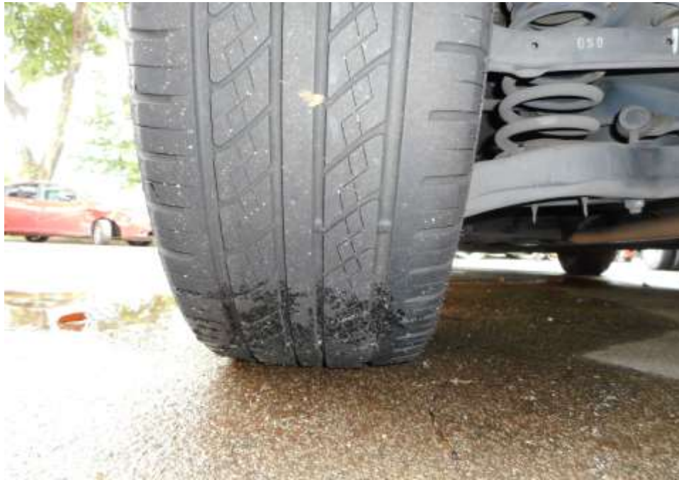
Photo 8 shows the condition of the rear left tyre of the Motor Taxi, which was observed to be in serviceable condition with remaining tread depth of approximately 4.6 mm. The tyre was also observed to be sufficiently inflated for vehicular operation with no tear, cut or burst mark(s).
