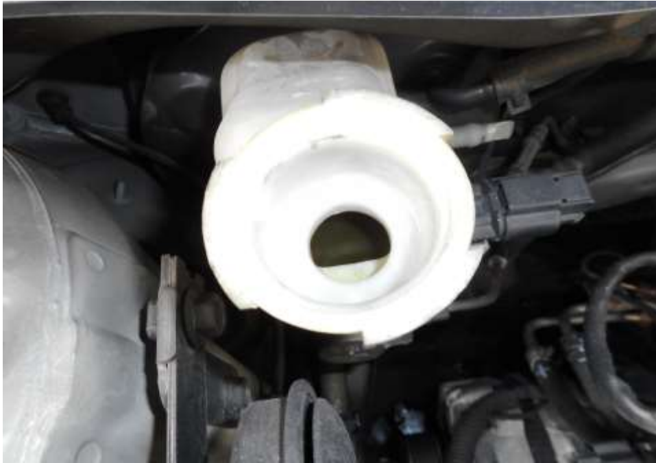
Photo 11 shows the brake fluid reservoir of the Motor Taxi at the time of my inspection. The brake fluid was observed to be of sufficient level and without any visible contamination.
