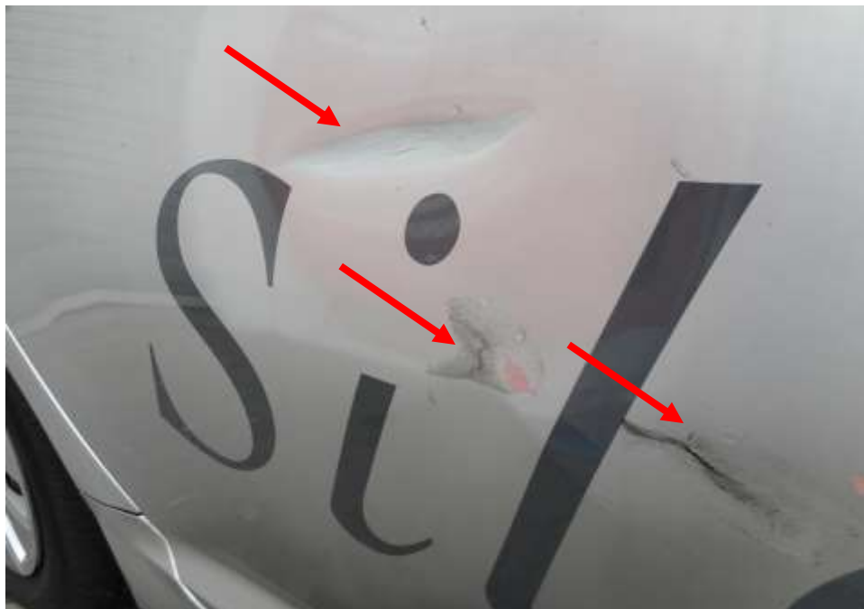
Photo 3 shows a general view of the Motor Taxi's right body panel at the time of my inspection. The right door panel portion (arrowed) of the Motor Taxi was observed to have sustained minor damages as a result of the accident.
