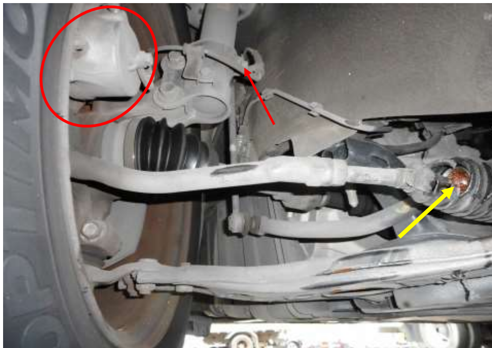
Photo 17 shows the brake hose/pipe (red arrow) at the front left wheel of the Motor Taxi. No leakage of brake fluid was observed. Visual examination of the various components, the inner rubber boot (yellow arrow) of the right steering rack was observed to be broken. However the other various components of the braking system like the brake caliper (circled), brake booster, brake pedal etc had revealed all to be intact and without visible damage.
