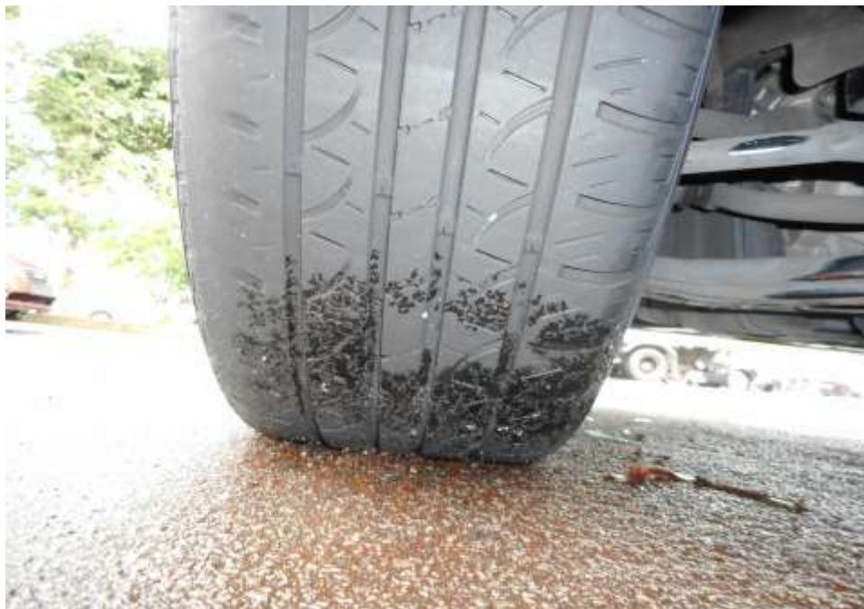
Photo 9 shows the condition of the front left tyre of the Motor Taxi, which was observed to be in serviceable condition with remaining tread depth of approximately 3.8mm. The tyre was also observed to be sufficiently inflated for vehicular operation with no tear, cut or burst mark(s).
