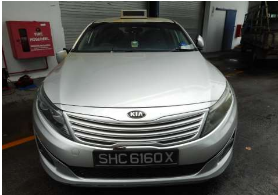
Photo 1 shows a front general view of the Motor Taxi's at the time of my inspection. The front portion of the Motor Taxi was observed to have been unaffected by the accident. The mileage of the Motor Taxi at the time of my inspection was recorded to be 364,863km.
