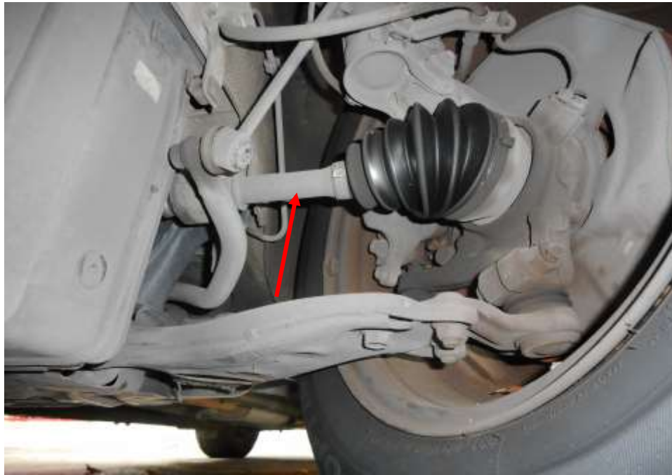
Photo 22 shows front right drive shaft (arrowed) undercarriage component at the front right wheel of the Motor Taxi, were found to be intact without any visible damage.
