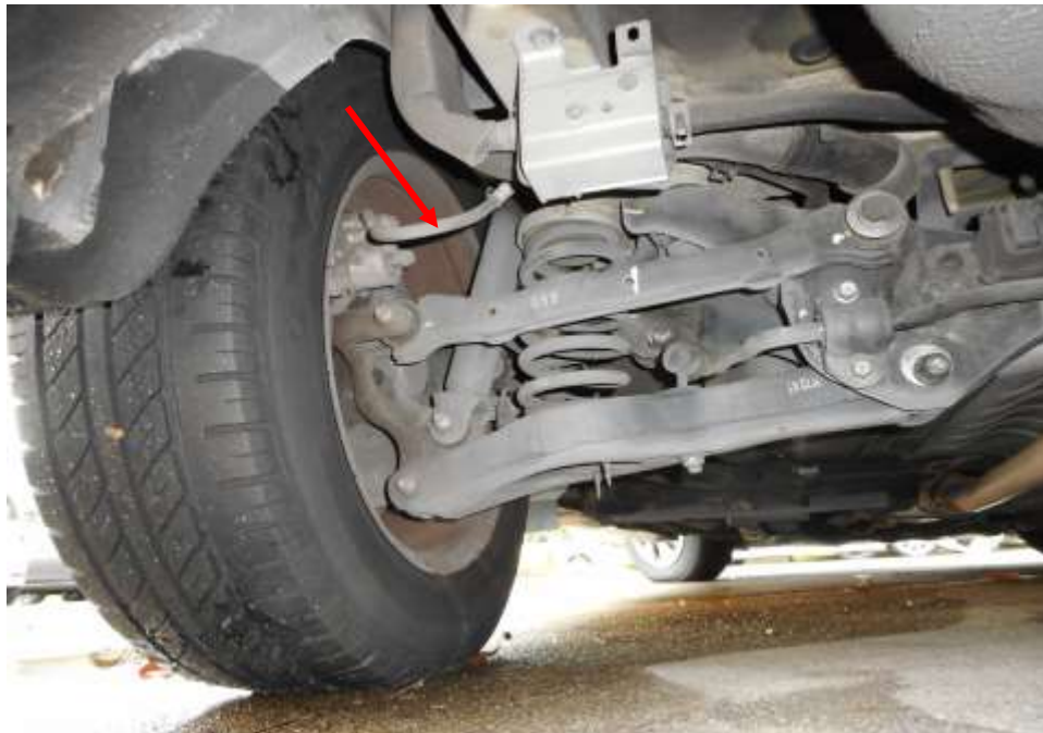
Photo 15 shows the brake hose/pipe (arrowed) at the rear left wheel of the Motor Taxi. I did not observe any leakage of brake fluid at the time of my inspection of the Motor Taxi. Static tests of the Motor Taxi's braking system had indicated that there was no internal leakage of pressure/vacuum. The undercarriage components of the Motor Taxi were also all found to be intact and without any visible damage.
