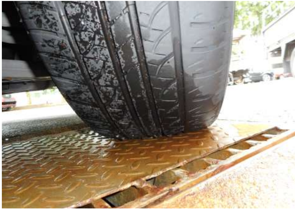
Photo 6 shows the condition of the front right tyre of the Motor Taxi, which was observed to be in serviceable condition with remaining tread depth of approximately 4.5mm. The tyre was sufficiently inflated for vehicular operation with no tear, cut or burst mark(s) on the outer and the inner sidewalls as well as across the tread. The 4 tyres of the Motor Taxi were wrapped around standard steel wheel rims without any damage.
