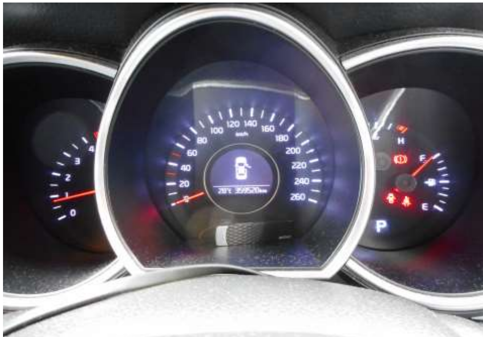
Photo 24 shows no warning lights illuminated on the instrument panel of the Motor Taxi after the engine was cranked. This would suggest that there was no abnormality to the various electronic operating systems of the Motor Taxi, like the ABS, EPS, TC and SRS etc.
