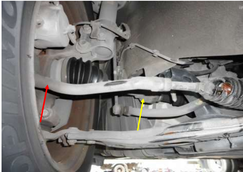
Photo 20 shows the various undercarriage components at the front left wheel of the Motor Taxi, which had included the steering tie rod (red arrow) and front left drive shaft (yellow arrow). The various undercarriage components of the Motor Taxi were all found to be intact without any visible damage.
