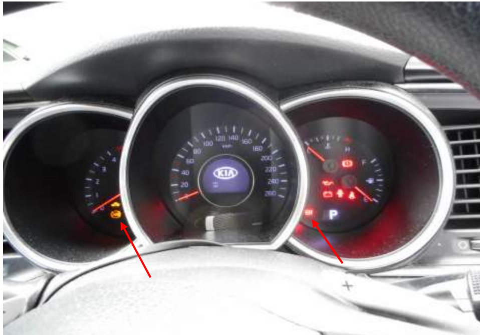
Photo 23 shows the warning light for Anti-Lock Brake System (ABS), Electric Power Steering System (EPS), Traction Control (TC) and Supplemental Restraint System (SRS) appearing on the instrument panel of the Motor Taxi during the self-test of its various electronic operating systems when its engine was cranked.
