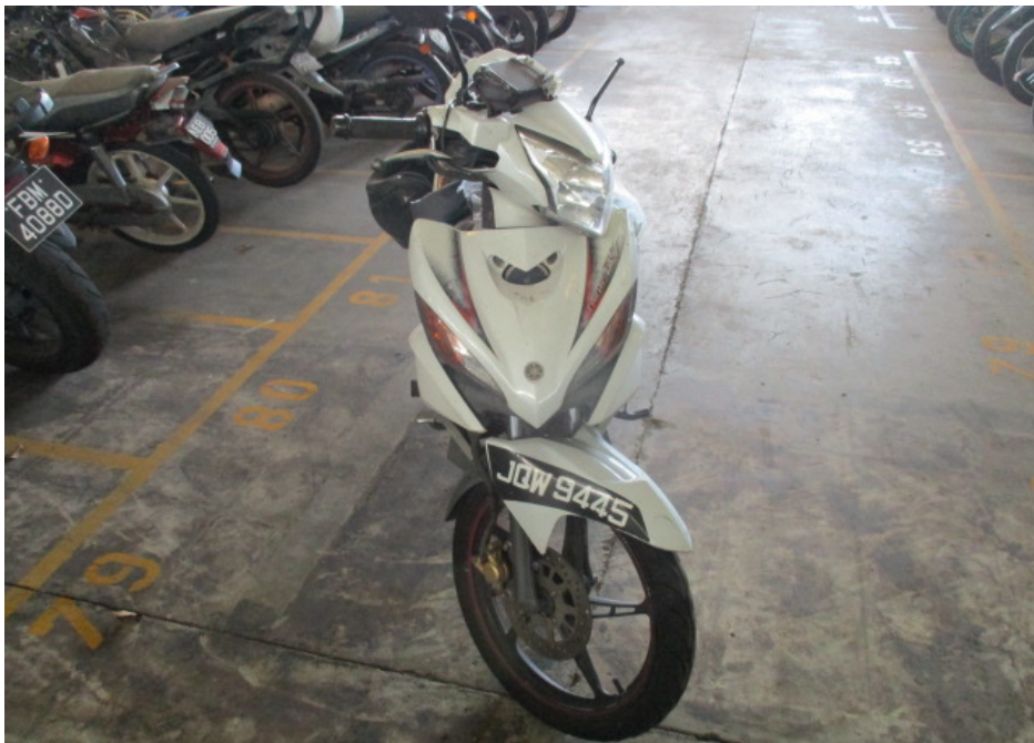
Photo 20 shows the front wheel of the Motorcycle turned towards its full left. Turning the Motorcycle's handle bar towards the left and right did not produce any abnormal free play and/or resistance. This would indicate that the steering system of the Motorcycle was in serviceable condition at the time of our inspection.
