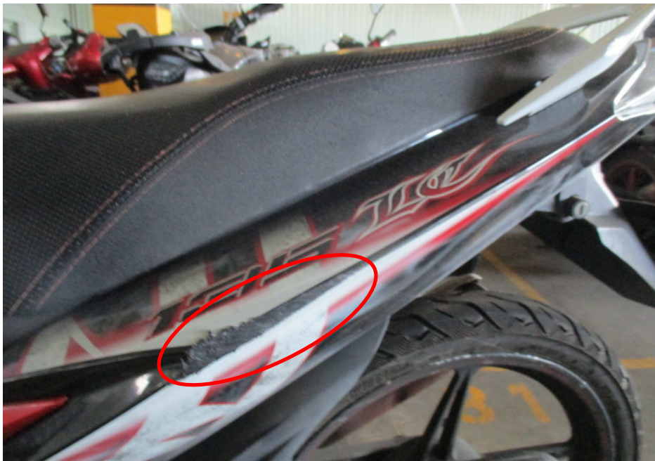
Photo 11 shows a closer view of the left rear side cover (circled) which was amongst the body parts of the Motorcycle that had sustained damage as a result of the accident.
