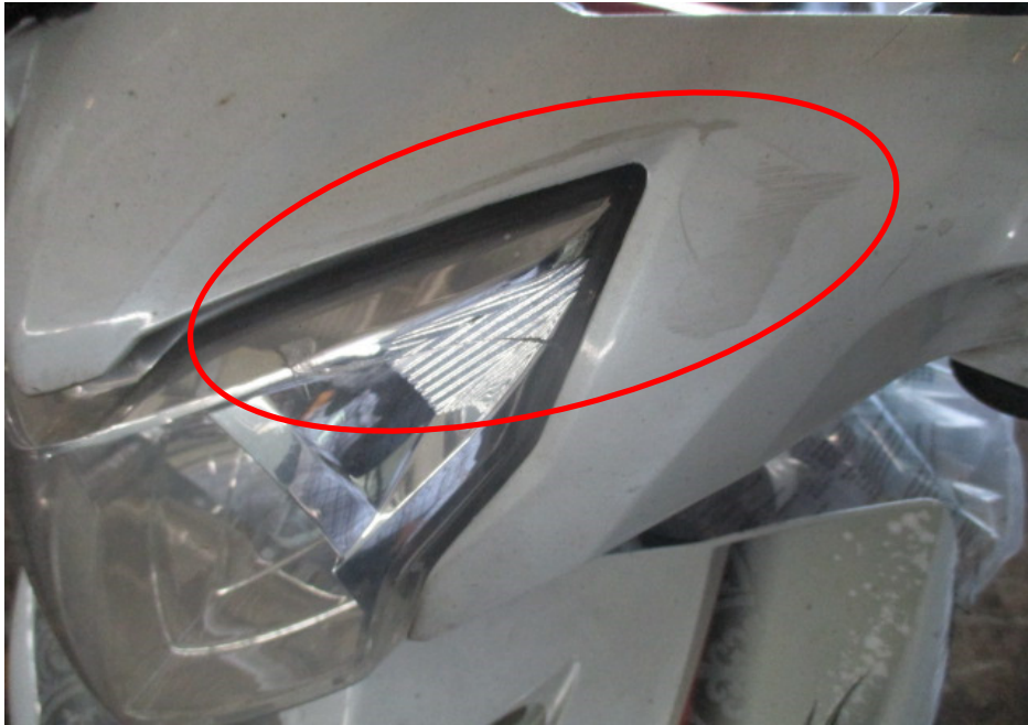
Photo 4 shows a closer view of the headlight assembly (circled) which was amongst the body parts at the front body of the Motorcycle that had sustained damage as a result of the accident.
