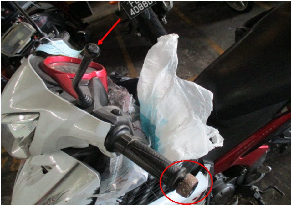
Photo 8 shows a closer view of the left side mirror (arrowed) and left handlebar end (circled) which were amongst the body parts of the Motorcycle that had sustained damage as a result of the accident.
