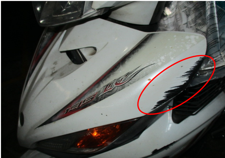
Photo 5 shows a close up view of the front cowling (circled) which was amongst the body parts of the Motorcycle that had sustained damage as a result of the accident.
