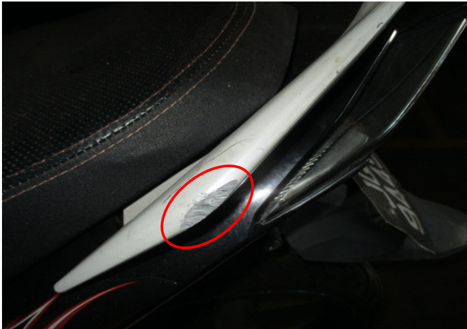
Photo 12 shows a closer view of the left pillion grab rail (circled) which was amongst the body parts of the Motorcycle that had sustained damage as a result of the accident.
