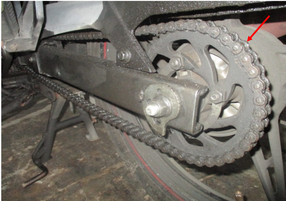
Photo 17 shows the general view of the gear train (arrowed) of the Motorcycle, which was observed to be intact with no misalignment. It was also adequately lubricated for operating purposes.
