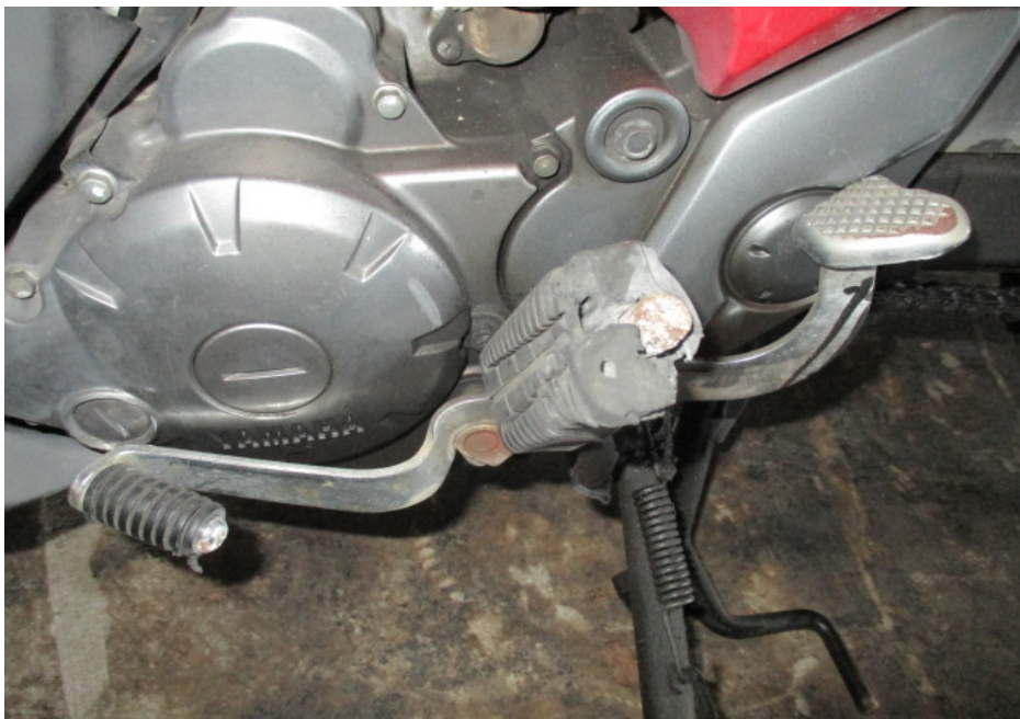
Photo 9 shows a closer view of the gear shift pedal, left front footrest and left front footrest bracket, which were amongst the body parts of the Motorcycle that had sustained damage as a result of the accident.
