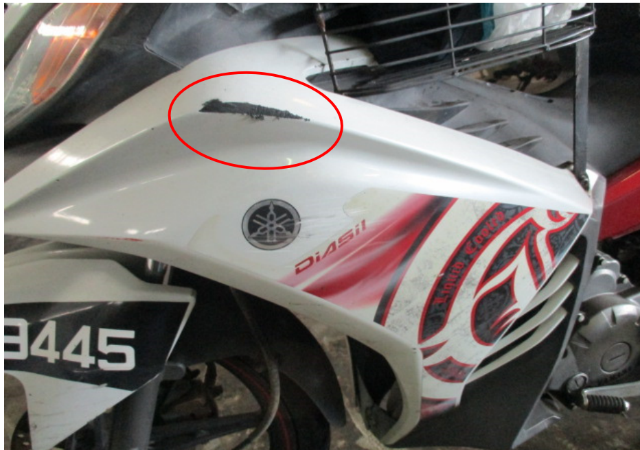
Photo 7 shows a closer view of the left cowling of the Motorcycle (circled) that had sustained damage as a result of the accident.
