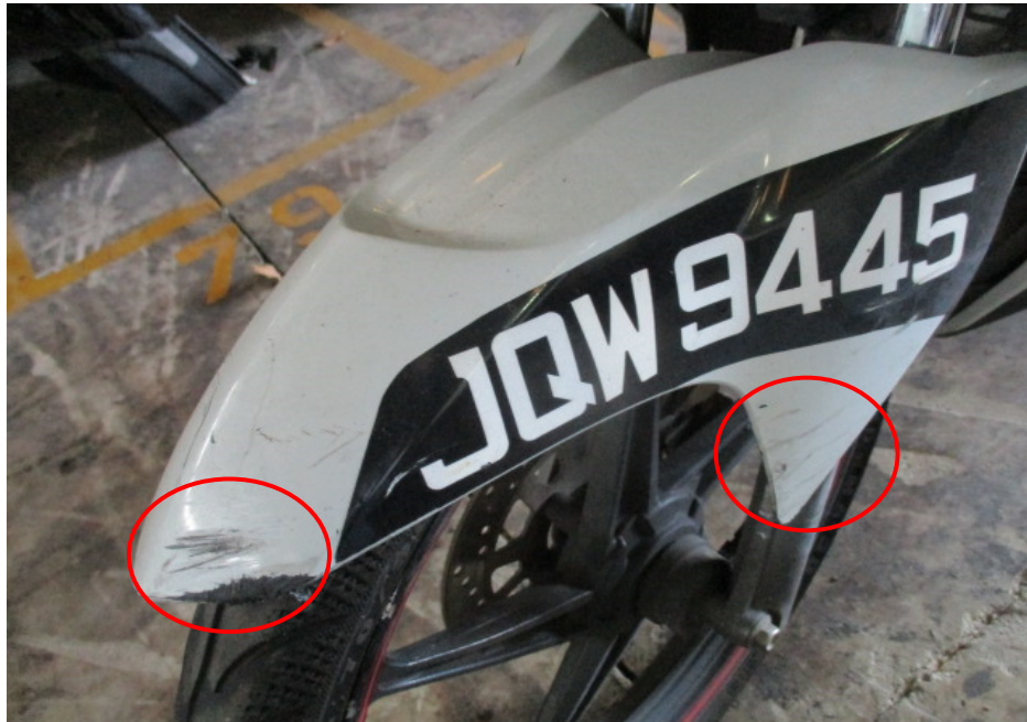
Photo 6 shows a closer view of the front mudguard (circled) which was amongst the body parts at the front body of the Motorcycle that had sustained damage as a result of the accident.
