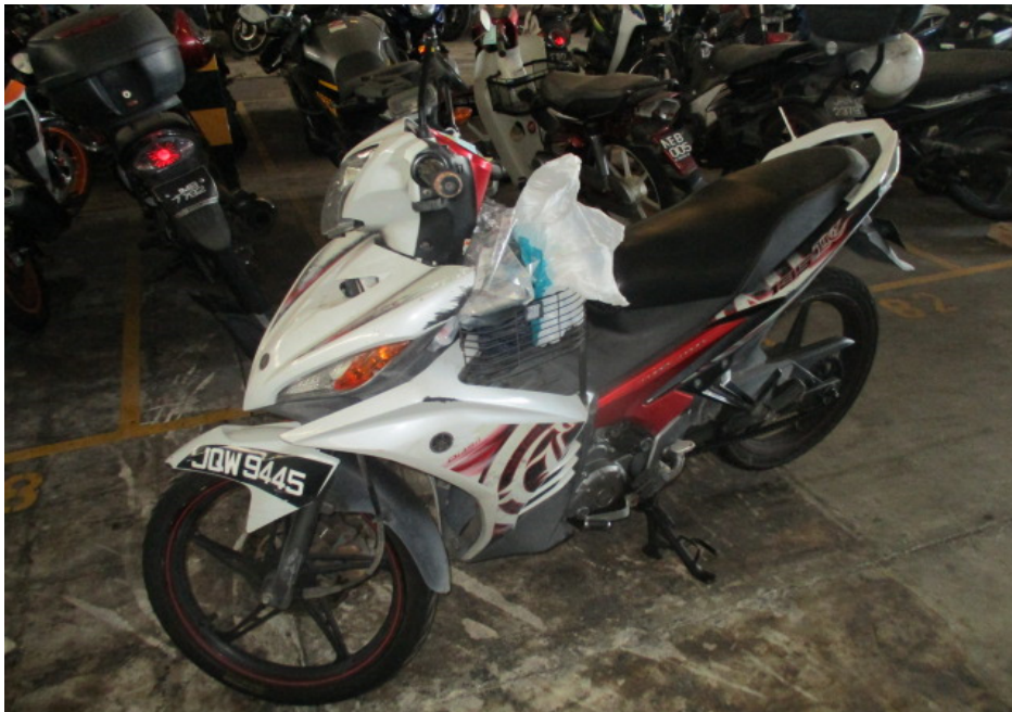
Photo 3 shows a general view of the left front body of the Motorcycle at the time of our inspection. The Motorcycle was observed to have sustained damages along its front and left side. Amongst the body parts that were found to have been damaged include its headlight assembly, front cowling, front mudguard, left side mirror, gear shift pedal, left front footrest and left rear side cover, amongst others.
