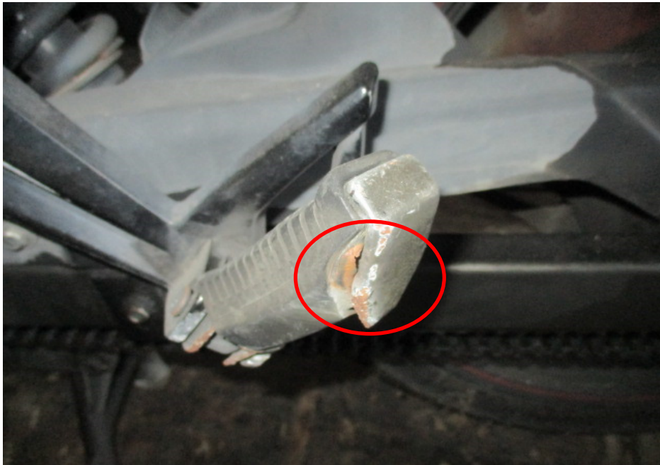
Photo 10 shows a closer view of the left pillion footrest (circled) which was amongst the body parts of the Motorcycle that had sustained damage as a result of the accident.
