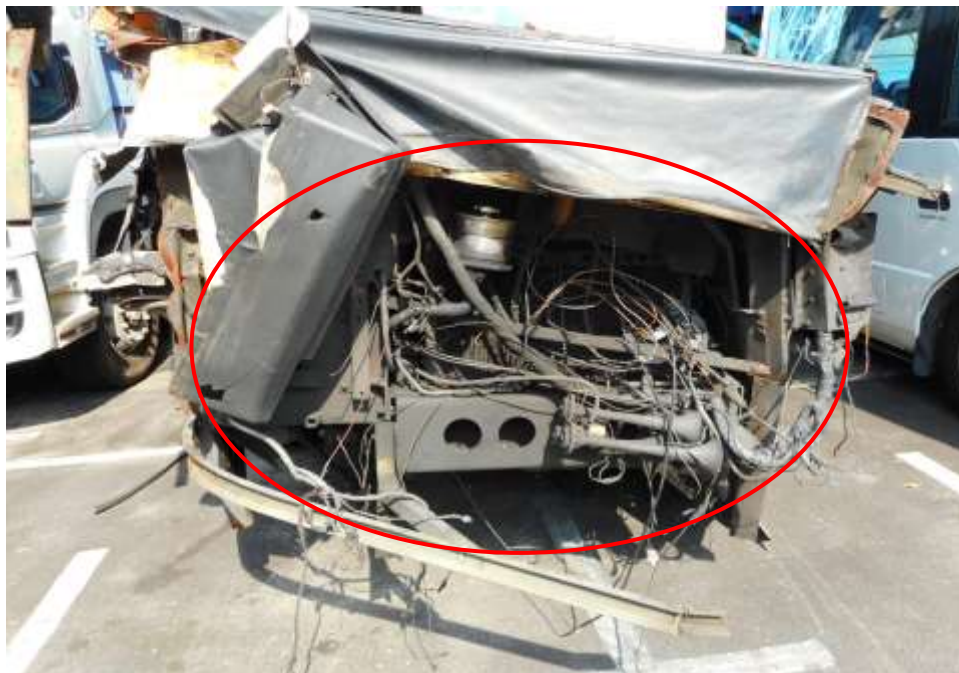
Photo 3 shows a general view of the front body of the Motor Bus at the time of our inspection. The Motor Bus was observed to have sustained extensive damages at its front portion (circled) as a result of the accident's collision.
