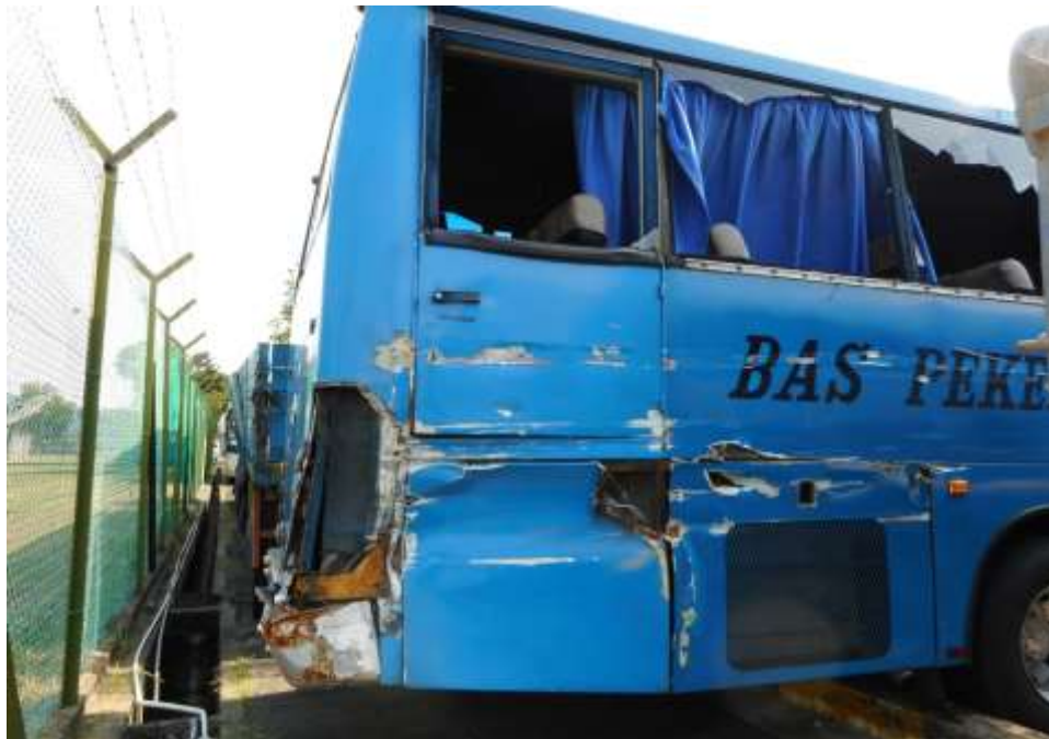
Photo 14 shows a general view of the rear right body of the Motor Bus at the time of our inspection. The Motor Bus was observed to have sustained extensive damages at its rear right portion as a result of the accident's collision.
