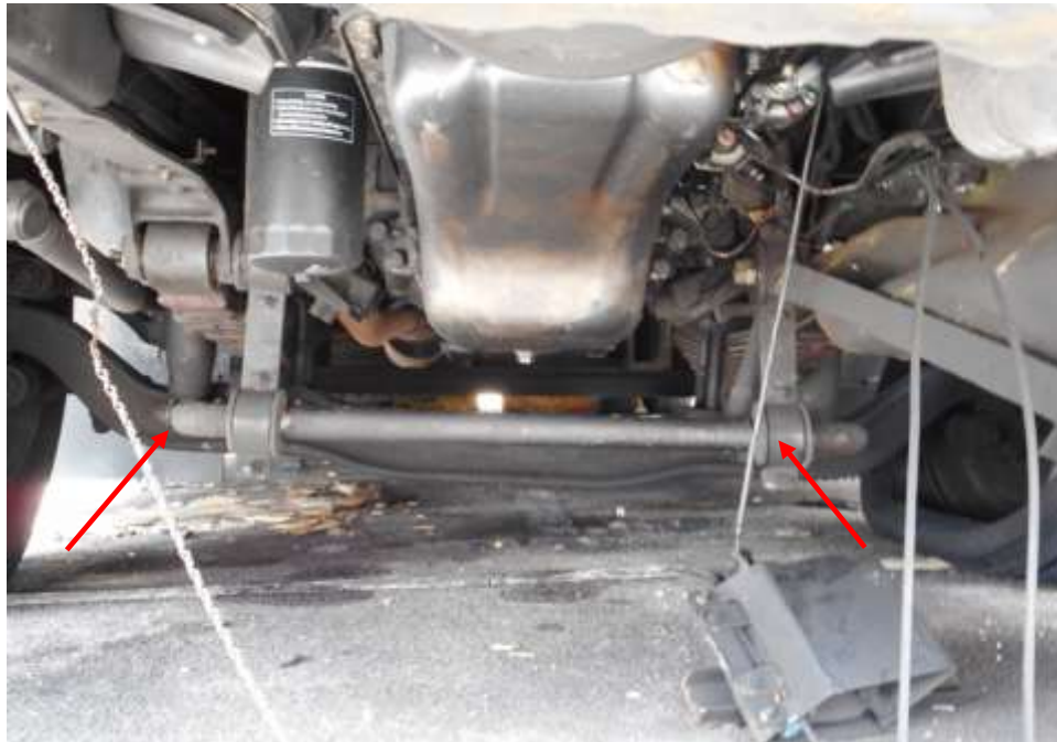
Photo 26 shows some of the mechanical components (arrowed) of the Motor Bus's steering system. The steering system of the Motor Bus shows to be intact and is likely to be in serviceable condition at the time of accident.
