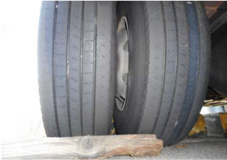
Photo 19 shows the condition of the rear right tyre of the Motor Bus, which was observed to be in serviceable condition with remaining tread depth of approximately 10.4mm. The tyre was also observed to be sufficiently inflated for vehicular operation.
