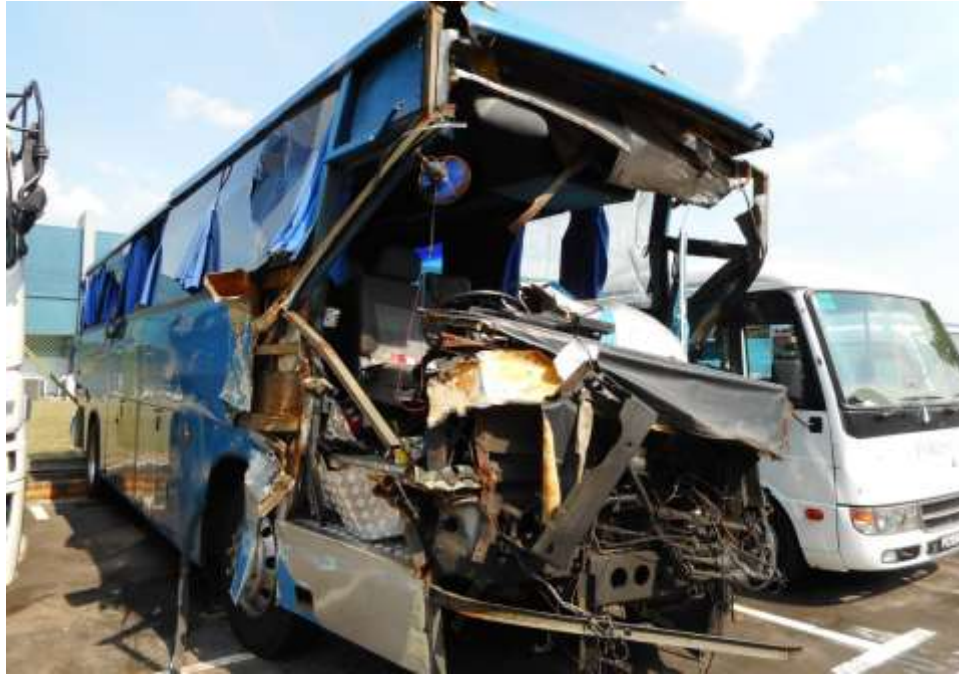
Photo 4 shows a general view of the front right side body of the Motor Bus at the time of our inspection. The Motor Bus was observed to have sustained extensive damages at its front right portion as a result of the accident's collision.
