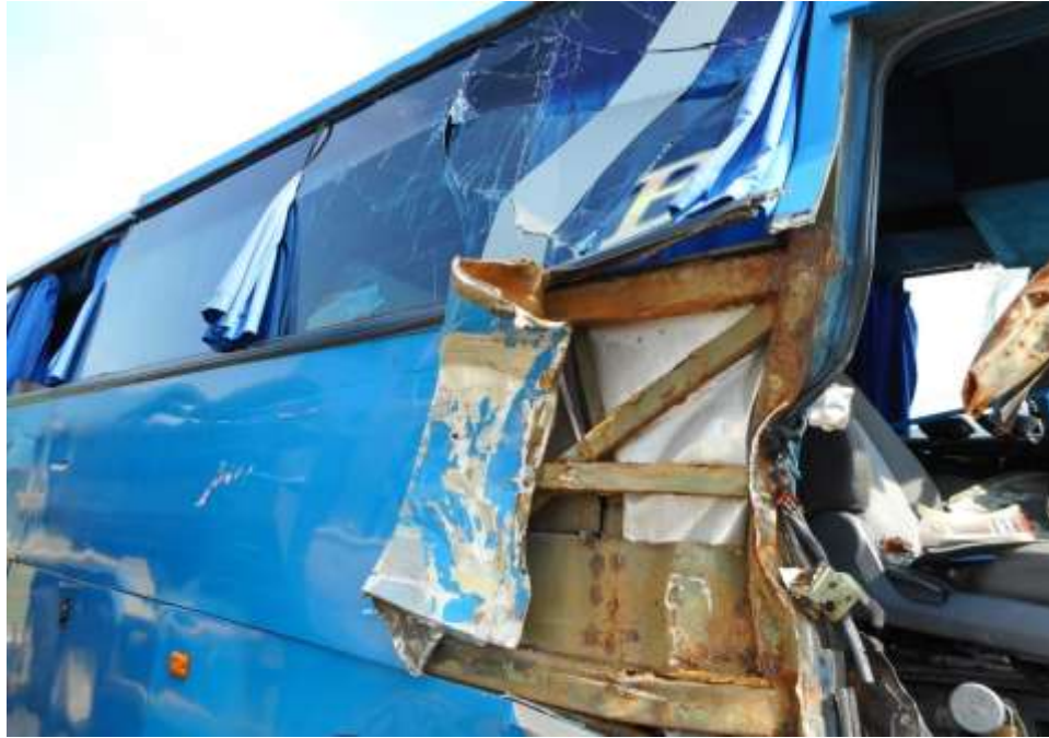
Photo 6 shows a close up view of the right side body of the Motor Bus at the time of our inspection. The Motor Bus was observed to have sustained extensive damages at its front portion as a result of the accident's collision.
