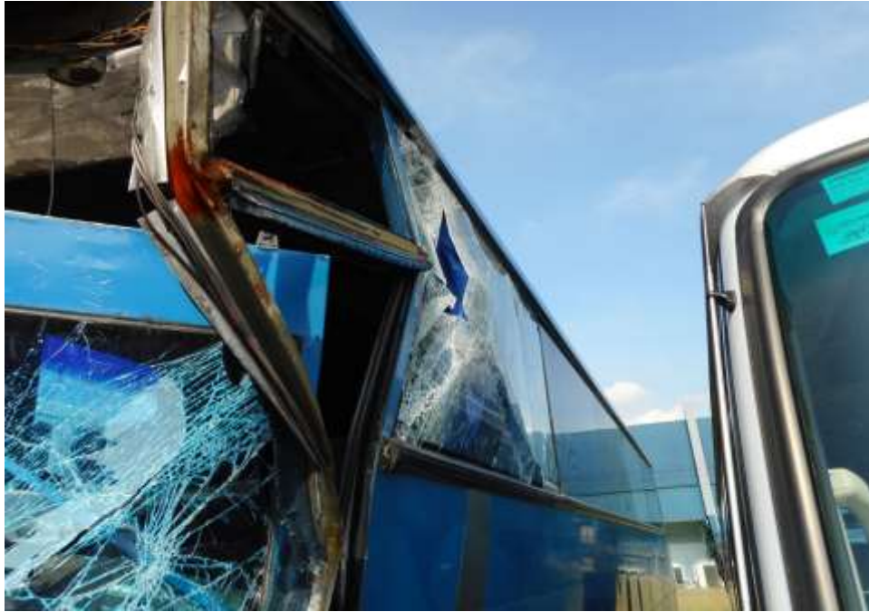
Photo 12 shows a close up view of the left side body of the Motor Bus at the time of our inspection. The Motor Bus was observed to have sustained extensive damages at its side windscreen as a result of the accident's collision.
