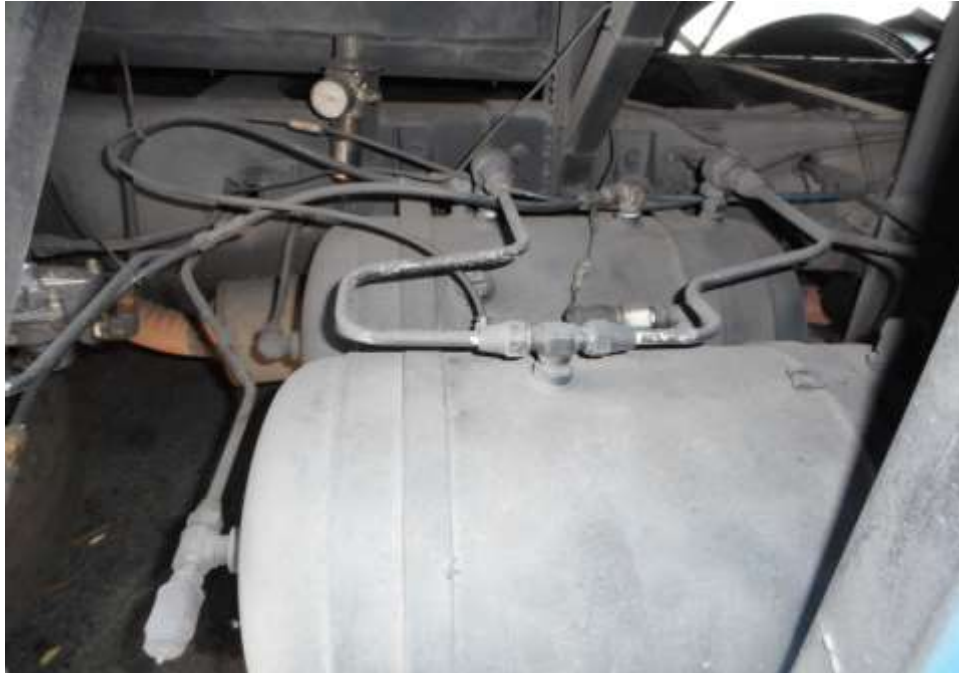
Photo 32 shows a close up view of first and second air cylinders, valves and hoses of the air-assisted braking system of the Motor Bus. This was at the underside of the Motor Bus's body. There were no damages observed at time of our inspection.
