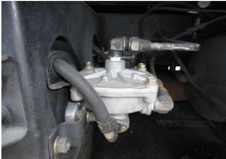
Photo 31 shows some of the Air-brake relay unit of the Motor Bus's braking system (including hoses). Visual check on the mechanical components shows that it was in serviceable condition at the time of accident.
