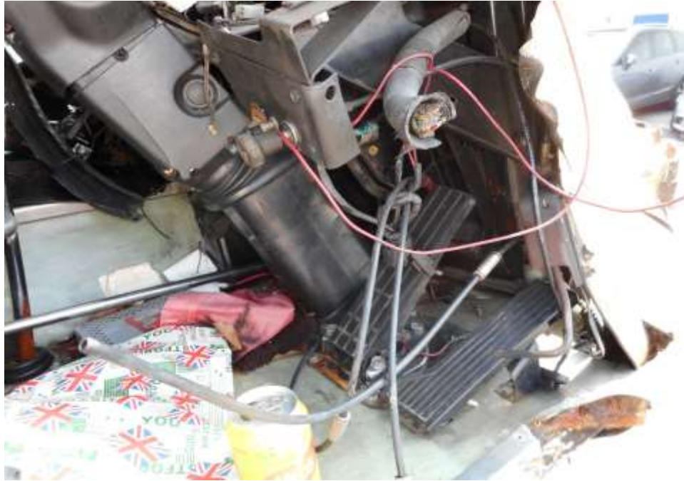
Photo 8 shows a close up view of the driver's foot well and its various driver systems at the time of our inspection and was observed to have sustained extensive damages, the operational road testing and electronics systems check of motor bus is immobilized as a result of the accident's collision.
