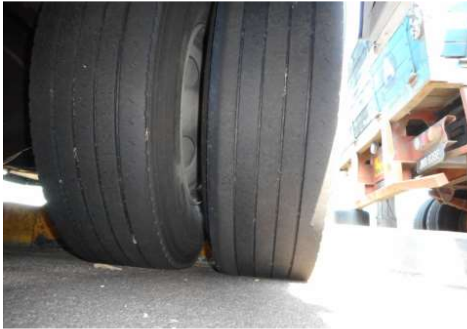
Photo 21 shows the condition of the rear right tyres of the Motor Bus, which were observed to be in serviceable condition with remaining tread depth of approximately 5.9mm. The tyres, which were wrapped around standard alloy wheel rims, were also observed to be sufficiently inflated for vehicular operation.
