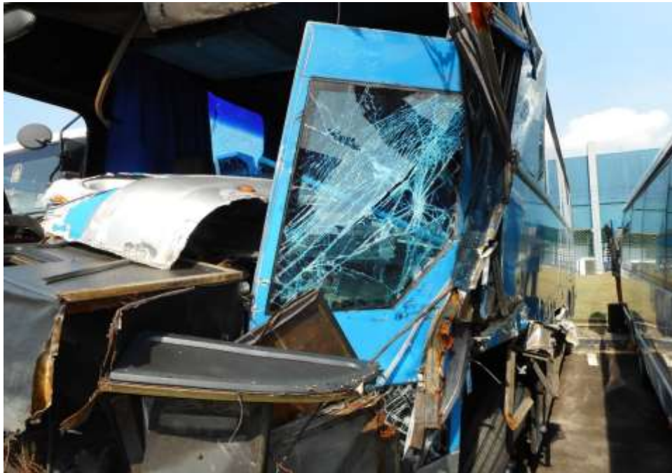
Photo 10 shows a close up view of the front and left side body of the Motor Bus at the time of our inspection. The Motor Bus was observed to have sustained extensive damages at its front entry/exit door upper portion as a result of the accident's collision.
