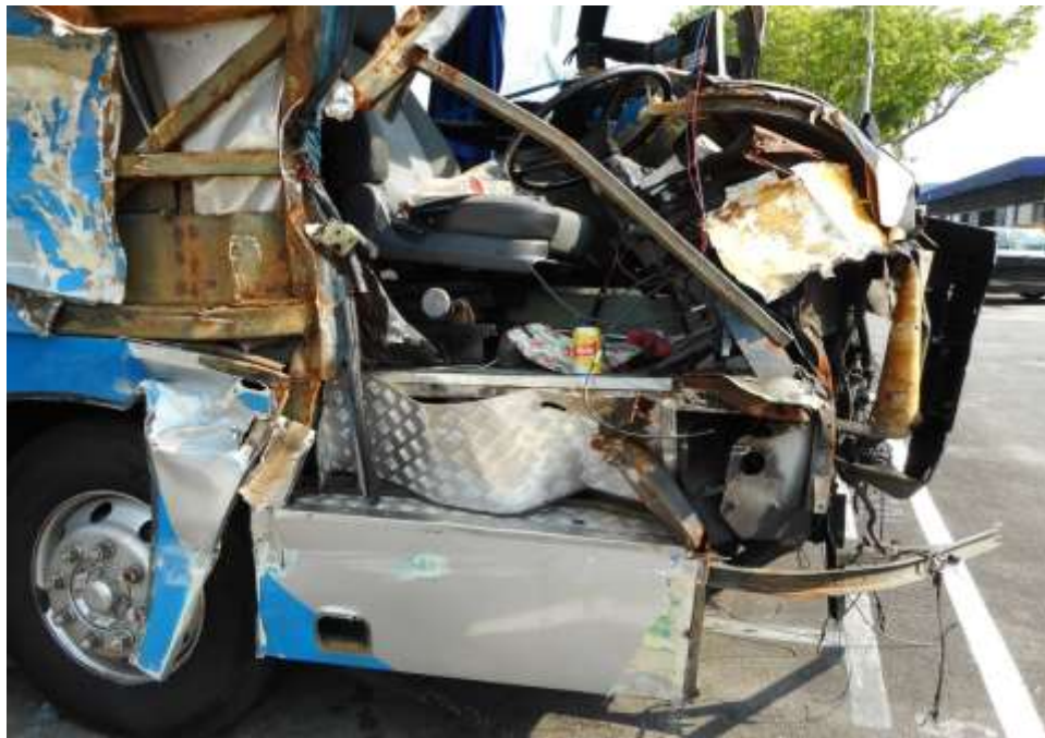
Photo 5 shows a close up view of the front right side body of the Motor Bus at the time of our inspection. The Motor Bus was observed to have sustained extensive damages at its front portion as a result of the accident's collision.
