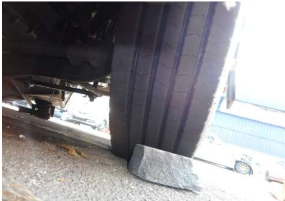
Photo 18 shows the condition of the front right tyre of the Motor Bus, which was observed to be in serviceable condition with remaining tread depth of approximately 14.2mm. The tyre was also observed to be sufficiently inflated for vehicular operation.
