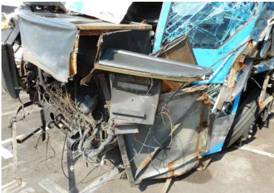
Photo 11 shows a close up view of the front and left side body of the Motor Bus at the time of our inspection. The Motor Bus was observed to have sustained extensive damages at its front entry/exit door lower portion as a result of the accident's collision.
