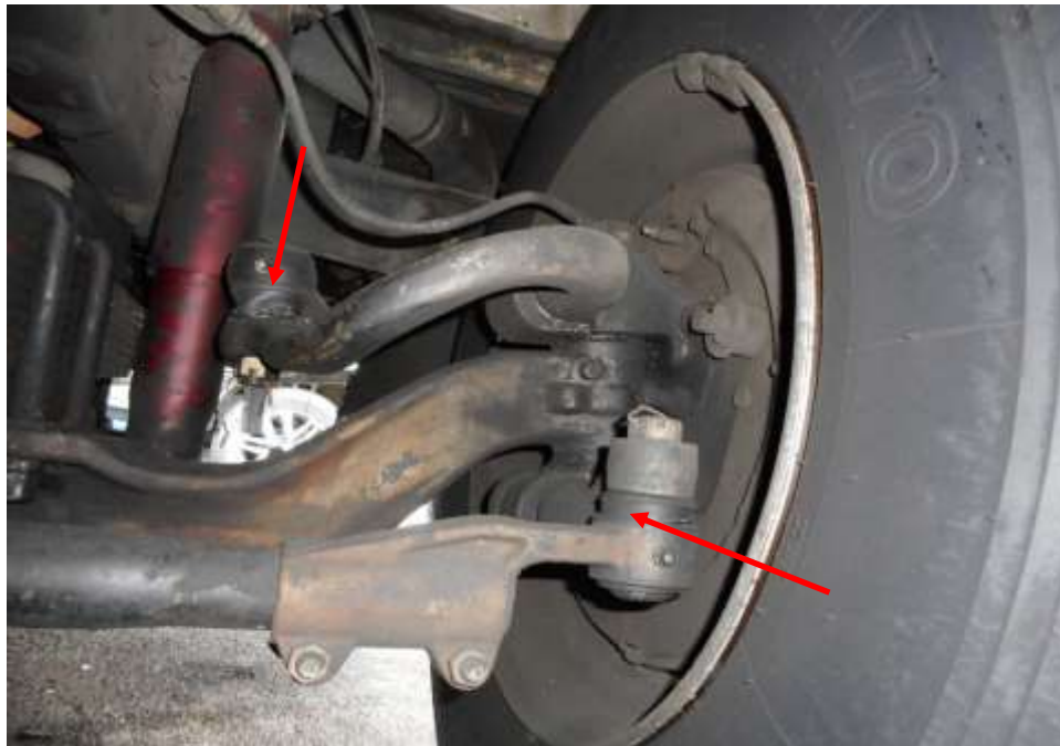
Photo 27 shows the front right wheel components of the front steering system of the Motor Bus. The various undercarriage components of the Motor Bus were all observed to be intact and without any visible damage. This had included the steering rack and steering ball joints (arrowed) of the Motor Bus, which were observed to be securely attached to the front right wheel.
