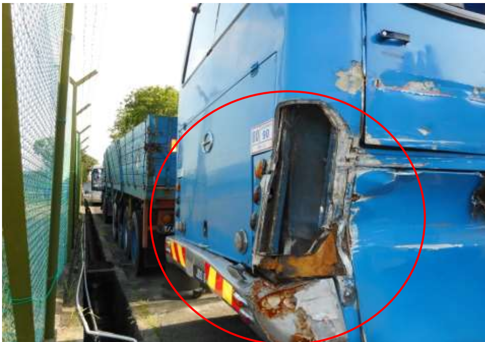
Photo 17 shows a general view of the rear right portion (circled) of the Motor Bus at the time of our inspection. The Motor Bus was observed to sustained extensive damages at its rear right portion as a result of the accident's collision.
