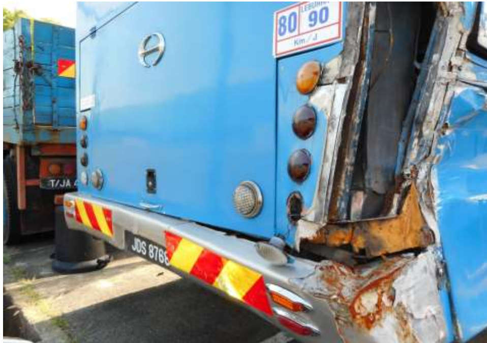
Photo 18 shows a close up view of the rear right portion of the Motor Bus at the time of our inspection. The Motor Bus was observed to sustained extensive damages at its rear right portion as a result of the accident's collision.
