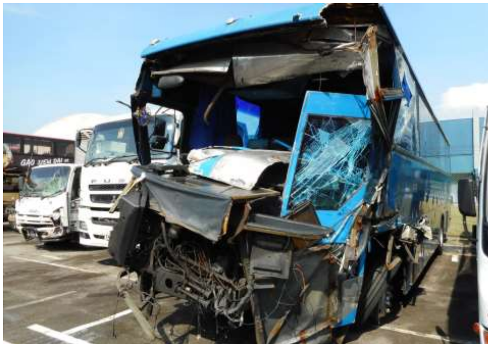
Photo 9 shows a general view of the front & left side body of the Motor Bus at the time of our inspection. The Motor Bus was observed to have sustained extensive damages at its side portion as a result of the accident's collision.
