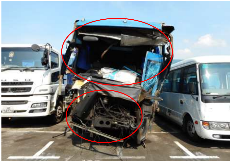
Photo 2 shows a general view of the front body of the Motor Bus at the time of our inspection. The Motor Bus was observed to have sustained extensive damages at its front portion and its entire front windshield (circled) was observed to be shattered and pushed inwards towards the rear as a result of the accident's collision.
