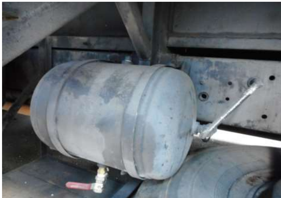
Photo 33 shows a close up view of the third air cylinder, valves and hoses of the air-assisted braking system of the Motor Bus. This was at the underside of the Motor Bus's body. There were no damages observed at time of our inspection.
