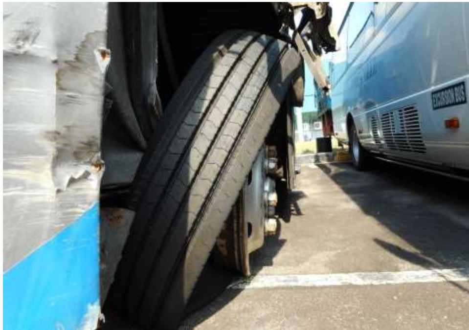
Photo 20 shows the condition of the front left tyres of the Motor Bus, which were observed to be deflated and dislodged from the rims likely due to the impact caused by the accident. With remaining tread depth of approximately 14mm.
