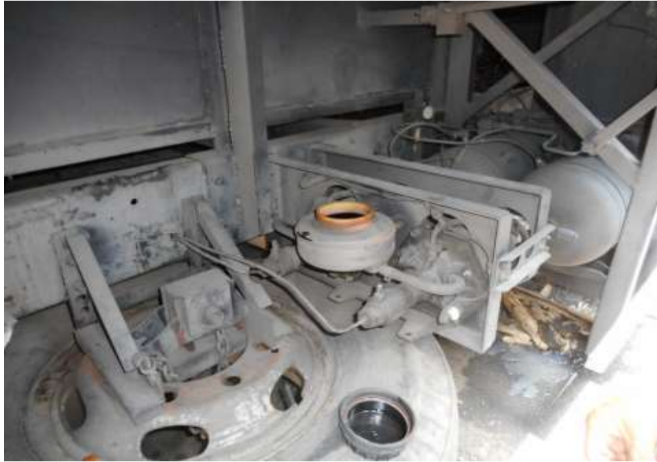
Photo 30 shows a general view of the air tank, valves, pipes and hoses, which are some of the components for the air-assisted braking system of the Motor Bus. This was at the underside of the Motor Bus's body. There were no damages observed at time of our inspection.
