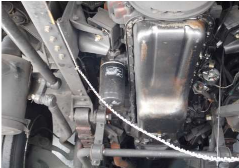
Photo 24 shows the engine undercarriage of the Motor Bus. No leakage or fluids was observed at time of our inspection.
