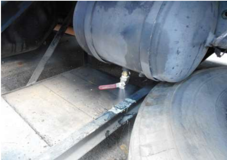
Photo 34 shows the release of residue air in cylinder indicating the air-cylinder was in serviceable condition during time of our inspection.
