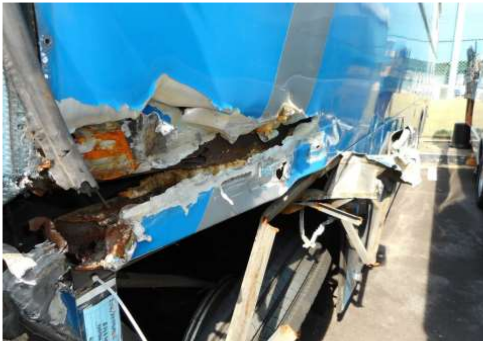
Photo 13 shows a close up view of the left side body of the Motor Bus at the time of our inspection. The Motor Bus was observed to have sustained extensive damages at its side wheel arch portion as a result of the accident's collision.
