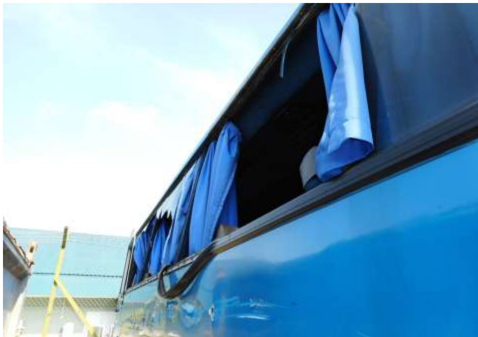
Photo 15 shows a close up view of the rear windscreen of the Motor Bus at the time of our inspection. The Motor Bus was observed to have sustained extensive damages at sections of its side windscreen and body panel portion as a result of the accident's collision.
