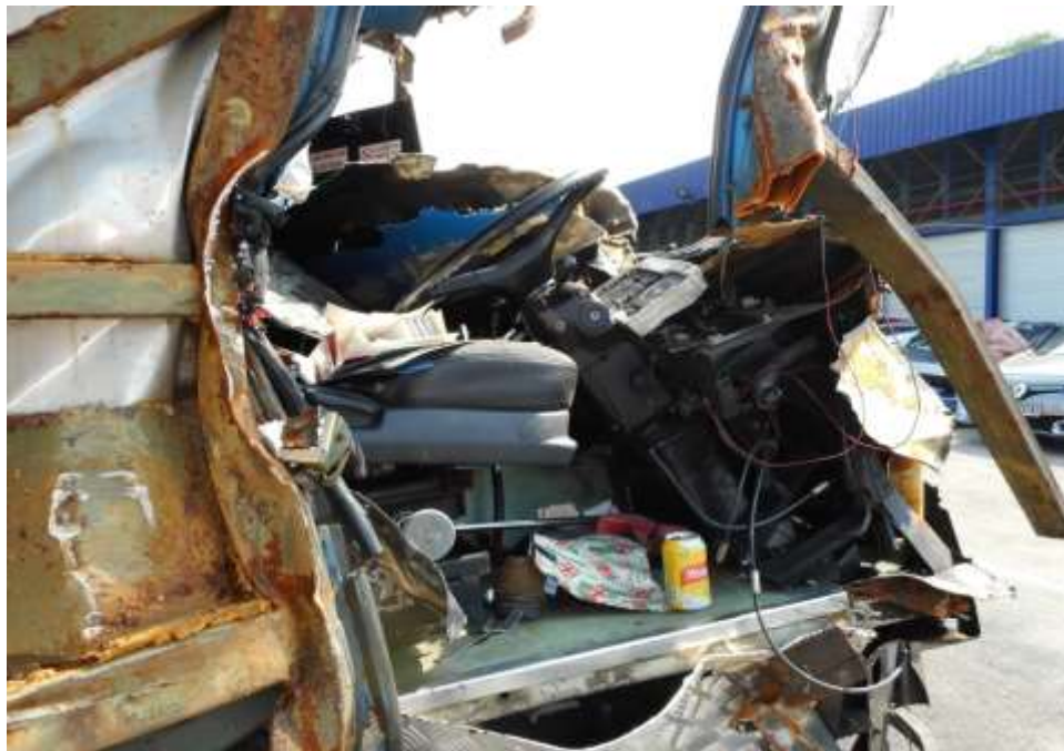
Photo 7 shows a close up view of the driver's cabin and its various driver systems at the time of our inspection and was observed to have sustained extensive damages, the operational road testing and electronics systems check of motor bus is immobilized as a result of the accident's collision.
