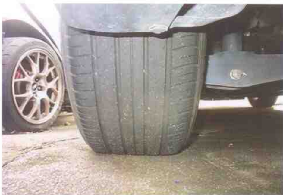
Photo 8 shows the condition of the rear left tyre of the Motor Car, which was observed to be in serviceable condition with remaining tread depth of approximately 4mm. The tyre, which was wrapped around alloy wheel rim, was also observed to be sufficiently inflated for vehicular operation. There was also no damage found on the 4 wheel rims of the Motor Car.
