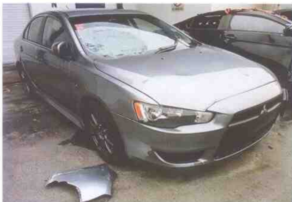
Photo 2 shows a general view of the front right body of the Motor Car at the time of our inspection. The Motor Car was observed to be in good general condition. However we had observed relatively minor impact damage that was confined to its right frontal portion. Its front bonnet was observed to have been dented; its front bumper was observed to be deformed while its front windscreen was observed to be cracked.
