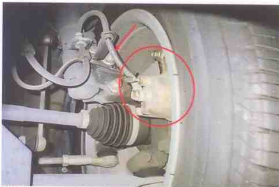
Photo 16 shows the brake hose/pipe (arrowed) at the front left wheel of the Motor Car. No leakage of brake fluid was observed. Visual examination of the various components of the braking system like the brake caliper (circled), brake pedal etc. had revealed all to be intact and without visible damage.
