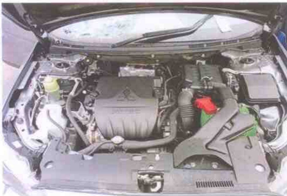
Photo 10 shows a general view of the Motor Car's engine compartment. The various parts and components inside the engine compartment were unaffected by the accident. There was also no sign(s) or indication(s) of fluid leakage and/or fluid stain within the engine compartment.
