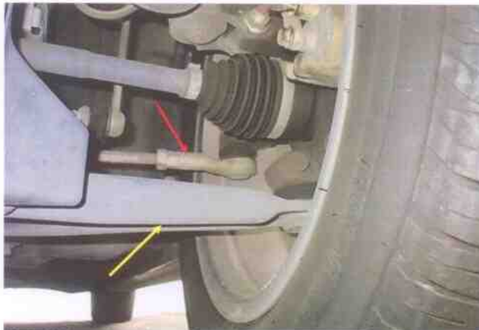
Photo 18 shows the various undercarriage components at the front left wheel of the Motor Car, which had included the steering tie rod (red arrow) and left drive shaft (yellow arrow). The various undercarriage components of the Motor Car were all found to be intact without any visible damage.
