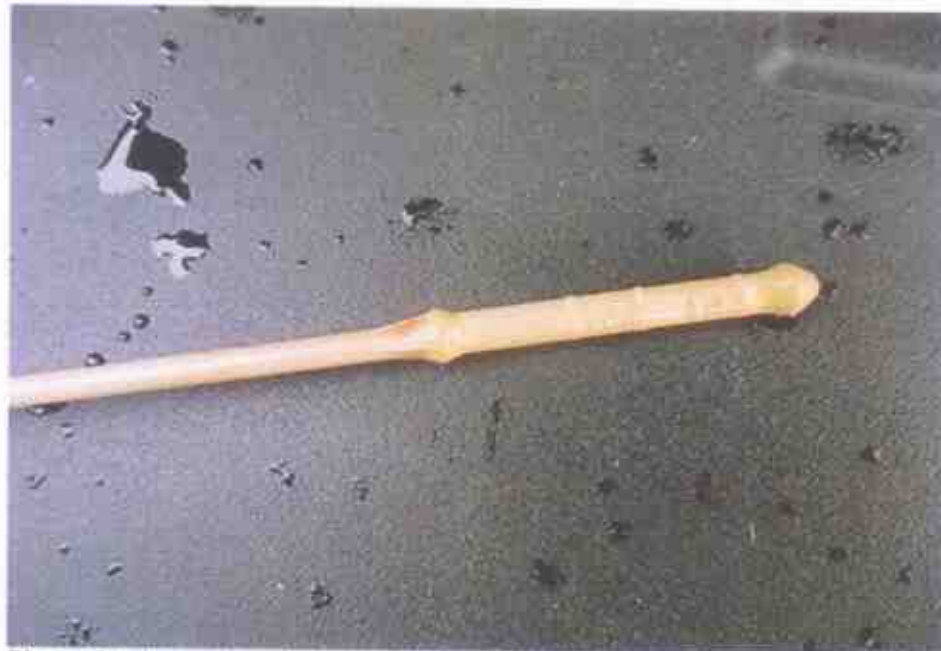
Photo 14 shows the auto transmission fluid (ATF) dip stick of the Motor Car at the time of our inspection. The ATF was observed to be of sufficient level and without any visible contamination.
