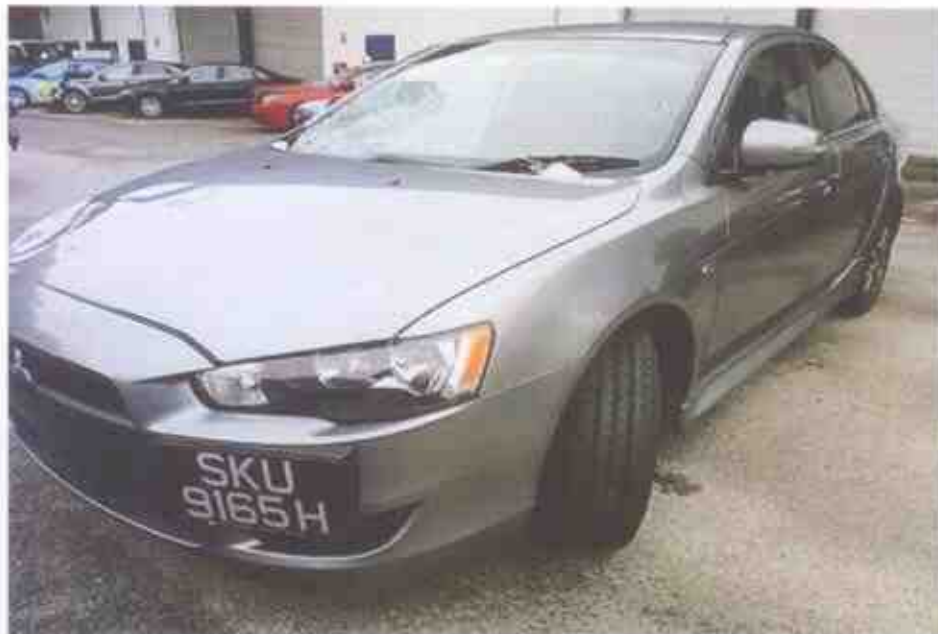
Photo 19 shows the front left wheel of the Motor Car turned to its full left. During our steering system test, we did not experience any abnormal free play and/or resistance when we had turned the steering wheel towards the left and right. This would suggest that the steering system of the Motor Car was likely to be in serviceable condition at the material time of accident.
