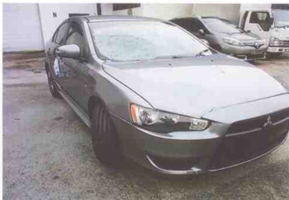
Photo 20 shows the front right wheel of the Motor Car turned to its full right. During our steering system test, we did not experience any abnormal free play and/or resistance when we had turned the steering wheel towards the left and right. This would suggest that the steering system of the Motor Car was likely to be in serviceable condition at the material time of accident.
