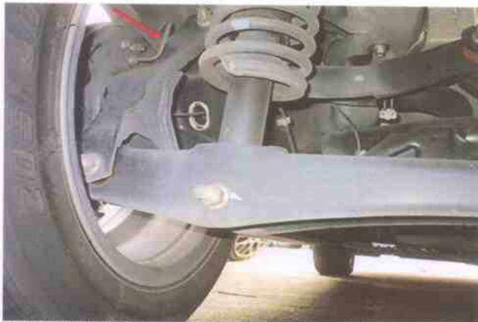
Photo 15 shows the brake hose/pipe (arrowed) at the rear left wheel of the Motor Car. We did not observe any leakage of brake fluid at the time of our inspection of the Motor Car. Static tests of the Motor Car's braking system had indicated that there was no internal leakage of pressure/vacuum. Hence the braking system was likely to be in serviceable condition at the material time of accident. The undercarriage components of the Motor Car were also all found to be intact and without any visible damage.
