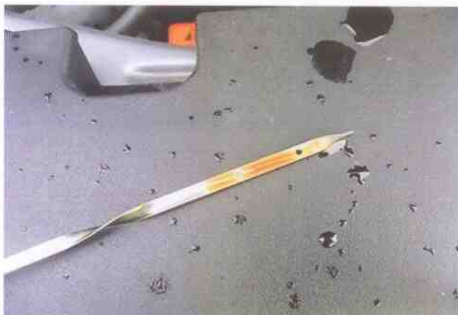
Photo 13 shows the engine oil dip stick of the Motor Car at the time of our inspection. The engine oil was observed to be of sufficient level and without any visible contamination.
