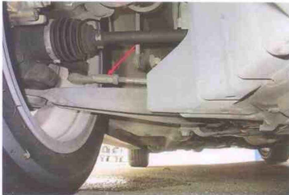
Photo 17 shows the various undercarriage components at the front right wheel of the Motor Car, in particular the steering tie rod (arrowed). The various steering components were all found to be intact, suggesting that the steering system of the Motor Car was likely to be in serviceable condition at the material time of accident. There was also no sign of fluid stain observed on the various undercarriage components at the front right wheel of the Motor Car.
