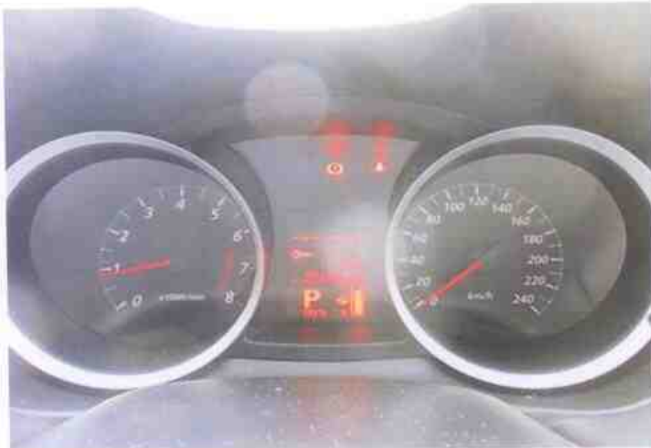
Photo 22 shows no warning lights illuminated on the instrument panel of the Motor Car after the engine was cranked. This would suggest that there was no abnormality to the various electronic operating systems of the Motor Car, like the ABS and SRS etc.
