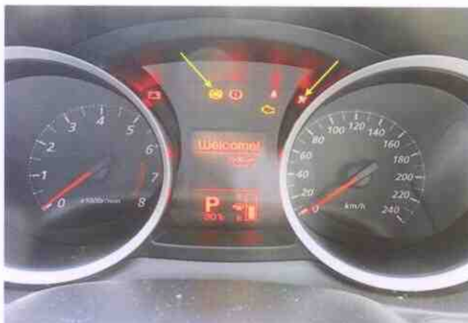
Photo 21 shows the warning lights for the various electronic operating systems of the Motor Car appearing on its instrument panel during the self-test when the engine is cranked, in particular the ABS light and SRS light (arrowed).
