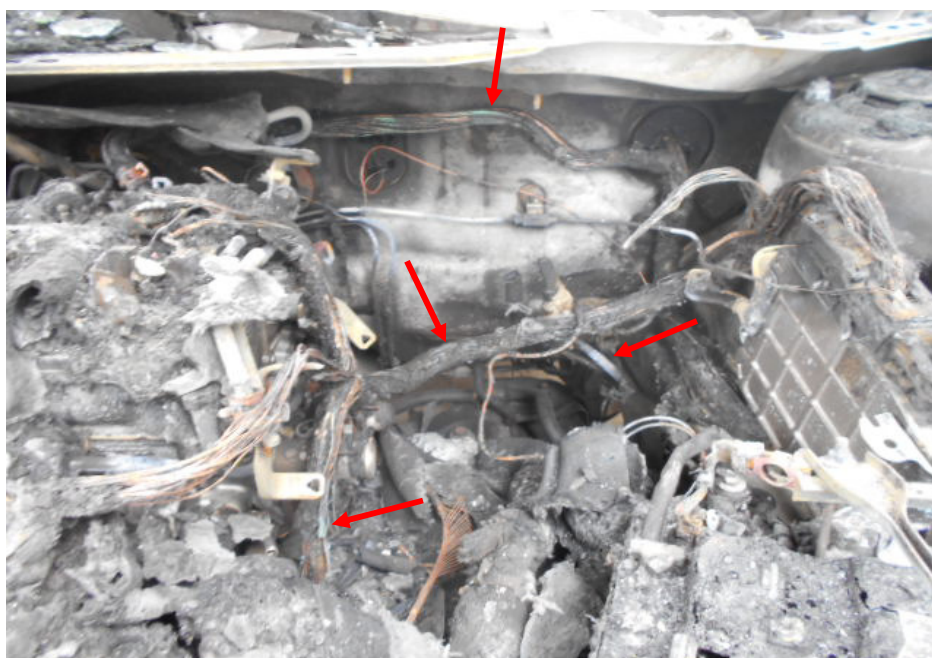
Photo 12 shows the wirings around the centre left area of the engine compartment, which was where the fire to the Insured Vehicle had originated. Greenish residue was found on several stretches of wirings (arrowed). These wirings were originally fitted wirings. The presence of such greenish residue suggests occurrence of an electrical short circuit.
