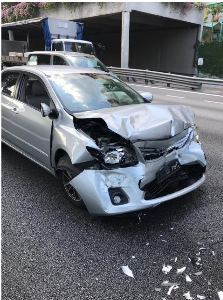
Photo 8 shows a general view of the Insured Vehicle at the accident scene along PIE towards Changi Airport. From my review of the photographs provided by Mr Lim, I note that the Insured Vehicle had sustained impact damage at its frontal portion. There was no damage of fire nature seen on the Insured Vehicle at the accident scene. There was also no leaked fluid seen on the road surface where the Insured Vehicle had come to a stop.
