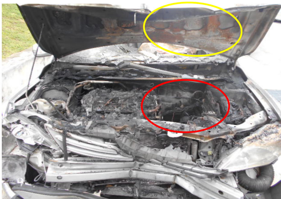
Photo 11 shows a general view of where the fire to the Insured Vehicle had originated, which was around the centre left area of the engine compartment (red circle). This was established basing on the burn pattern (whitish burn marks and rust) that was found on the top side and the underside (yellow arrow) of the Insured Vehicle's front bonnet.
