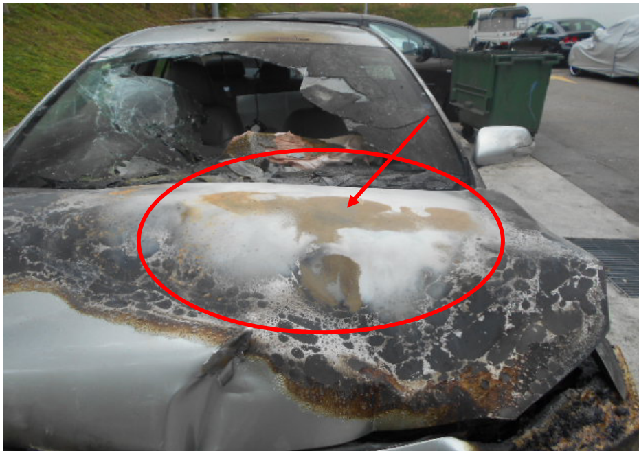
Photo 10 shows the whitish burn marks (circled) that were found on the centre left area of the Insured Vehicle's front bonnet. Such whitish burn marks are a result of exposure to prolonged heat intensity. Rust (arrowed) would normally start to develop around these areas soon after a fire as prolonged exposure to high heat intensity usually causes steel/metal material body parts to be exposed to natural environmental condition. Following the characteristic of heat rising upwards, the fire to the Insured Vehicle can then be determined to have originated around the centre left area of the engine compartment.
