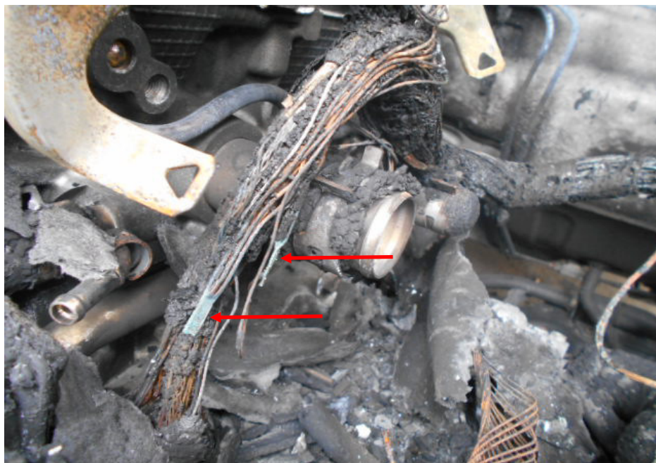
Photo 15 shows another stretch of wirings with greenish residue (arrowed) at the centre left area of the Insured Vehicle's engine compartment. The physical condition of the wirings as seen during my inspection of the Insured Vehicle supports the cause of fire being due to electrical in nature.
