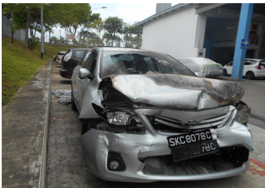
Photo 1 shows a general view of the front right portion of the Insured Vehicle at the time of my inspection. The fire damage to the Insured Vehicle was confined to its frontal portion. Its front bonnet and front windscreen were amongst the body parts that were found to have been affected as a result of the fire. Apart for the fire damage, the Insured Vehicle was also observed to have sustained impact damage at its frontal portion. Its front bumper, front fenders, front grille and front bonnet were all observed to have been damaged. The impact damage pattern suggests that the direction of impact was from the front to rear of the Insured Vehicle.
