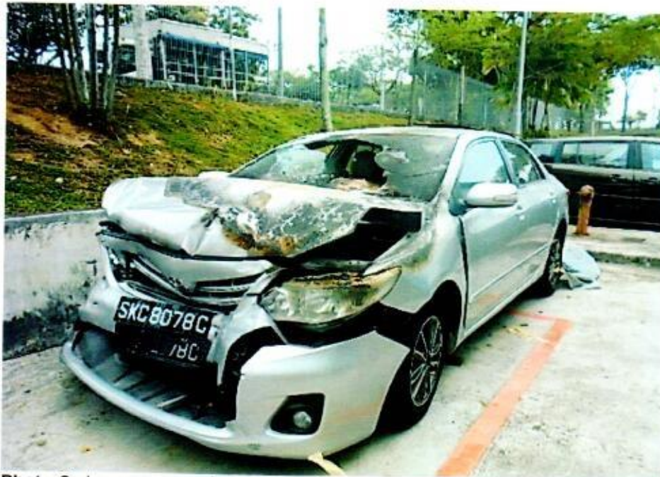
Photo 2 shows a general view of the front left portion of the Insured Vehicle at the time of my inspection. The fire damage to the Insured Vehicle was confined to its front portion. Its front bonnet, front left headlamp and front left fender were amongst the body parts that were found to have been affected as a result of the fire. Apart for the fire damage, the Insured Vehicle was also observed to have sustained impact damage at its frontal portion.
