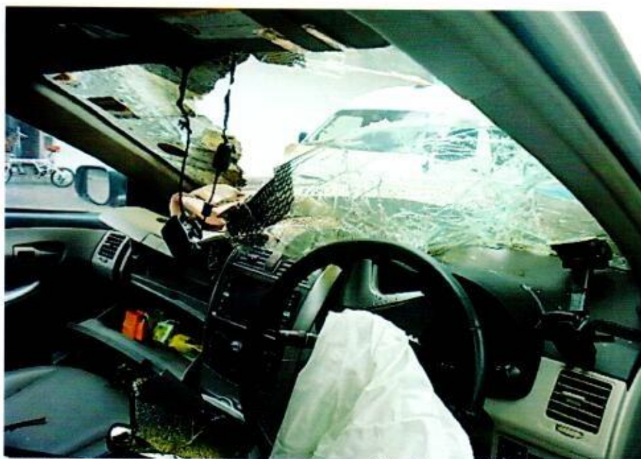
Photo 4 shows the interior compartment of the Insured Vehicle, which was observed to be partially burnt at the front area. The front dashboard and roof upholstery were amongst the parts that were found to have been burnt and/or melted as a result of the fire.
