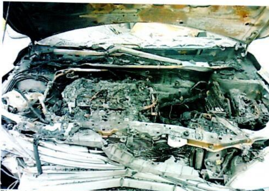
Photo 3 shows the engine compartment of the Insured Vehicle at the time of my inspection. The engine compartment of the Insured Vehicle was observed to be severely burnt. Most of the parts inside the engine compartment were found to be burnt and/or melted as a result of the fire.
