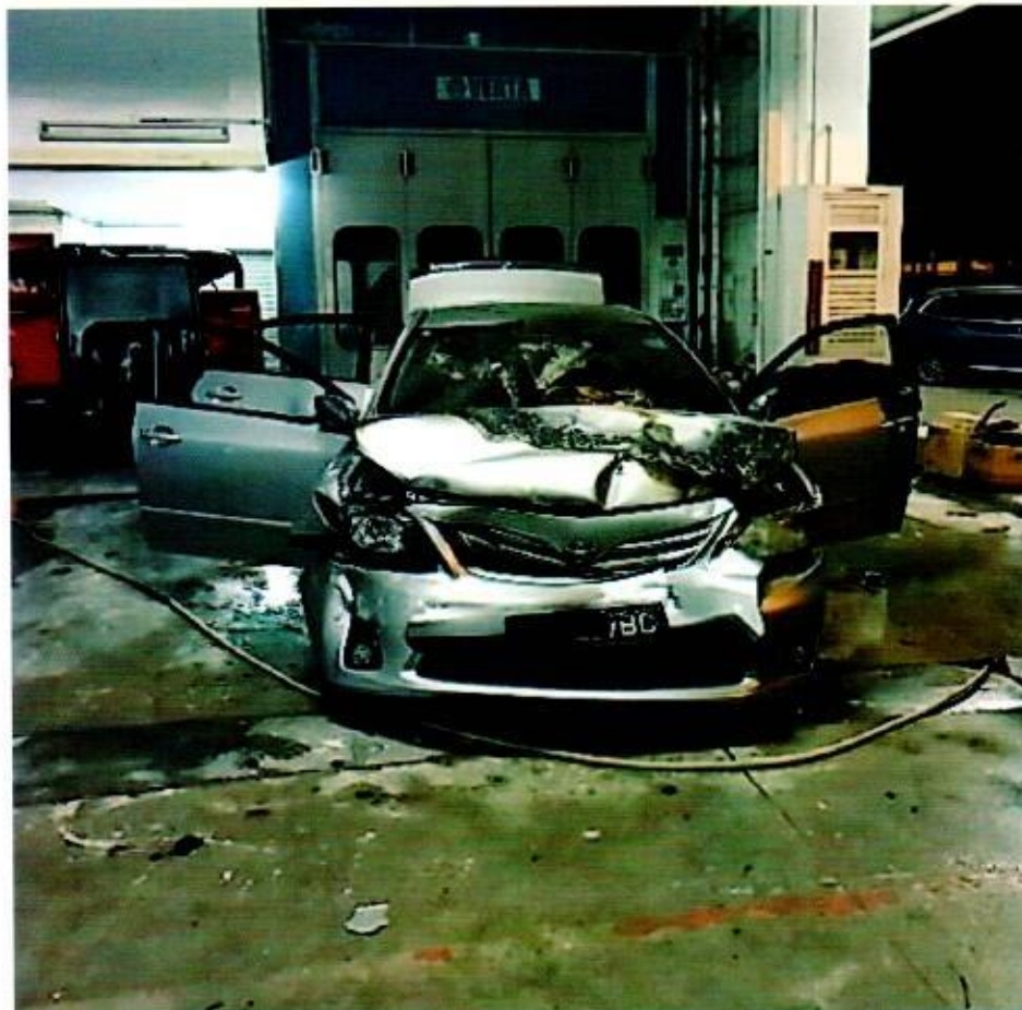
Photo 9 shows a general view of the Insured Vehicle at the premise of M/s Chin Meng Motors. This was after the fire was extinguished. Upon close examination of the photographs, there appears to be no unusual foreign material(s) and/or object(s) found on the ground in the immediate area of where the Insured Vehicle was parked.
