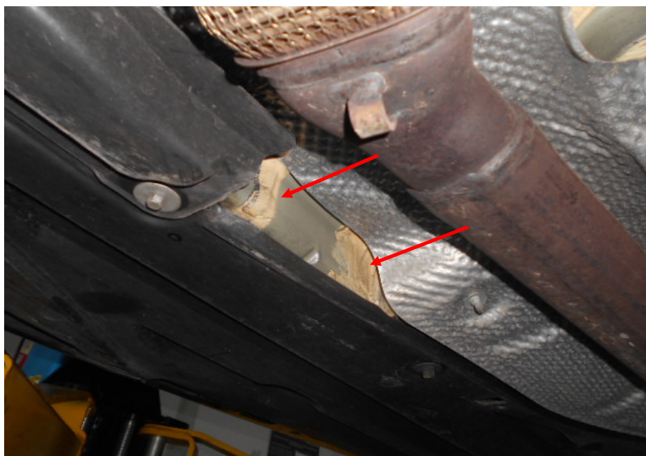
Photo 15 shows the structural body at the centre right underside of the Motor Car. The original factory sealant at the joints (arrowed) along the chassis body was untouched, indicating no work was done on the chassis body of the Motor Car and that the chassis body was originally fitted.
