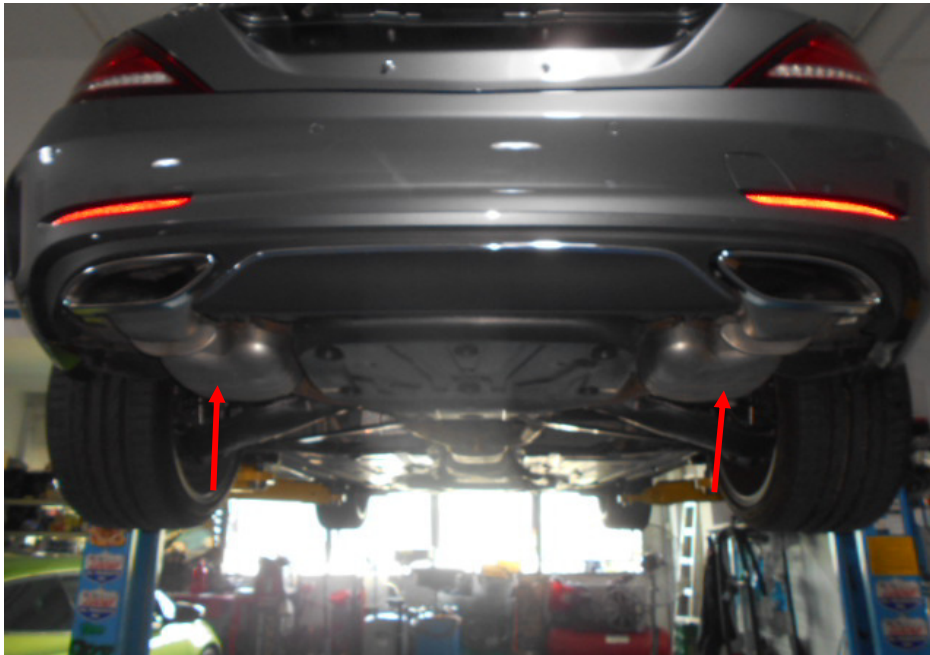
Photo 8 shows the Motor Car hoisted up for checks on its undercarriage. There was no sign(s) or indication(s) of fluid leakage and/or fluid stain(s) found on the underside of the Motor Car. The undercarriage components were all observed to be intact and secured in an appropriate manner. My examination of the Motor Car's exhaust system revealed no sign(s) or indication(s) of any cut or weld marks along its exhaust pipes and on its rear mufflers (arrowed).
