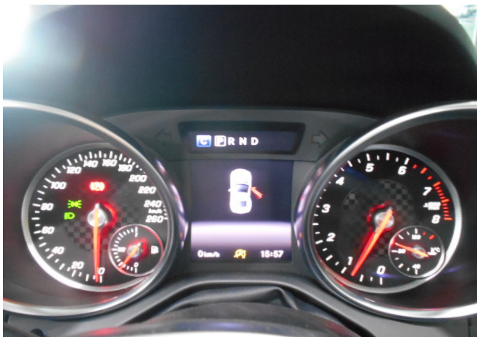
Photo 7 shows the respective warning lights no longer illuminated, indicating that there is no fault detected to the ABS, SRS, TPM and TCS systems of the Motor Car during the self-test. These electronic systems were hence in working condition at the time of my inspection.
