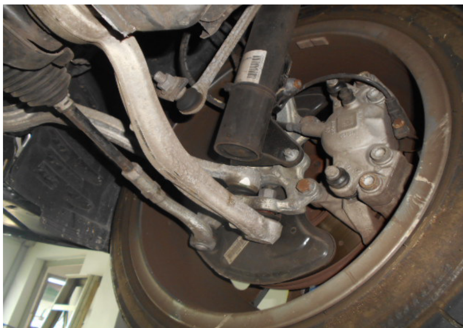
Photo 11 shows the various undercarriage components at the front right wheel of the Motor Car. The mechanical components, control arms and linkages were all found to be intact and secured in an appropriate manner. I did not observe any fluid leak and/or fluid stain on the underside of the Motor Car.
