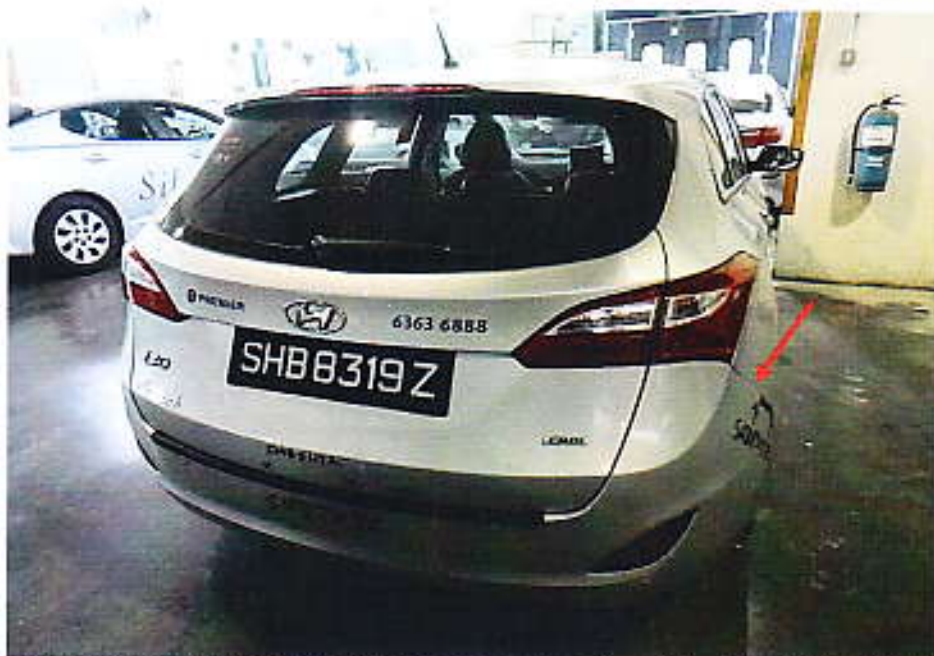
Photo 3 shows a general view of the rear right portion of the Third Party Vehicle at the time of inspection by LKK Auto Consultants Pte Ltd. The right side of the rear bumper (arrowed) was detached from its holding bracket.
