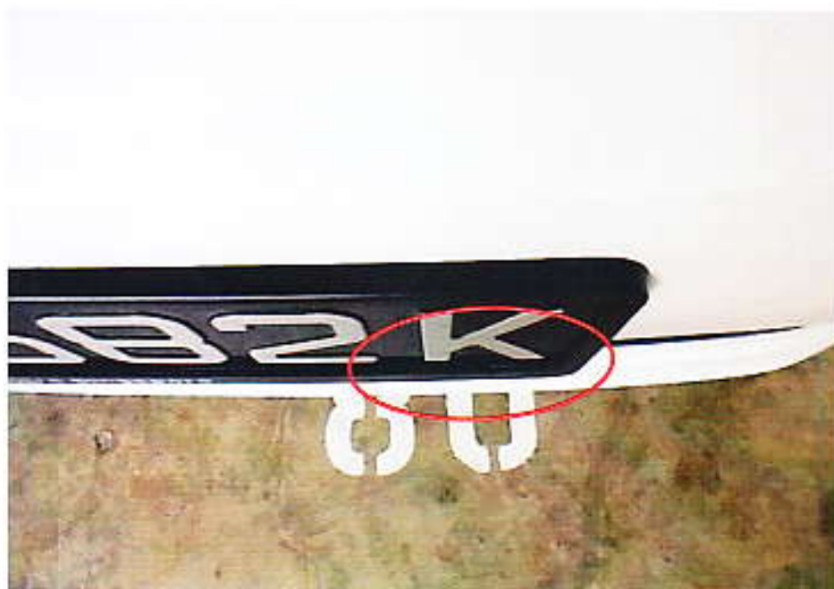
Photo 8 shows the front number plate and front number plate casing of the Insured Vehicle slightly bent inwards at a single area (circled). This was at the left bottom corner area.
