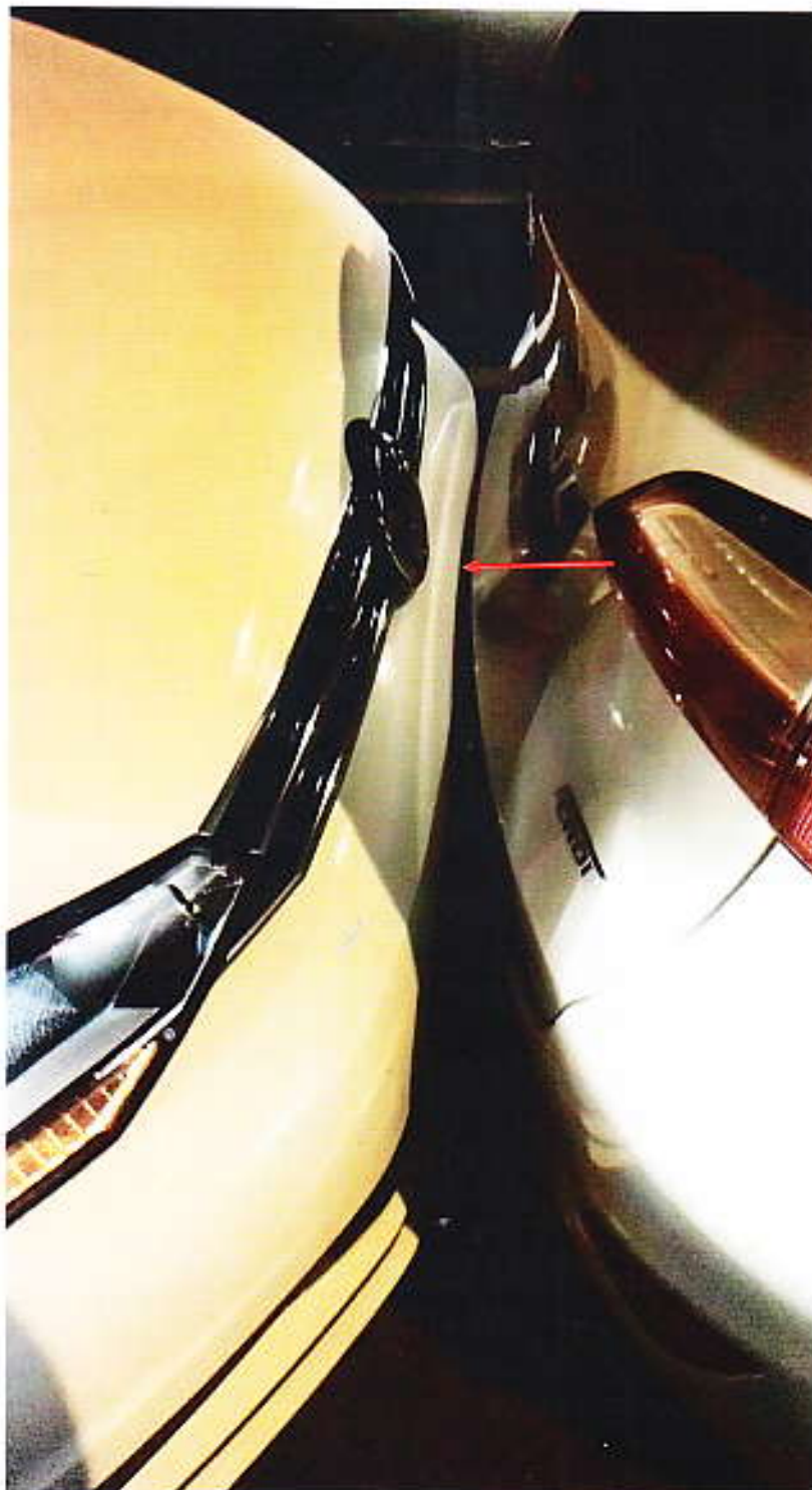
Photo 11 shows the Insured Vehicle and the Third Party Vehicle at the incident scene. The inward compression (arrowed) of the Insured Vehicle's front bumper, at the surface area directly below the radiator grille indicates that there was contact between the frontal portion of the Insured Vehicle and the rear portion of the Third Party Vehicle.
