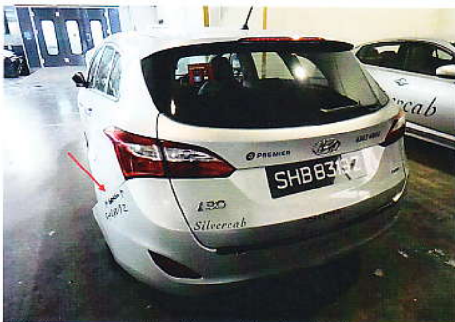
Photo 1 shows a general view of the rear left portion of the Third Party Vehicle at the time of inspection by LKK Auto Consultants Pte Ltd. The left side of the rear bumper (arrowed) was detached from its holding bracket.
