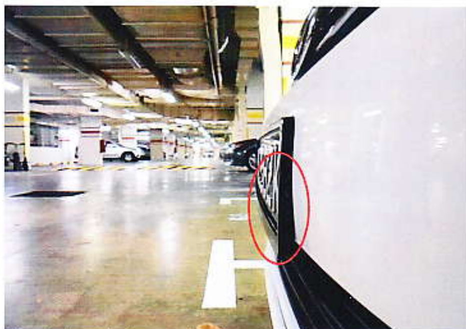
Photo 9 shows the front number plate and front number plate casing of the Insured Vehicle slightly bent inwards at a single area (circled). This was at the left bottom corner area. Apart from this, I did not observe any other visible damage to the frontal portion of the Insured Vehicle at the time of my inspection.
