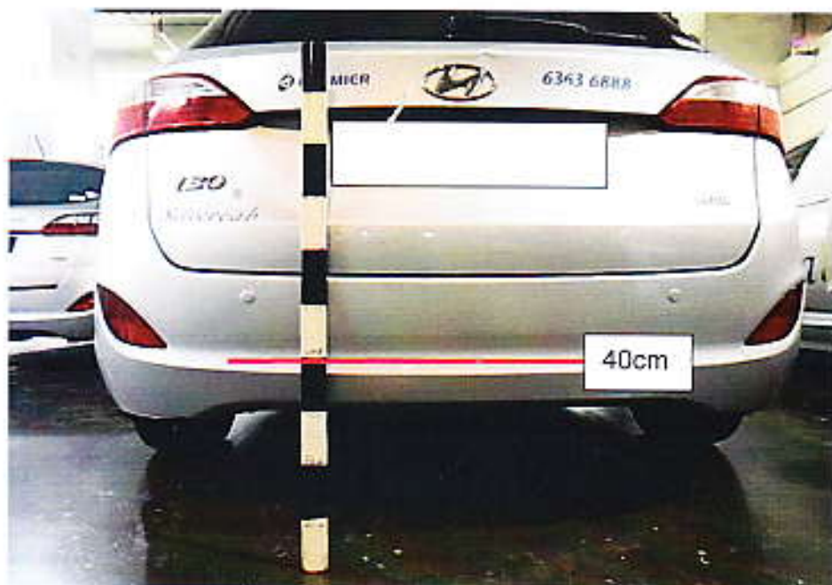
Photo 13 shows the height measurement that was conducted on the rear portion of a similar make and model vehicle as the Third Party Vehicle. 40cm above ground level, was at the area slightly above the curve shape of the rear bumper. The bottom of the vertical indentation of the Third Party Vehicle's rear bumper, shown in photograph 5 above, was also slightly above the curve shape of the rear bumper.
