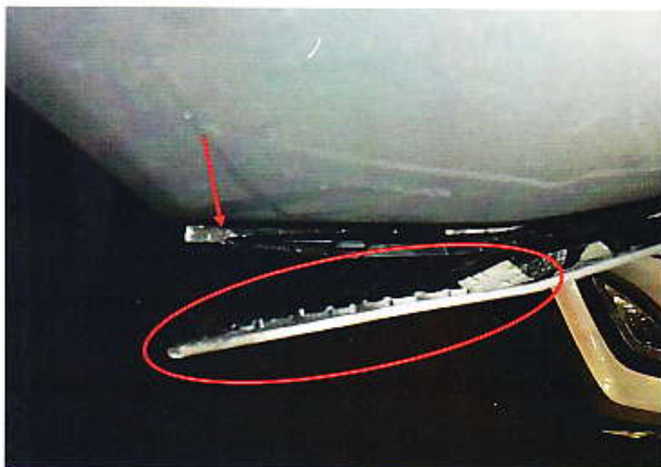
Photo 2 shows the mounting area at the left side of the rear bumper broken (circled and arrowed)
