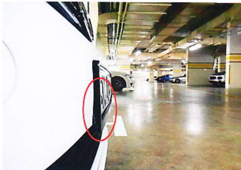
Photo 10 shows the front number plate and front number plate casing of the Insured Vehicle, at the right bottom corner area (circled) for comparison purposes with the left bottom area that was shown in photograph 9 above. The right side of the front number plate and front number plate casing is in an original curve shape whereas the same area at the left side was bent in comparison.
