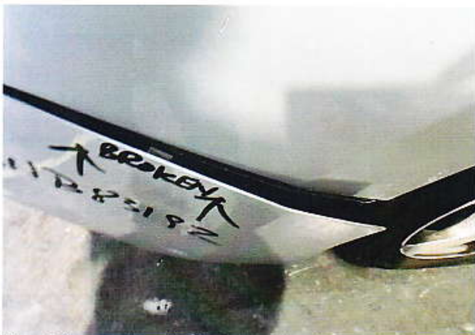
Photo 4 shows a closer view of the right side of Third Party Vehicle's rear bumper, which was detached from its holding bracket.
