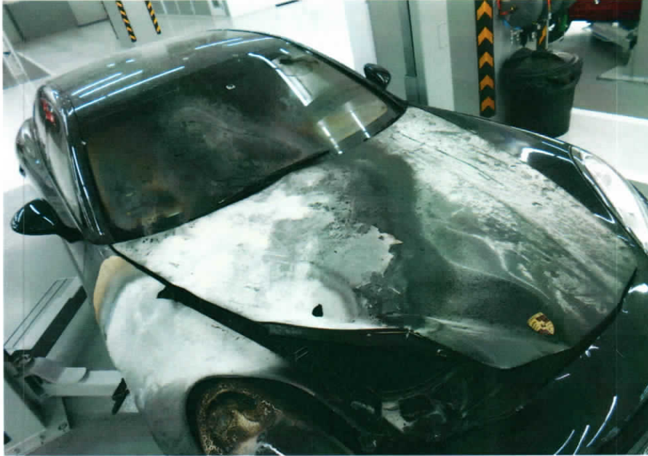
Photo 6 shows the burn pattern and whitish burn marks that were found on the topside of the front bonnet of the Insured Vehicle. Such whitish burn marks are a result of exposure to prolong heat intensity, which may indicate where the fire had started. Rust would also begin to develop on these areas soon after the fire.
