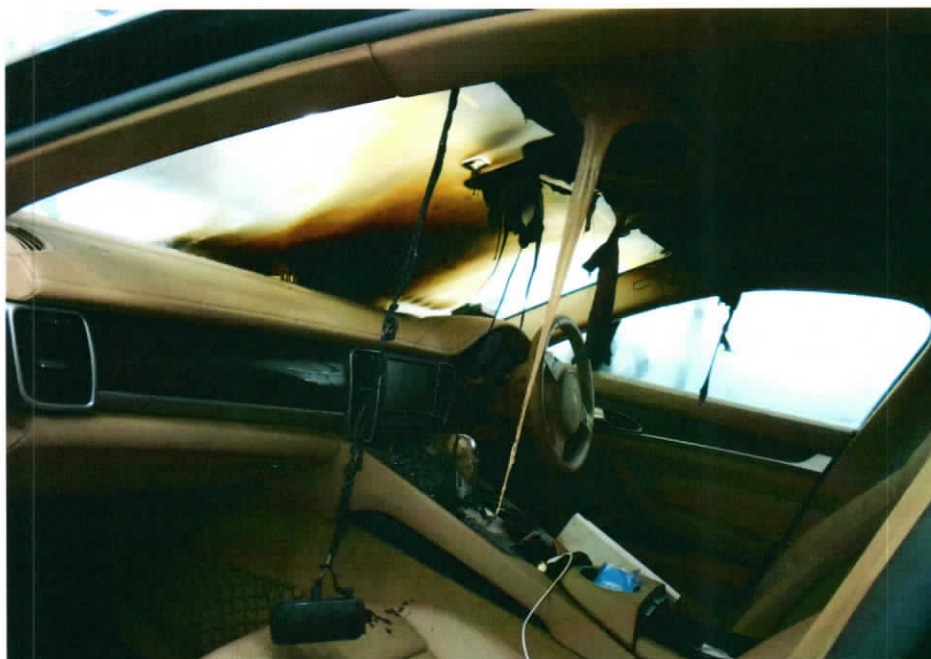
Photo 4 shows the interior compartment of the Insured Vehicle, which was observed to be affected by the fire incident. Burnt video camera was also noted to be dangling at time of our visit to the workshop.
