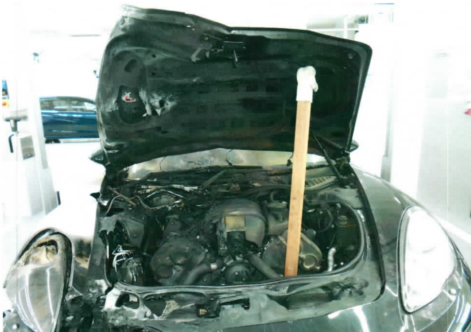
Photo 2 shows the general view of the front engine portion of the Insured Vehicle at the time of our inspection. The fire damage to the Insured Vehicle was confined to its front bonnet and most engine parts were amongst the body parts that were found to have been affected as a result of the fire.
