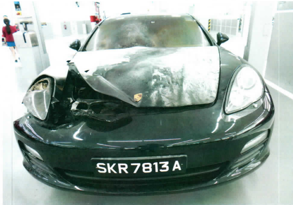
Photo 1 shows the general view of the Insured Vehicle at the time of our inspection. The fire damage to the Insured Vehicle was confined to its front bonnet and most engine parts were amongst the body parts that were found to have been affected as a result of the fire.
