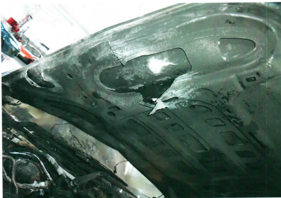
Photo 5 shows the burn pattern and whitish burn marks that were found on the underside of the front bonnet of the Insured Vehicle. Such whitish burn marks are a result of exposure to prolong heat intensity, which may indicate where the fire had started. Rust would also begin to develop on these areas soon after the fire.
