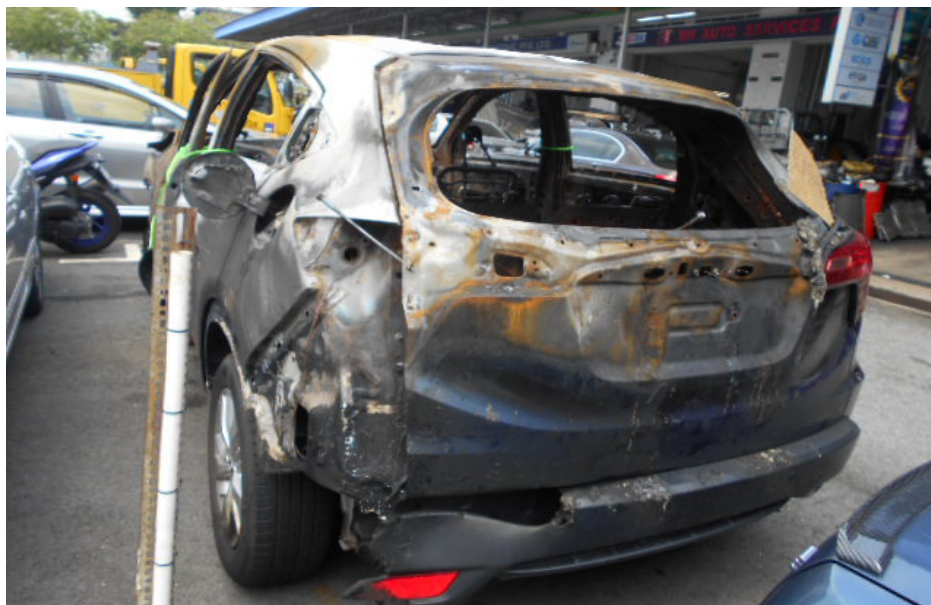
Photo 5 shows the rear left body of the Insured Vehicle. Comparing the overall extent of fire damage like the rear tyres vs the front tyres, condition of rear body panels vs front body panels etc, it would appear that the front body of the Insured Vehicle was more severely affected than its rear portion.
