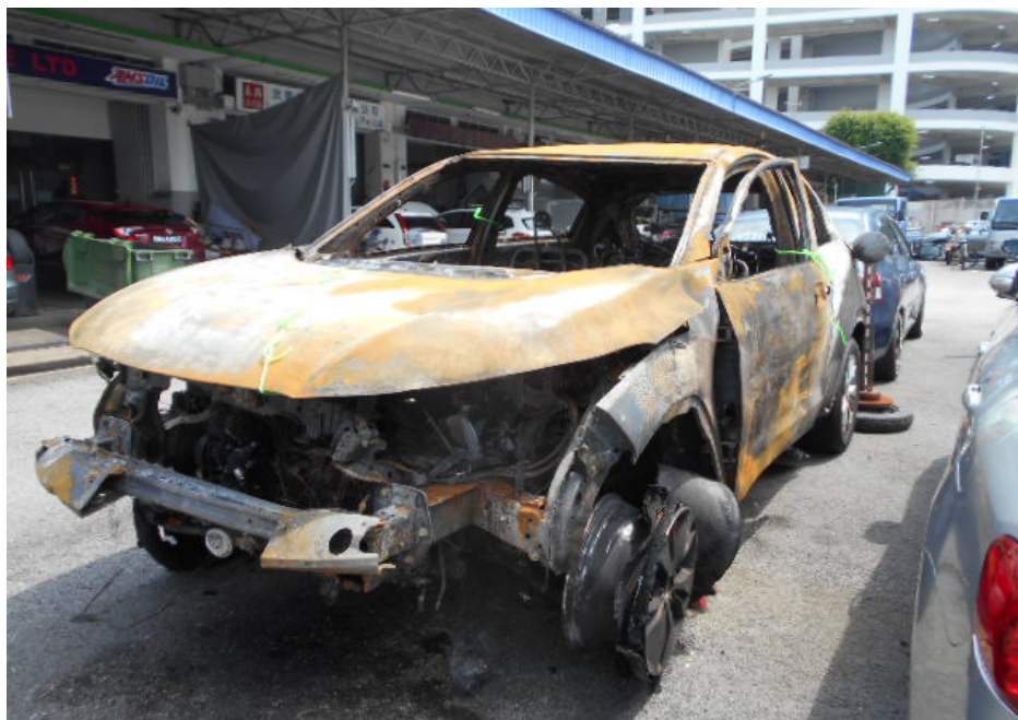
Photo 2 shows a general view of the front left body of the Insured Vehicle at the time of inspection. The Insured Vehicle was observed to have sustained extensive fire damage. The body panels at the front body like the front bonnet, front fenders, front door amongst others were all burnt to bare metal state.
