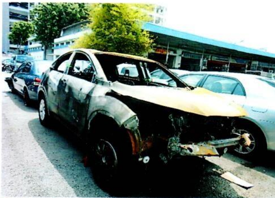
Photo 1 shows a general view of the front right body of the Insured Vehicle at the time of inspection. The Insured Vehicle was observed to have sustained extensive fire damage. The body panels at the front body and the undercarriage components at the front underside were all found to have been burnt to char.
