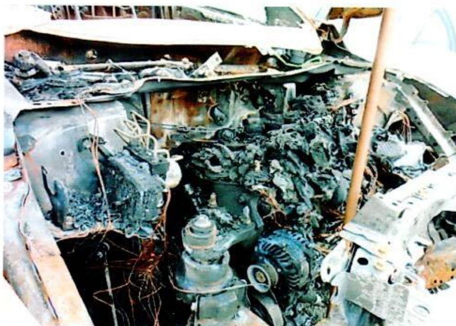
Photo 4 shows the engine compartment of the Insured Vehicle. The various parts and components within the engine compartment of the Insured Vehicle were all extensively affected by the fire. This had included the engine and transmission of the Insured Vehicle.
