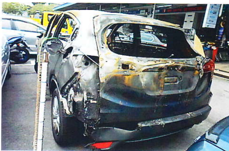
Photo 5 shows the rear left body of the Insured Vehicle. Comparing the overall extent of fire damage like the rear tyres vs the front tyres, condition of rear body panels vs front body panels etc, it would appear that the front body of the Insured Vehicle was more severely affected than its rear portion.
